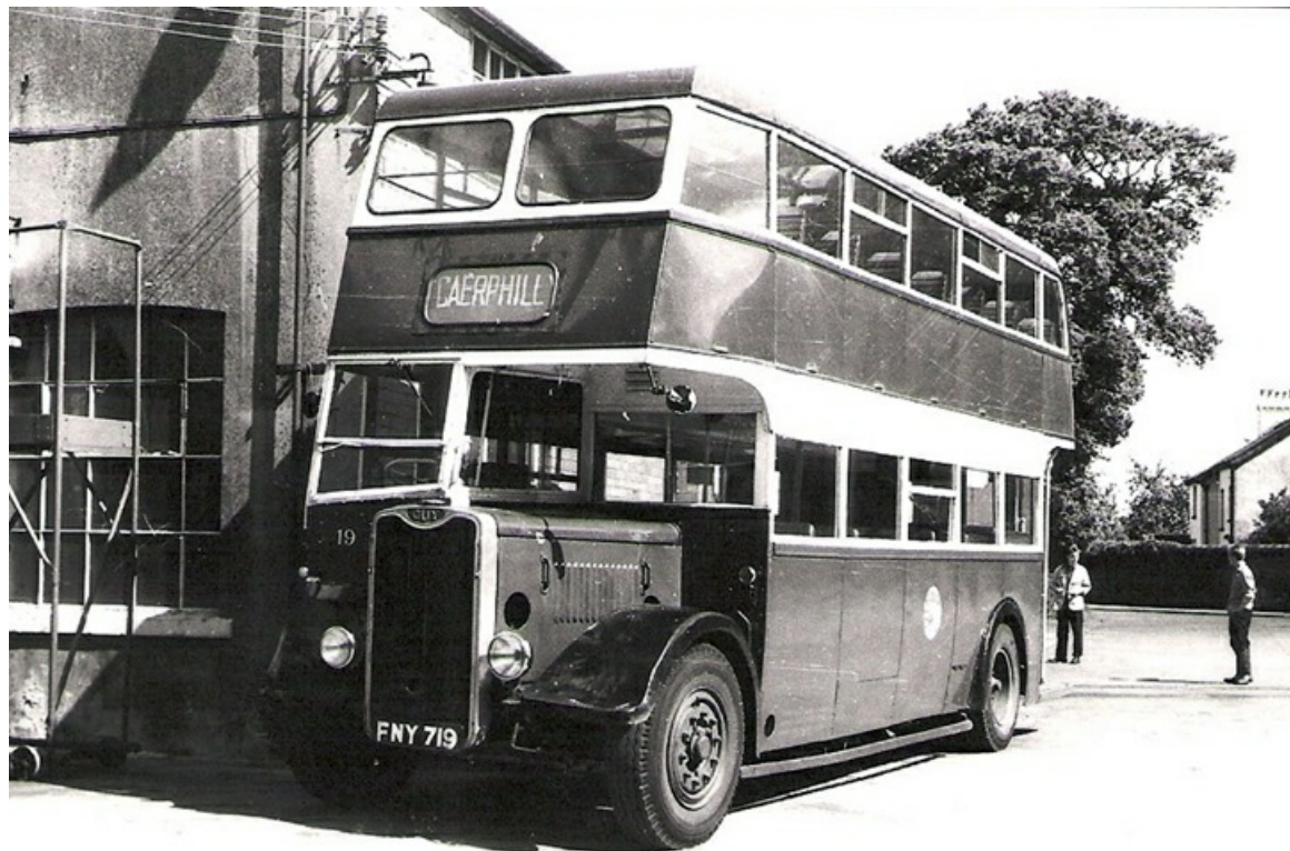
No. 19 (FNY719) was a wartime addition to the fleet in 1944. It was a Guy Arab II with Roe L27/28R bodywork that survived until 1963. (LTHL collection).
