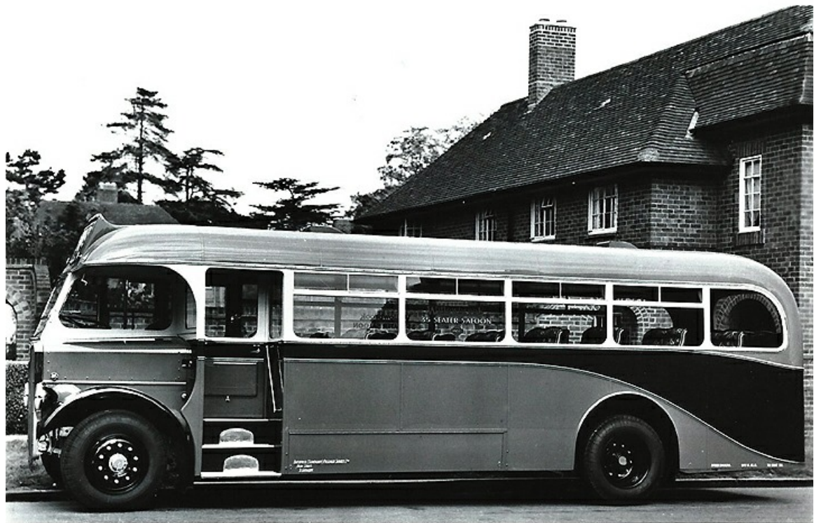
New in 1948 was No. 38 (EFW387) an AEC Regal III with Willowbrook dual-purpose 35-seat bodywork. (Bus Archive).
