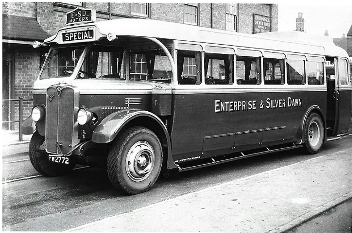
Sporting its original Harrington 32-seat rear entrance coachwork is No. 50 (FW2772), a 1932 AEC Regal. It was later re-bodied with a second-hand Willowbrook bus body. (Bus Archive).
