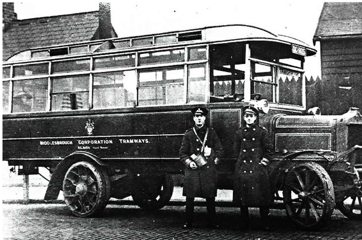
DC805 was a 1919 AEC YC chassis that had been new to the War Department but was refurbished and bodied with this Dodson B29R body. (Bus Archive).
