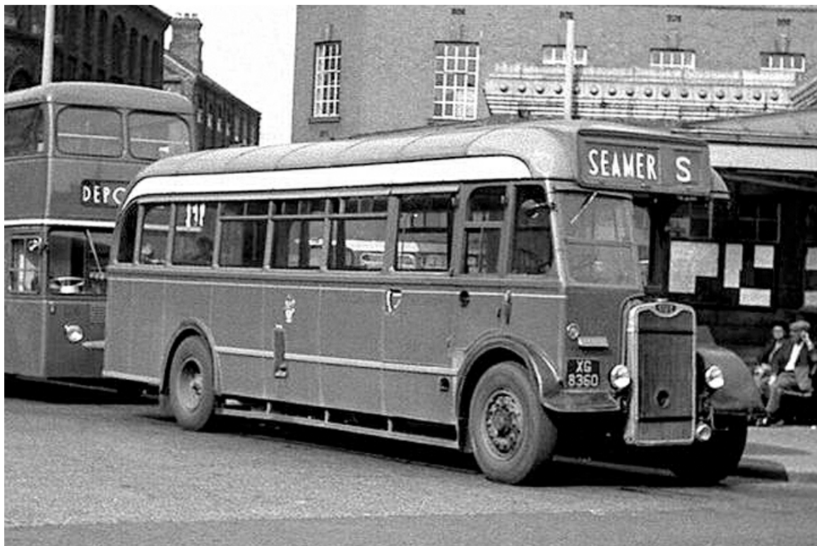
No. 3 (XG8360) was a solitary Guy Arab III with Roe B35R bodywork purchased in 1946. It was re-numbered 100 (as seen here) in 1952. (John Kaye).
