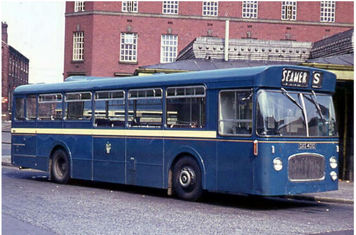
No. 1 (DXG401D) was a Leyland PSRC1/1 'Panther' with Northern Counties B44F bodywork, seen in Exchange Bus Station in August 1967. (John Kaye).
