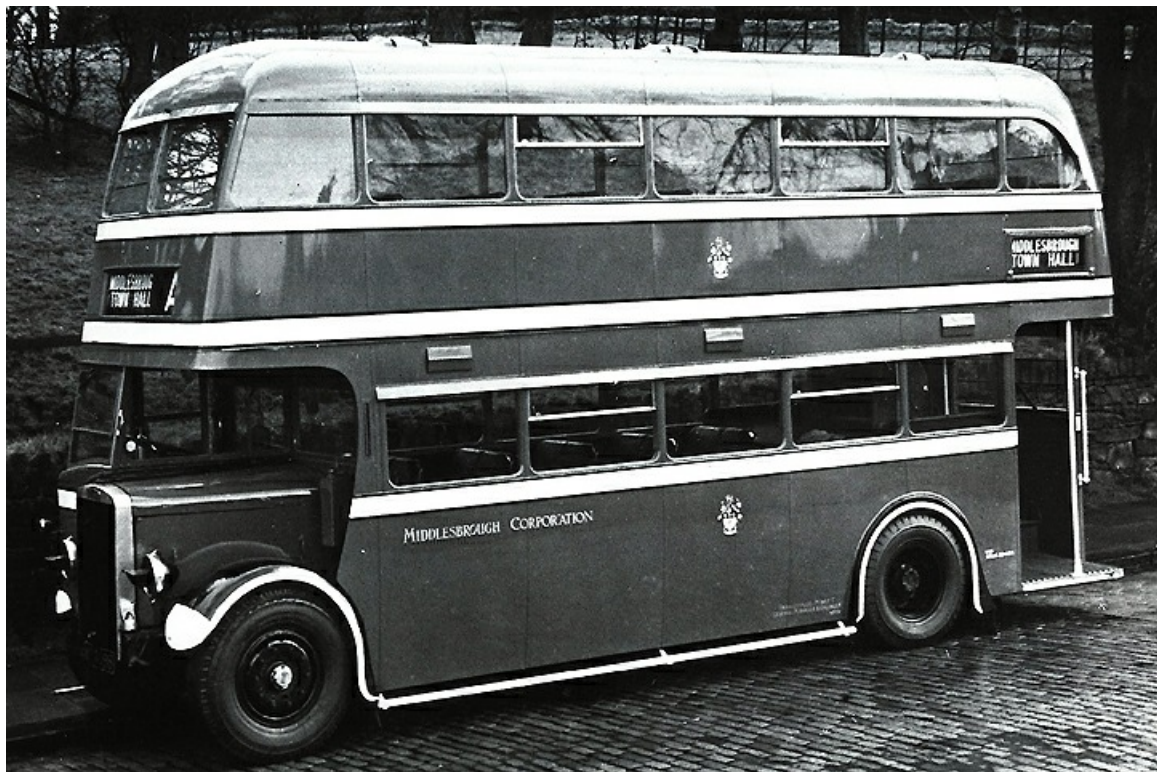
No. 93 (XG7498) was a 1940 Leyland TD7c with ECW H30/26R bodywork that was re-bodied in 1943 after suffering fire damage and was burnt out again in 1945 and withdrawn. (Bus Archive).
