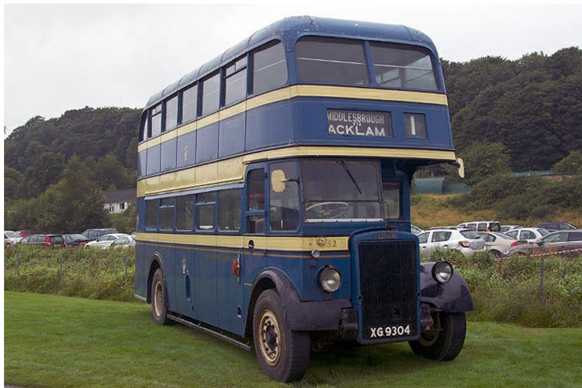
No. 52 (XG9304), a 1947 Leyland PD1A with Northern Counties L27/26R bodywork, now surviving in preservation. (Alan Hall).
