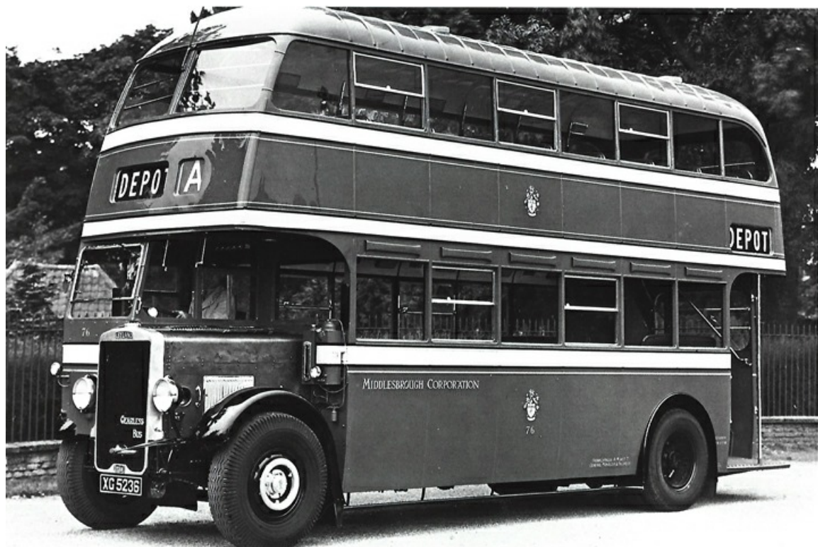
No. 76 (XG5236), a 1937 Leyland TD5c with Eastern Coach Works H30/26R bodywork. (Bus Archive).
