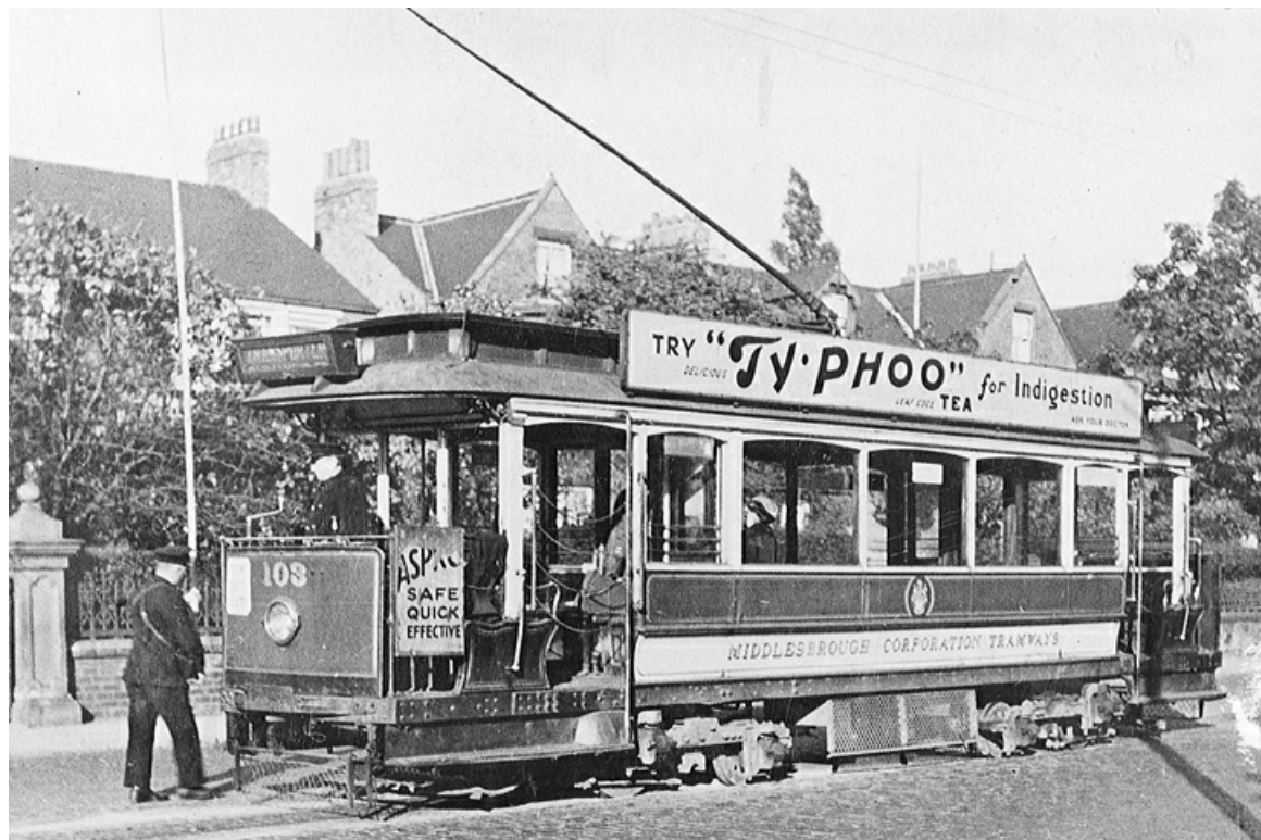
Middlesbrough car No. 103 was formerly No. 57 in the Imperial Tramways fleet inherited in April 1924. It was an 1901 Milnes-built single-deck bogie car. (LTHL collection).
