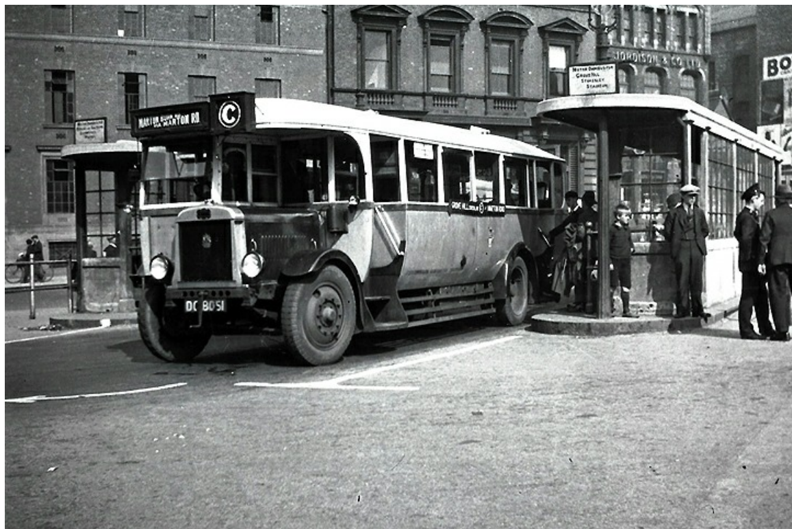
Waiting time in the original two-stand Exchange Bus Station is No. 65 (DC8051) a Leyland PLSC3 'Lion' with Edmond B32D bodywork, new in 1928. (Bus Archive).
