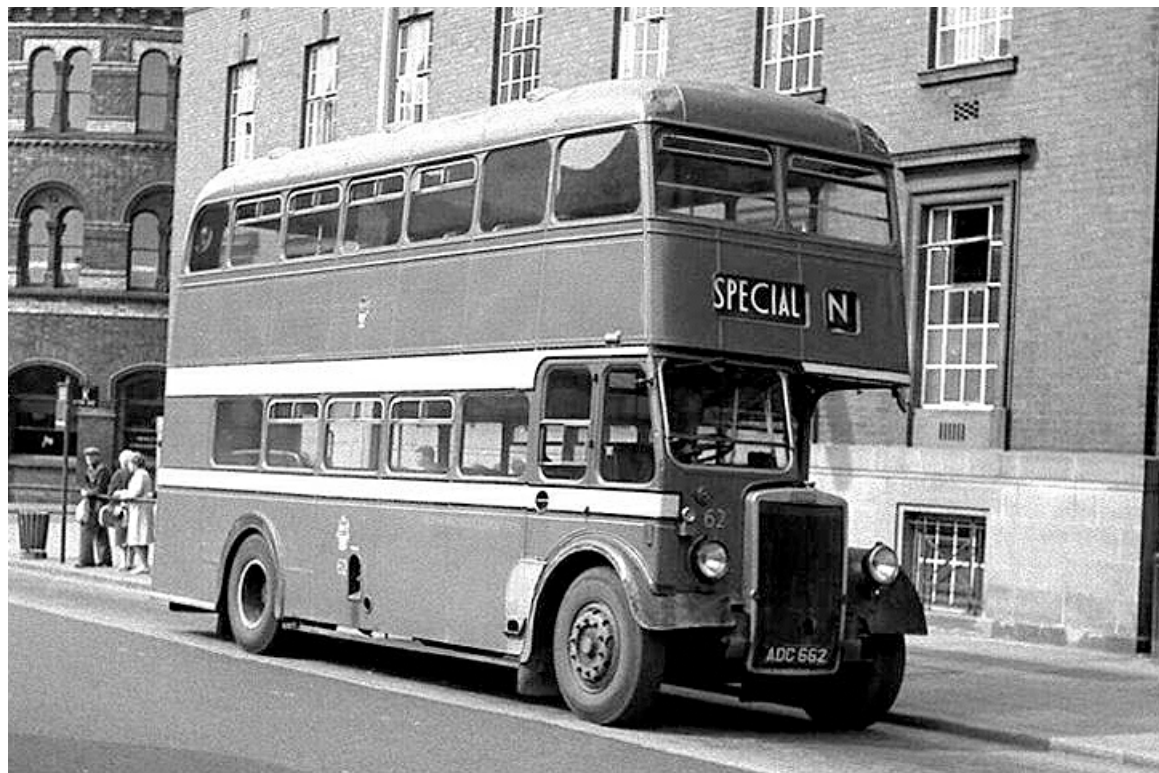
No. 62 (ADC662) a 1948 Leyland PD1/3 with ECW H30/26R bodywork seen here at Middlesbrough Exchange in May 1964. (John Kaye).
