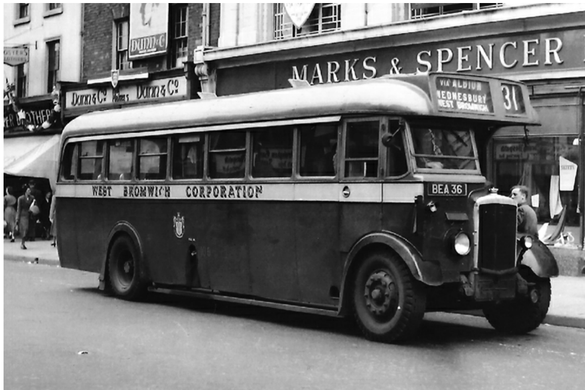
No. 106 (BEA36) was a 1941 Daimler COG6 with a B38F body by Jensen Motors, the successors to WJ Smith. It was the very last full-sized PSV body built by Jensen. (Bus Archive).
