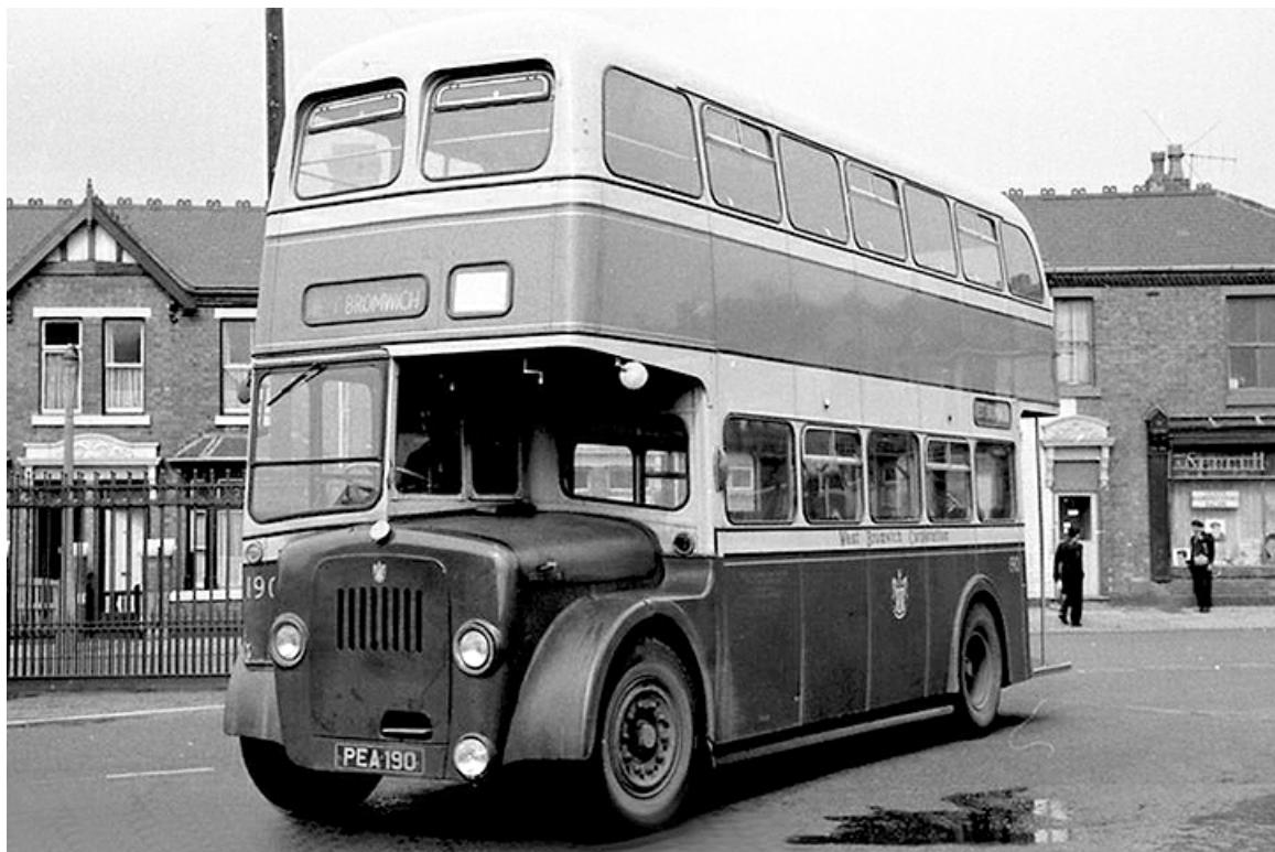
No. 190 (PEA190) was a 1957 Daimler CVG6 with Willowbrook H34/26R bodywork, a departure from the normal Metro-Cammell bodywork. (John Boylett courtesy John Kaye).
