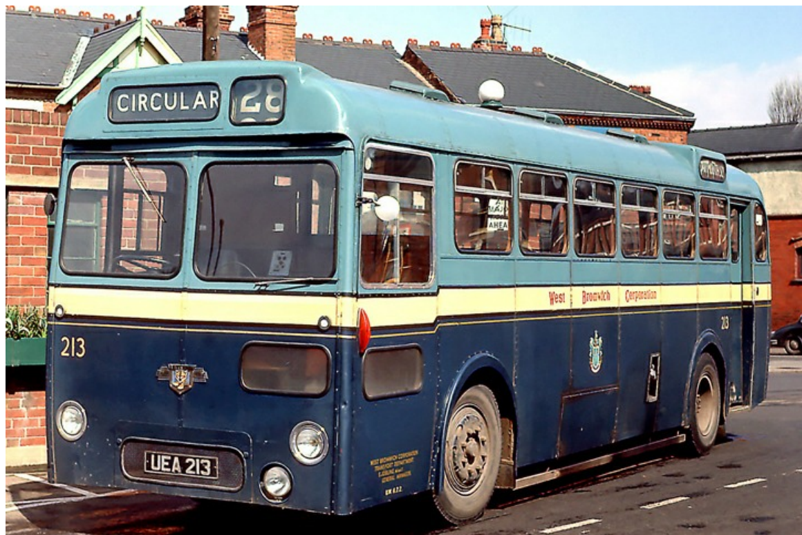
Mulliner B38RD bodywork adorns this Leyland PSUC1/4 'Tiger Cub' dating from 1958. (Alan Snatt).
