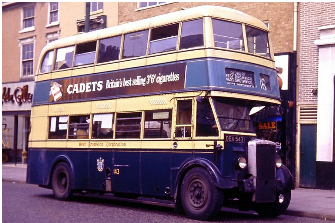
No. 143 (DEA543) was a Daimler CVG6 with Metro-Cammell H30/26R bodywork purchased in 1949 and withdrawn in 1965. (John Huddleston).
