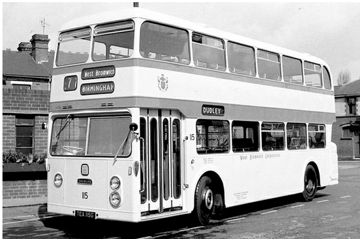
No. 115 (TEA115G) was numerically the first of the final batch of buses delivered to West Bromwich before they were absorbed into West Midlands PTE. It was a 1969 Daimler CRG6LX with ECW H45/28F bodywork. (John Boylett courtesy John Kaye).
