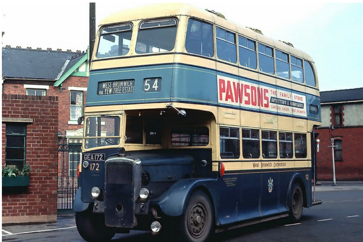
No. 172 (GEA172) was a 1952 Daimler CVG6 with Weymann H30/26R bodywork that survived long enough to pass to West Midlands PTE in 1969. (Alan Snatt).
