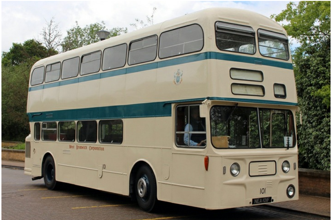
No. 101 (NEA101F) was a replacement for the original No. 101 which was destroyed by fire whilst at the coachbuilders. It was a Daimler CRG6LX with MCW H42/31F bodywork. (John Huddleston).
