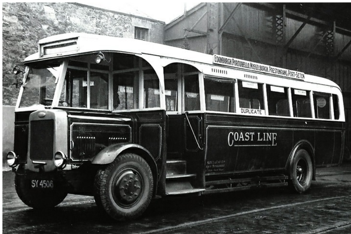
SY4506 was one of two Bristol B chassis with Bristol B32F bodywork purchased in 1931. (Bus Archive).
