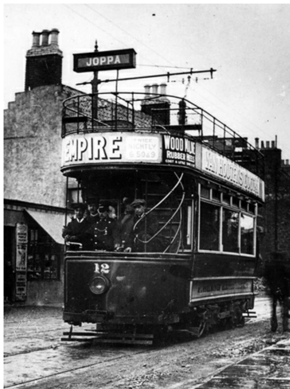
Car 12 was built in 1905 by Brush and seated 57. It was fitted with a top-cover in 1909. (LTHL collection).
