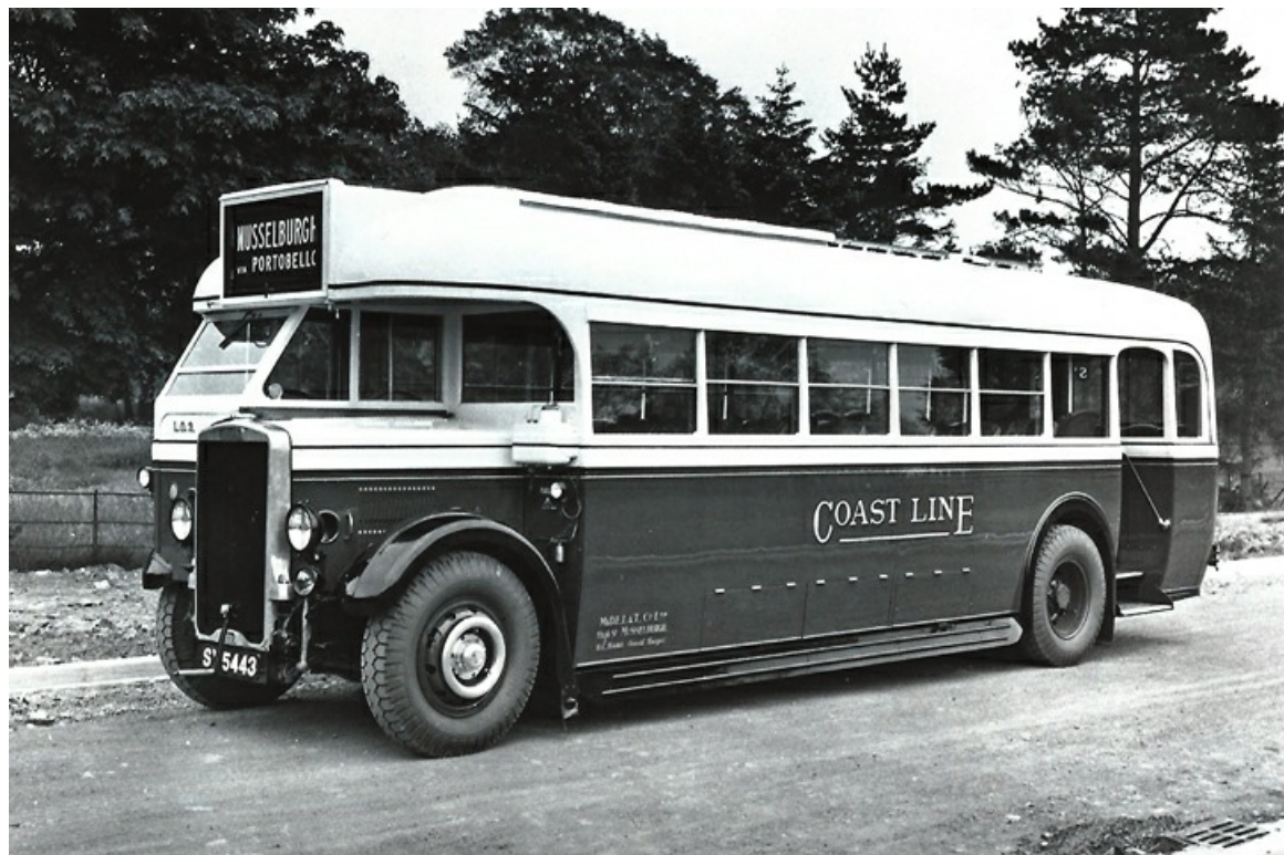
No. L03 (SY5443) was a Leyland TS7 with Brush B32R bodywork new in 1935. It passed to SMT in 1/37 where it was numbered H146. (Bus Archive).
