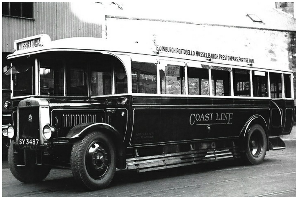
SY3487, a 1928 Leyland PLSC3 with Leyland B31R bodywork used on the Edinburgh-Portobello-Musselburgh-Prestonpans-Port Seton route of the Musselburgh & District Electric Light & Traction Co using the Coast Line fleetname. (Bus Archive)
