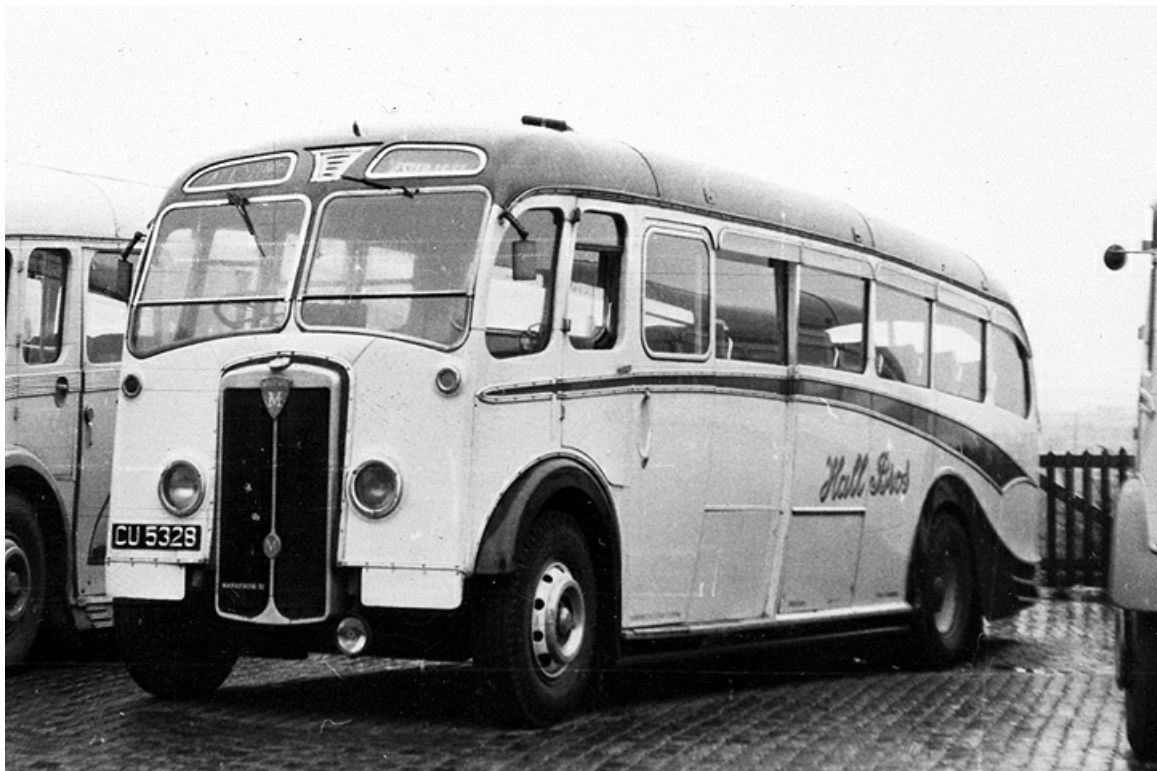
CU5328 was a 1950 Maudslay Marathon III with Gurney Nutting 33-seat full-front coachwork. (Geoff Stainthorpe).
