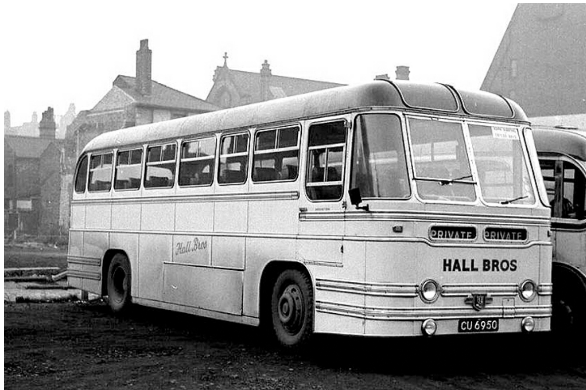
Strachan's 'Everest' 41-seat coachwork adorns this 1954 Leyland PSUC1/2 'Tiger Cub', pictured here in December 1957. (John Kaye).
