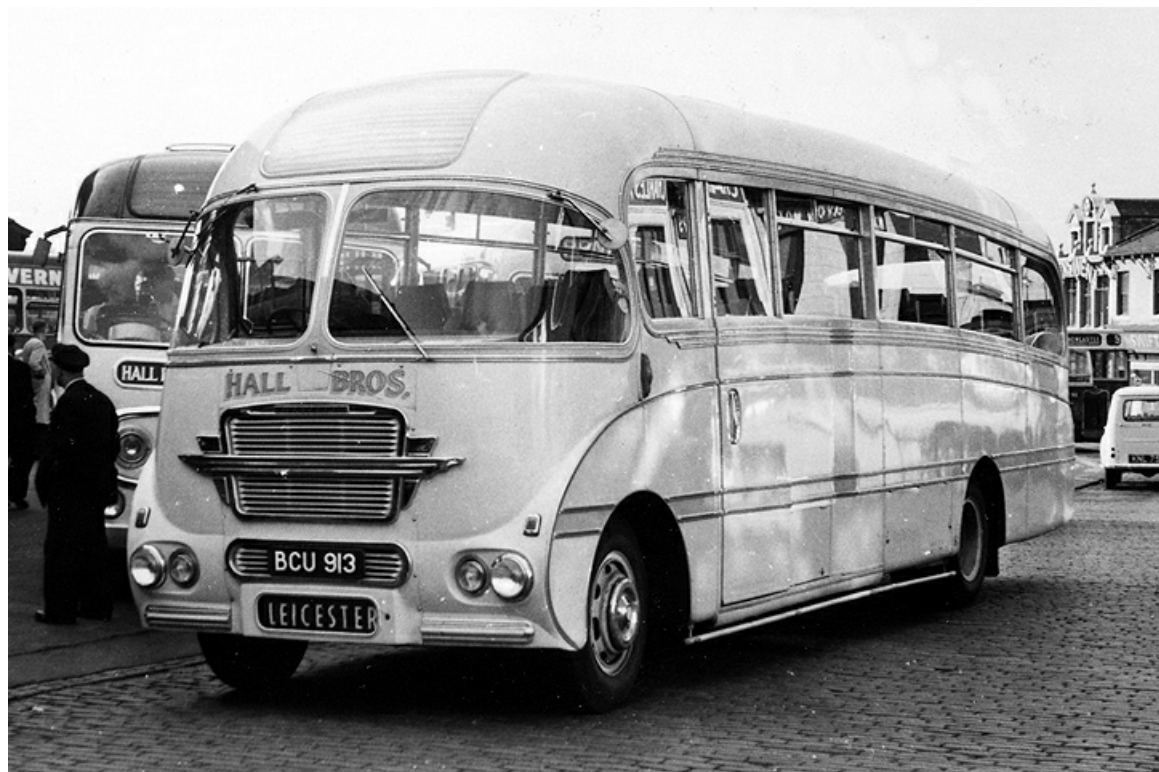
BCU913 spent a little over six months in the fleet and was a 1959 Bedford SB1 with Burlingham C41F coachwork. (Geoff Stainthorpe).
