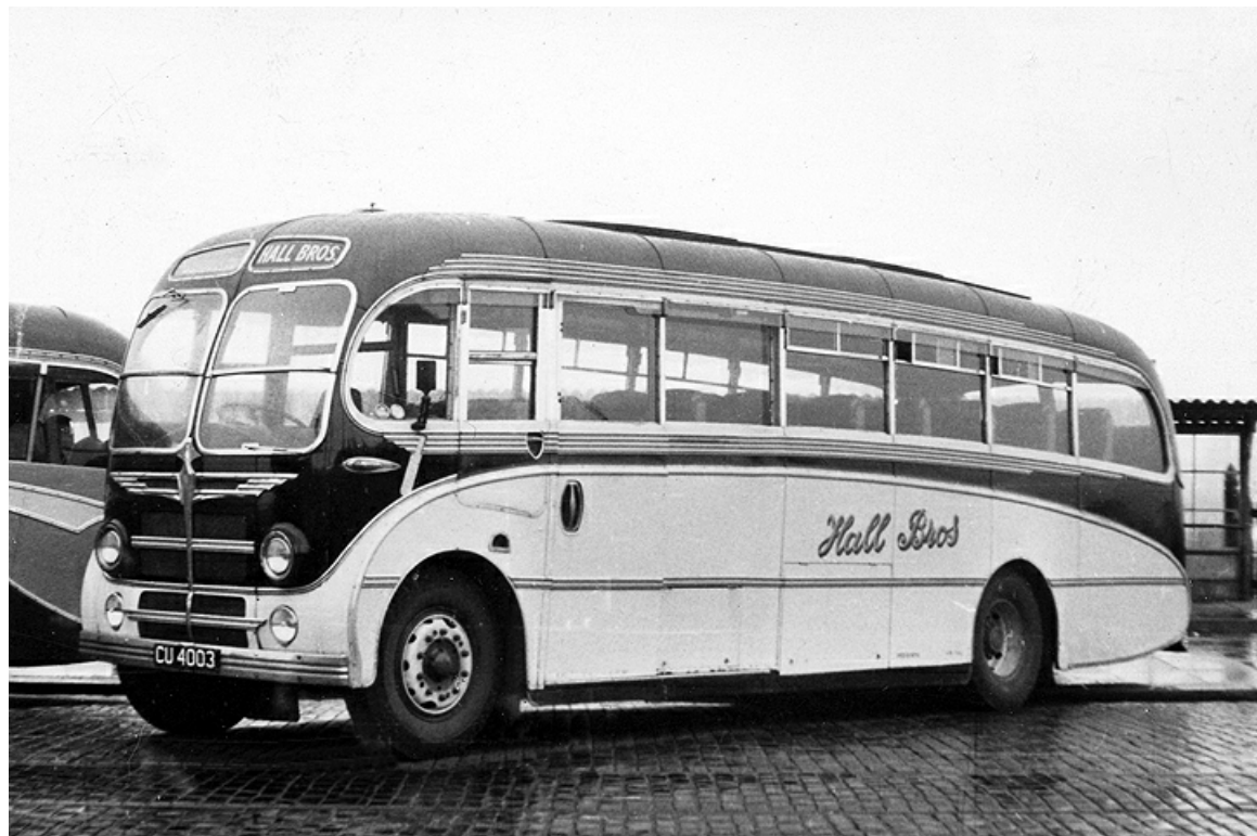
CU4003 was a 1938 AEC Regal, that originally carried a Mulliner C32F body but was re-bodied with the Burlingham C35F body shown here. (Geoff Stainthorpe).
