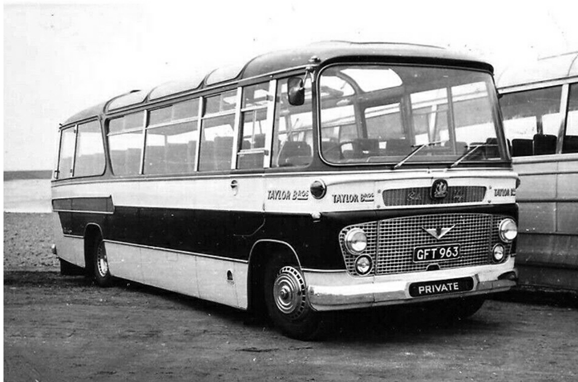
GFT963 was a 41-seat Duple 'Bella Vega' bodied Bedford SB8 of 1963. (Geoff Stainthorpe).
