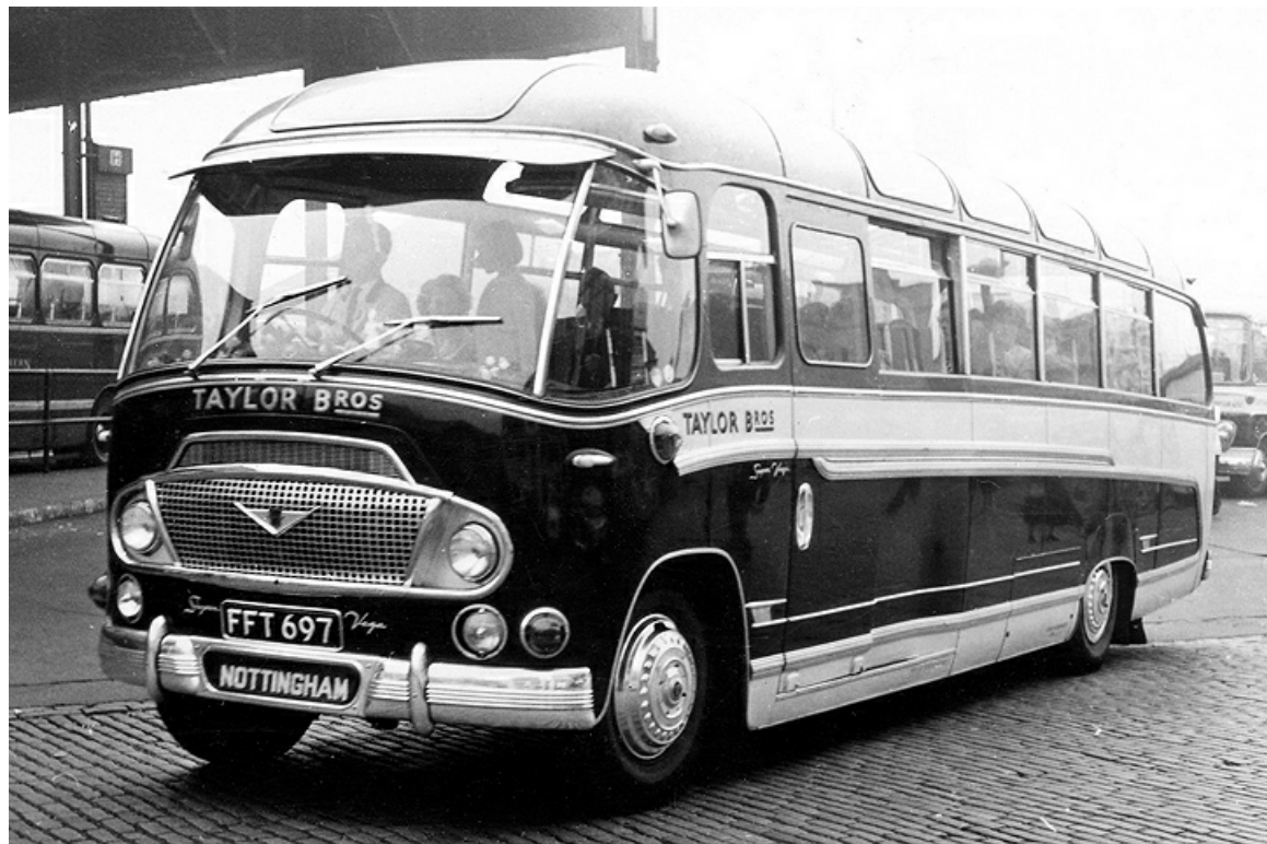
FFT697 was a Bedford SB5 with Duple 'Super Vega' 41-seat coachwork dating from 1962. (Geoff Stainthorpe).
