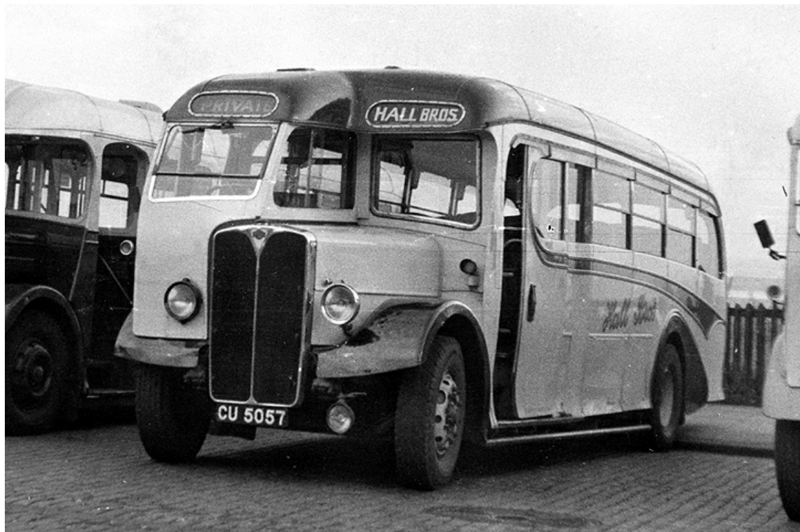
CU5057 was a 1948 AEC Regal III with Burlingham 33-seat half-cab coachwork. (Geoff Stainthorpe).
