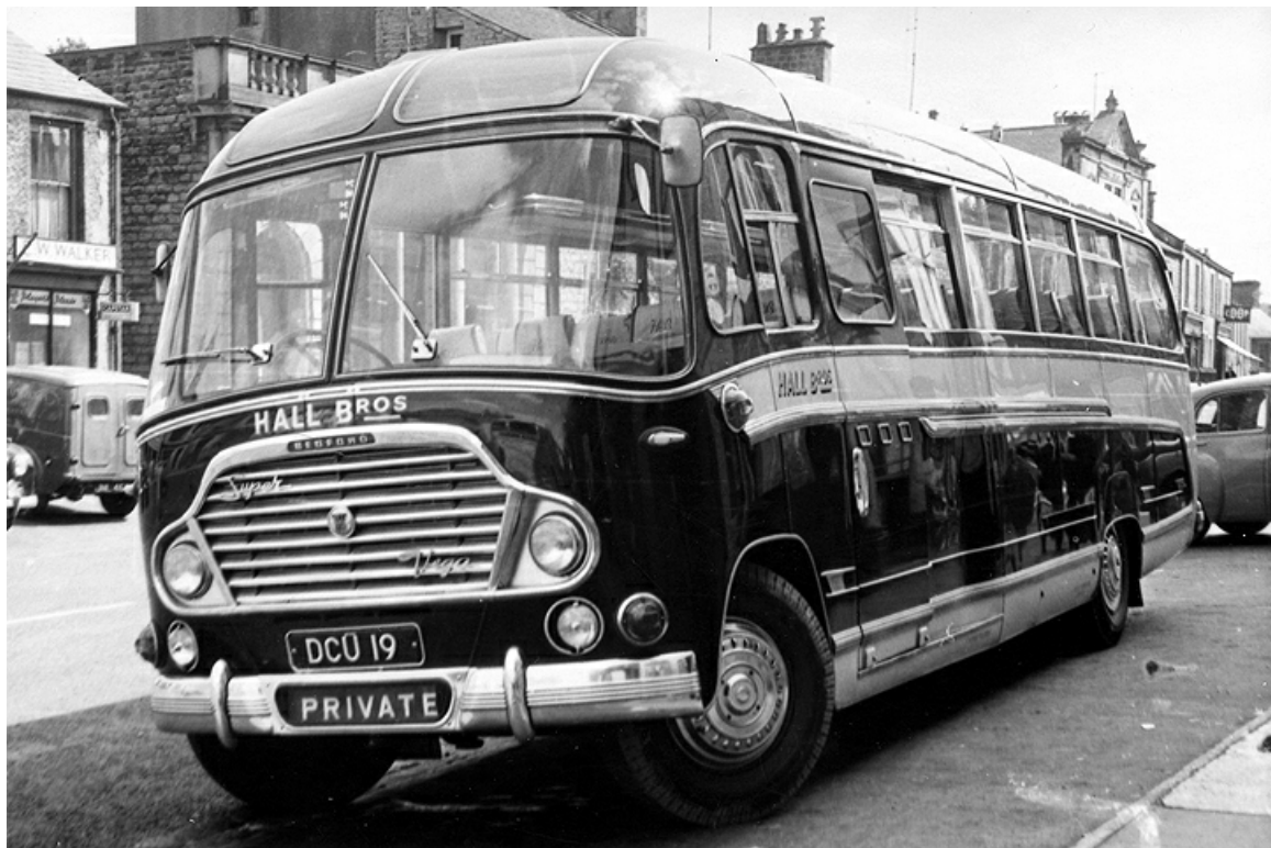
Duple 'Super Vega' 41-seat coachwork sits on DCU19, a Bedford SB1 chassis dating from 1960. (Geoff Stainthorpe).
