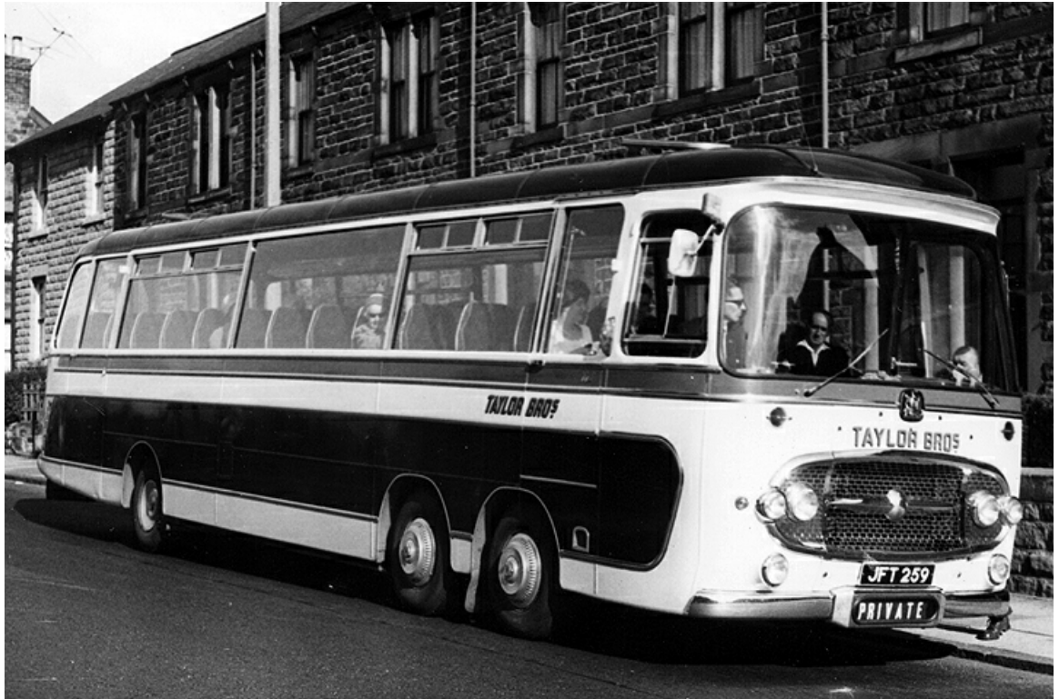
JFT259 was a solitary Bedford VAL14 added to the fleet in 1964 and carried Plaxton 52-seat coachwork. (Geoff Stainthorpe).
