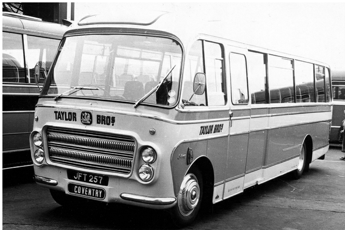
Dating from 1964 is JFT257, a Bedford SB5 with Plaxton 41-seat coachwork. (Geoff Stainthorpe).
