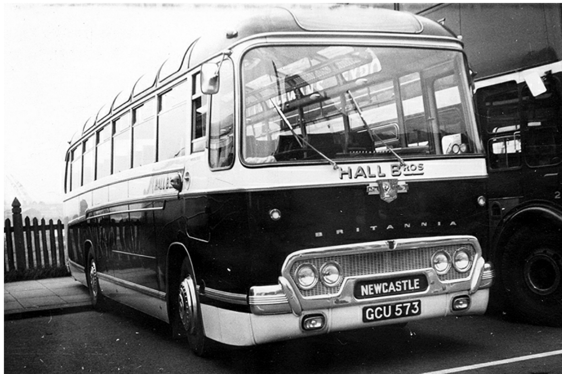
GCU573 was a 1962 Leyland L2 'Leopard' with Duple 'Britannia' 43-seat coachwork. (Geoff Stainthorpe).
