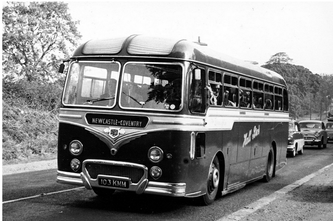
103KMM was an ex-Duple demonstrator that carried 'Donnington' 43-seat coachwork on a Leyland PSUC1/2 'Tiger Cub' chassis and was new in 1955. (Geoff Stainthorpe).
