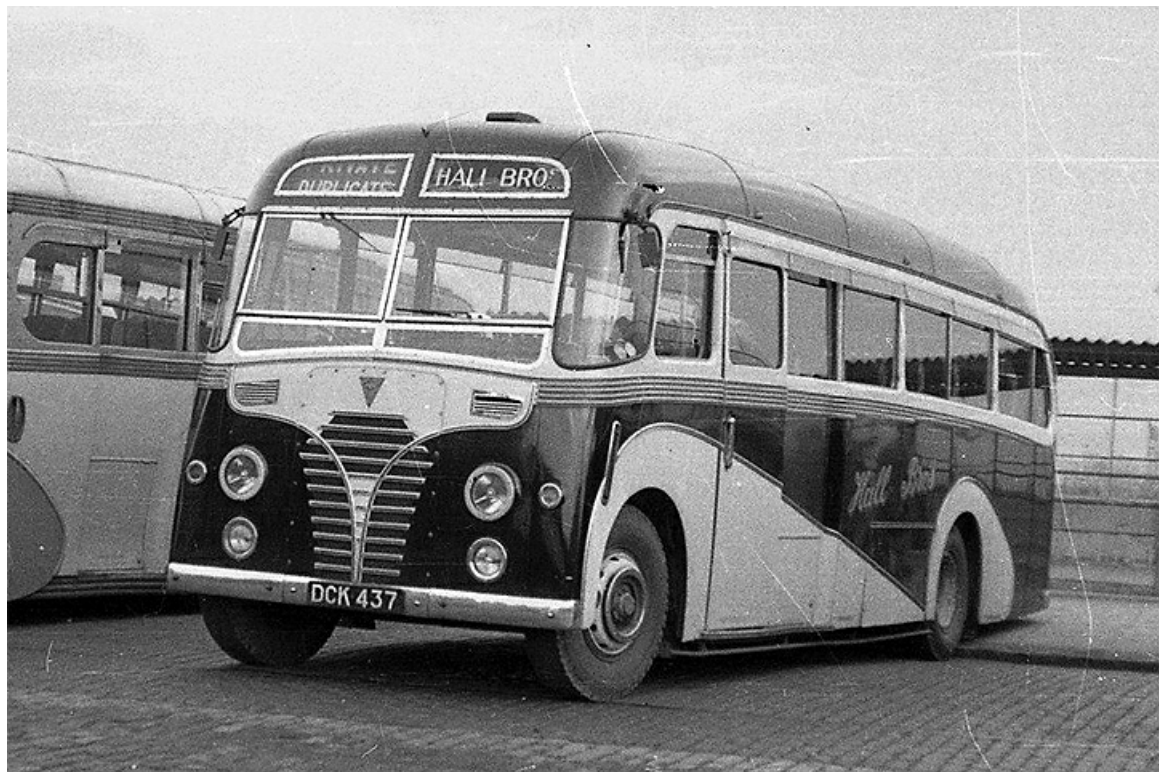
A second-hand purchase in 1955 was DCK437, a 1950 AEC Regal III with Harrington FC35F coachwork that had been new to Premier Motor Tours of Preston. (Geoff Stainthorpe).
