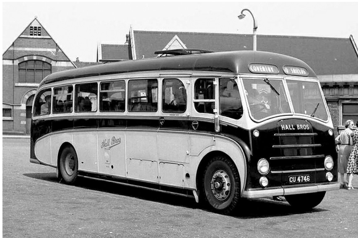
1947 Burlingham-bodied Leyland PS1/1 'Tiger' CU4746 was rebuilt to full-front in 1955 by Picktree as shown. (John Kaye).
