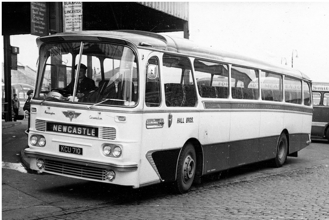
New in 1964 was KCU710, a solitary AEC Reliance with Harrington 51-seat coachwork. (Geoff Stainthorpe).
