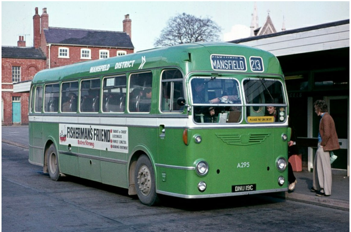
No. A295 (DNU19C) was a 1965 Bristol MW6G with ECW 43-seat dual-purpose bodywork ex-Midland General in 1965, seen here in Newark Bus Station. (Richard Simons).
