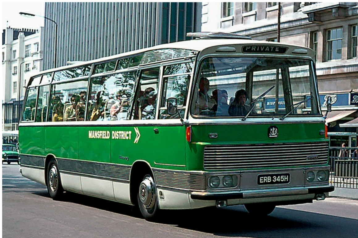
No. MC28 (ERB345H), seen here on a private hire to London in 1973, was a 1970 Bedford VAM70 with Duple 41-seat coachwork that was originally numbered 228. (Alan Snatt).
