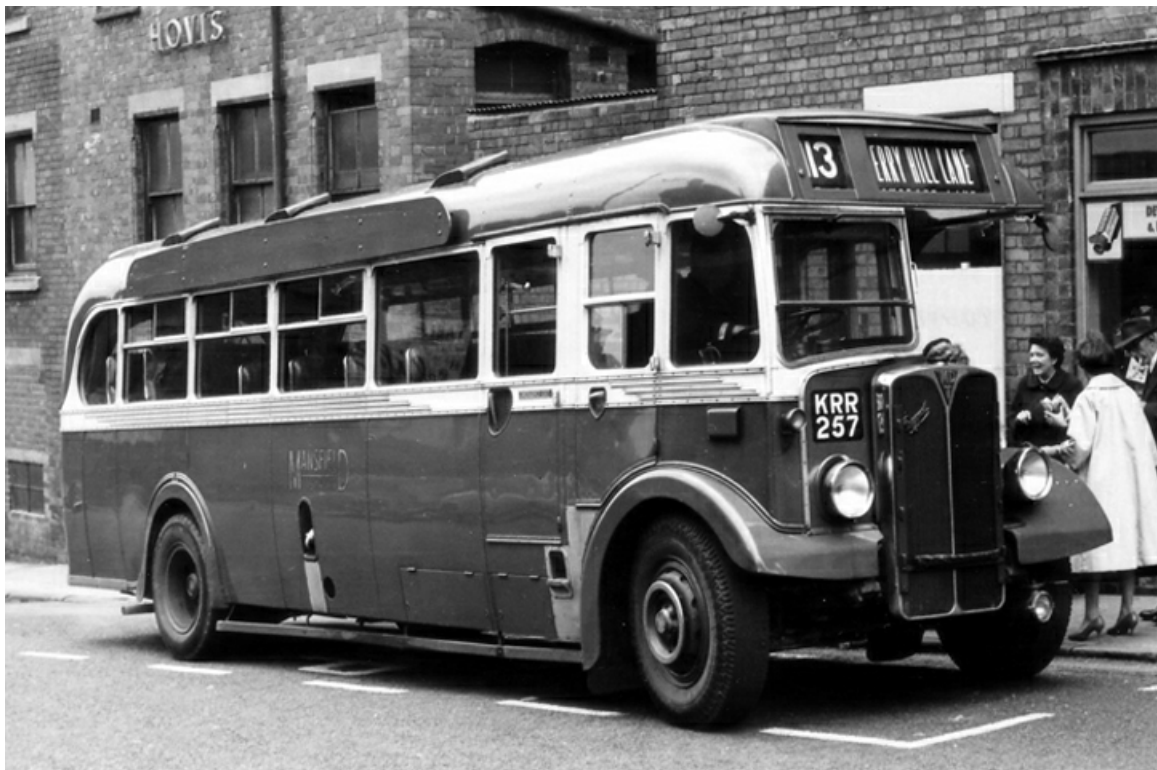
No. 11 (KRR257) was a 1949 AEC Regal III with with Weymann 43-seat dual-purpose bodywork, seen here on stage carriage duties. (LTHL collection).
