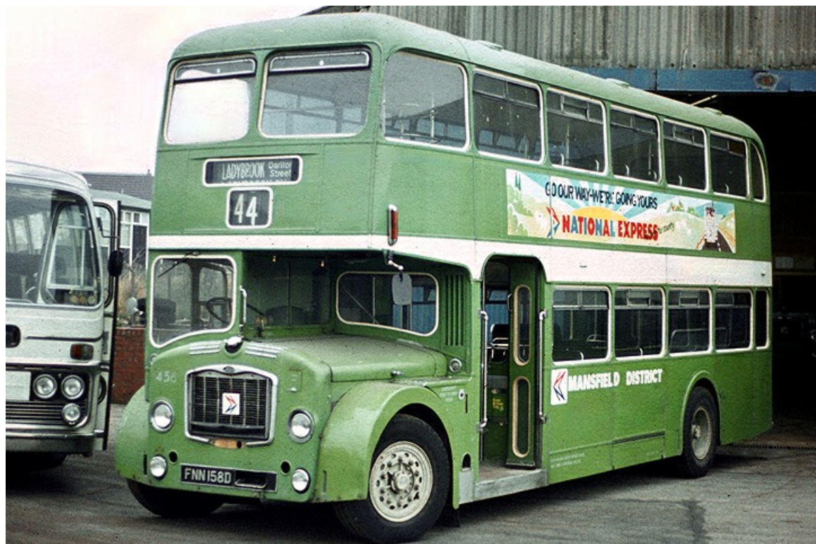
Seen here after transfer to East Midland is No. 456 (FNN158D), a Bristol FLF6G with ECW H38/32F bodywork that was numbered B456 whilst with Mansfield District. (Richard Simons).
