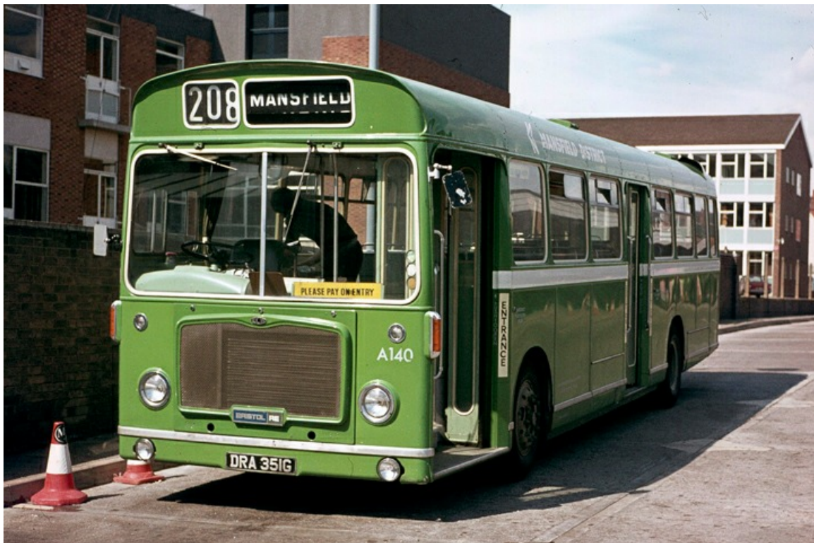
A140 (DRA351G), a 1969 Bristol RELL6G with ECW 44-seat dual-door bodywork, seen here laying over in Newark Bus Station. (Richard Simons).
