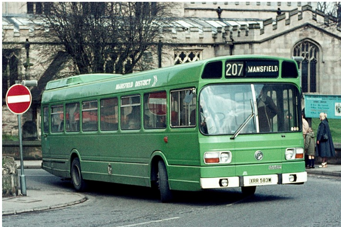
No. A583 (XRR583M) was a 1973 Leyland National with 44-seat dual-door bodywork. (Richard Simons).
