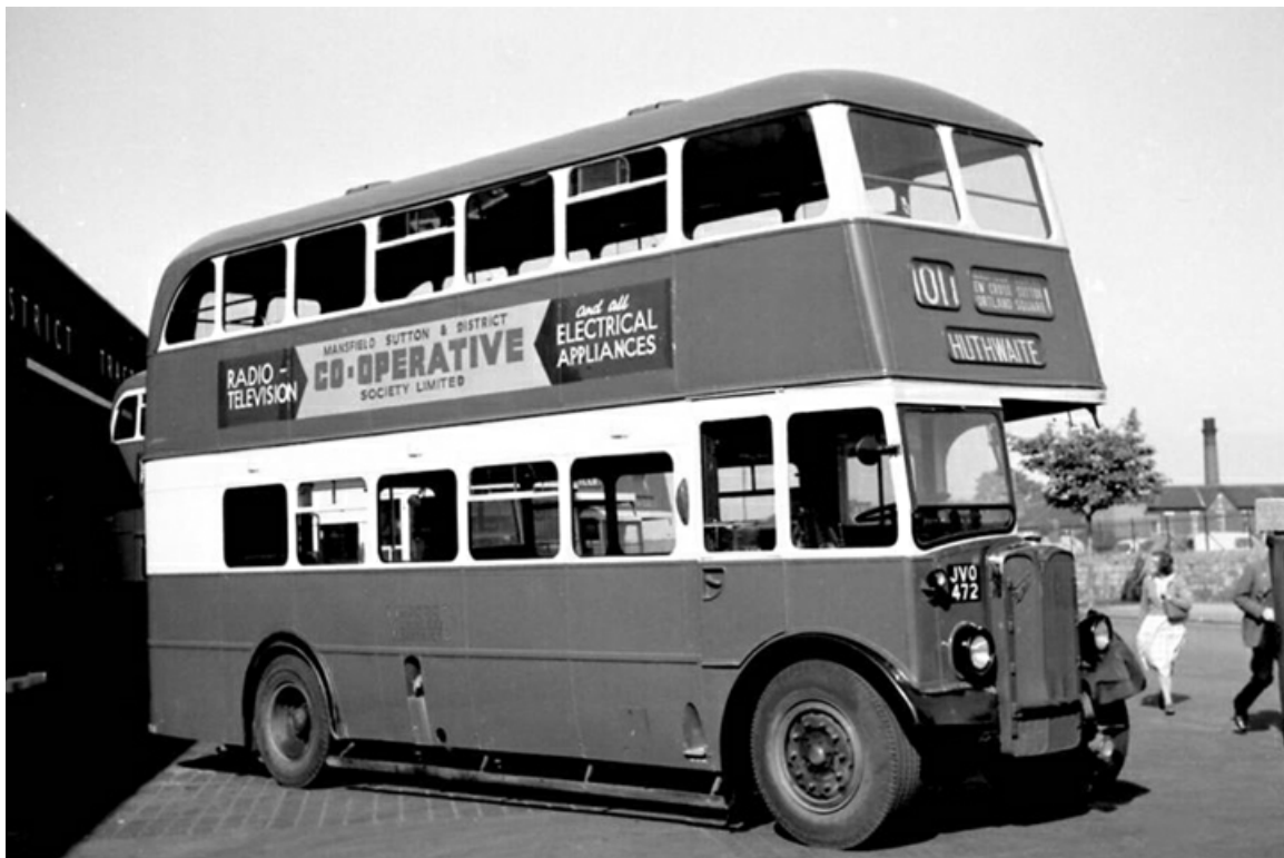
No. 162 (JV0472) was a 1948 AEC Regent III with Crossley H30/26R bodywork that came with the business of Red Bus Services of Mansfield Woodhouse in 1957. (John Boylett courtesy John Kaye).
