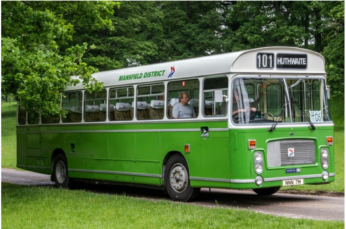
Now in preservation is Mansfield District No. MC7 (NNN7M), a 1974 Bristol RELH6L with ECW 47-seat dual-purpose bodywork. (Len Wright).
