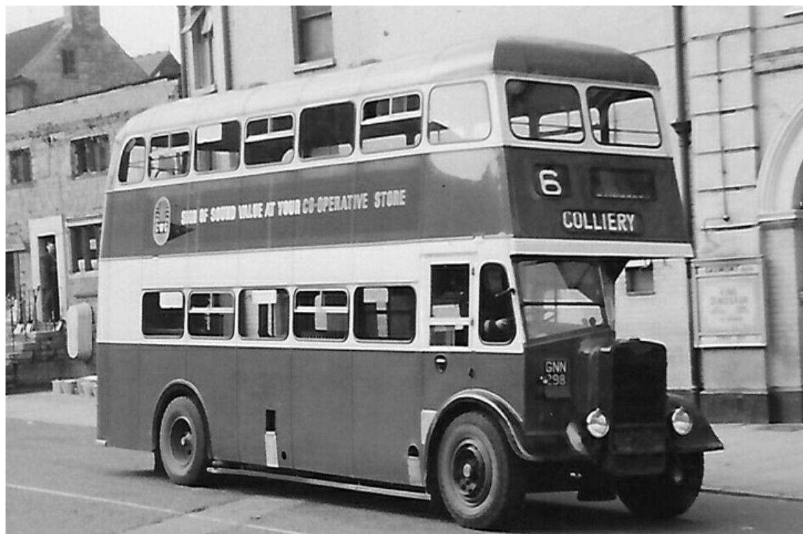
No. 110 (GNN2988) was a 1944 Guy Arab II with Northern Counties H30/26R bodywork. (RHG Simpson).
