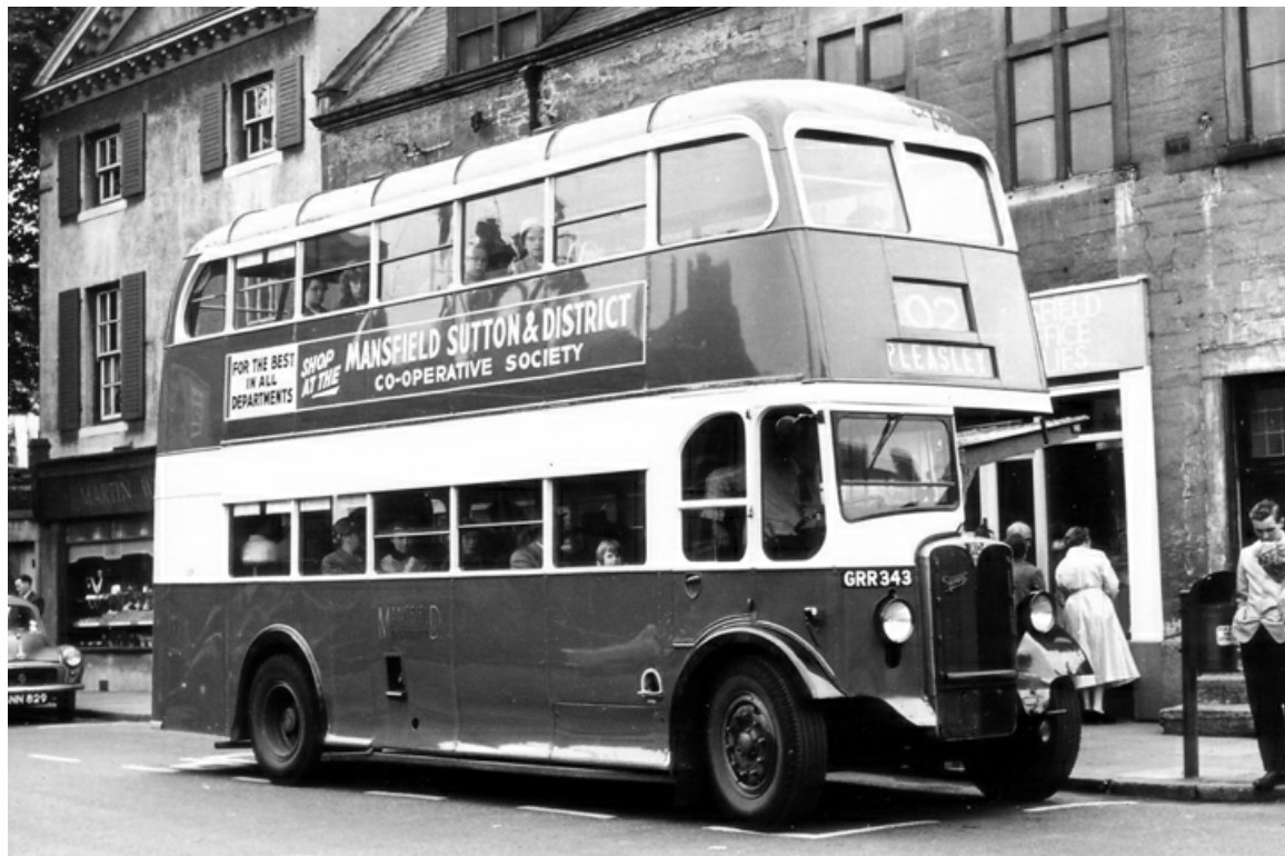
No. 121 (GRR343) was a 1946 AEC Regent II with Weymann H30/26R bodywork about to depart for Pleasley. (LTHL collection).
