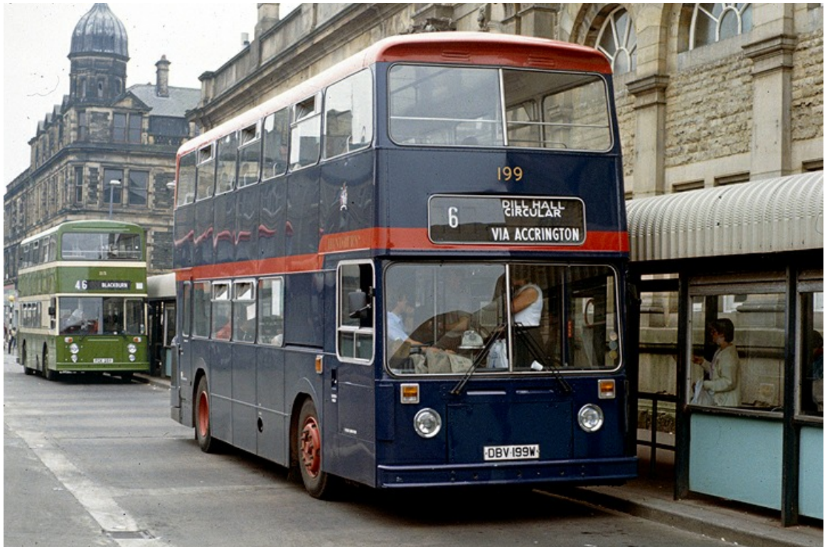
No. 199 (DBV199W) was a Leyland AN68A/1R with East Lancs H45/33F bodywork new in 1980. (Richard Simons).
