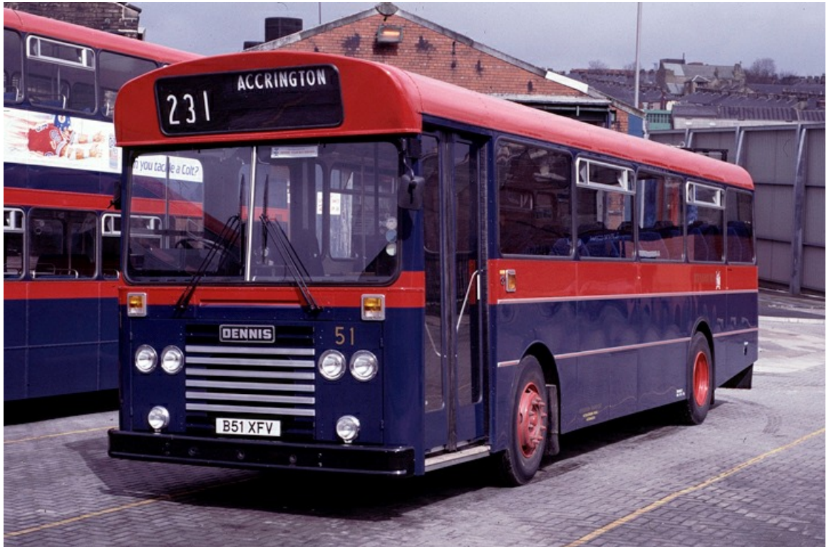
No. 51 (B51XFV) dating from 1985 was a Dennis Falcon with East Lancs DP43F bodywork. (Richard Simons).
