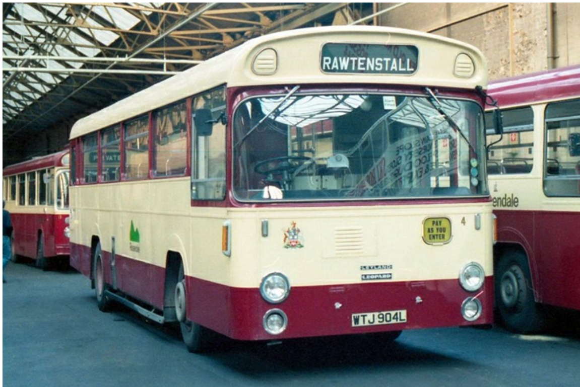
No. 4 (WTJ904L) was a Leyland PSU4B/2R 'Leopard' with East Lancs B46F bodywork new in 1973 and seen here in the depot. (Joe Gornall courtesy Malcolm Jones).
