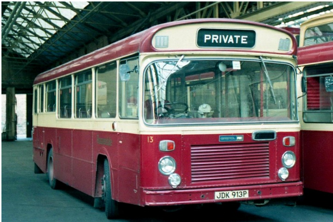
No. 13 (JDK913P) was one of four Bristol RESL6L's delivered in 1975, this one had B45F bodywork by East Lancs. (Joe Gornall courtesy Malcolm Jones).
