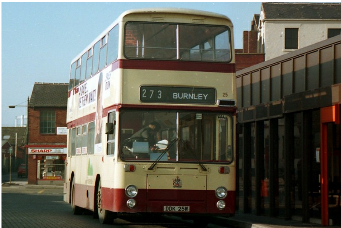
Leyland AN68B/1R No. 25 (DDK25W) with East Lancs H43/32F bodywork dating from 1979. (Joe Gornall courtesy Malcolm Jones).
