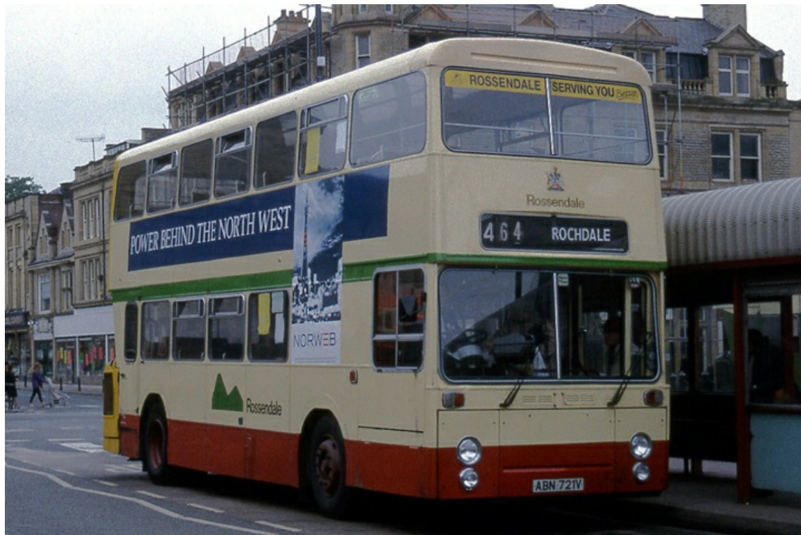
No. 21 (ABN721V) was a 1969 Leyland AN68A/1R with East Lancs H43/32F bodywork that passed to Rossendale Transport Ltd in 10/86. (John Law).
