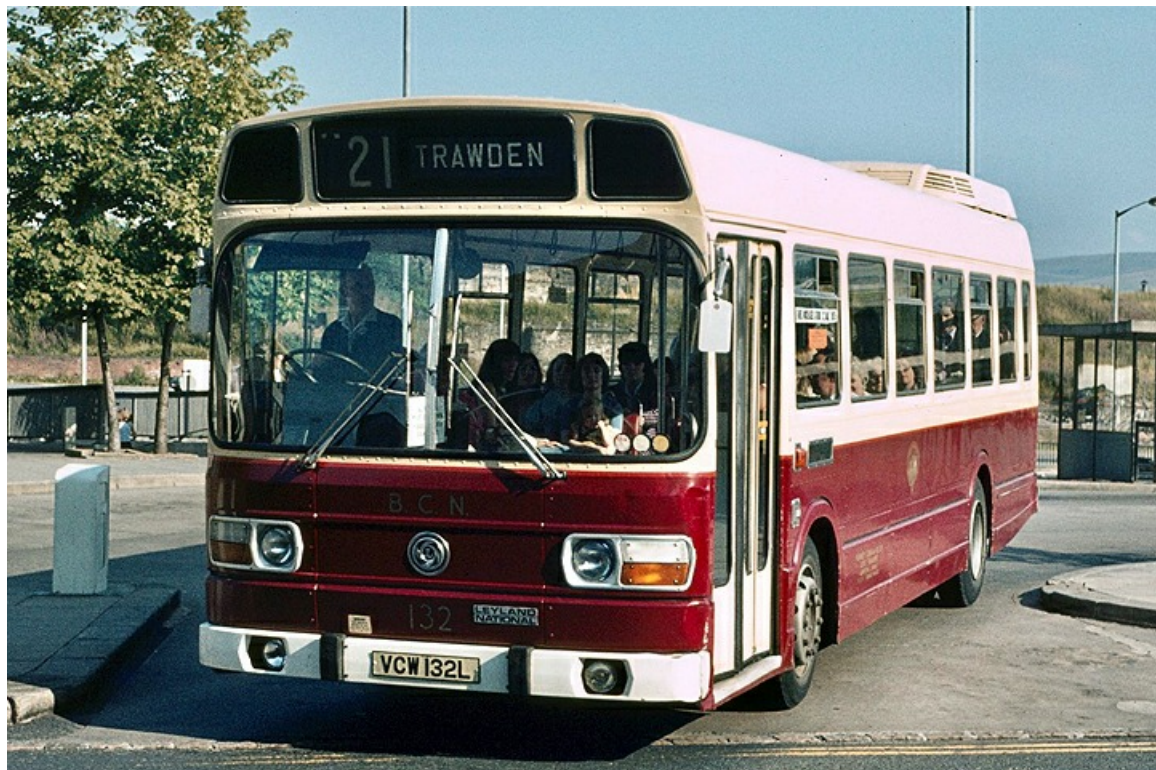
New in 1973 was No. 132 (VCW132L), a Leyland National which was of integral construction and carried a B44F body. (Richard Simons).
