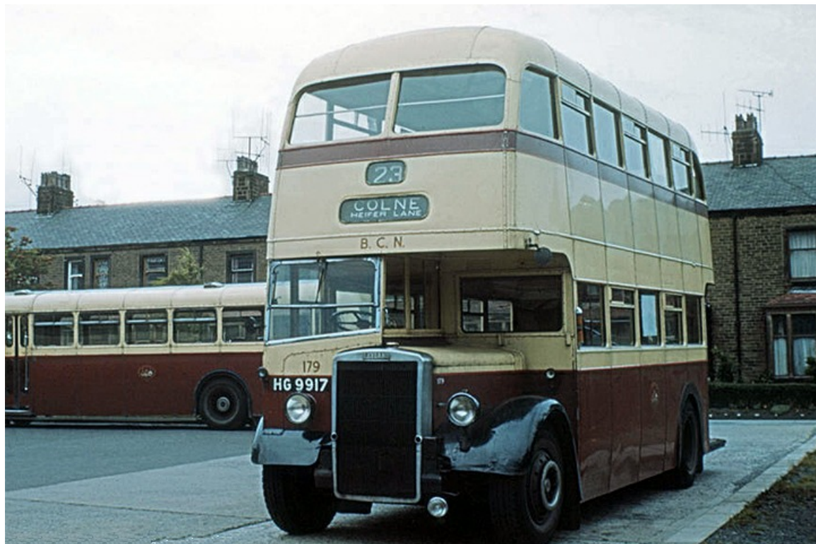
No. 179 (HG9917) was a 1948 Leyland PD2/3 with Northern Counties H30/26R bodywork, seen here at Colne depot in 1966 a couple of years before it was withdrawn. (John Stringer).
