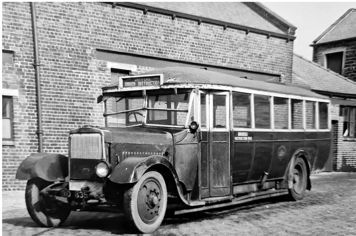
Former Nelson No. 14 (TD8354) was in use as a 'Driver Instruction Bus' when photographed in March 1954. It was a 1927 Leyland PLC1 'Lioness' with Leyland B26F bodywork. (Chris Heaps).
