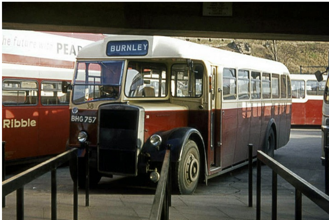
No. 38 (BHG757), a 1953 Leyland PS2/14 with East Lincs B35R bodywork, rebuilt to B35F in 1959, seen in Burnley Bus Station in 1974. (John Stringer).
