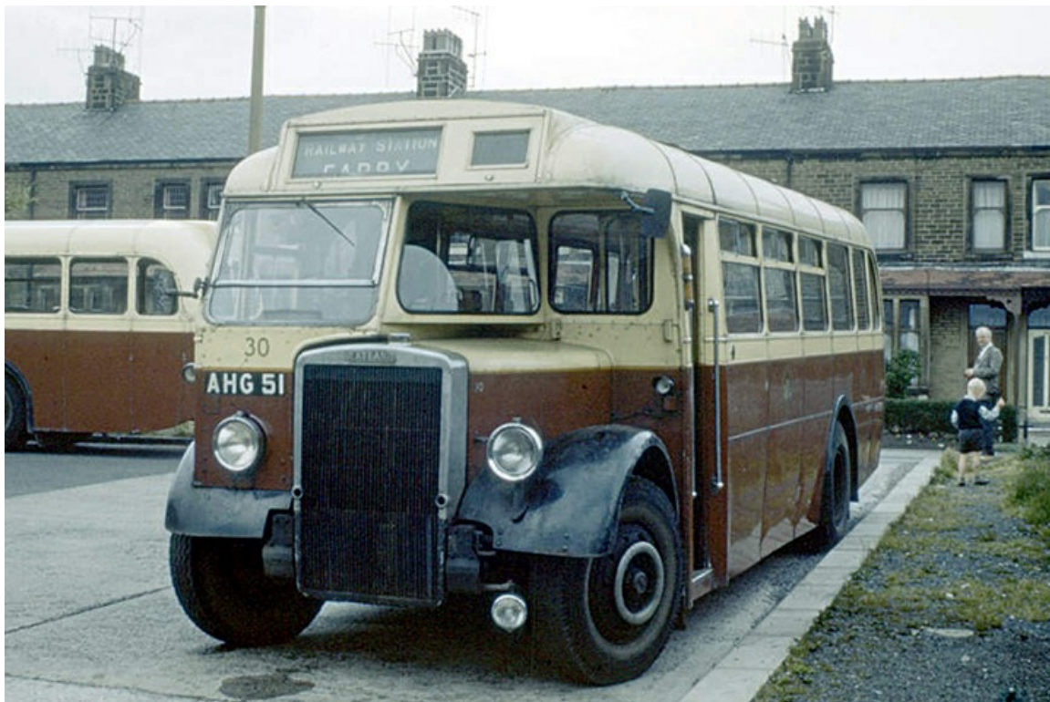
No. 30 (AHG51) was a 1950 Leyland PS1 with Massey B35R bodywork that was converted to forward entrance for one-man operation in 1959. (John Stringer).
