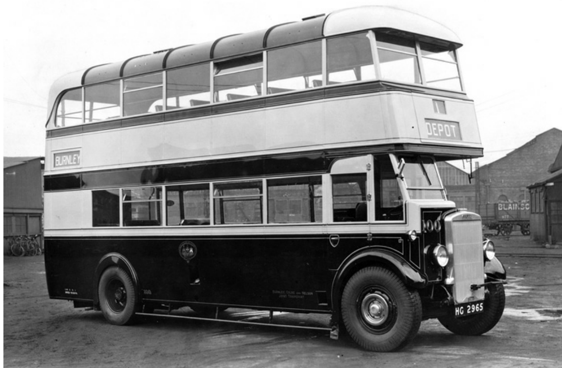
No. 100 (HG2965) was a 1934 Leyland TD3c with English Electric H29/22R bodywork. Note the unusual offside destination indicator. (GEC Collection courtesy David Beilby).
