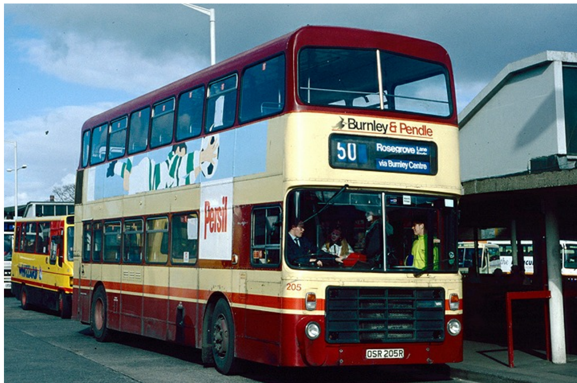
No. 205 (OSR205R) was one of a number of Bristol VRT,s with Alexander H49/34D bodywork purchased from Tayside Regional Council in 1982; all were converted to H49/35F in 1982 or 1983. (Richard Simons)
