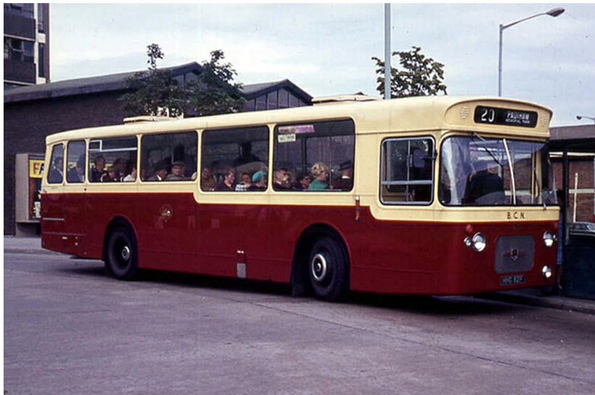
No. 82 (HHG82F) a 1968 Northern Counties B50F-bodied Leyland PSUR1/1R 'Panther' stands in Burnley Bus Station in August 1968. (John Kaye).
