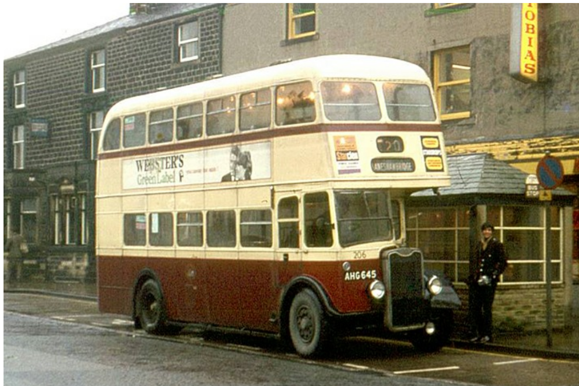
No. 206 (AHG645), a 1951 Guy Arab III with East Lancs H31/26R bodywork, seen here at the Commercial Hotel in Keighley Road, Colne. (Brian Pask).
