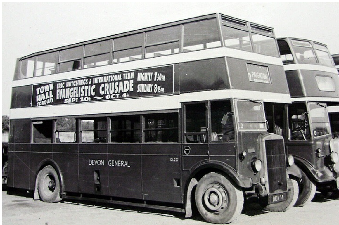
1936 Leyland TD4 No. DL227 (BDV14) originally had a Beadle 52-seat body which was replaced in 1945 by this Northern Coachbuilders 56-seat body. (LTHL collection).
