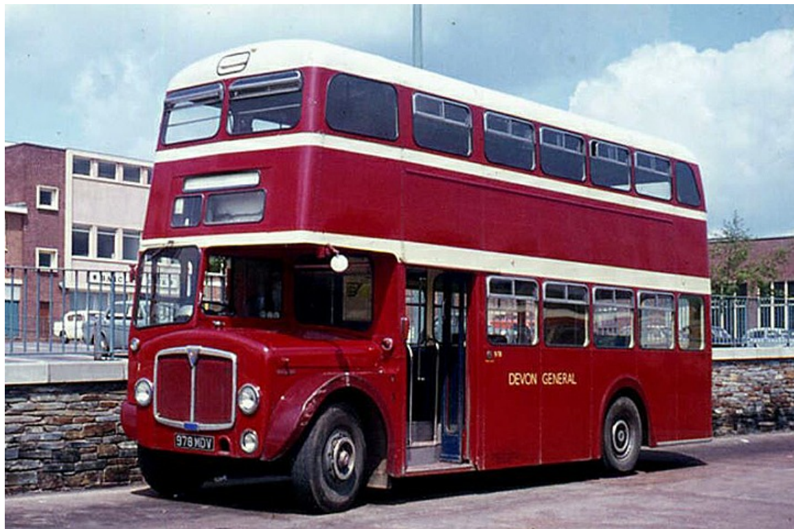
No. 978 (978MDV) was one of the first batch of forward entrance AEC Regent V's with MCCW 59-seat bodywork purchased in 1963. (John Kaye).
