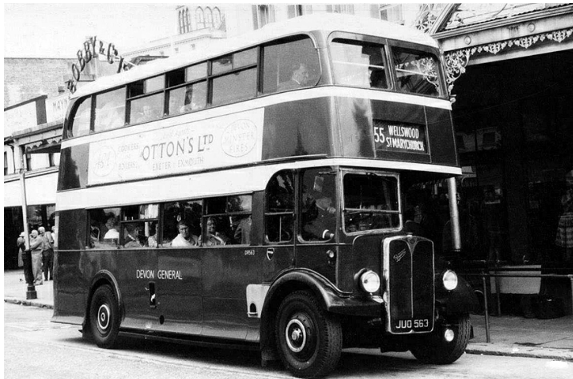
DR563 (JU0563), a 1948 AEC Regent III with Weymann 56-seat bodywork stands outside Bobby & Co with a full load. (LTHL collection).
