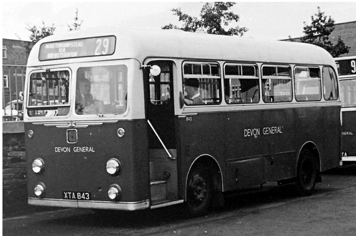
SN843 (XTA843) was a 1958 Albion NS3N 'Nimbus' with Willowbrook 41-seat bodywork. (Edward Busst).
