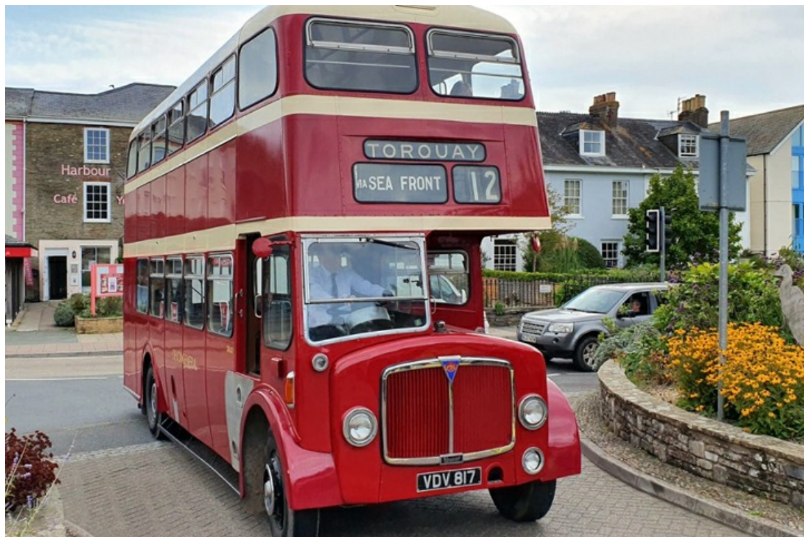
DR817 (VDV817) is a preserved 1957 AEC Regent V with Weymann 59-seat bodywork. (LTHL collection).
