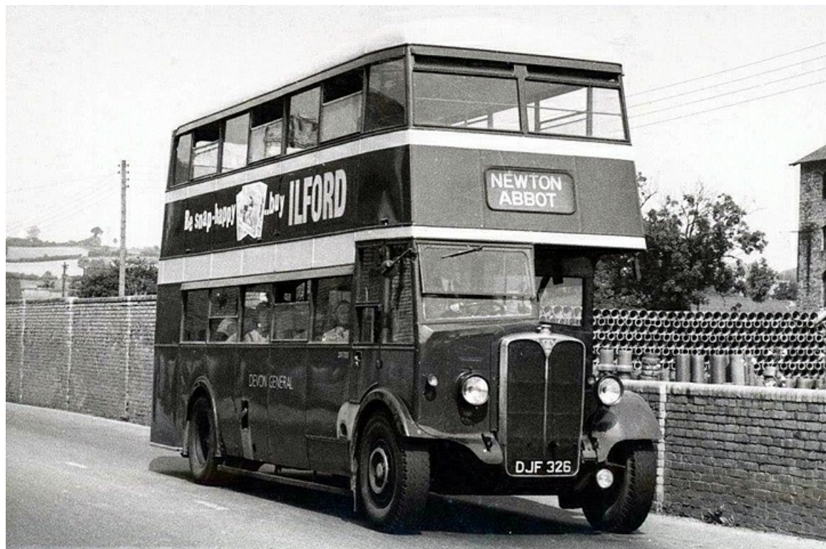
DR700 (DJF326) was a 1946 AEC Regent II with Park Royal 56-seat bodywork and was one of six that came from Leicester City Transport in part exchange for six AEC Regal's. (LTHL collection).
