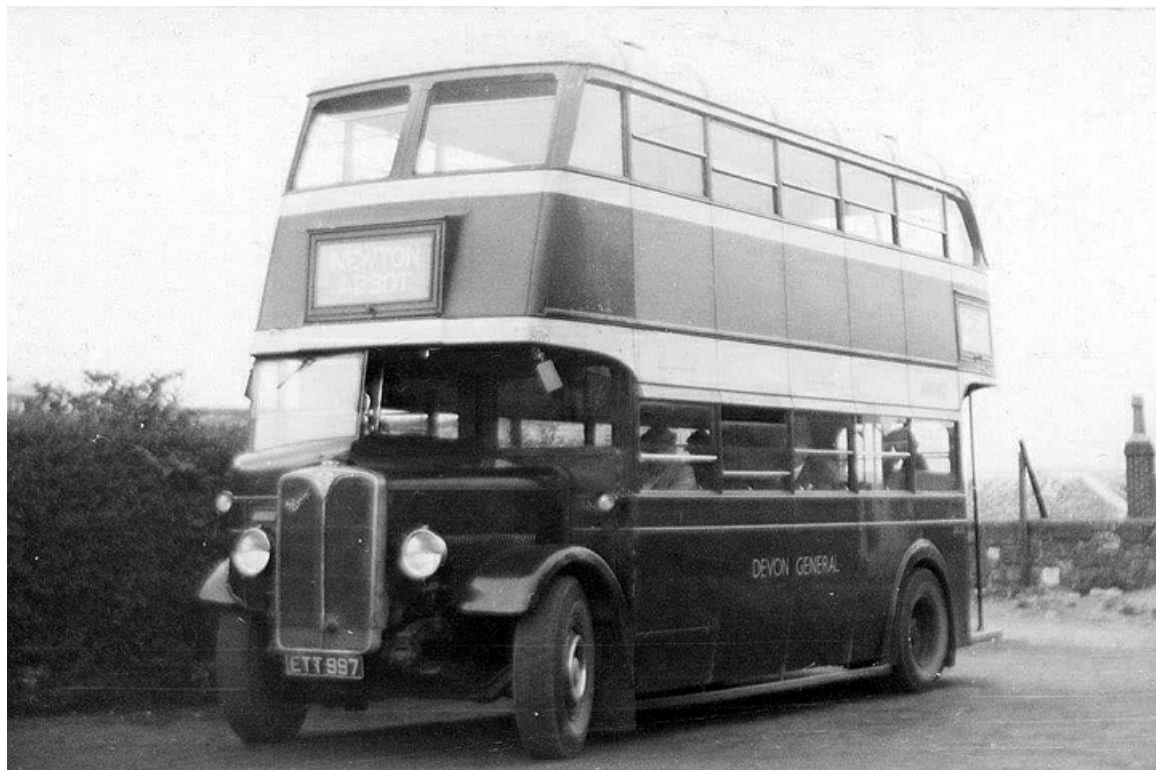
DR236 (ETT997) was a 1938 AEC Regent with Weymann H28/26R bodywork that gave sterling service until withdrawal in 1956. (LTHL collection).
