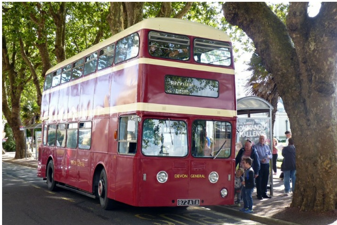
The first rear-engined vehicles arrived in 1959 in the shape of the Leyland PDR1/1 'Atlantean'. The first of the batch was DL872 (872ATA) with MCCW 78-seat bodywork, now in preservation. (Kevin Cripps).
