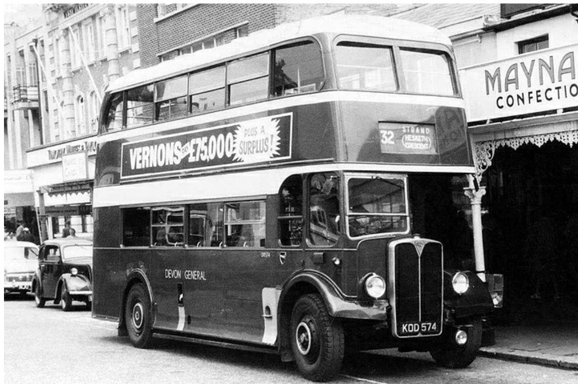
DR574 (KOD574), a 1949 AEC Regent III with Weymann 56-seat bodywork, which became the favoured Devon General bus combination postwar. (LTHL collection).
