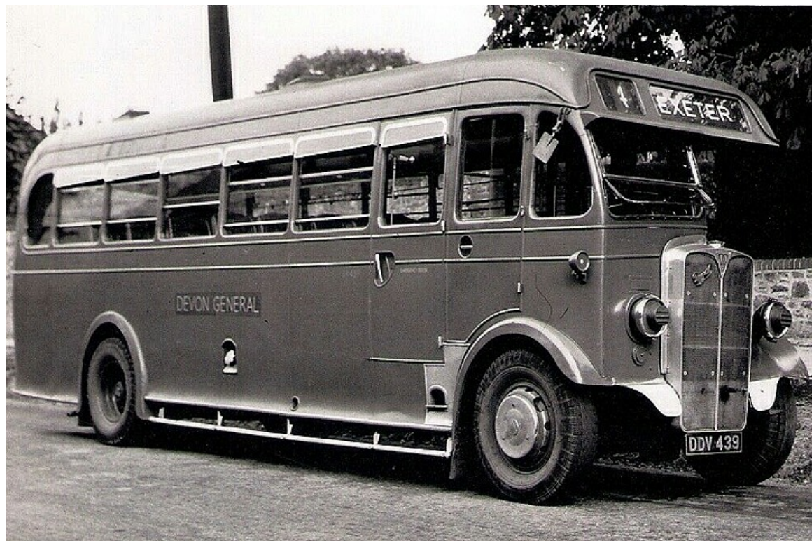
SR439 (DDV439), a 1939 AEC Regal with Harrington B35F bodywork, seen here in wartime grey livery. (LTHL collection).
