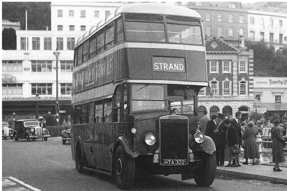
DL239 (HTA302) was a solitary 'unfrozen' Leyland TD7 with Weymann H30/26R bodywork added to the fleet in 1942. (The Bus Archive).
