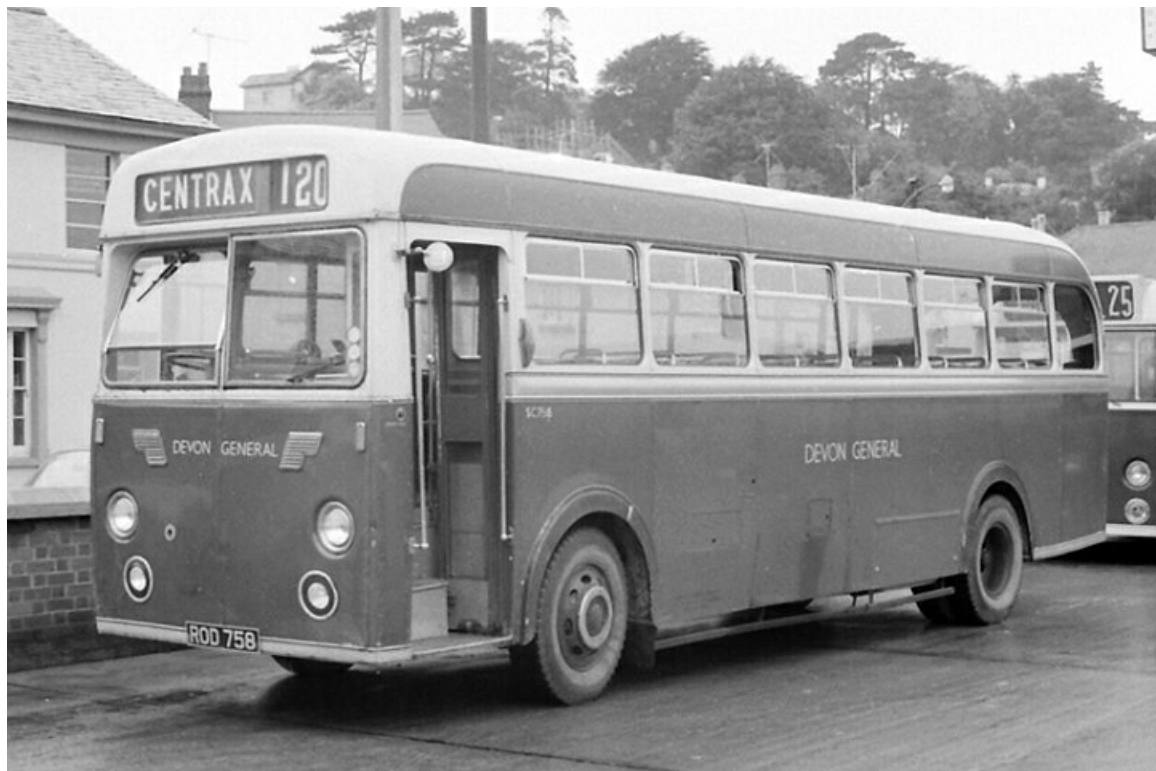
SC758 (ROD758) was a Beadle-Commer rebuild dating from 1956 and carried a Beadle B40F body. (Stuart Johnson).
