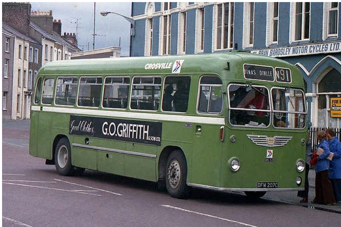
SMG538 (DFM207C) was a 1965 Bristol MW6G with ECW 45-seat bodywork, loading in Castle Square, Caernarfon in August 1977. (Patrick Keeley courtesy Michael Keeley).
