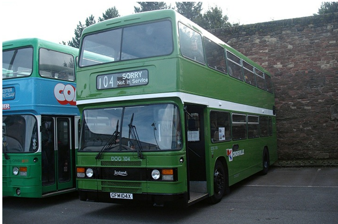
Introduced in 1982 was the Leyland 'Olympian'. DOG104 (GFM104X) was one of the first batch delivered and carries an ECW 77-seat body. (Ian Simpson).
