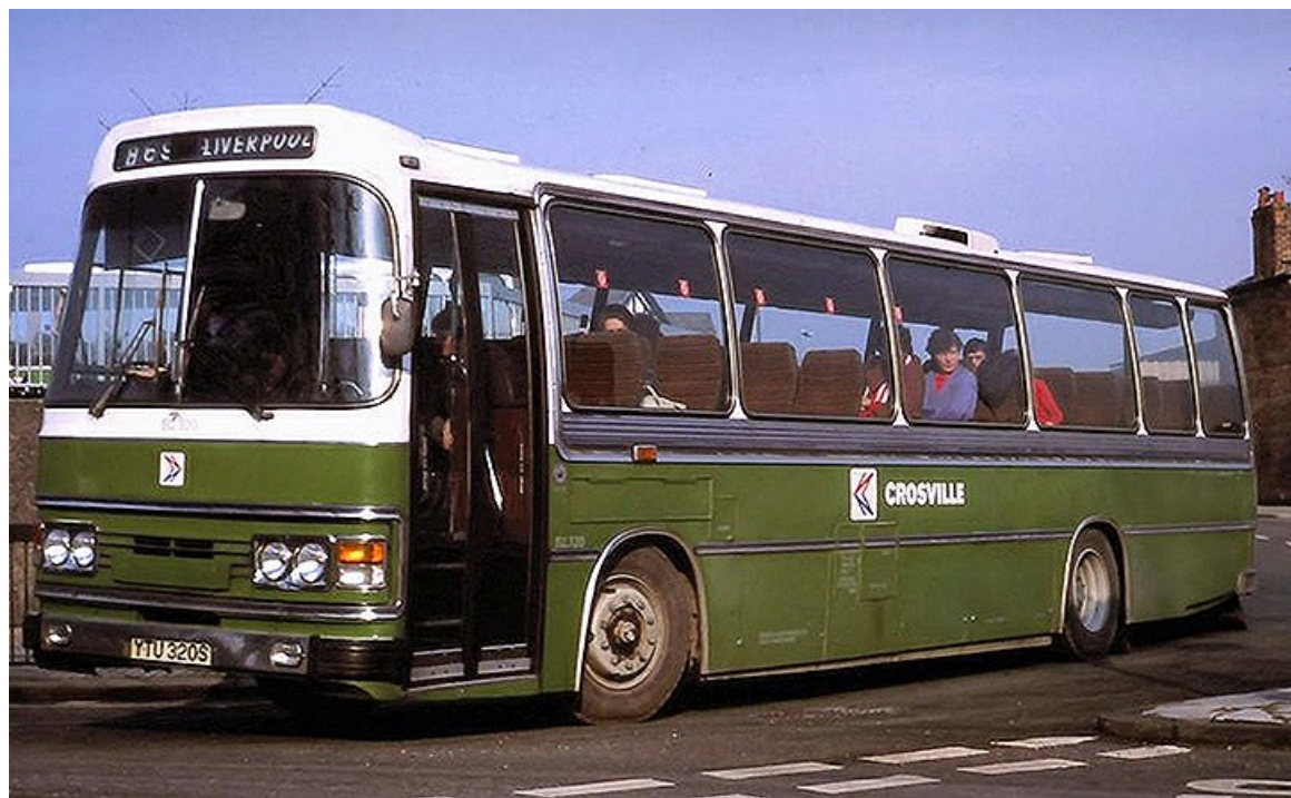
En route to Liverpool is CLL320 (YTU320S), a 1977 Leyland PSU3E/4R 'Leopard' with Duple 49-seat coachwork. (LTHL collection).
