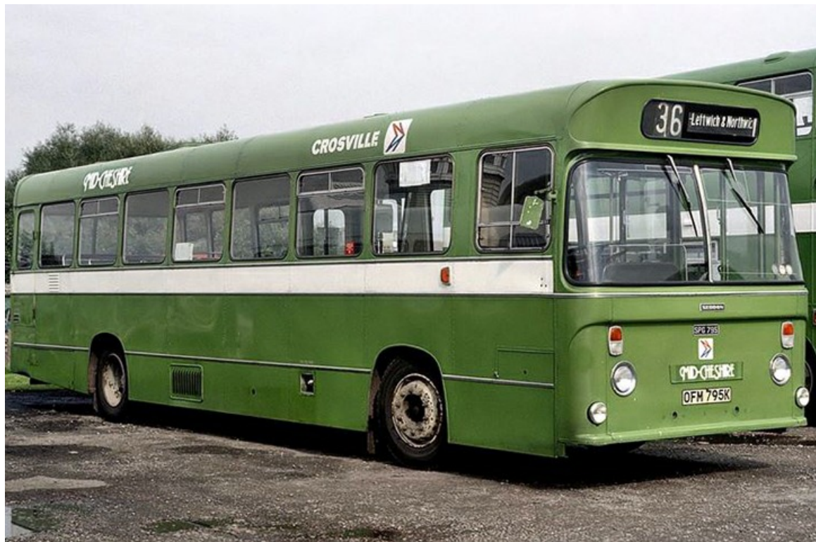
SPG795 (OFM795K), a 1971 Seddon Pennine with Pennine 45-seat dual entrance/exit bodywork. (LTHL collection).
