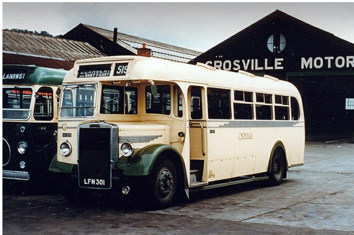
KA225 (LFM301) was a 1950 Leyland PS1/1 'Tiger' with Weymann 35-seat dual-purpose bodywork. (Dennis Kerrison courtesy Ron Hughes).
