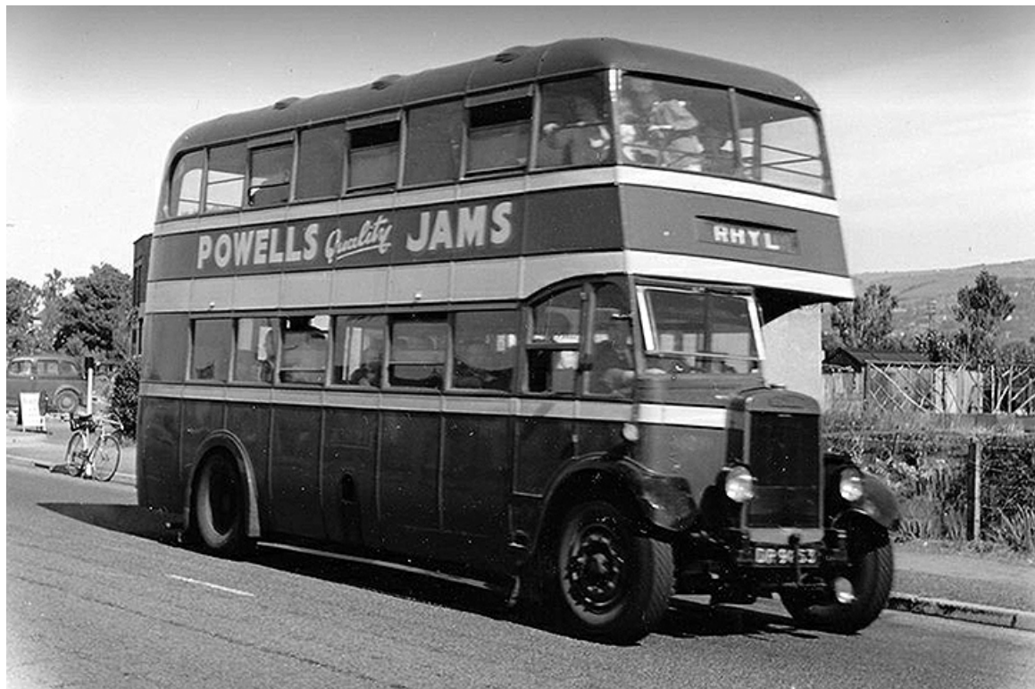
L83 (DR9853) was a 1932 Leyland TD2 with Mumford 48-seat bodywork. It was rebuilt by ECW and fitted with an oil engine during 1945-46, re-classified and re-numbered M239 as seen here. (Dennis Kerrison courtesy Ron Hughes).
