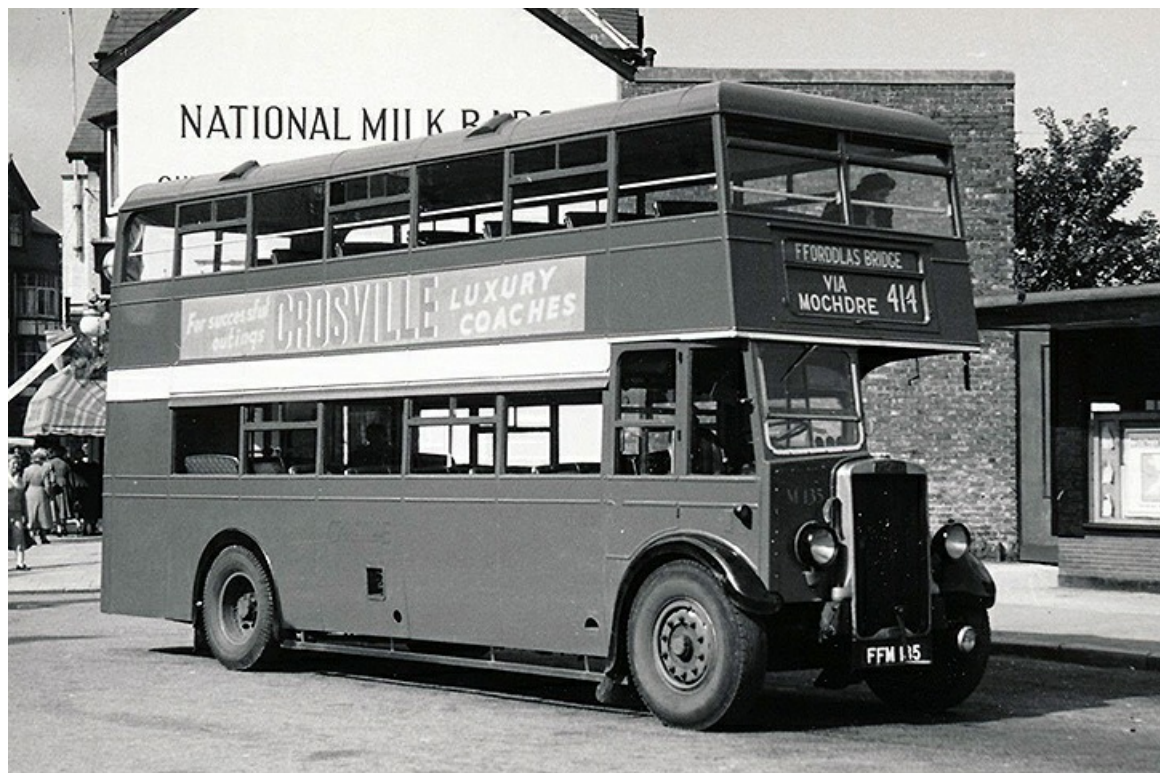
M135 (FFM185), a 1942 Leyland TD7 with Willowbrook utility 55-seat lowbridge bodywork. (LTHL collection).
