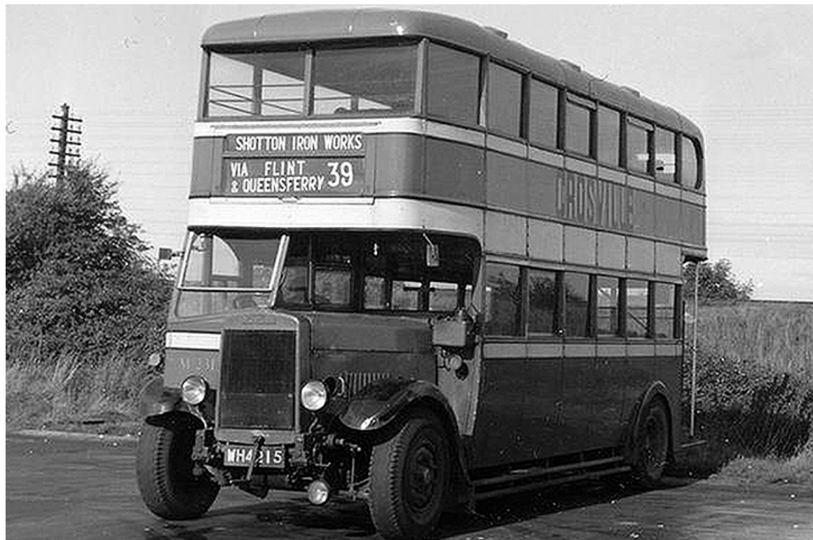
M231 (WH4215), formerly L70, was a 1933 Leyland TD2 with Bromilow & Edwards 48-seat lowbridge bodywork that was ex-Bolton Corporation. It had been fitted with an oil engine and rebuilt in 1947 by ECW. (Dennis Kerrison courtesy Ron Hughes).
