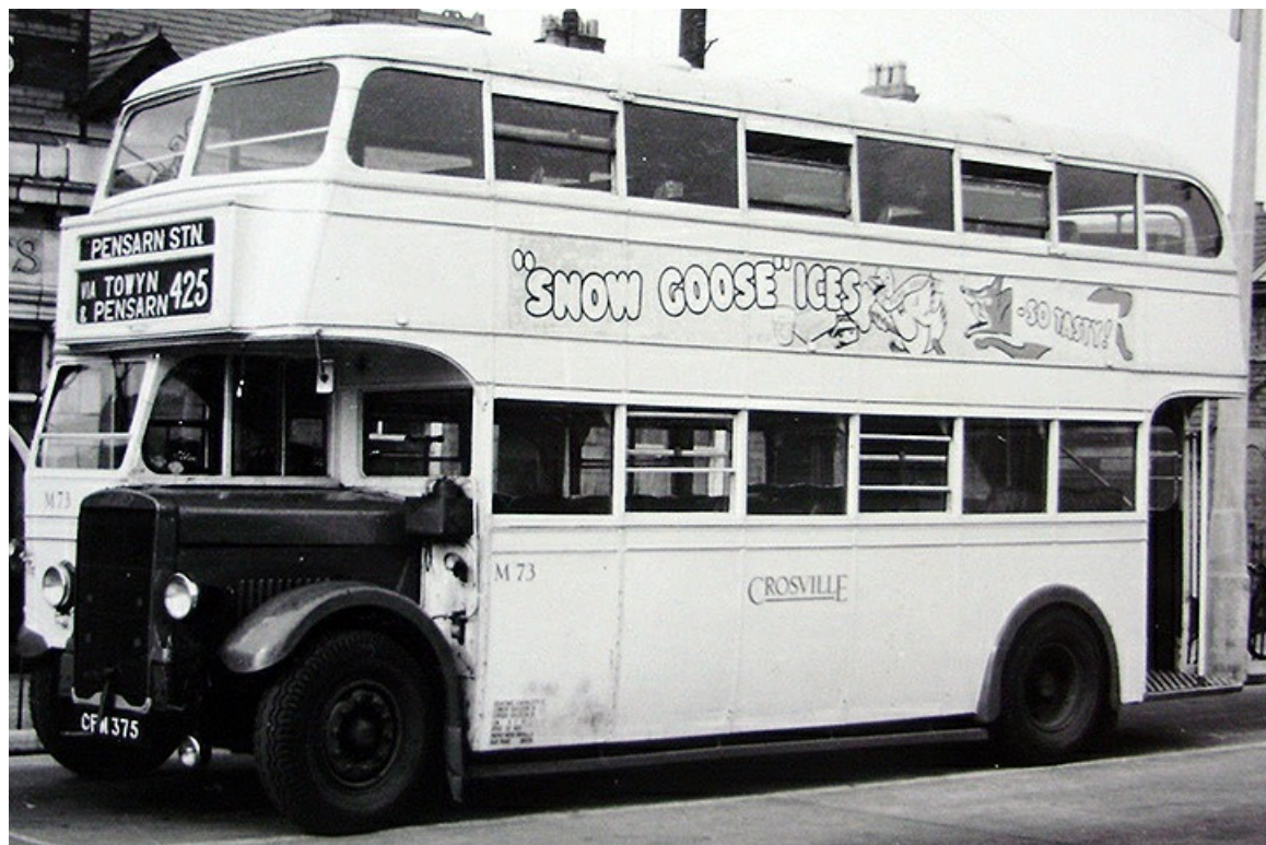
M73 (CFM375) was a 1938 Leyland TS8 unusually bodied as double-deck with an ECW convertible open top 52-seat lowbridge body. (LTHL collection).
