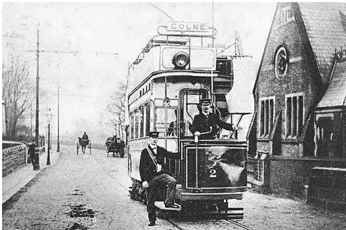
Nelson Car 2 was built in 1902 by Brush of Loughborough and seated 40. It is seen here at Reedyford ready to depart for Colne sometime before 1916 when it was withdrawn. (LTHL collection).
