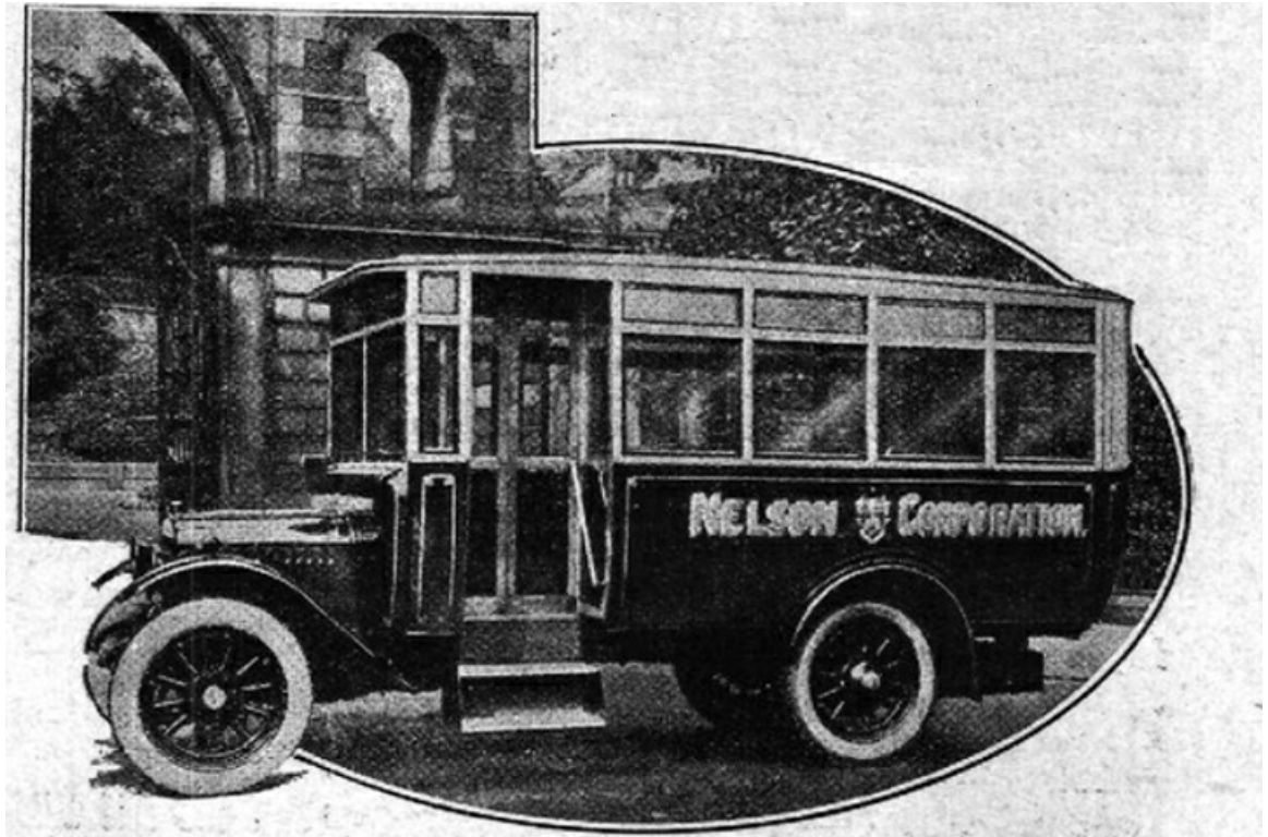
One of the five GMC K16 buses with 17-seat bodywork by Leaver which introduced bus services to Nelson in 1923. (Commercial Motor Archive).
