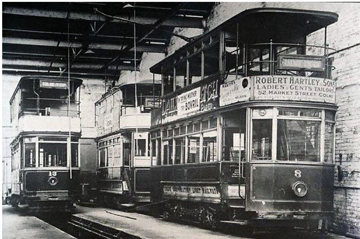
No. 8 was a 1905 Brush-built car on Brush bogies and seating 48 ex-Colne & Trawden in 1914. Car No. 13 was new to Colne Corporation in 1914 and was a United Electric Car-built balcony top covered double-decker car seating 52 on Preston bogies. (LTHL collection).
