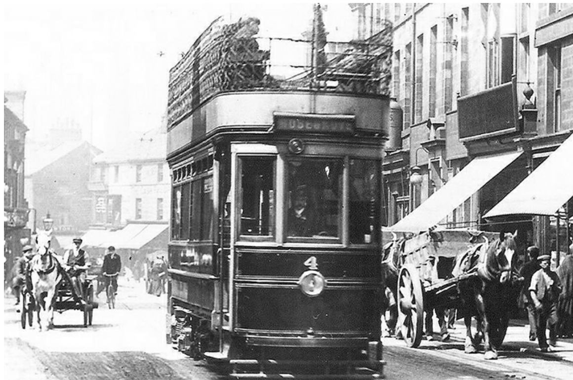
Burnley Corporation Tramways No. 4 was a Milnes-built 71-seat bogie car of 1901, seen here c. 1905 in original condition. It was fitted with top cover by 1920. (LTHL collection).
