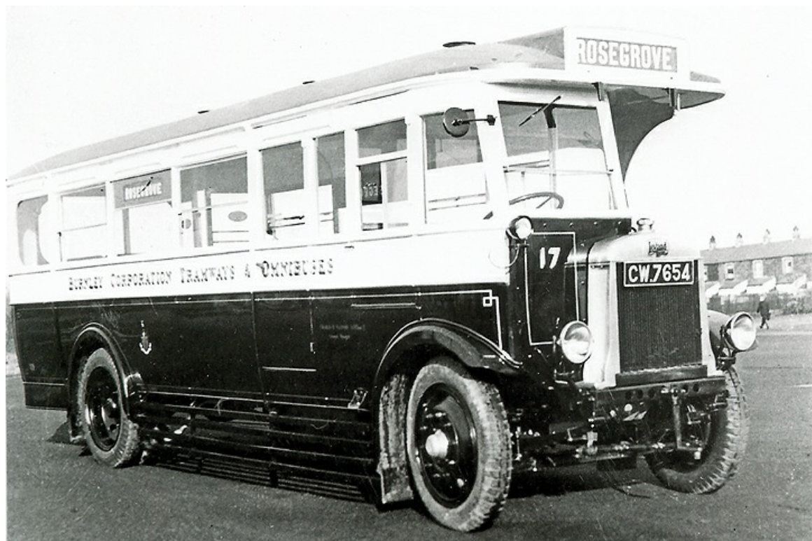
No. 17 (CW7654) was a Leyland PLSC1 'Lion' with Knappe B30R bodywork. (The Bus Archive).
