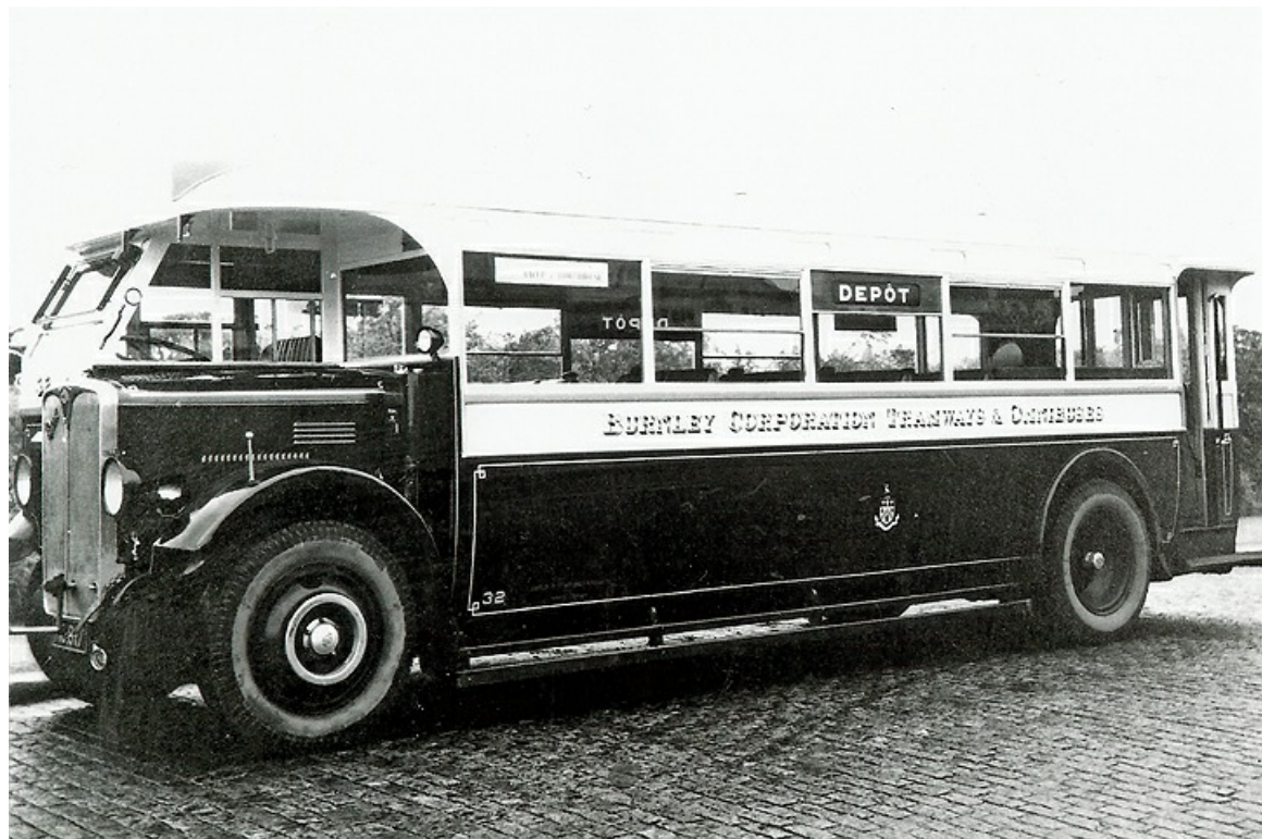
No. 32 (HG817) was a 1931 AEC Regal with Roe B31R bodywork. It passed to the Joint Committee in 1933. (The Bus Archive).
