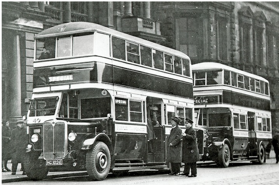
No. 40 (HG1026), a 1931 AEC Regent with Roe 50-seat centre-entrance bodywork was one of Burnley's first batch of double-deckers. It passed to the Joint Transport Committee in 1933. (The Bus Archive).
