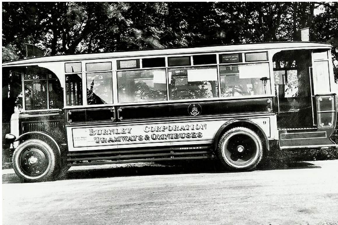
No. 9 (CW6808) was a 1926 Leyland PLSC1 with Knape B30R bodywork. It was rebuilt by Roe in 1929 and passed to the Joint Transport Committee in 1933. (The Bus Archive).
