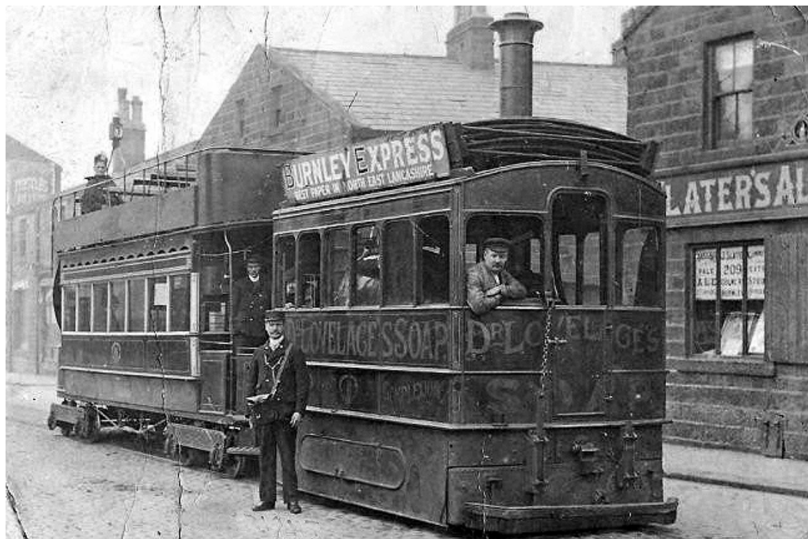
Burnley & District Tramways' 1883 Falcon loco No. 8 towing Starbuck bogie trailer No. 6 dating from 1885. (LTHL collection).
