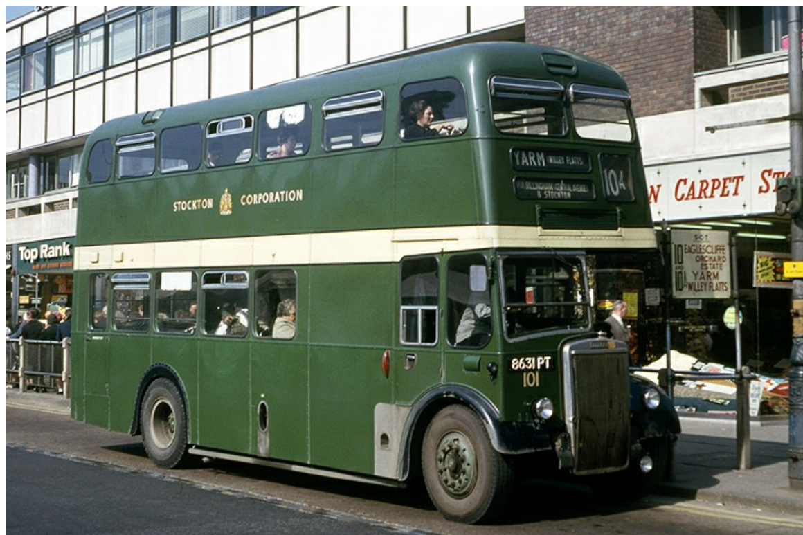
Stockton's first forward entrance double-deckers were seven Leyland PD2/40's with Weymann H36/28F bodywork delivered in 1962 This is No. 101 (8631PT). (LTHL collection).
