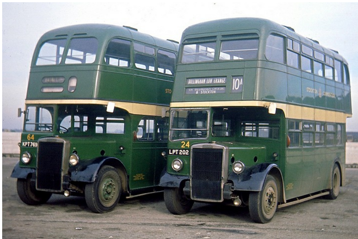
No. 24 was a 1950 Leyland PD2/3 with Weymann H30/26R bodywork, whilst No. 64 was a 1949 Leyland PD2/3 with Massey H30/26R bodywork. Both passed to Teesside Municipal Transport in 4/64. (John Huddleston).
