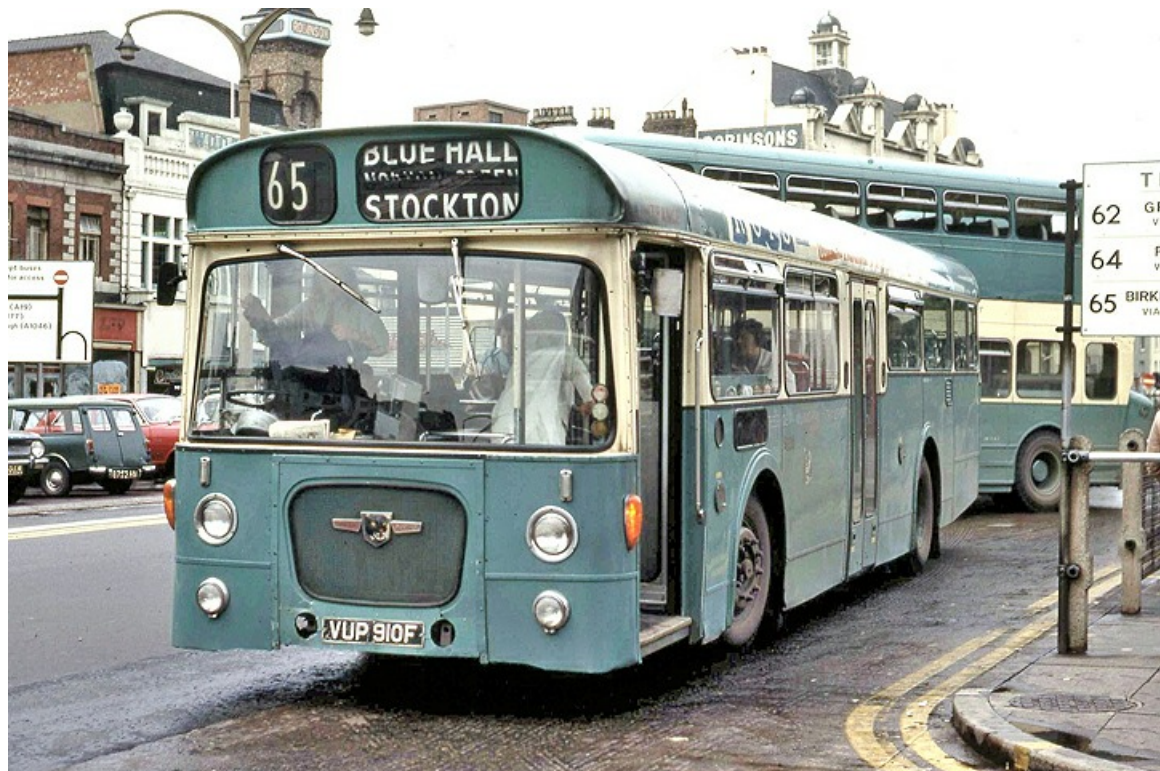
Stockton's final deliveries were a batch of Leyland PSUR1/1 chassis with Park Royal B48D bodywork that included No. S10 (VUP910F). (Charles Dean).
