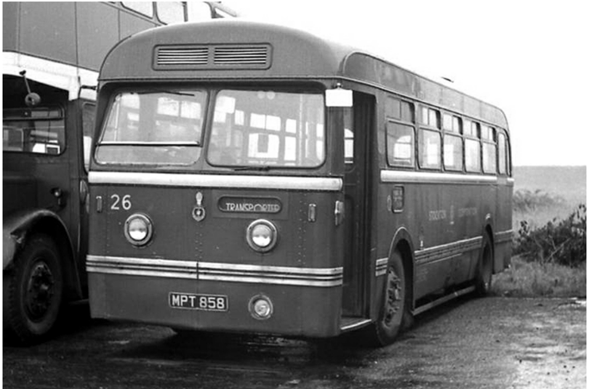
No. 26 (MPT858) was a solitary 1951 Leyland HR44/96 'Olympic' originally with Weymann B41D bodywork but later converted to front entrance for one-man operation as seen here. Note the rather small destination box. (John Kaye).
