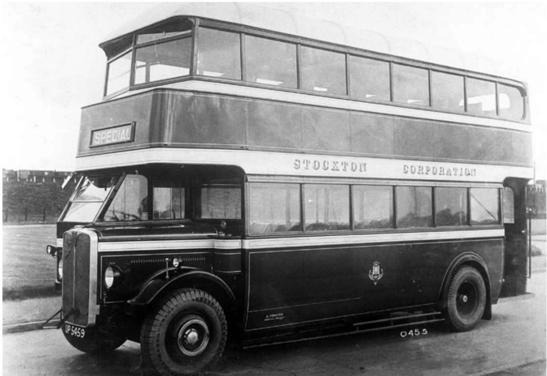
AEC vehicles were never favoured by Stockton although tried out. No. 61 (UP5459) was purchased in 1931 but no further orders were forthcoming. It was an AEC Regent with Short Bros H24/26R bodywork. (Bus Archive)
