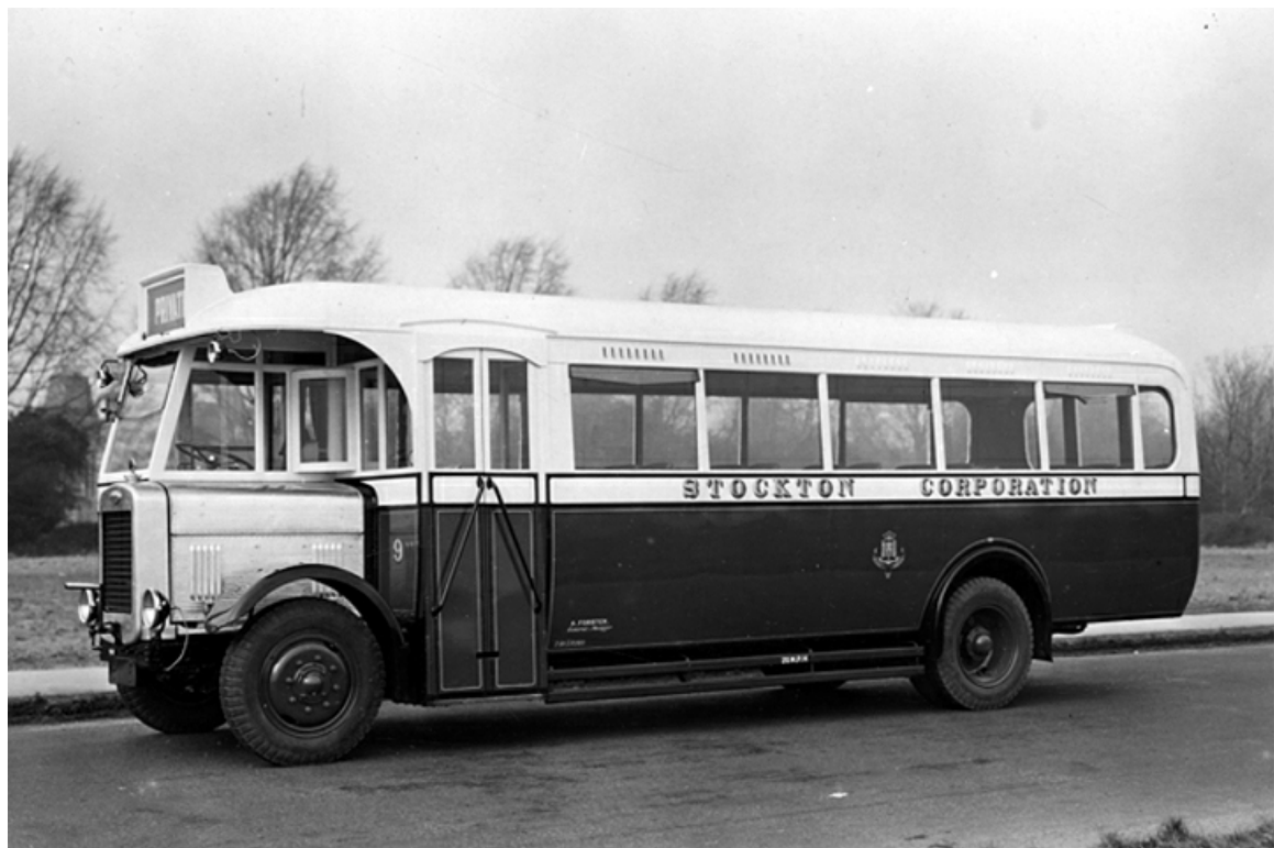
No. 9 (UP3712) was one of a number of different chassis purchased for comparison in the early 1930's. It was a Bristol B with Bristol B26F bodywork. (Bus Archive).
