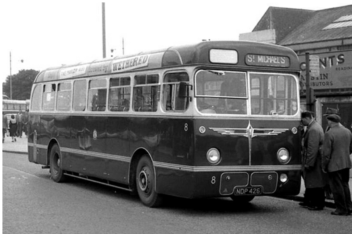
No. 8 (NDP426), was a 1957 AEC Reliance with Burlingham B34D standee-type bodywork licensed for 26 standing passengers. (John Boylett courtesy John Kaye).
