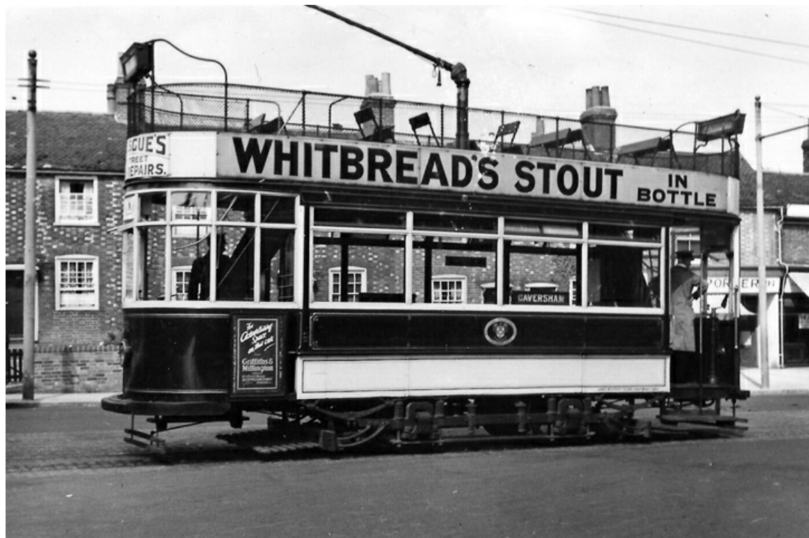
An unidentified Reading Corporation 4-wheel double-deck car seen here after being re-bodied and fitted with end vestibules by the Corporation. (LTHL collection).
