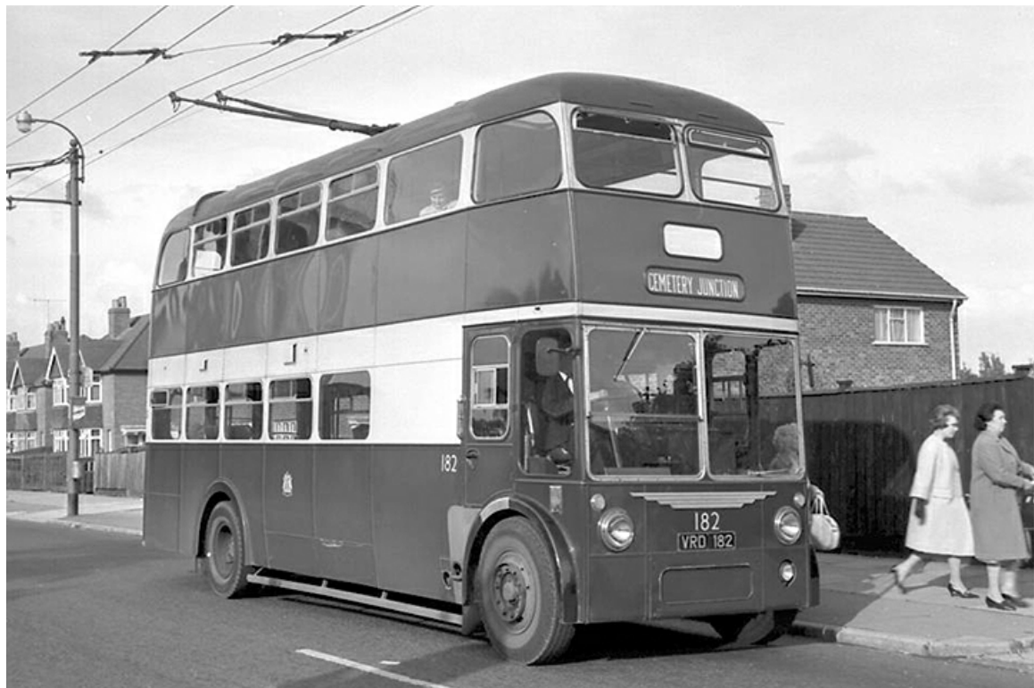
Reading's final batch of trolleybuses was delivered in 1961. This is No. 182 (VRD182) a Sunbeam F4A with Burlingham H38/30F bodywork. (John Boylett courtesy John Kaye).
