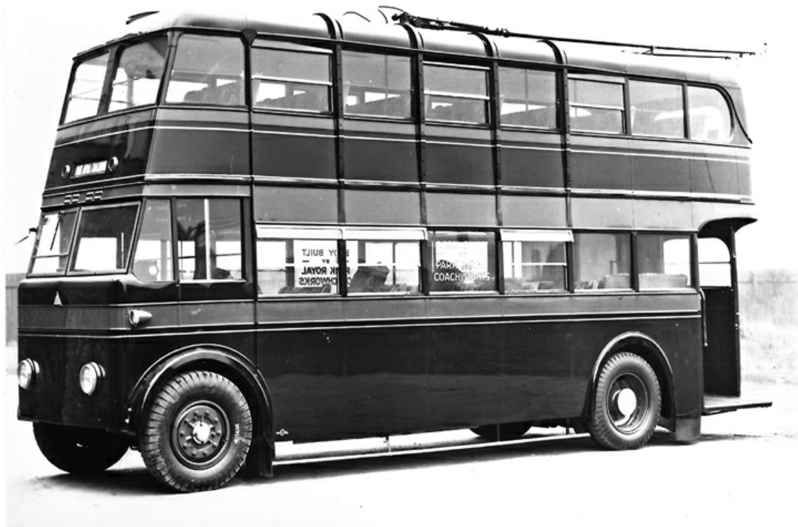
Reading's first trolleybus numerically in 1936 was No. 1 (RD8085), a Sunbeam MF2A with Park Royal L26/24R bodywork, which had been new as a prototype in 1933. (Bus Archive).
