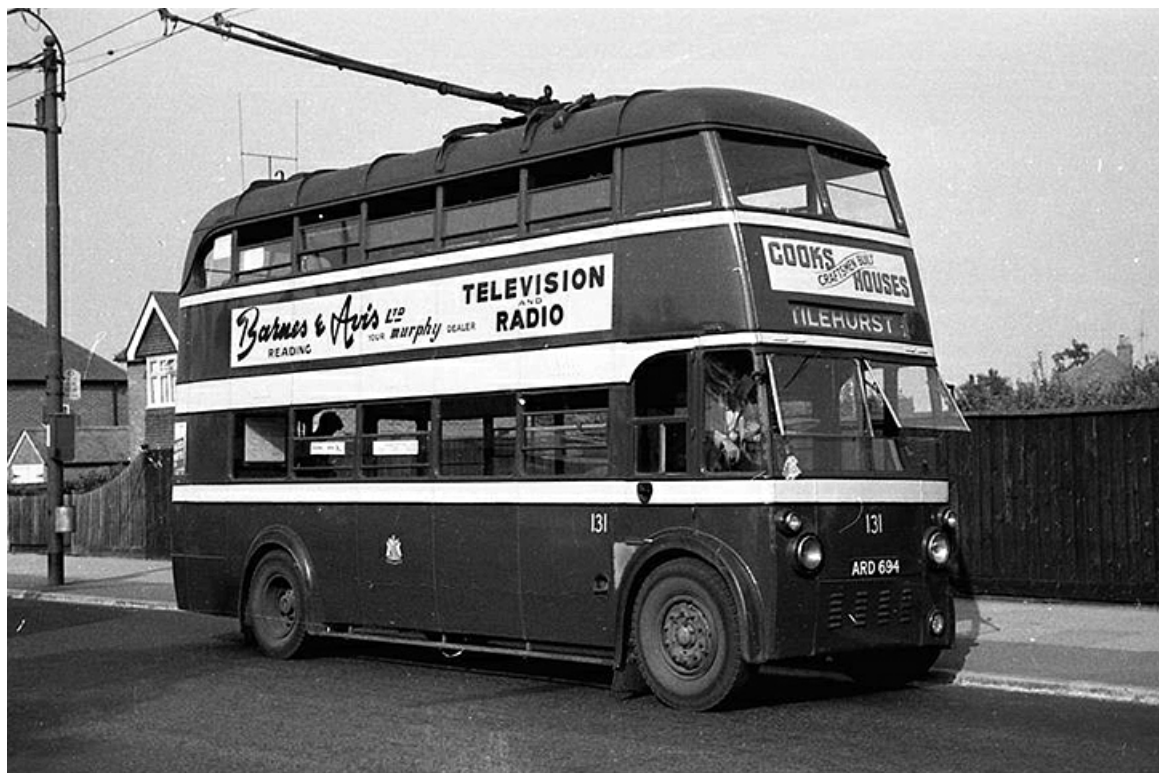
No. 131 (AED694), the last of 25 AEC661T trolleybuses with Park Royal H30/26R bodywork delivered in 1939. Seen here in Park Lane, Tilehurst in August 1959. (John Boylett courtesy John Kaye).
