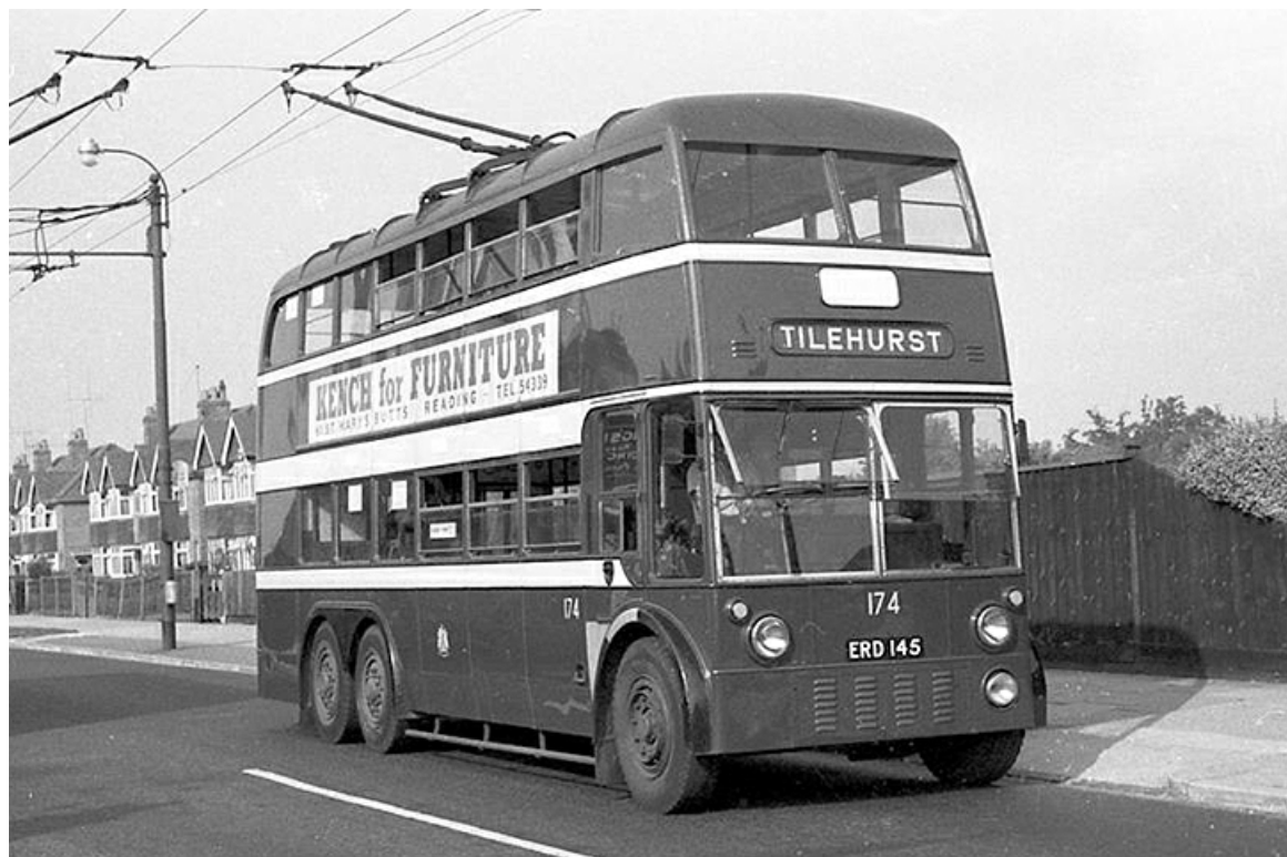
No. 174 (ERD145), a 1950 Sunbeam S7 with Park Royal H38/30RD bodywork travels along Park Lane, Tilehurst in August 1959. (John Boylett courtesy John Kaye).
