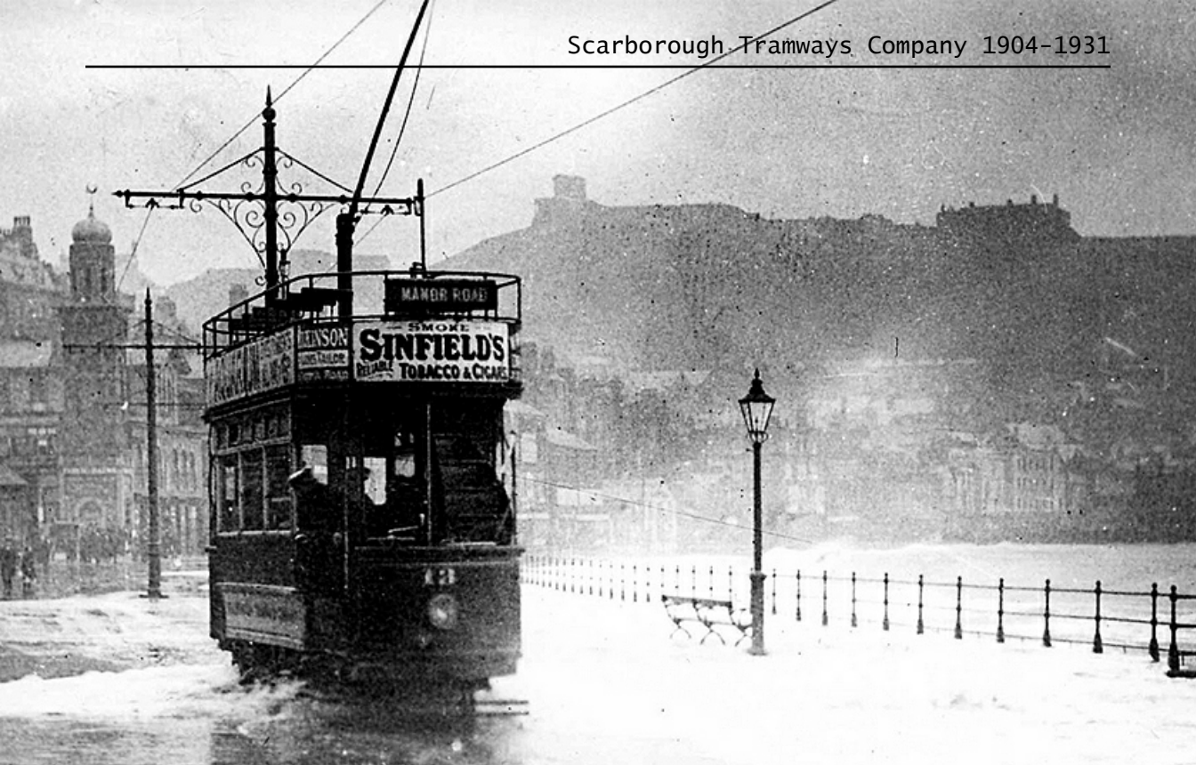
Car No. 13, a 1904 Brush-built open-topper battles its way around the bay on a stormy day sometime prior to 1907. Note the absence of passengers! (LTHL collection).
