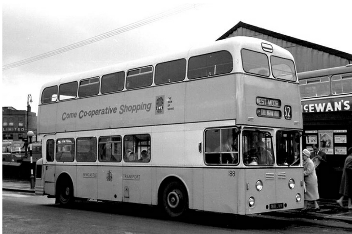
No. 188 (JVK188) was one of two Leyland PDR1/1 'Atlanteans' purchased in 1960 and were Newcastle's first rear-engined buses. This particular vehicle was bodied by Metro-Cammell to H44/34F. (John Boylett).
