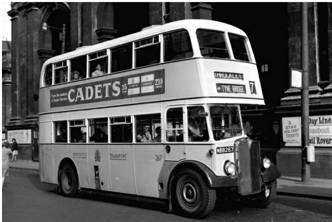
No. 267 (NBB267) dating from 1949 was an AEC Regent III with local Northern Coachbuilders H30/26R bodywork. (John Boylett)
