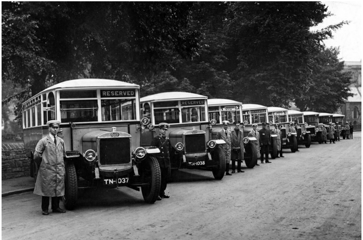
A 1925 line up of new buses shows the six Guy BB chassis with Strachan & Brown B29R bodies headed by Nos. 33 (TN1037) and 34 (TN1038). The last three buses are thought to be of AEC manufacture. (LTHL collection).
