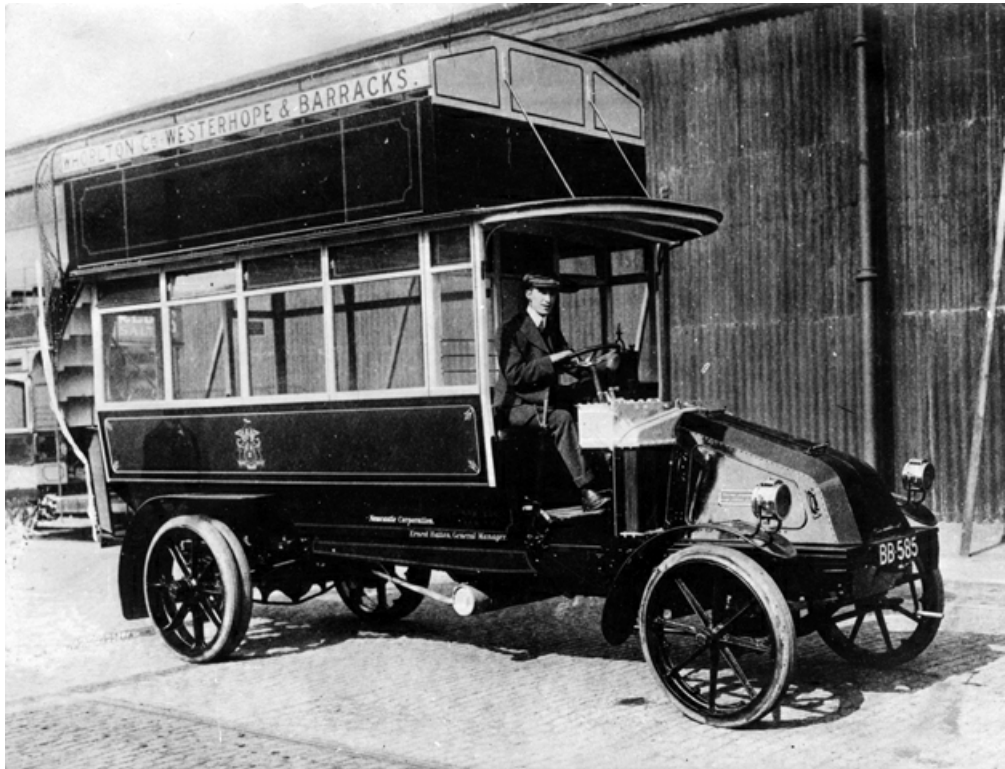
Newcastle's first bus was BB585, a Tilling-Stevens TTA1 with 34-seat bodywork probably built by the Corporation themselves. (Newcastle Libraries).
