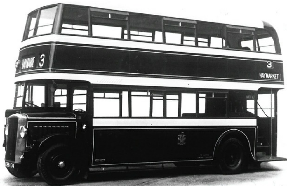
In 1937 Newcastle purchased 21 of these Daimler COG5's. This is No. 174 (EBB174) which carried a Metro-Cammell H28/24R body. (Bus Archive).
