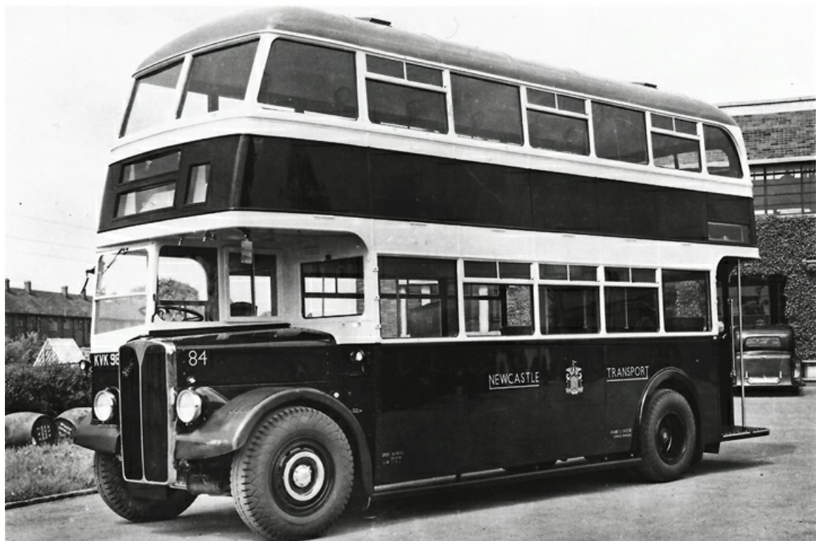
No. 84 (KVK984) was an AEC Regent III with Roe H31/25R bodywork, seen here in a pre-delivery photo. (Bus Archive).
