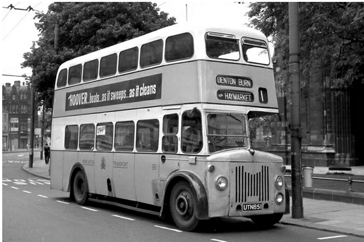
No. 351 (UTN851) was a Leyland PD2/20 with Metro-Cammell H32/26R bodywork that had been exhibited at the 1954 Commercial Motor Show. (John Boylett).
