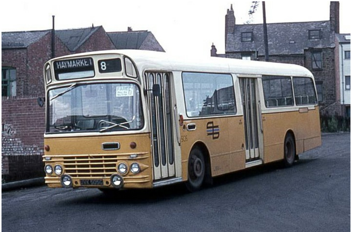
No.505 (UVK505G) was a Leyland PSUR1A/1 'Panther' with Alexander B45D bodywork, seen here wearing its Tyneside PTE emblem in June 1970 on Morden Street bus park. (Donald Hudson).
