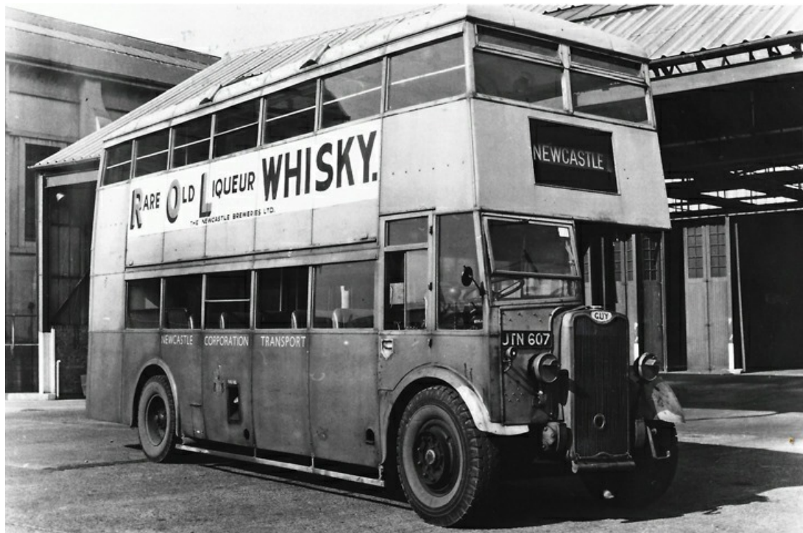
Wartime deliveries included No. 247 (JTN607) a Guy Arab I with Strachans lowbridge 55-seat bodywork, seen here in its wartime grey livery. (Bus Archive).
