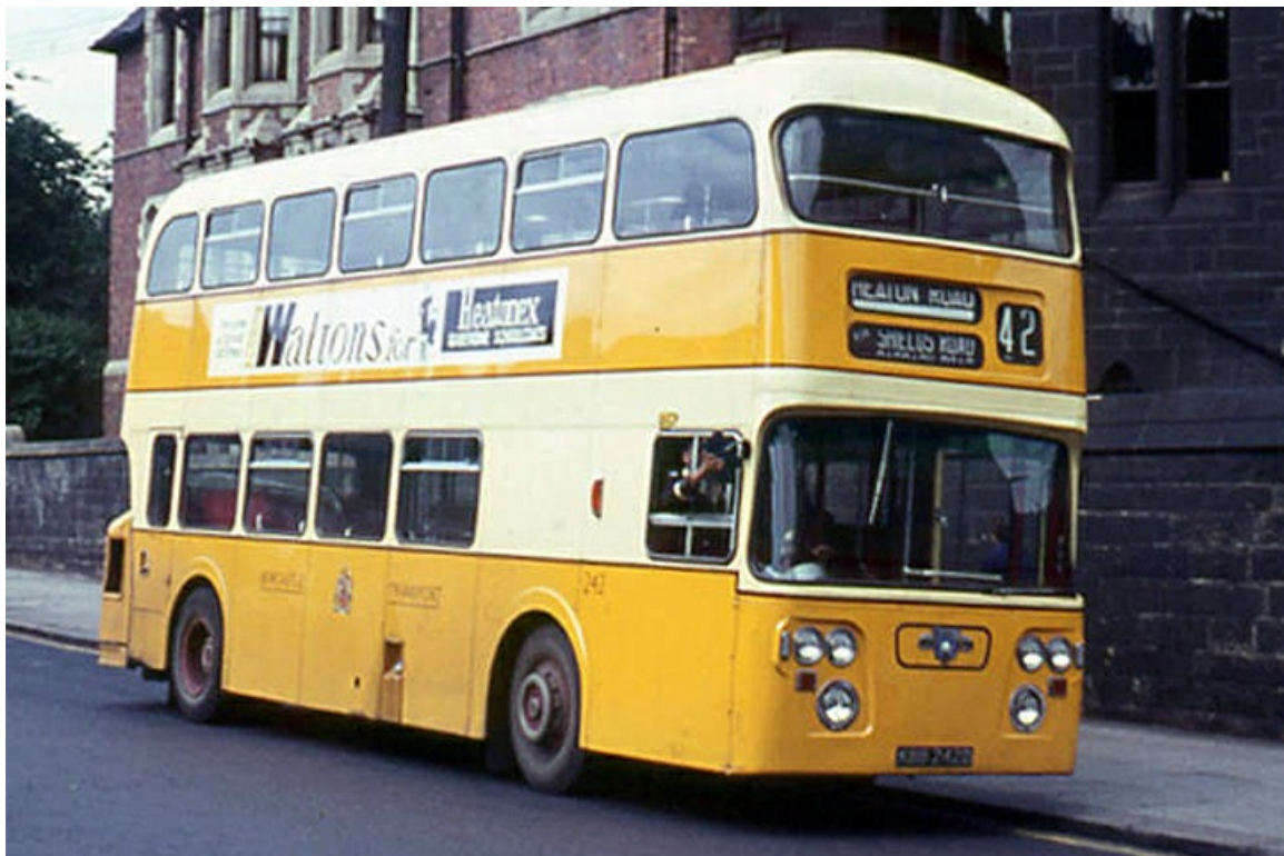
No. 242 (KBB242D) was a 1966 Leyland PDR1/1 with the distinctive Alexander H44/34F bodywork. (John Kaye).
