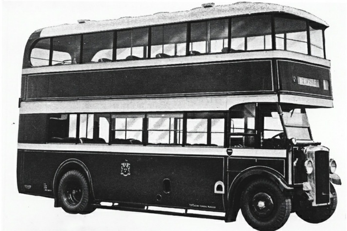
No. 137 (VK4081) was a 1931 Daimler CH6 with Park Royal H28/24R bodywork. It survived until the end of World War II in 1945 before being withdrawn. (Bus Archive).
