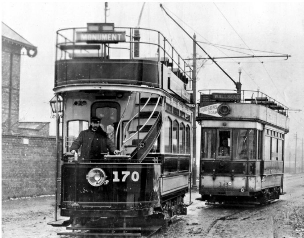
No. 170 was built in 1904 by Newcastle Corporation and shows how exposed tram drivers were in bad weather. It was rebuilt with top-cover and enclosed c. 1927. (LTHL collection).
