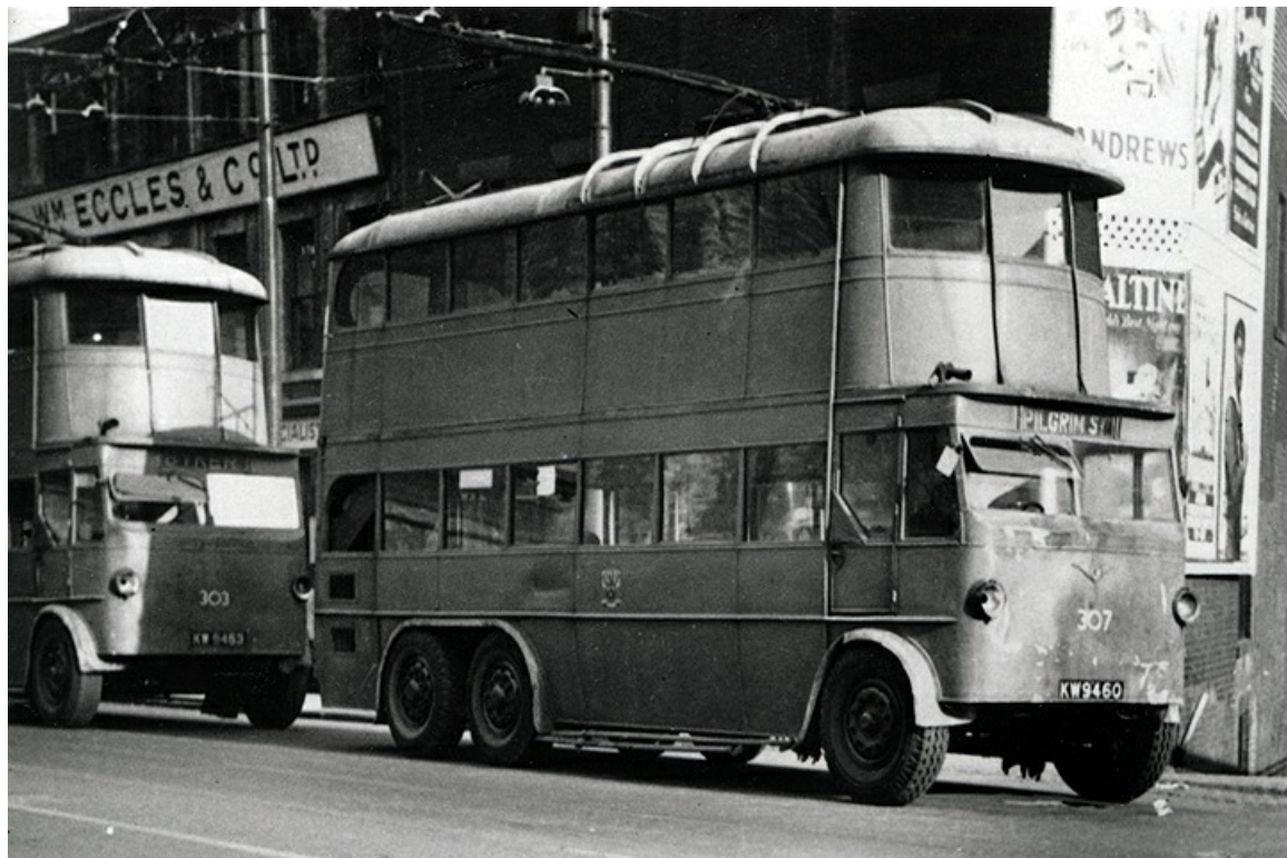
Painted in drab wartime grey these archaic looking vehicles were purchased from Bradford Corporation in 1943. No. 307(KW9460) was a 1929 English Electric E11 with English Electric H30/26R bodywork. (Newcastle Libraries).
