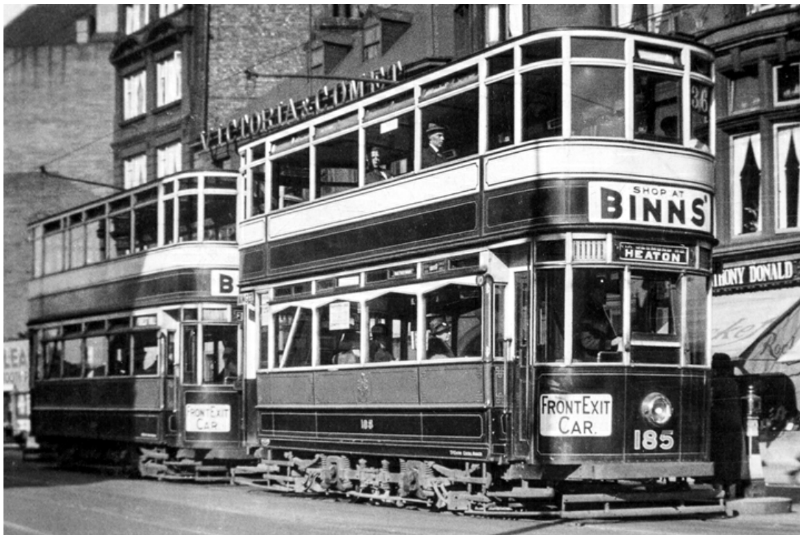
No. 185 built by Newcastle Corporation in 1904-05 showing the top covers and vestibules fitted to this batch of cars in 1927-1929. (LTHL collection).
