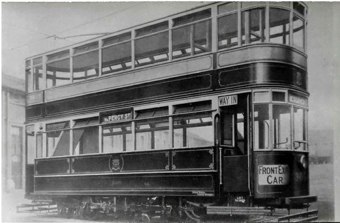
No. 300 was built by Newcastle and fitted with six-wheel truck for trials as seen here. It was later fitted with conventional single truck. (LTHL collection).
