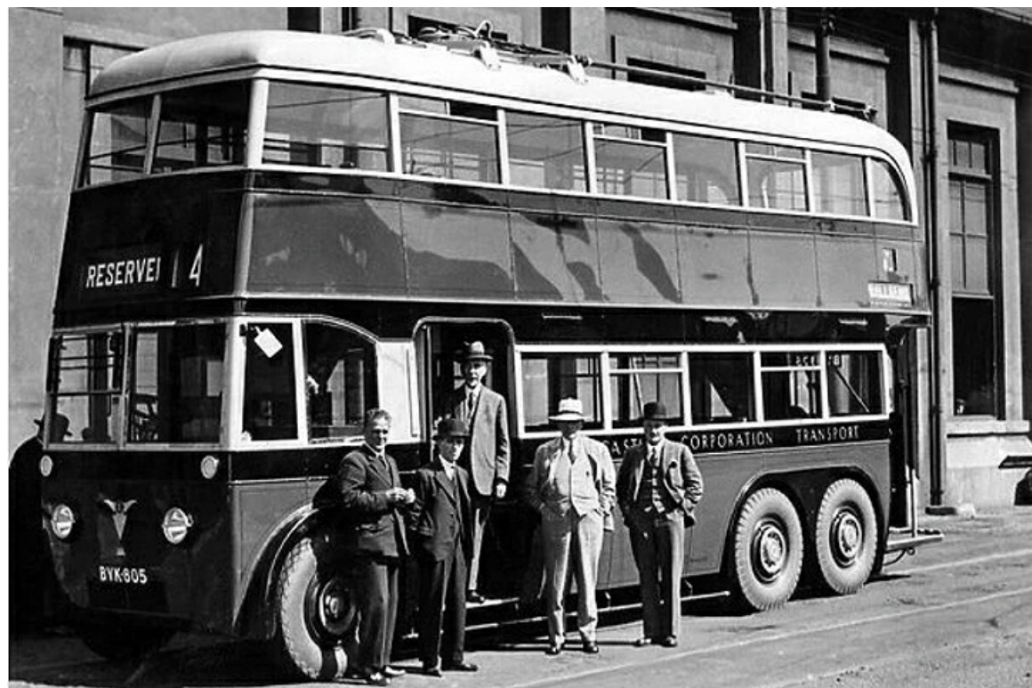
No. 15 (BVK805) was among the first intake of trolleybuses in 1935. It was an AEC 664T six-wheeler with Brush H33/27D bodywork and is seen here soon after delivery. (Newcastle Libraries).
