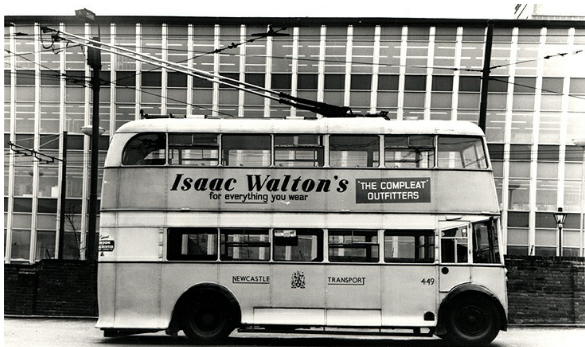
No. 449 (LBB49) was a 1949 Sunbeam F4 with Metro-Cammell H30/26R bodywork. (Newcastle Libraries)
