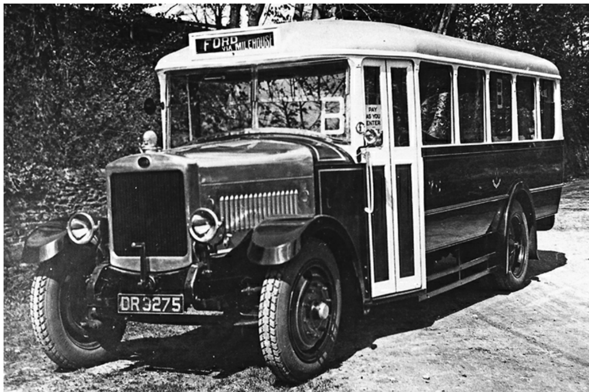
No. 78 (DR3275) was this normal control Guy B with Guy 20-seat bodywork dating from 1929. (The Bus Archive).
