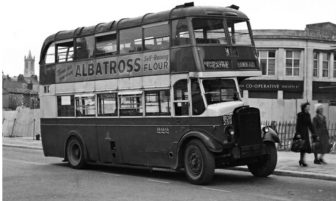
No. 222 (BDR259) was a 1939 Leyland TD5c with Weymann L24/24R bodywork that remained in the fleet until 1951. (The Bus Archive).
