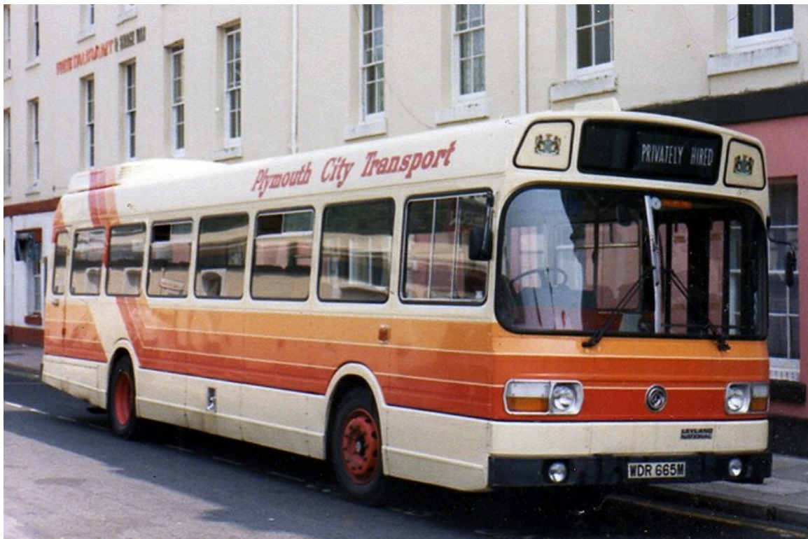
No. 65 (WDR665M) was a 1974 Leyland National originally B46D configuration it was rebuilt to DP41F in 1981 for private hire work and given this distinctive livery. (Les Eddy).
