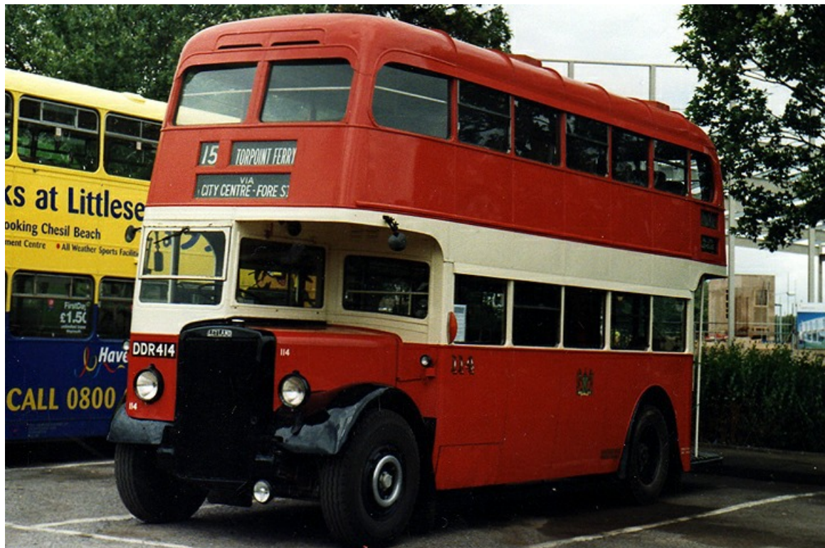
No. 114 (DDR414) is a Leyland PD1A with Weymann/Mumford L27/26R bodywork new in 1947 and now in preservation. (Les Eddy).
