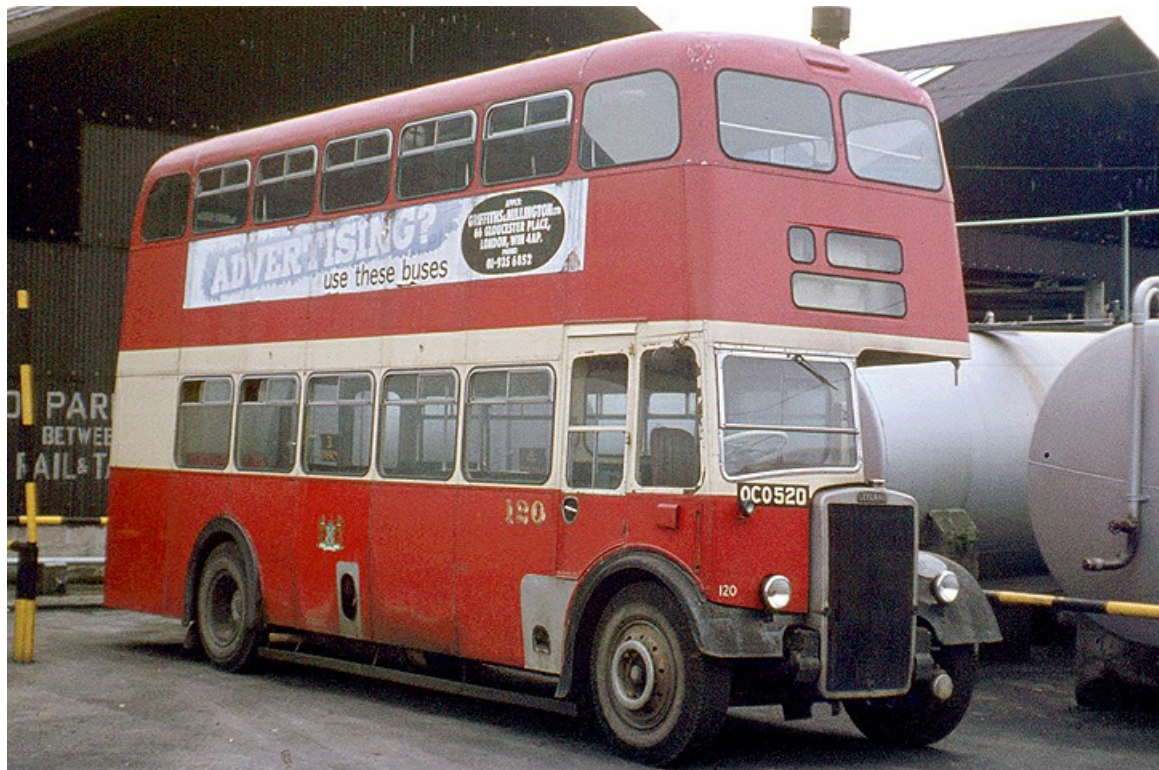
No. 120 (OC0520) was a 1958 Leyland PD2/40 with Metro-Cammell H30/26R bodywork. Withdrawn in June 1974 it is pictured here still at Milehouse in January 1975 albeit in withdrawn condition. (LTHL collection).
