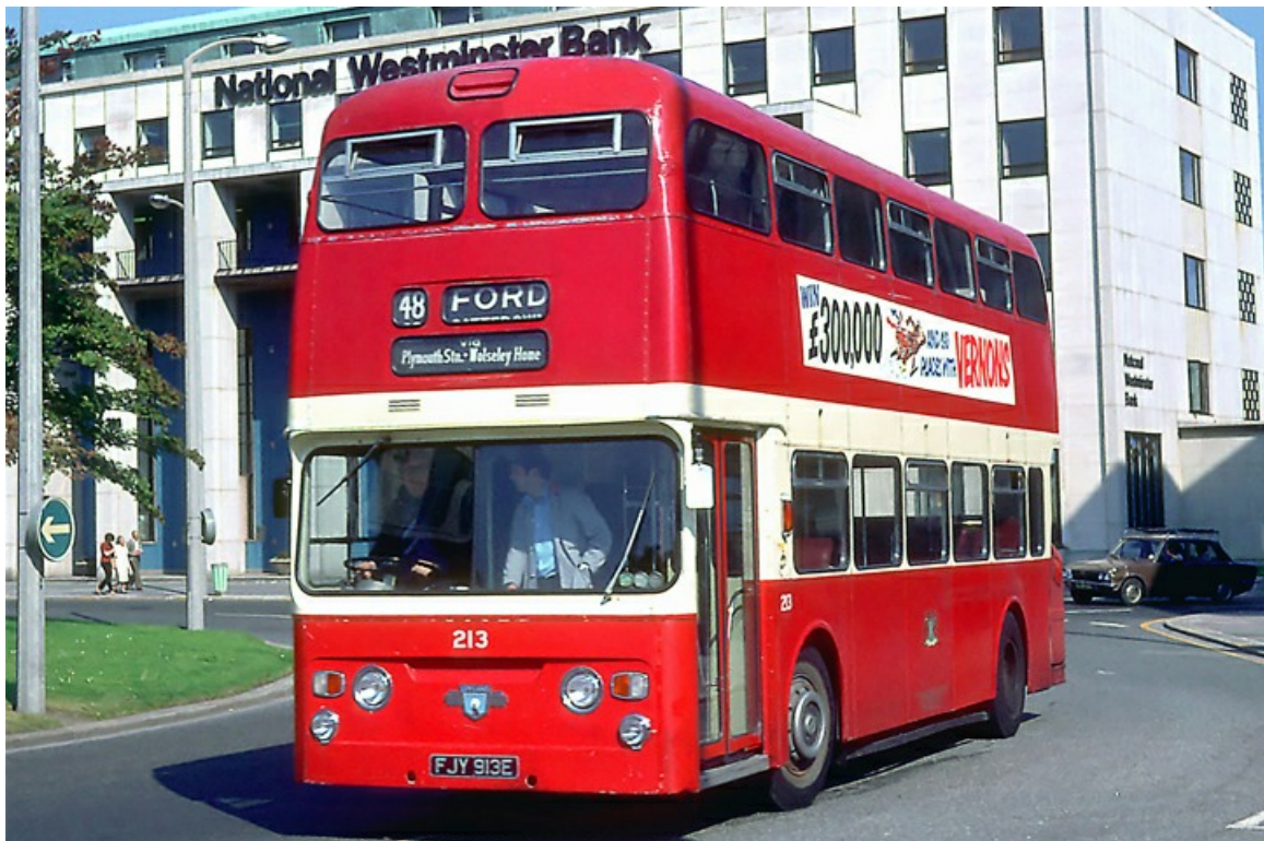
No. 213 (FJY913E) is a 1967 Leyland PDR1/1 with Metro-Cammell Weyman H43/32F bodywork, seen here in Royal Parade in September 1972. (Alan Snatt).
