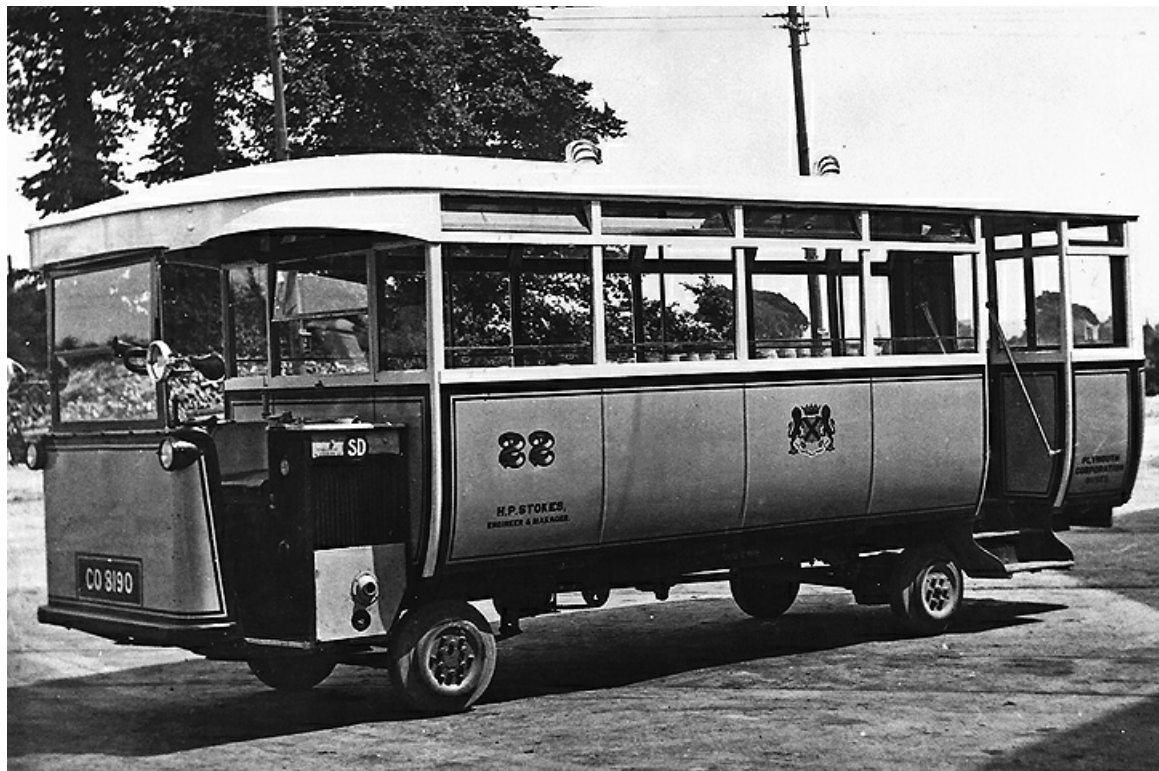
No. 22 (C08190) was an unusual vehicle for a municipal fleet. It was a Shelvoke and Drewry Freighter with Hickman 20-seat bodywork. It was withdrawn and converted by the Transport Department to a gully cleaner in 1929. (The Bus Archive).
