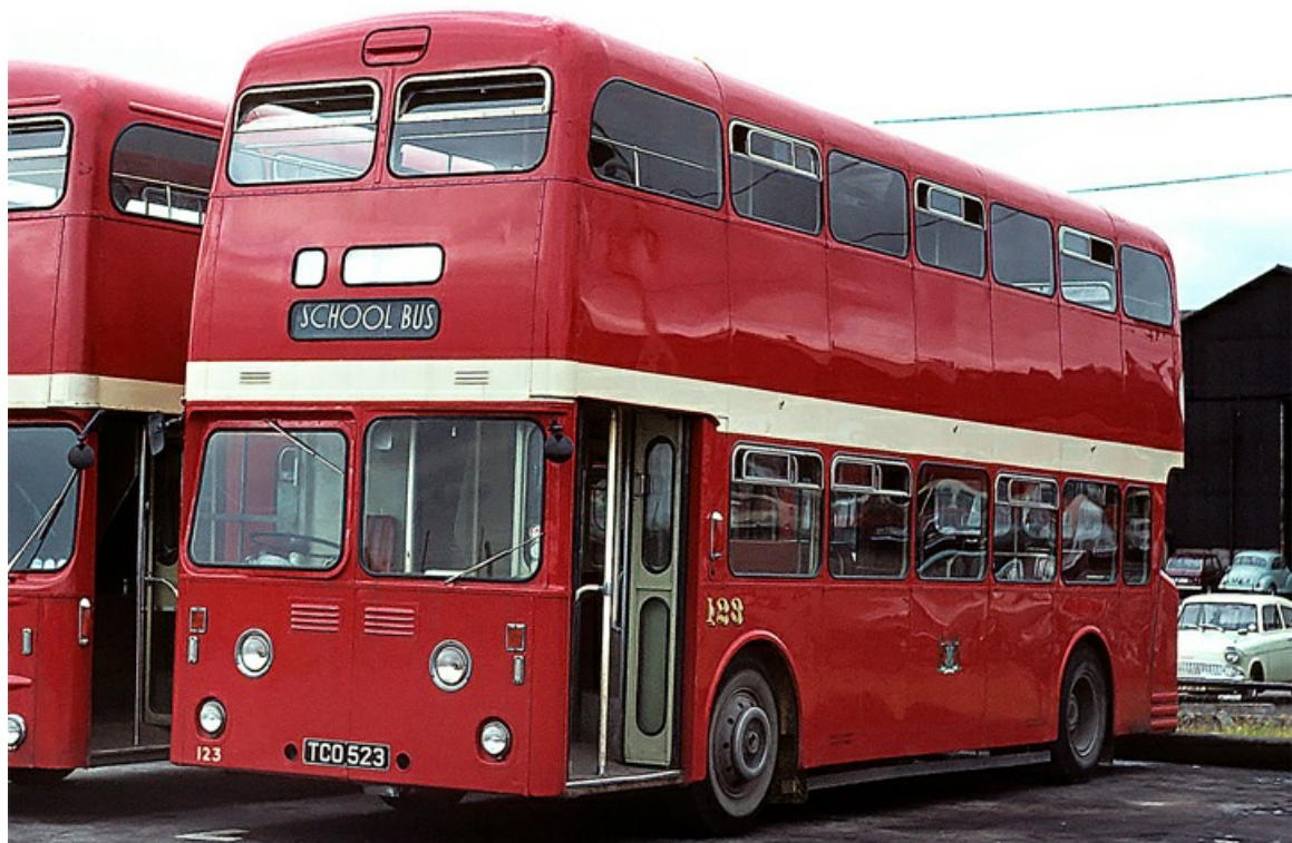
No. 123 (TCO523) was one of Plymouth's first rear engined vehicles. It was a 1960 Leyland PDR1/1 'Atlantean' with MCCW H44/33F bodywork. (Alan Snatt).
