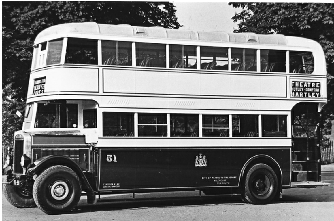
No. 51 (DR9840) was a Leyland TD2 with Weymann L24/24R bodywork. This particular vehicle was unfortunately destroyed by enemy action in March 1941. (The Bus Archive).
