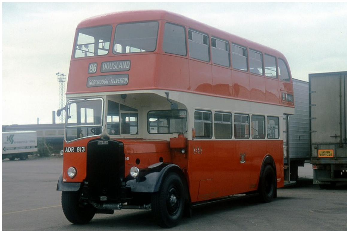
ADR813 is a 1938 Leyland TD5c originally numbered 213 and with a Weymann L24/24R body, it was re-bodied by Leyland in 1953 and re-numbered 141 and survives today in preservation. (John Law).
