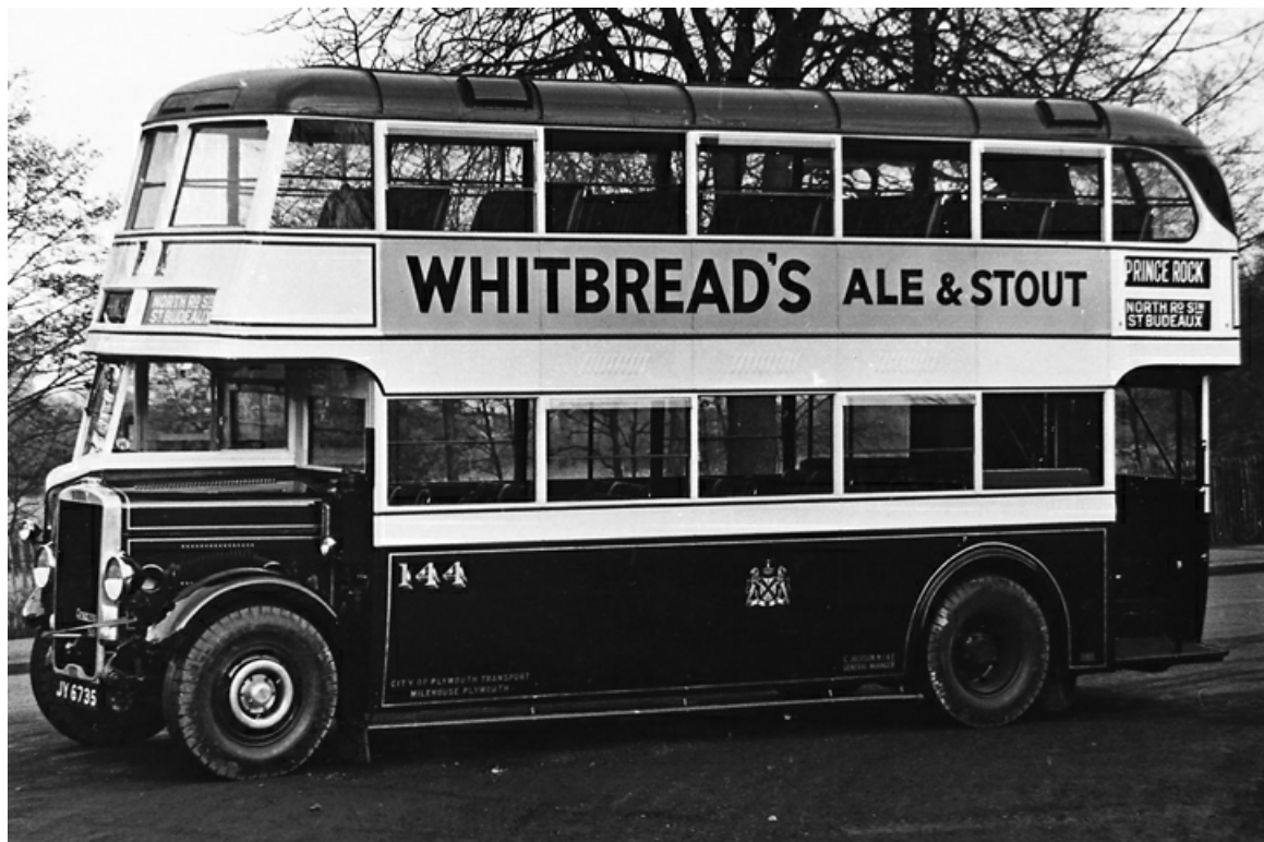
No. 144 (JY6735) was a 1935 Leyland TD4c with Weymann L24/24R bodywork. (The Bus Archive).
