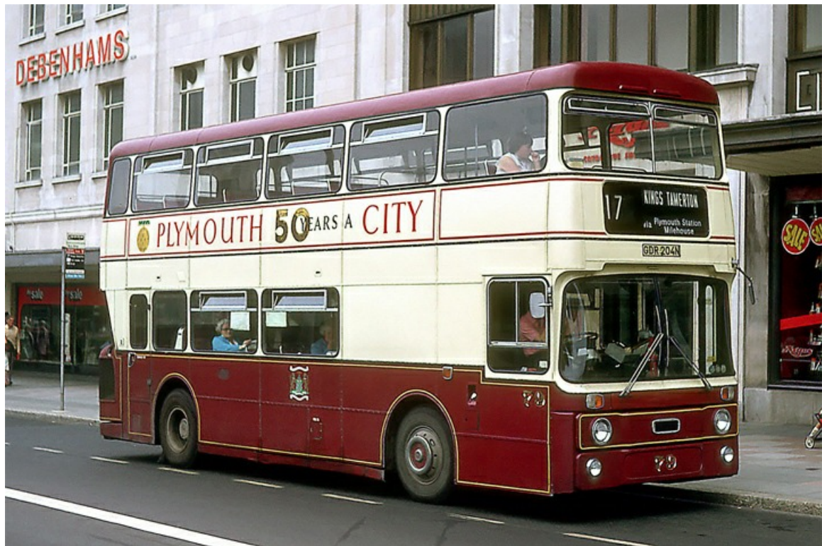
Celebrating 50 years of Plymouth being granted city status is No. 79 (GDR204N) a 1975 Park Royal H43/28D bodied Leyland AN68/1R 'Atlantean' seen in Royal Parade in 1980. (Alan Snatt).
