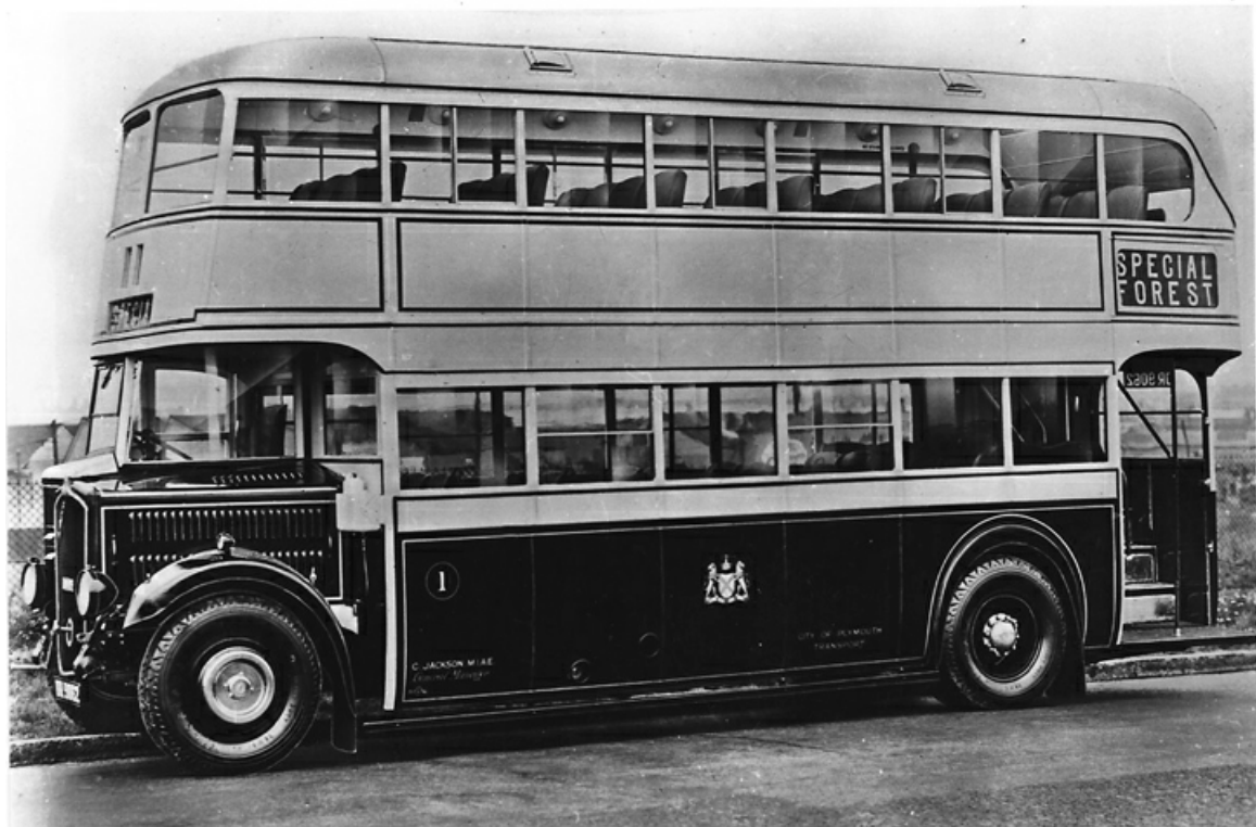
No. 1 (DR9062) was the first of four Dennis Lance II chassis with Park Royal L24/24R bodywork purchased in 1931. (The Bus Archive).
