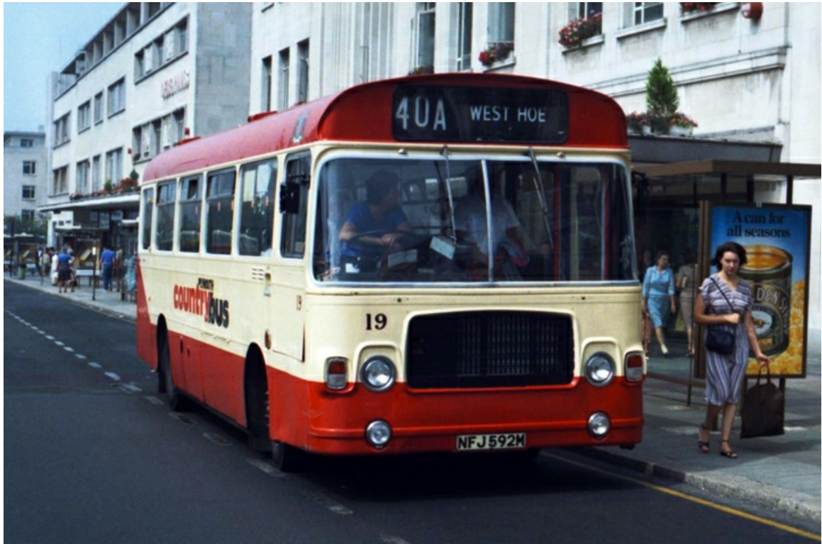
No. 19 (NFJ592M) was one of five Bristol LH6L's with ECW B43F bodywork purchased from Western National in 1982 and branded for Plymouth 'Countrybus' routes. (Jos van Hemert).
