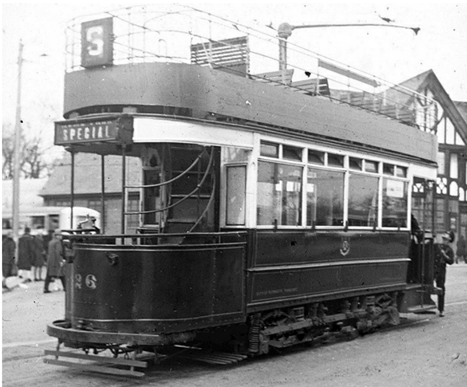
No. 26 was built by Brush in 1902 on Peckham trucks and seated 55. It was withdrawn from service by 1931. (LTHL collection).
