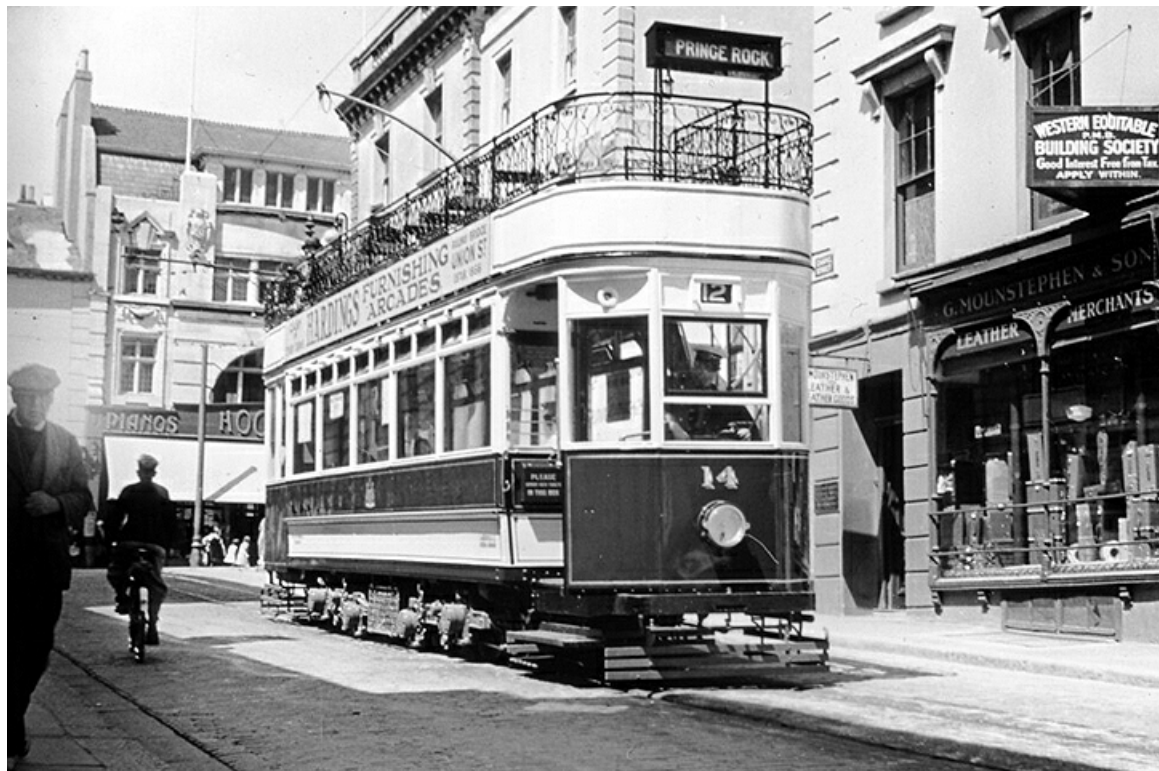
No. 14 was a Brush-built bogie car seating 76 formerly in the fleet of Torquay Tramways and was acquired in 1934. (LTHL collection).
