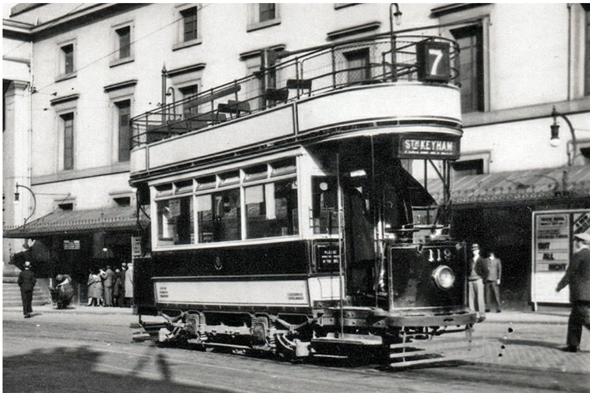
No. 119 en-route to South Keyham was an ex-Plymouth, Stonehouse & Devonport Tramways car acquired following the expiry of the lease in 1922. It was built by ERTCW on Brill 21E trucks. (LTHL collection).
