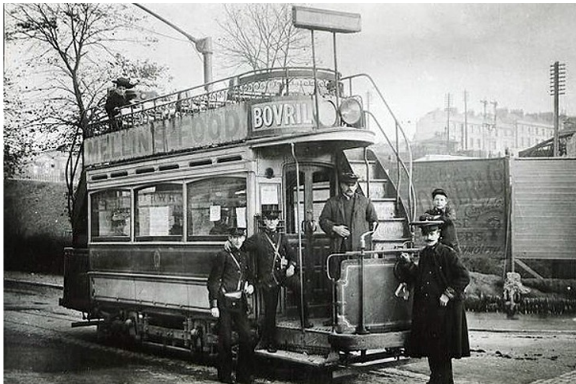
Tram No. 4 of the Devonport & District Tramways Company was built in America by Brill & Co of Philadelphia and seated 46. (LTHL collection).
