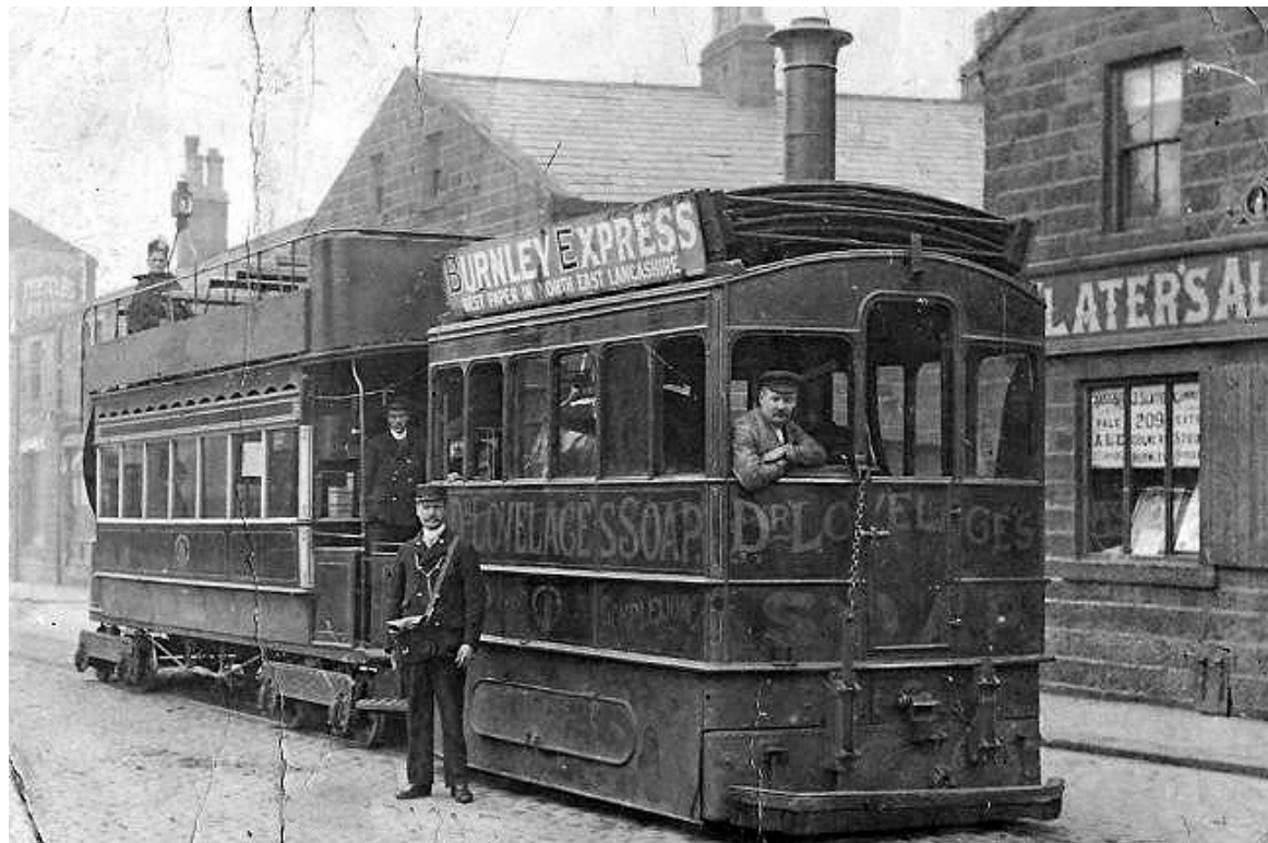
Falcon loco No. 8 of the Burnley & District Steam Tramways Company hauling trailer car No. 6. (LTHL collection).
