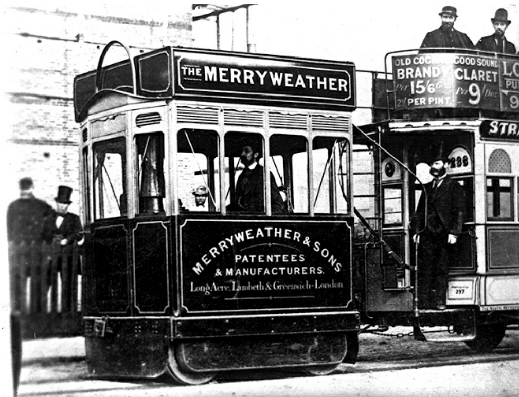
A Merryweather steam locomotive on trial with the North London Tramways in 1878. (LTHL collection).
