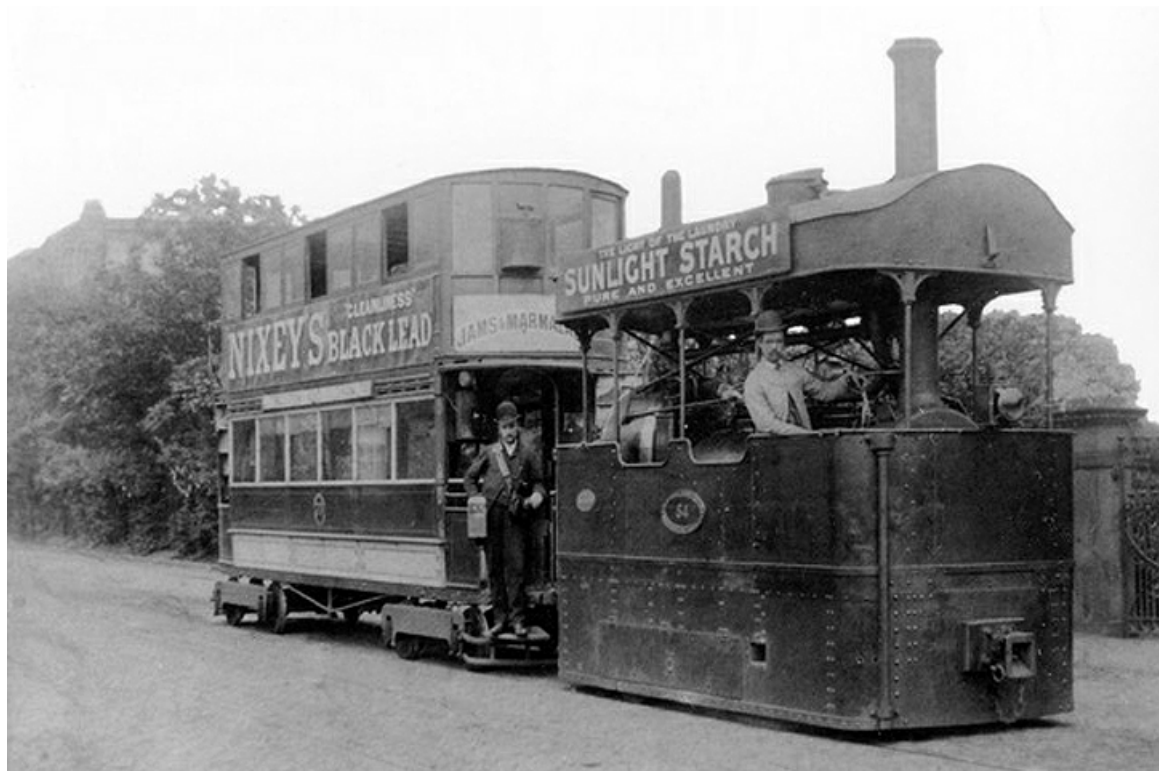
Built in 1885 was Manchester, Bury, Rochdale & Oldham Steam Tramways Company's No. 54, a Manning Wardle steam loco one of just 3 standard gauge locos built. (LTHL collection).
