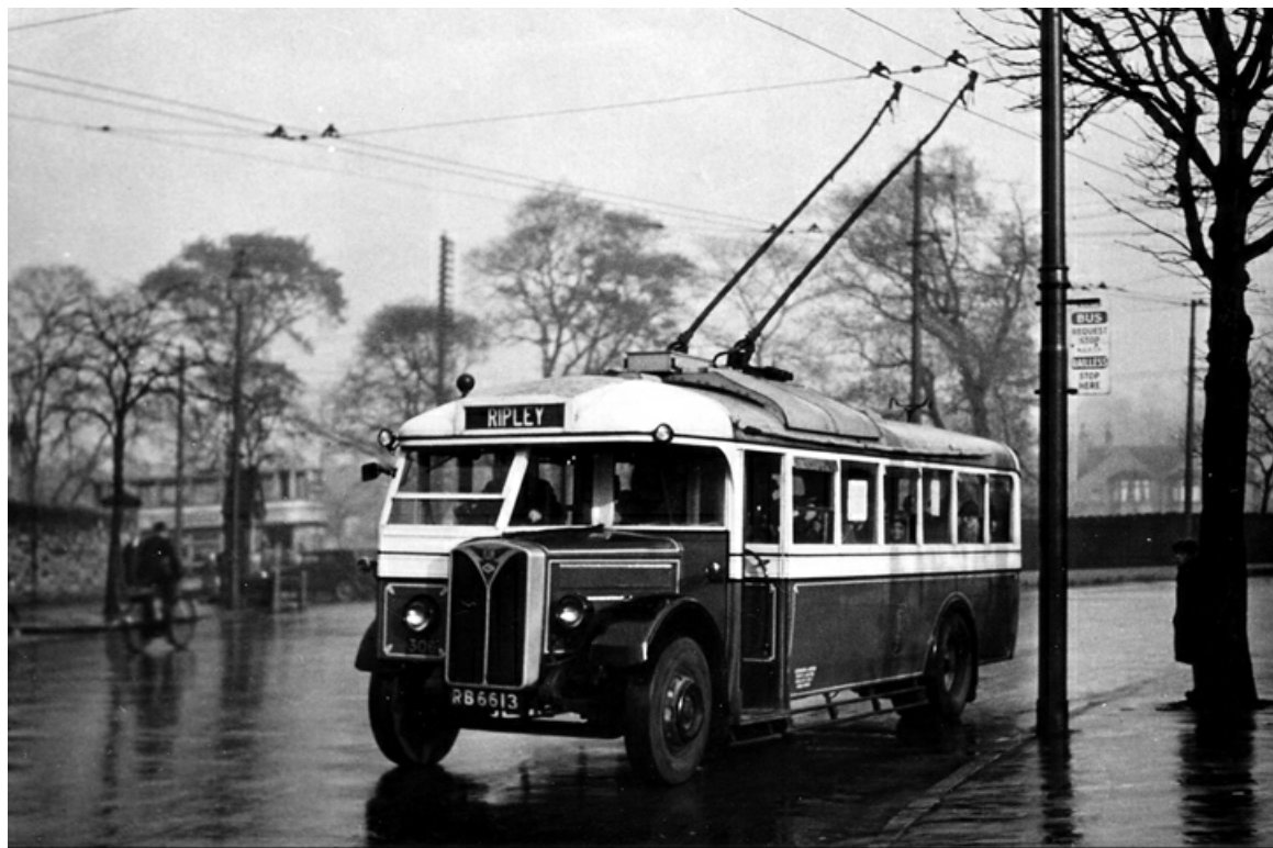
No. 306 (RB6613) was an AEC 662T trolleybus with English Electric B32F bodywork. (LTHL collection).
