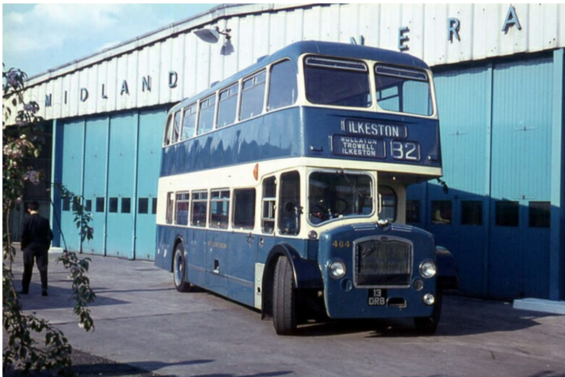
No. 464 (13DRB) was a solitary Bristol LD6G with ECW H37/33R bodywork that joined the fleet in 1957. (John Kaye).
