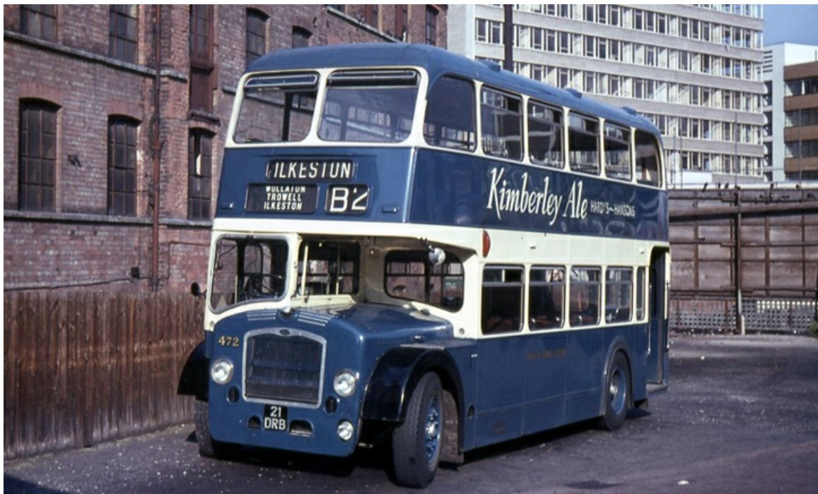
No. 472 (21DRB) was a Bristol LD6G with ECW H33/25R bodywork, seen here after platform doors had been fitted in 1964. (Brian Bennett).
