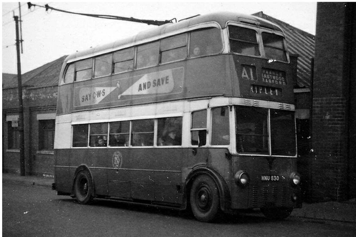
No. 337 (HNU830) was a 1941 AEC 661T trolleybus with Weymann H30/26R bodywork without the dummy radiator which by now was no longer in fashion. (LTHL collection).
