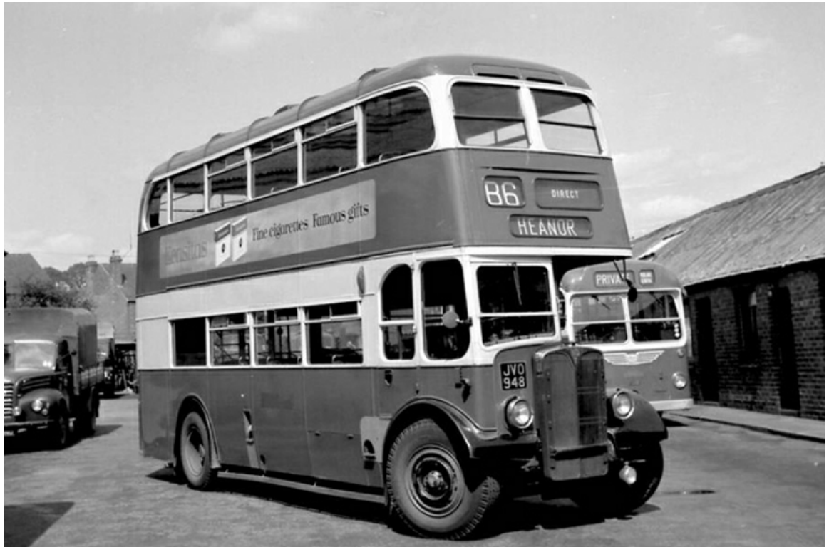
No. 322 (JV0948), a 1949 AEC Regent III with Weymann H30/26R bodywork that was transferred from the associated Mansfield & District Traction Company in 1953 for trolleybus replacement services. (John Boylett courtesy John Kaye).
