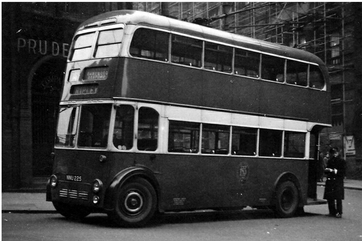
The last batch of trolleybuses arrived in 1949. This is No. 344 (NNU225), a BUT 9611T with Weymann H30/26R bodywork. (LTHL collection).
