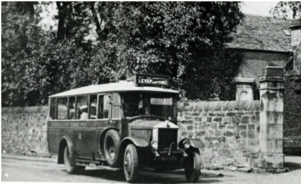
FG1938 was a 1926 Albion PJ26 with B25F bodywork probably by Cowieson and numbered 16. (LTHL collection).
