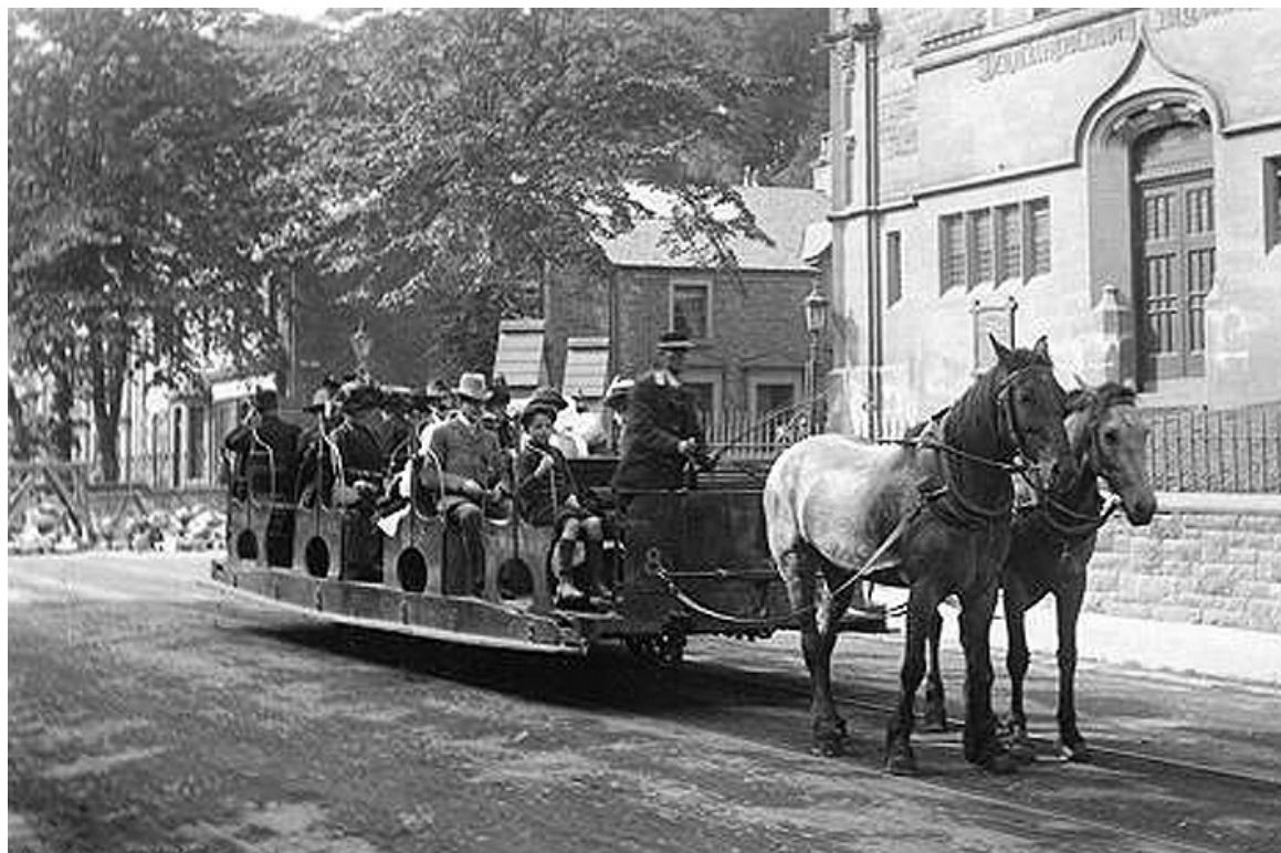
No. 8 of 1894 was a single-deck toastrack seating 32 built by an unknown builder. (LTHL collection).
