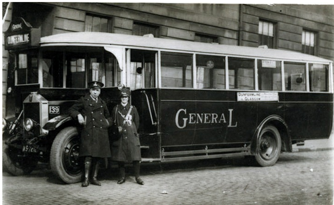
No. 139 (MS7212) was a 1927 Albion PM28 with B32F bodywork by an unknown builder. (LTHL collection).
