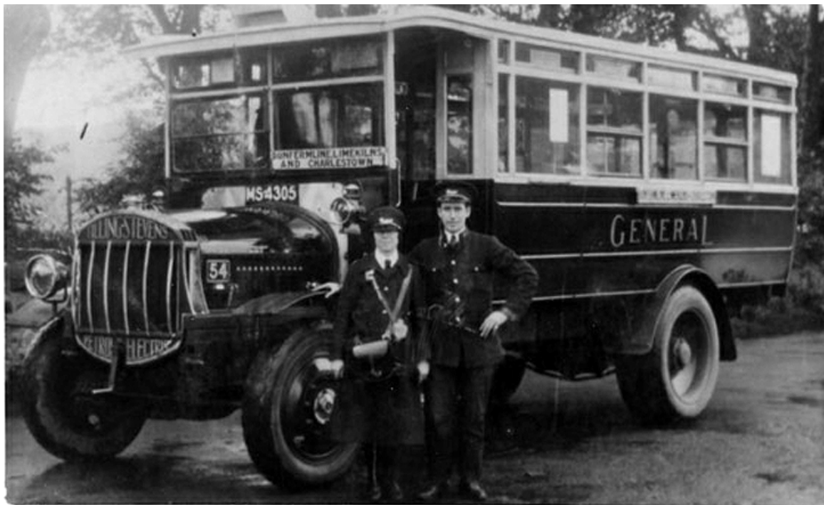
No. 54 (MS4305), a 1923 Tilling-Stevens with B26F bodywork by an unknown builder. (LTHL collection).
