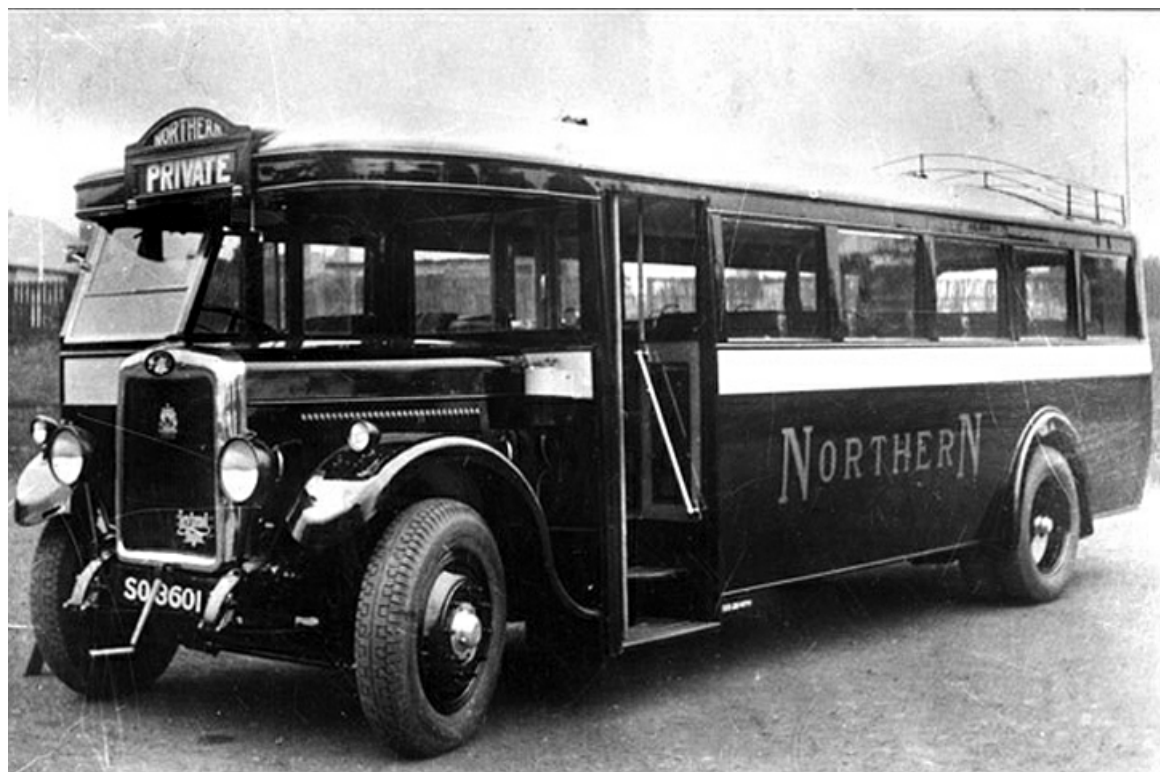
No. 172 (S03601) in the Scottish General (Northern) fleet was this 1929 Leyland TS2 with Stewart of Wishaw 32-seat bodywork. (LTHL collection).
