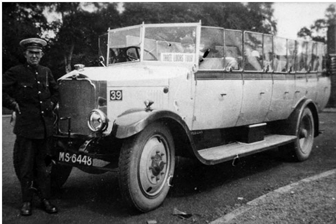
No. 39 (MS6448) was a 1926 Albion PF26 with this 18-seat charabanc body by an unknown builder about to depart on the 'Three Lochs Tour'. (LTHL collection).
