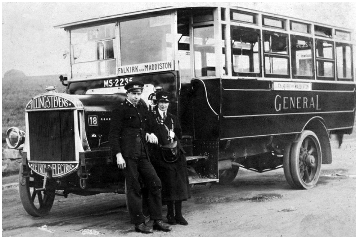
No. 18 (MS2235) was 1919 Tilling-Stevens TS3 with B24F bodywork by Cowieson. (LTHL collection).
