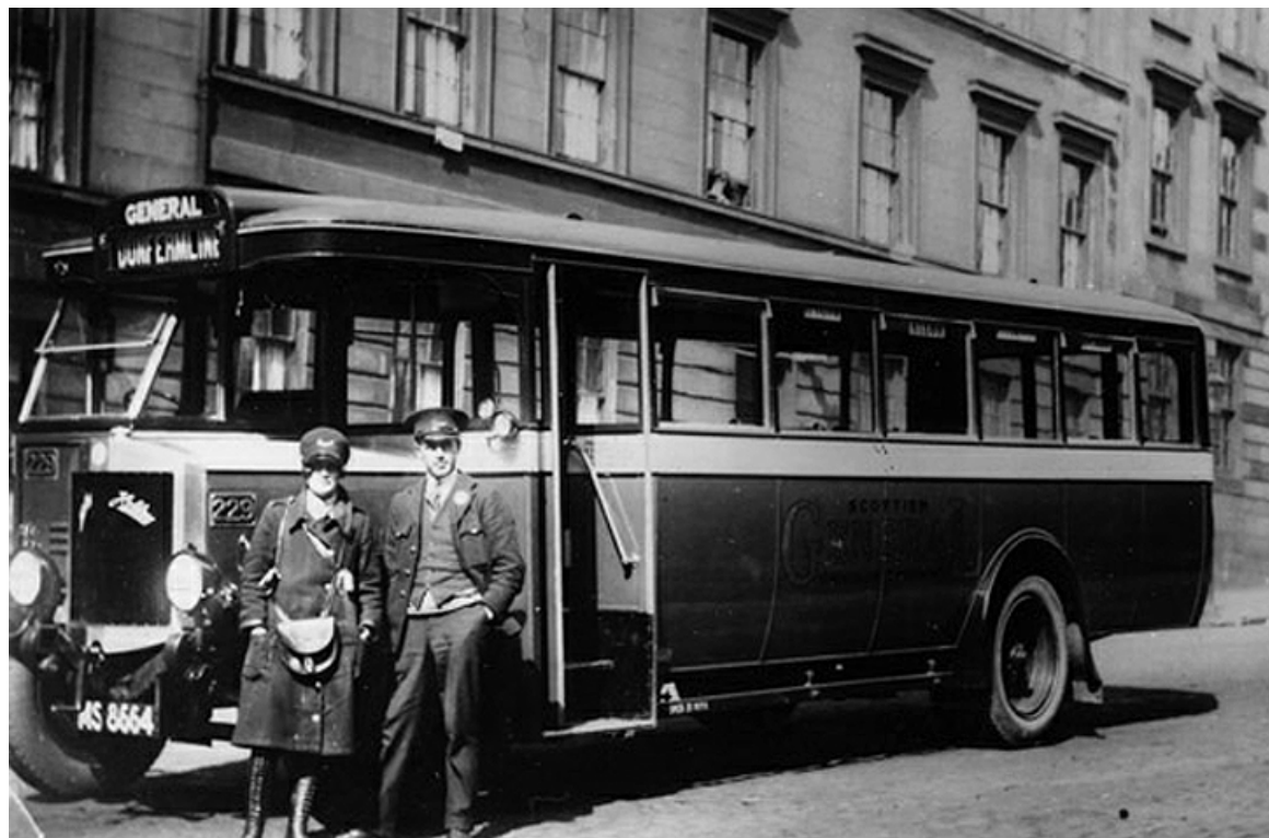
An unusual purchase in 1929 was No. 229 (MS8664) a Halley Conqueror with Cowieson B32F bodywork one of six new in May that year. (LTHL collection).
