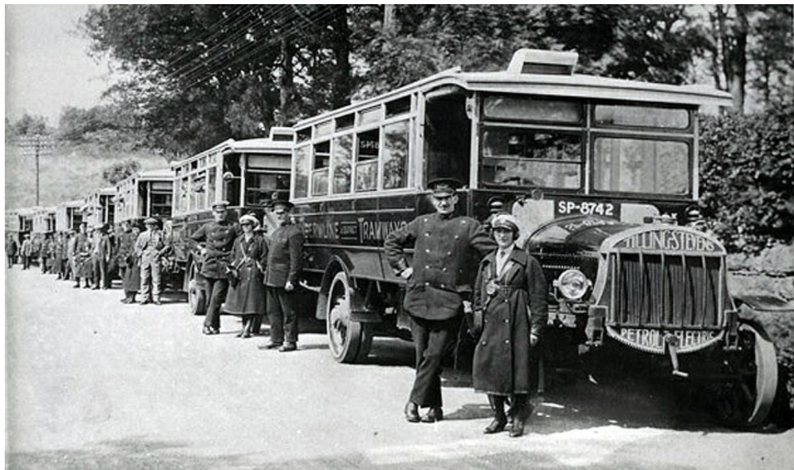
Heading this line up of Dunfermline buses is No. 2 (SP8742), a 1924 Tilling-Stevens TS3A with 26-seat bodywork by an unknown builder. It was re-numbered 96 in 1926. (LTHL collection).
