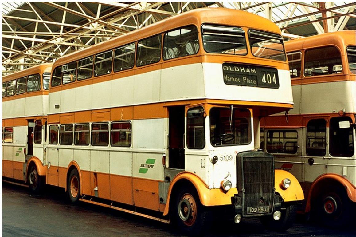
No. 5109 (109HBU), a Leyland PD3/5 with Roe H41/32F bodywork dating from 1964. (Richard Simons).
