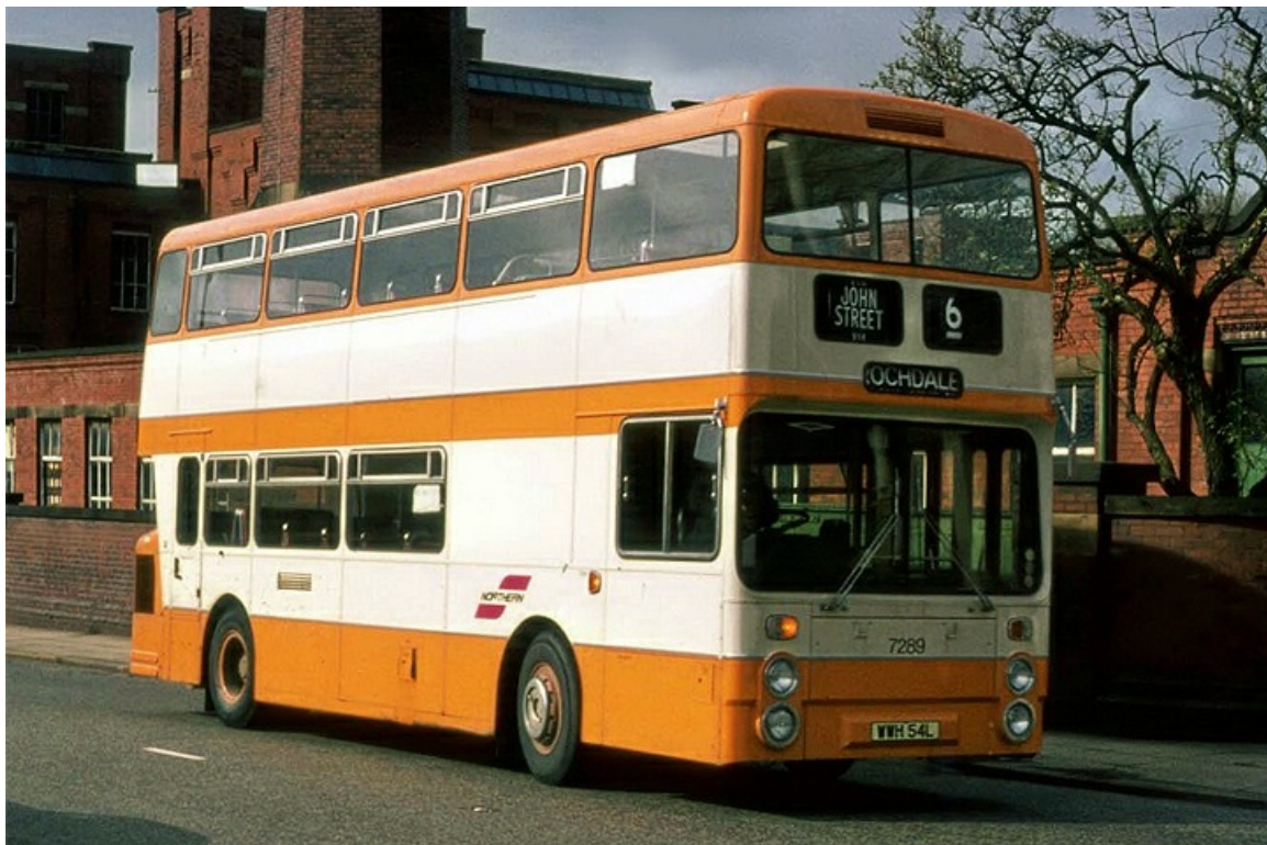
No. 7289 (WVH54L) was a dual-door Daimler CRG6LXB with Northern Counties 75-seat bodywork. (Derek Gordon).
