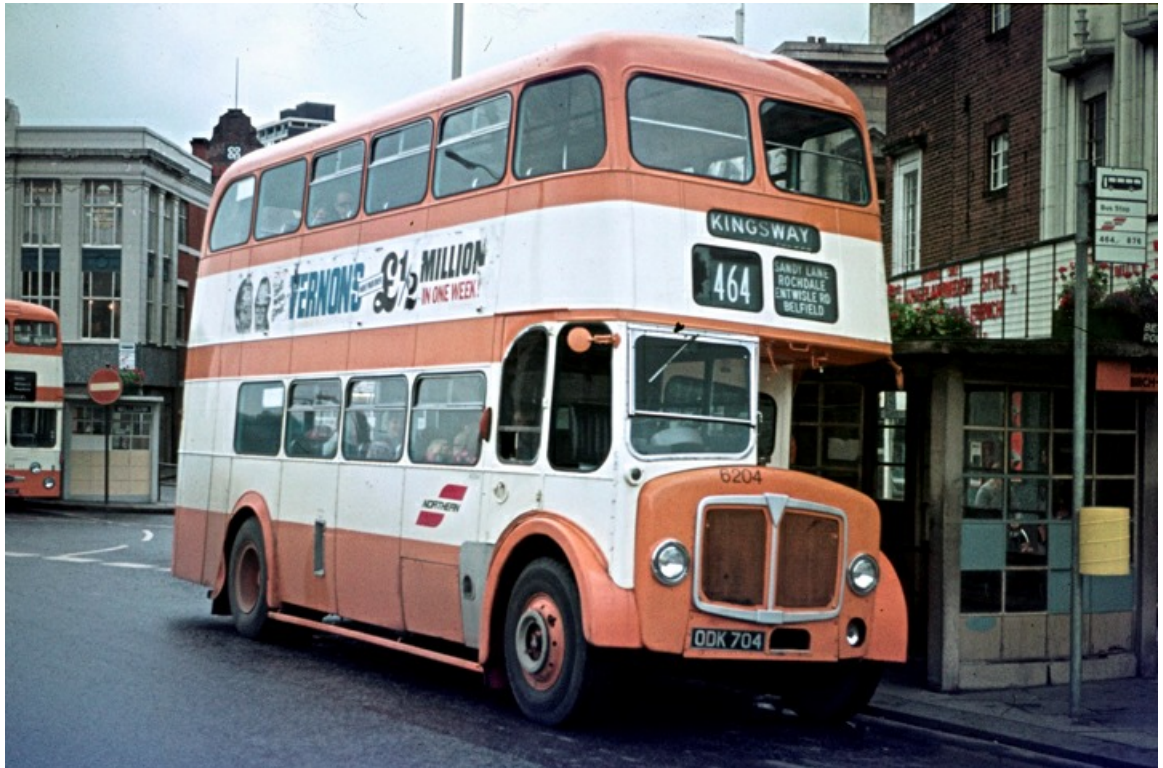
Ex-Rochdale AEC Regent V with Weymann H33/28R bodywork seen here numbered 6204 in the SELNEC fleet. (Richard Simons).
