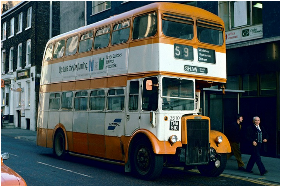
No. 3510 (TNA510) was a 1958 Leyland PD2/40 with Burlingham H37/28R bodywork. (Richard Simons).
