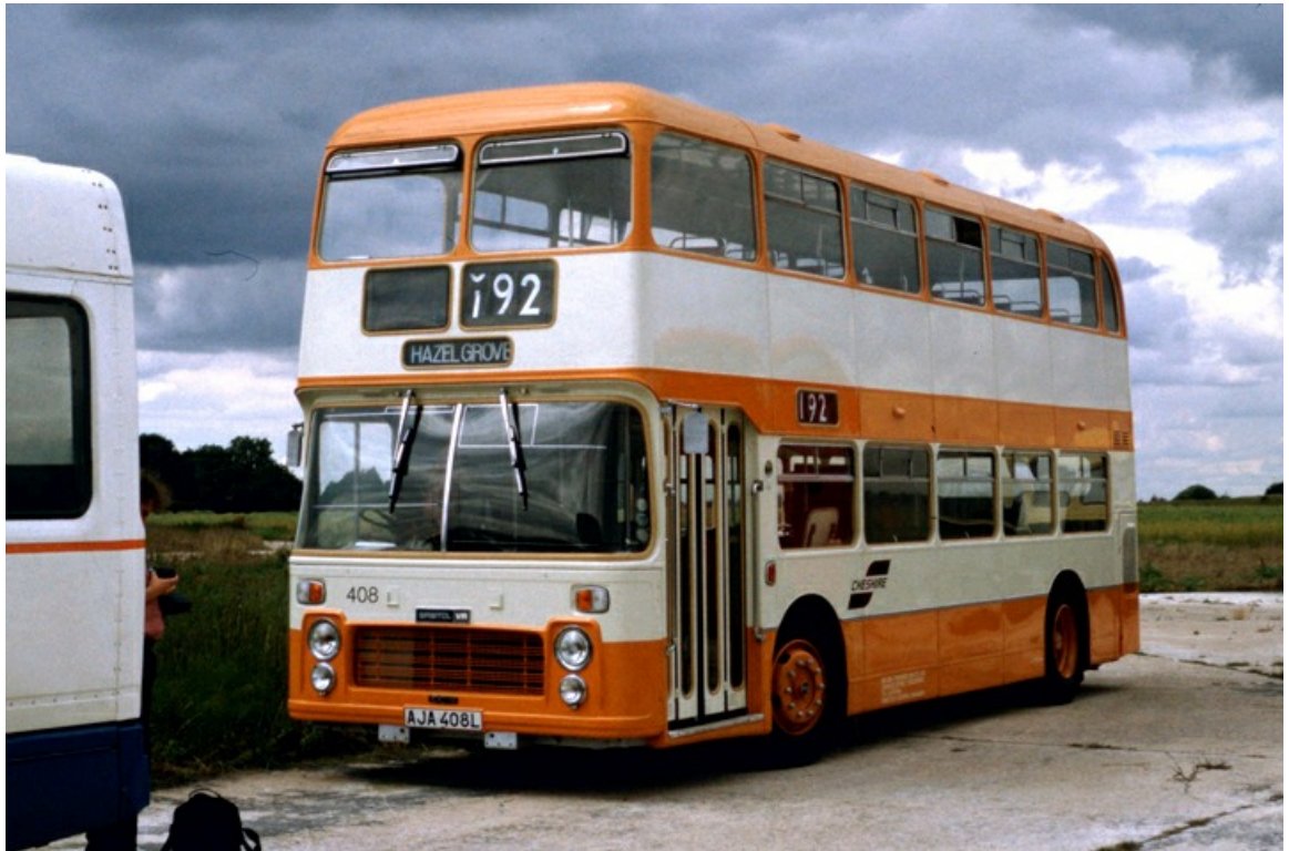
No 408 (AJA408L) was a Bristol VRTSL6G with ECW H43/32F bodywork ordered by North Western Road Car Company before the take-over. (Richard Simons).
