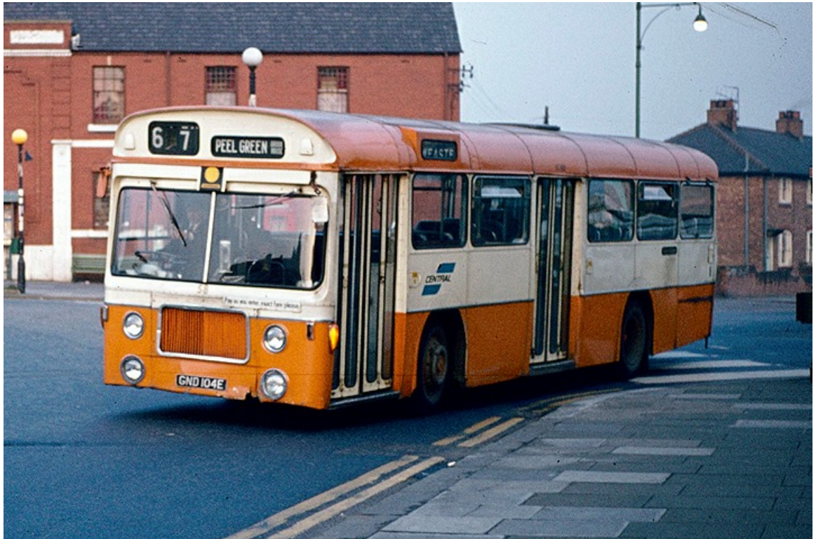
No. 58 (GND104E) was a Leyland PSUR1/1 with MCW B44D bodywork that was formerly Manchester Corporation No. 104 dating from 1967, and was re-numbered in the March 1970 scheme. (Richard Simons).
