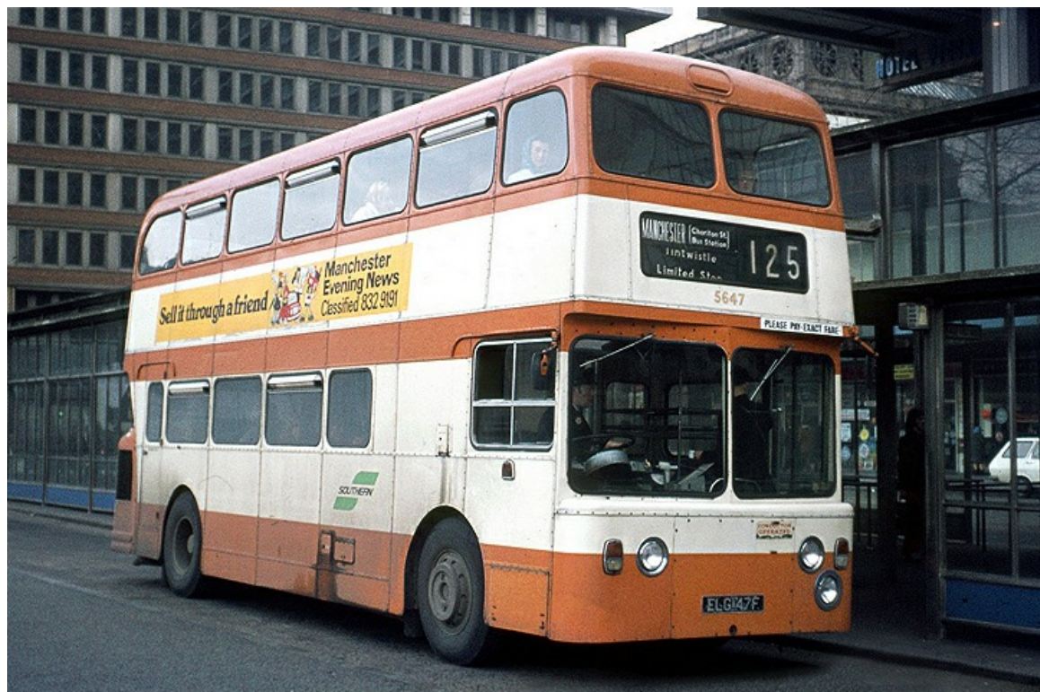
No. 5647 (ELG47F) a 1967 Daimler CRG6LW with Northern Counties H41/27D bodywork that came from the SHMD fleet. (LTHL collection).
