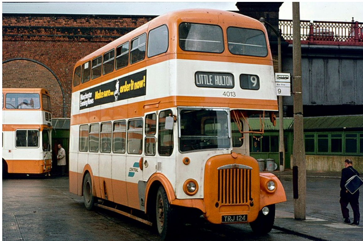
Seen in Victoria Bus Station is former Salford No. 124 (TRJ124), a 1962 Daimler CVG6 with MCW H37/28R bodywork, now sporting its SELNEC number 4013. (Richard Simons).
