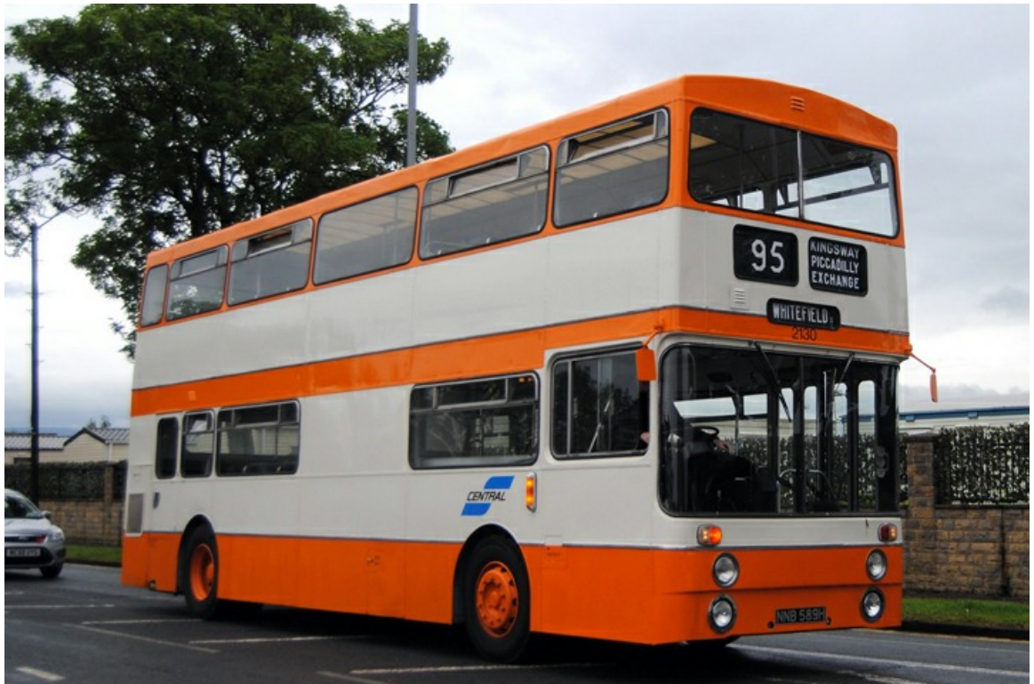
No. 2130 (NNB588H) was a 1970 Daimler CRG6LXB with Park Royal H47/28D bodywork, now in preservation. (Hesterjenna Photography).
