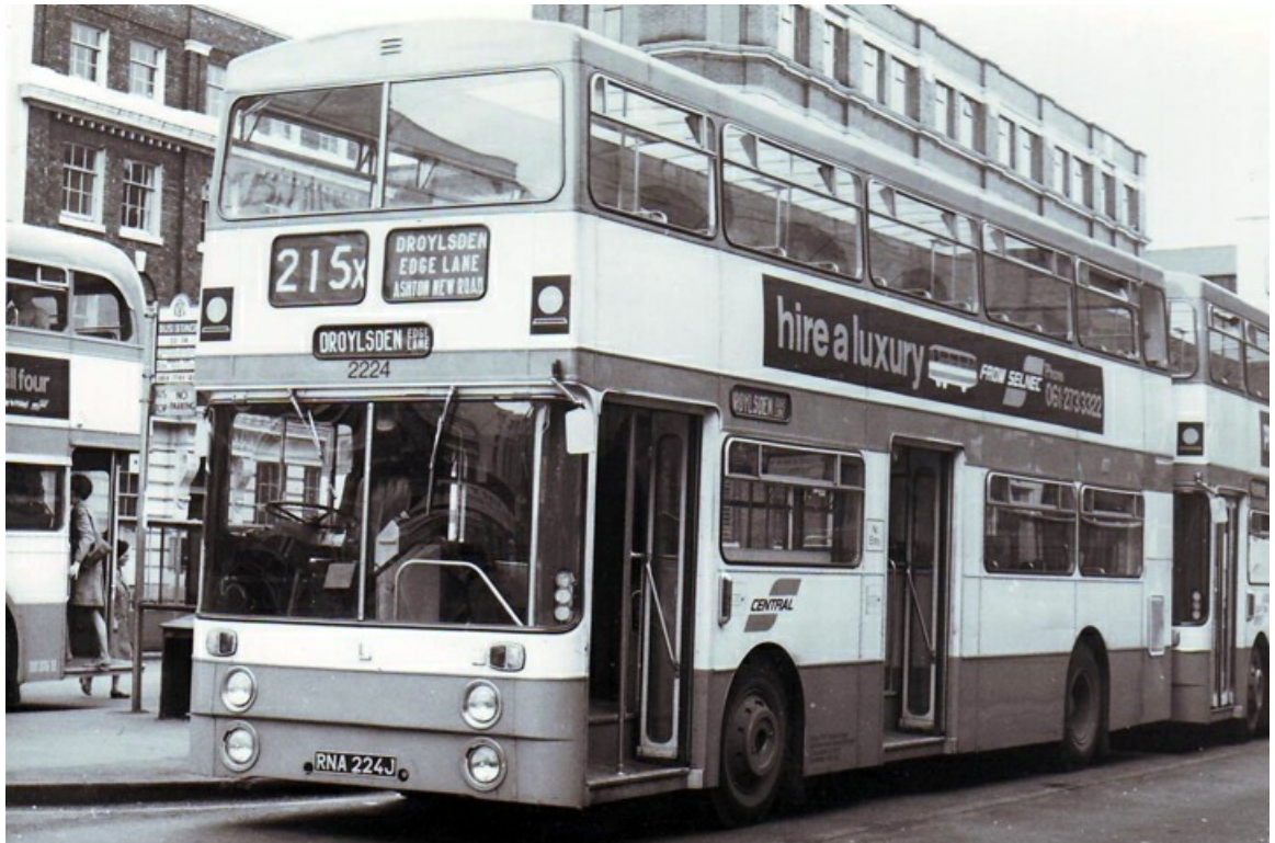
Central No. 2224 (RNA224J) was a 1971 Daimler CRG6LXB with Park Royal H47/29D bodywork. (Derek Gordon).
