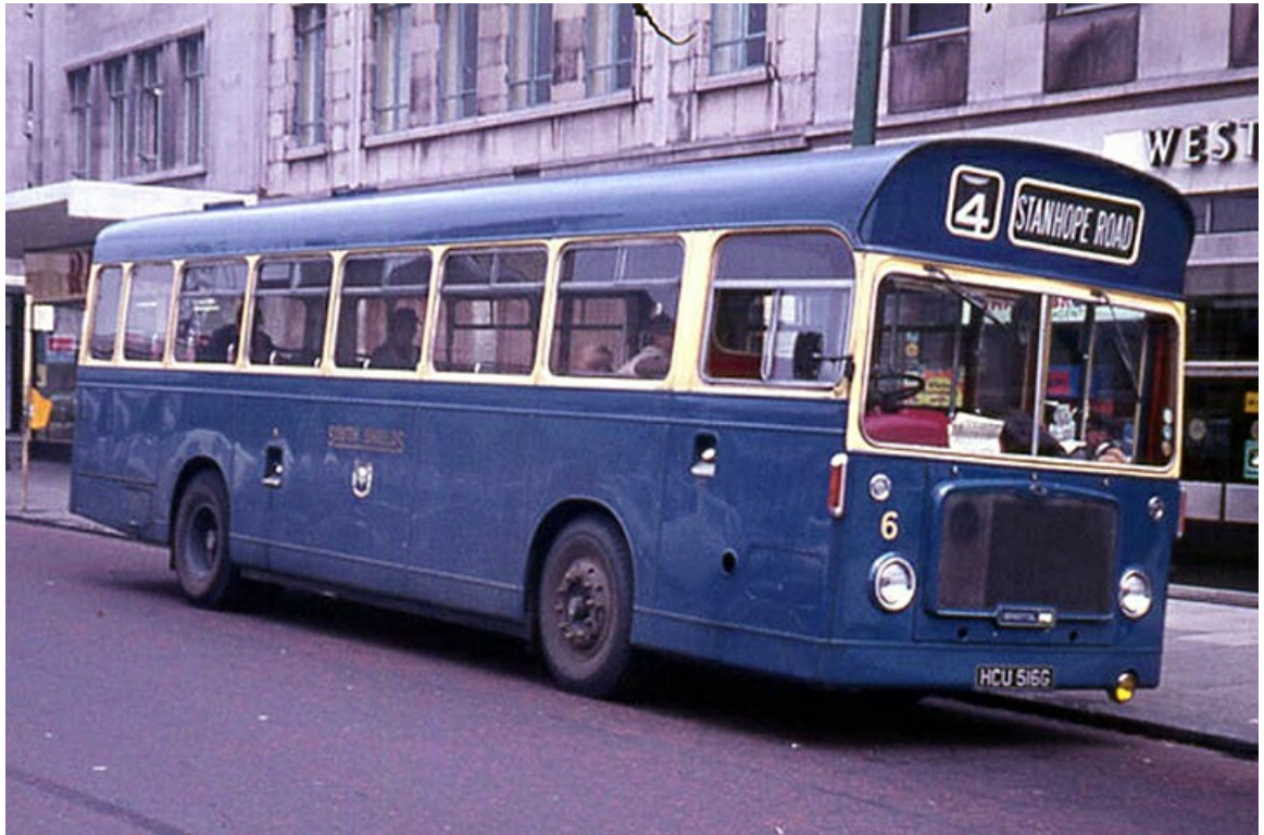
The final batch of vehicles were delivered in 1968 and included No. 6 (HCU516G) a Bristol RESL6L with ECW B45D bodywork. (John Kaye).
