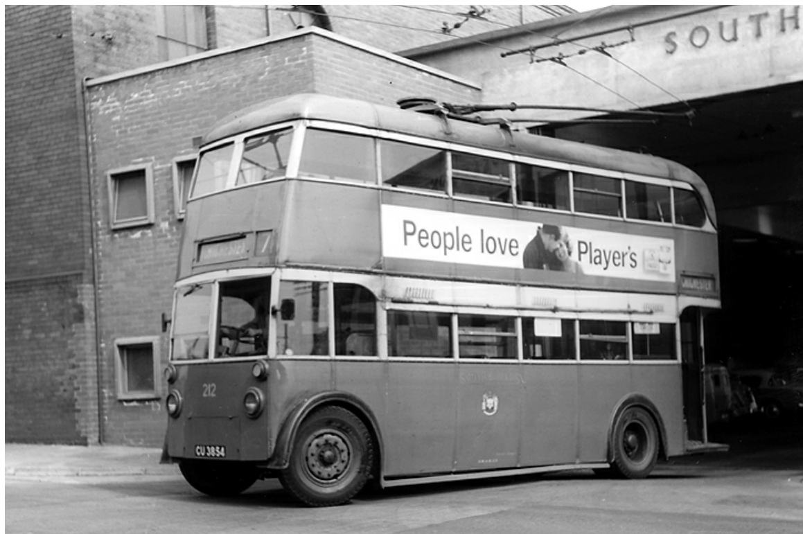
No. 212 (CU3854) was a 1938 Karrier E4 with Weymann H29/26R bodywork seen emerging from Dean Street depot. (Bus Archive).
