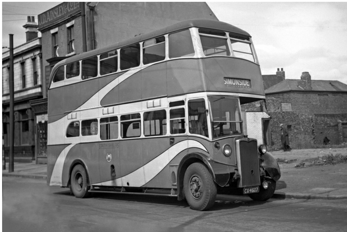
Wearing Manchester-style streamline livery is No. 134 (CU4607) a 1946 Crossley DD42/3T with Crossley H30/26R bodywork. (Bus Archive).
