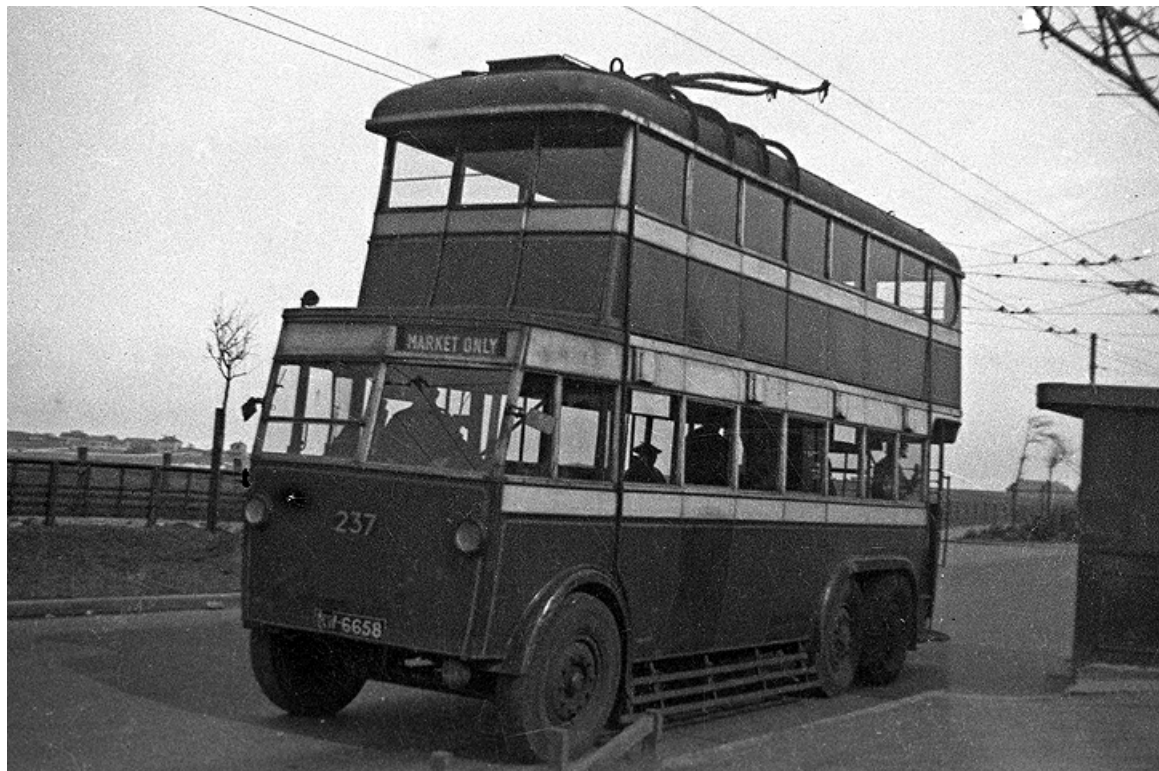
No. 237 (KW6658) was a second-hand purchase from Bradford Corporation in 1945. It was a six-wheel English Electric E11 with a rather dated looking English Electric H30/26R body. It was withdrawn in 1946. (LTHL collection).
