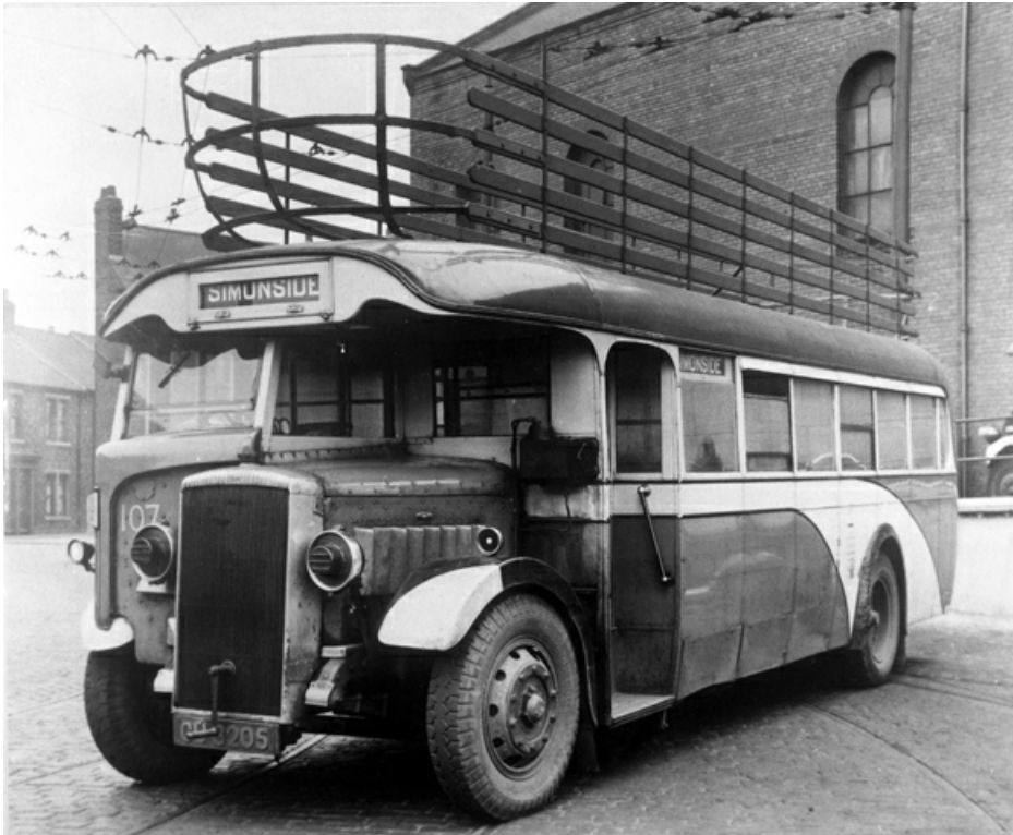
No. 107 (CU3205) a 1934 Daimler COG5 with Weymann 32-seat bodywork was formerly No. 5 and was fitted with a roof support for a gas bag during 1940, but in the event this vehicle never operated on town gas. (Bus Archive).
