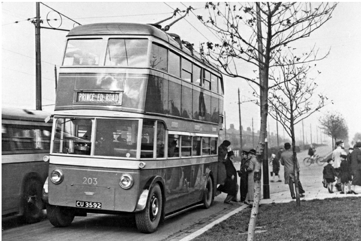
No. 203 (CU3592) was a 1936 Karrier E4. Its original body was destroyed by enemy action in 1941 so it was re-bodied with a new Weymann H30/26R body in 1942 as seen here. (Bus Archive).
