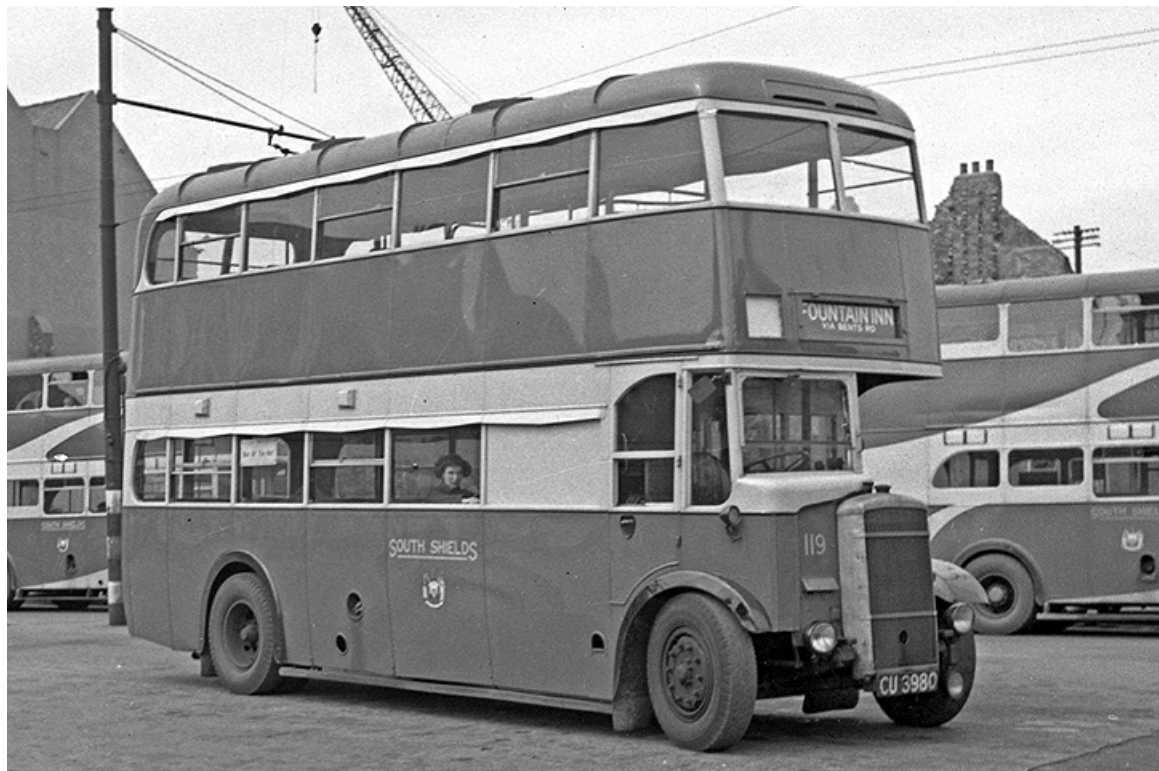
No. 119 (CU3980) was a 1938 Daimler COG5 with Weymann 55-seat forward entrance bodywork. (Bus Archive).
