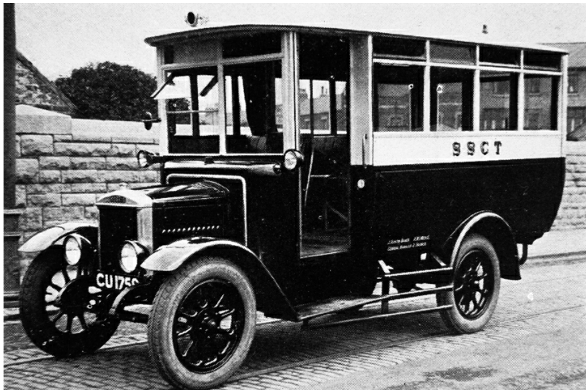
CU1760 was a 1925 Moris 1-ton chassis with Davidson 14-seat bodywork. It was later named 'Commerce' and withdrawn in 1932 (Bus Archive).
