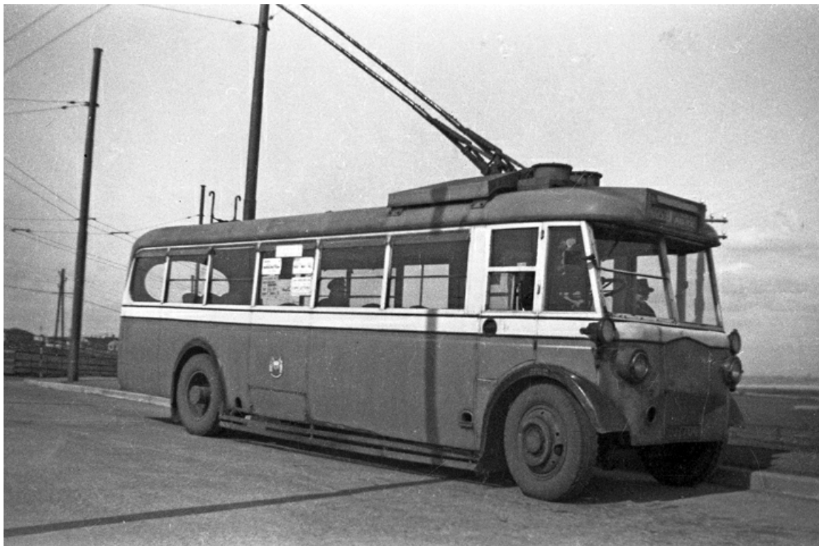
South Shields only single-deck trolleybus was No. 236 (LJ7704), a 1933 Thornycroft BD with Brush 32-seat centre-entrance bodywork purchased in 1942 from Bournemouth Corporation and it remained in the fleet until 1960. (Bus Archive).
