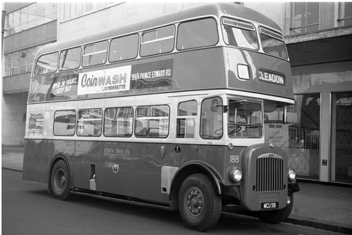
No. 188 (MCU56) was a 1964 Daimler CCG6 with Roe H35/28R. It passed to Tyneside PTE in 1/70. (John Law).
