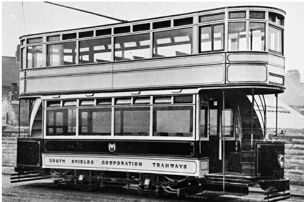
1906 UEC-built car No. 14 is seen here after being fitted with its fully-enclosed top-deck. It survived in this form until 1938. (Bus Archive).
