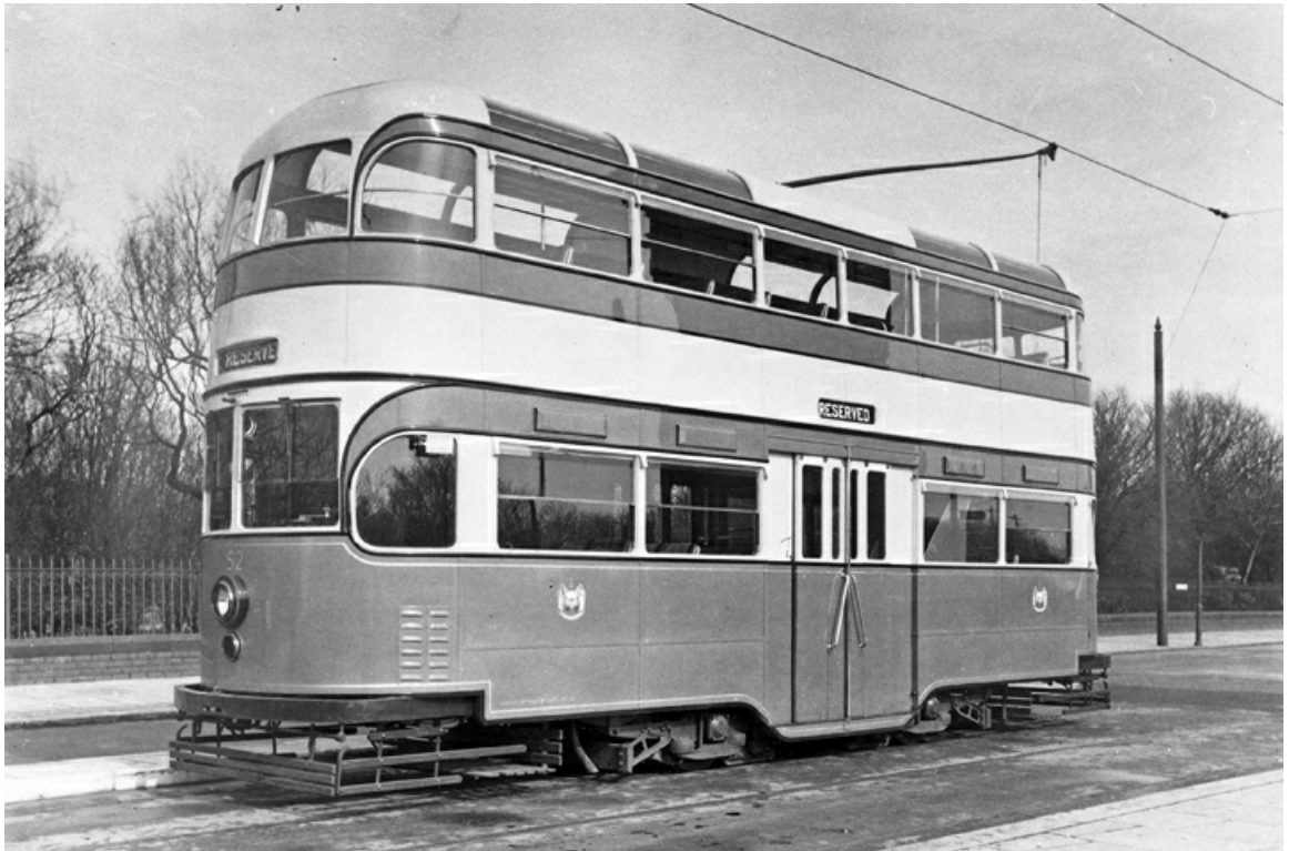
The only modern car in the South Shields fleet was No. 52, a 1936 Brush-built fully-enclosed car seating 60. It remained in service until the end of the system in 1946. (Bus Archive).
