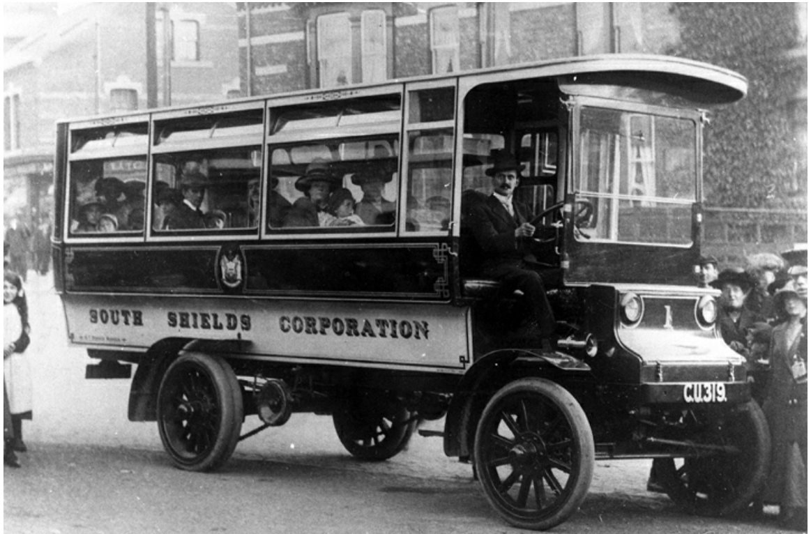
South Shields first buses were two Edison battery-electric buses. This is No. 1 (CU319) of 1914, which carried a Hora 22-seat body. (Bus Archive).
