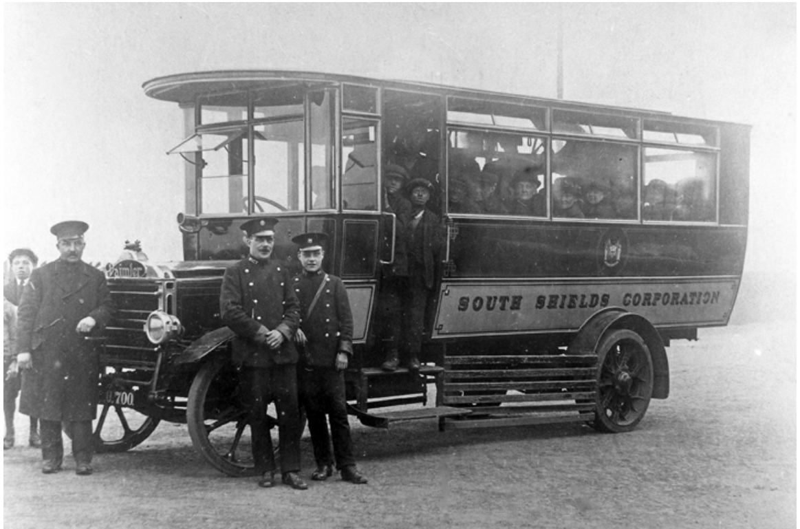
South Shields second No. 1 was this 1919 Daimler CJ (CU700), which had the same Hora 22-seat body that was fitted to the original No. 1, although modified to fit the new chassis. (Bus Archive).
