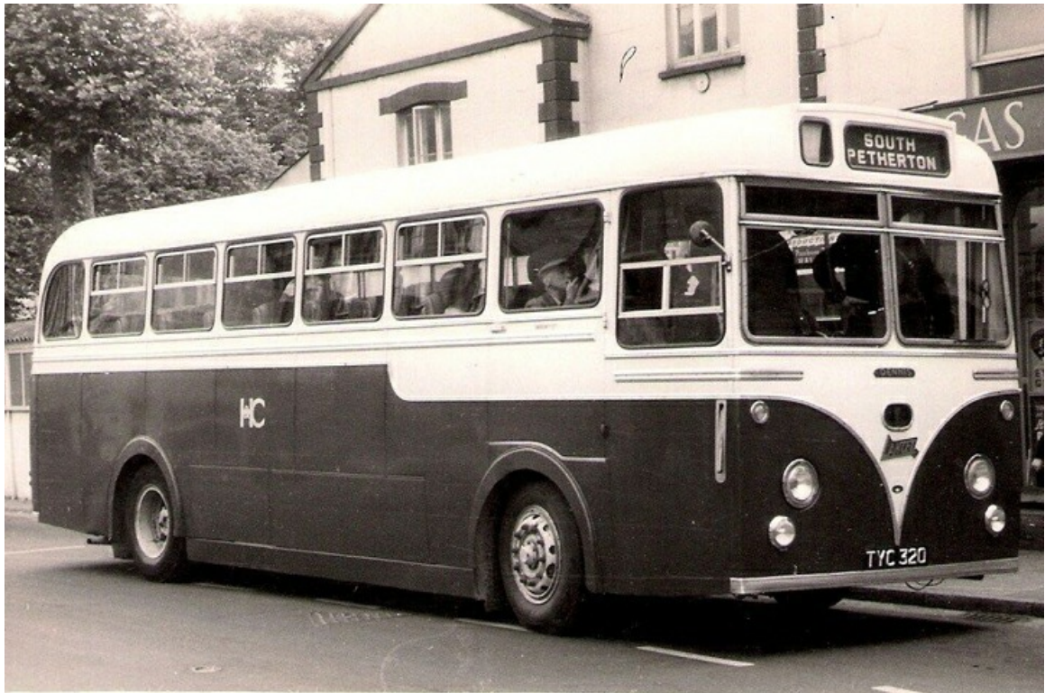
Heading for South Petherton is TYC320 a 1955 Dennis Lancet LU2 with Strachans DP41F bodywork. (LTHL collection).
