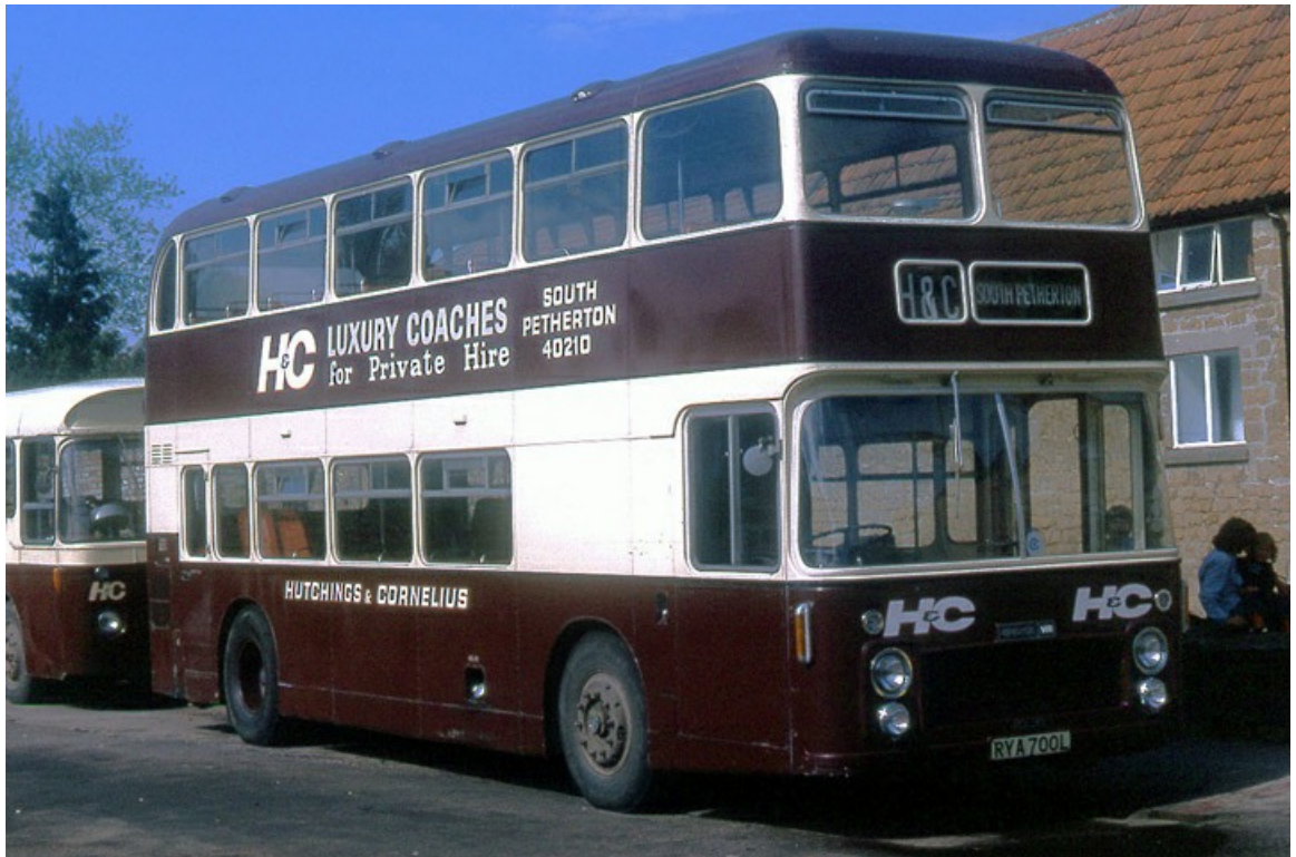
RYA700L was the replacement for the 1958 flagship Dennis Loline and was a Bristol VRT with ECW H39/31F bodywork that enabled H&C to complete 100% one-man operation. (John Law).
