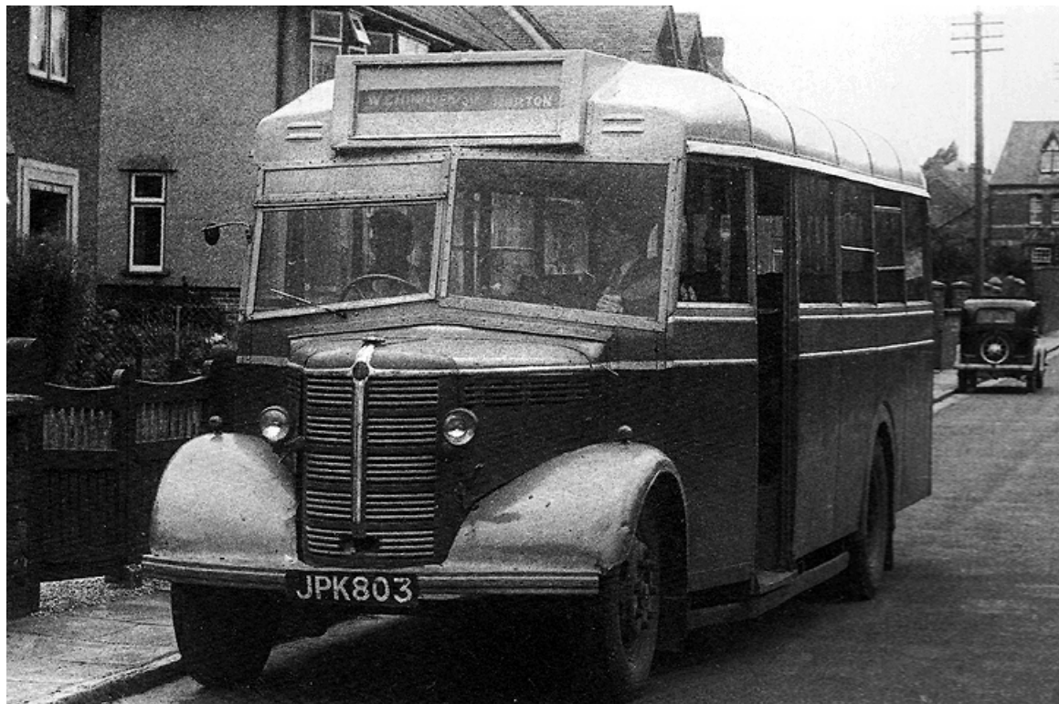
JPK803 was a 1942 Bedford OVB with Mulliner B30F bodywork that had been new to Yellow Bus of Stoughton before joining H&C in 1947. (Bus Archive)
