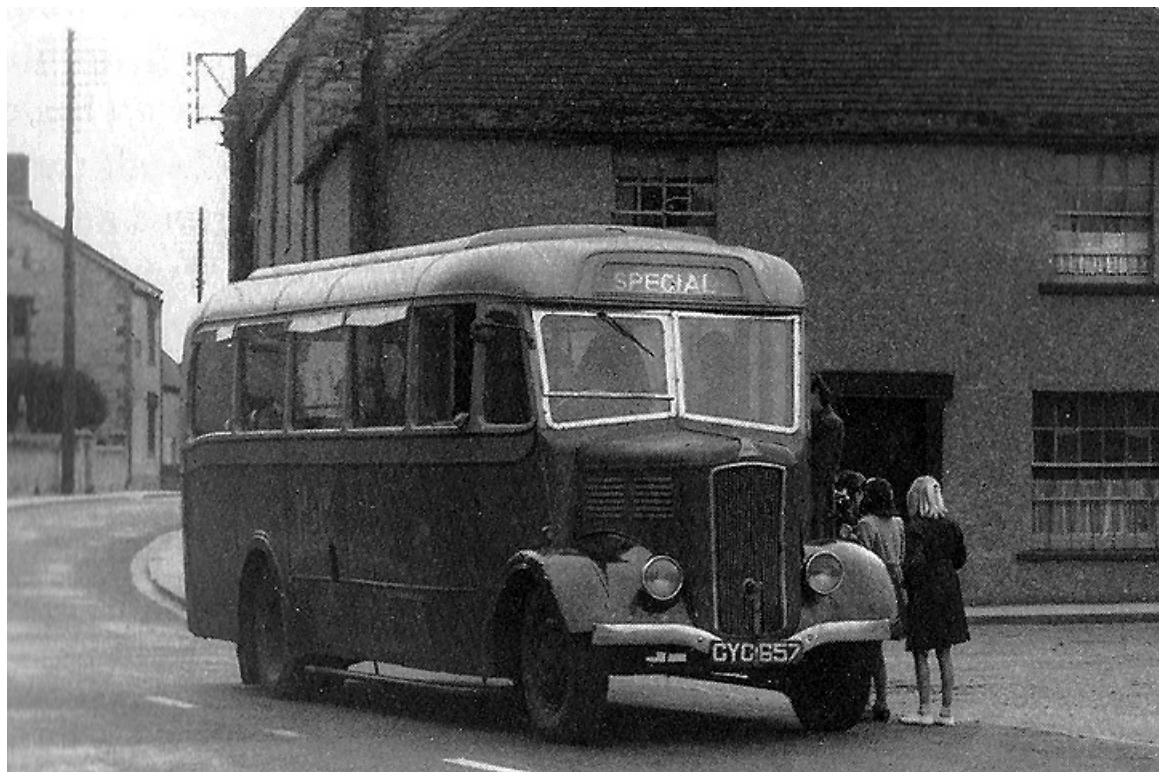
CYC657 was a 1937 Dennis Arrow Minor with Dennis B26F bodywork, seen here on a private hire away from H&C's usual operating area. (Bus Archive).
