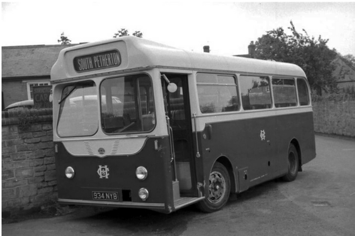
1962 Albion Nimbus NS3AN 934NYB with Harrington B31F bodywork is seen at the garage in South Petherton in June 1968. (John Boylett courtesy John Kaye).
