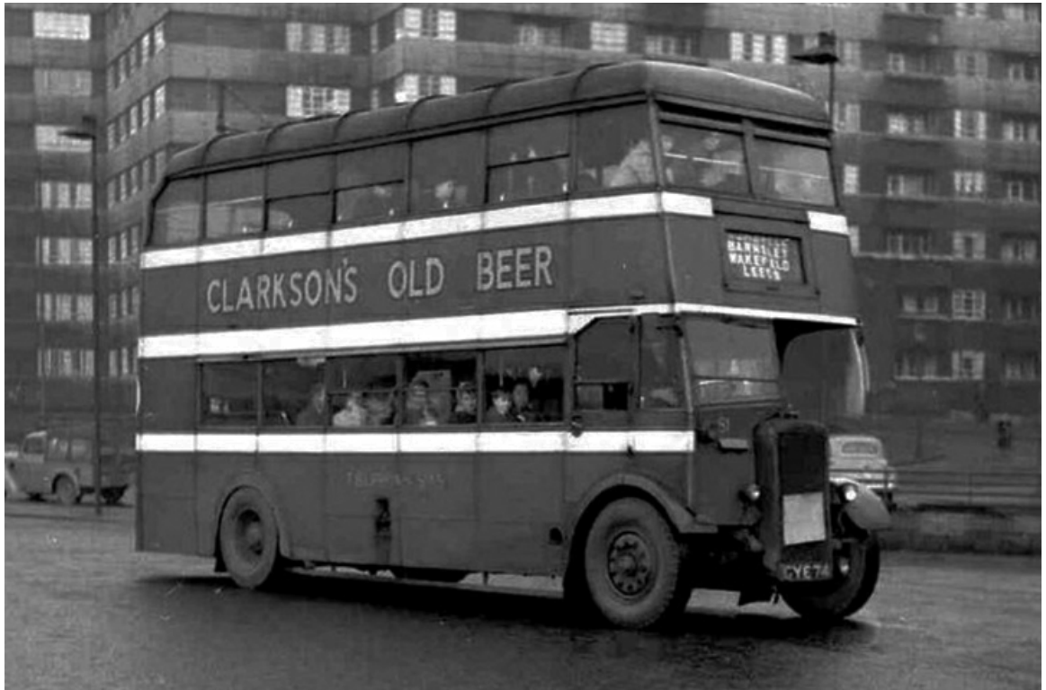
No. 81 (GYE74) was one of three ex-London Transport Daimler CWA6's purchased in 1953. It was new in 1946 and carried a Duple H30/26R body which was replaced with a new Burlingham H33/28RD body in 1957. (John Kaye).
