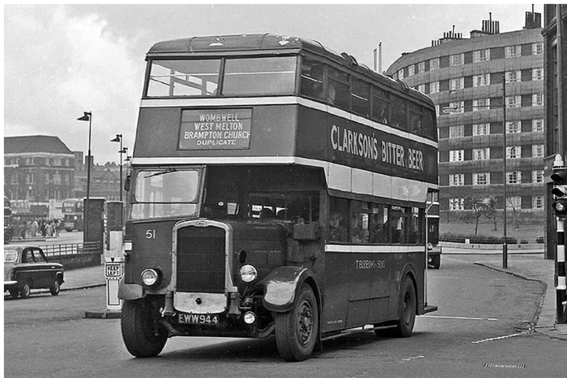
No. 51 (EWW944) was one of a pair of Bristol K6A chassis with Strachans L27/28R bodywork purchased in 1945. This particular vehicle was withdrawn in 1958. (LTHL collection).
