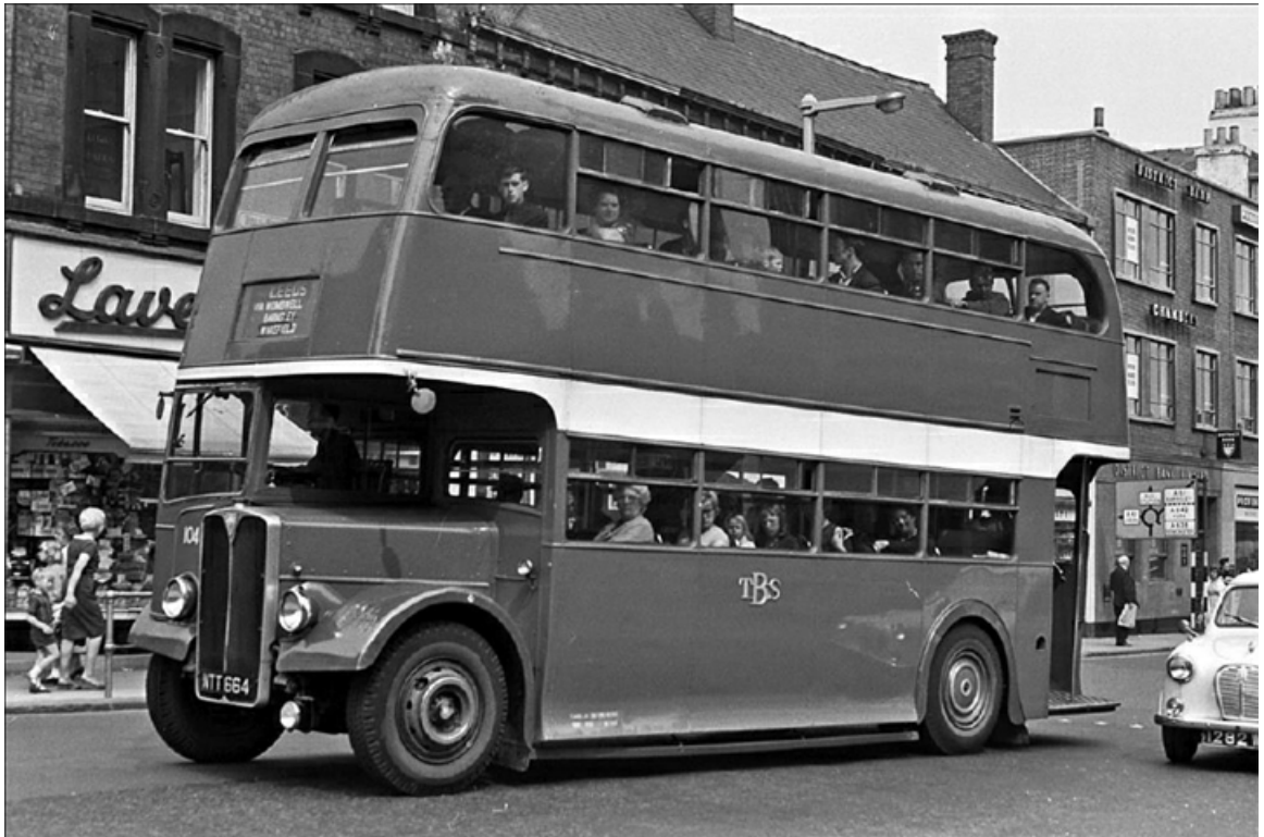
In 1965 Burrows purchased a quartet of former Devon General AEC Regent III's with Weymann H30/26R bodywork new in 1952. This is No. 104 (NTT664) en route to Leeds. (LTHL collection).
