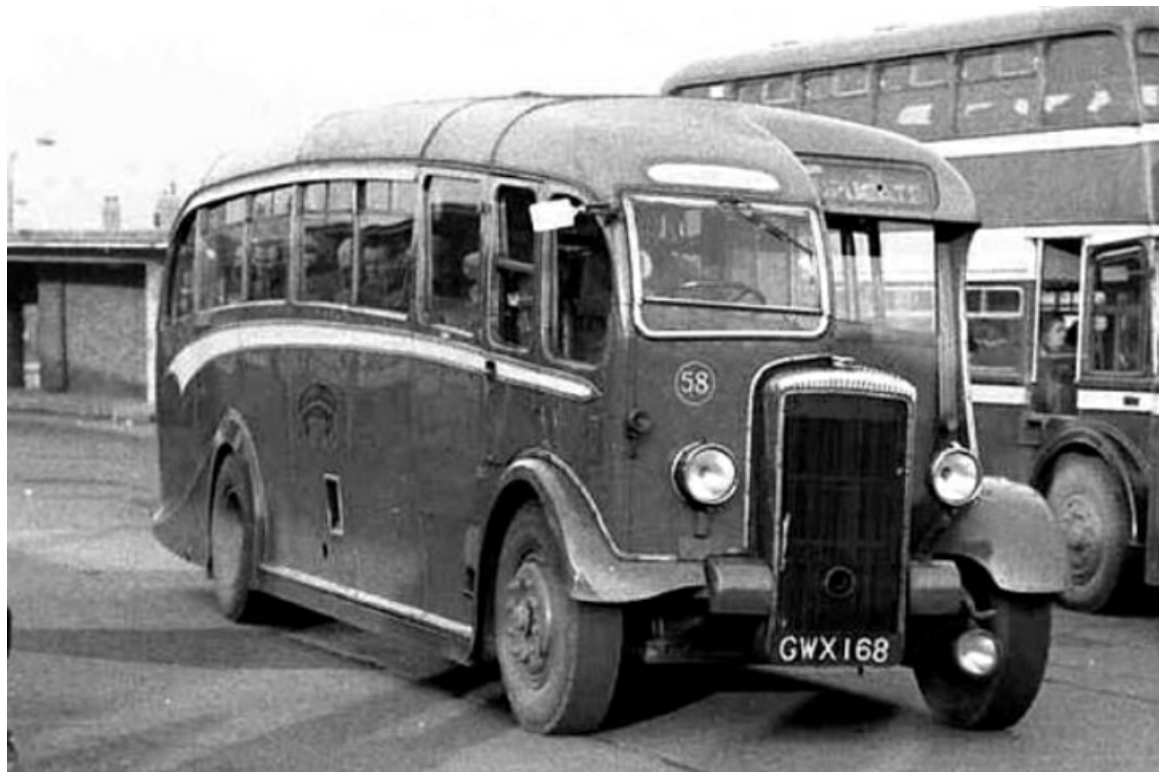
No. 58 (GWX168) was a 1948 Daimler CVD6 with Wilks & Meade C33F bodywork. (John Kaye).
