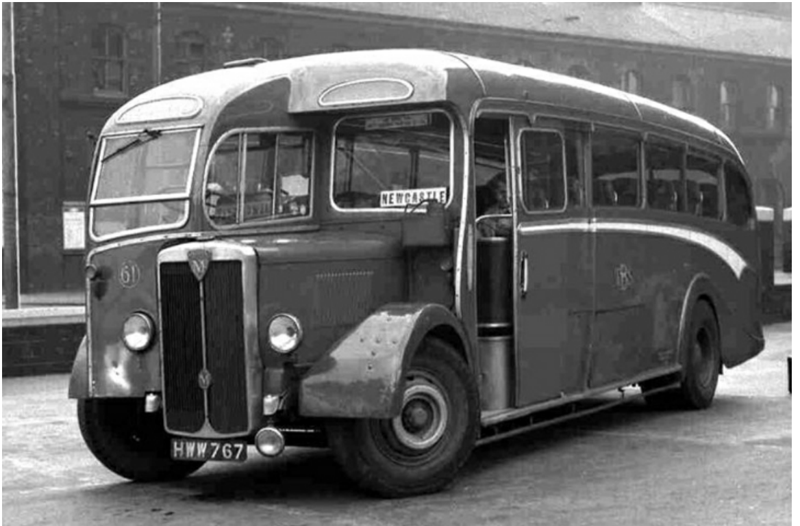
No. 61 (HWW767) purchased in 1949 was a Maudslay Marathon III with Duple C33F coachwork. {John Kaye}.
