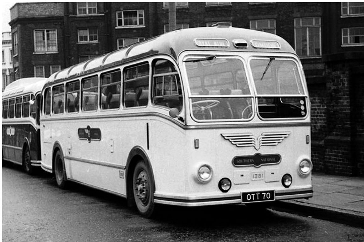
No. 1361 (OTT70), a 1953 Bristol LS5G with ECW C41F coachwork, seen here in June 1958 parked at Ebury Bridge, close to London Victoria Coach Station. (John Boylett courtesy John Kaye).
