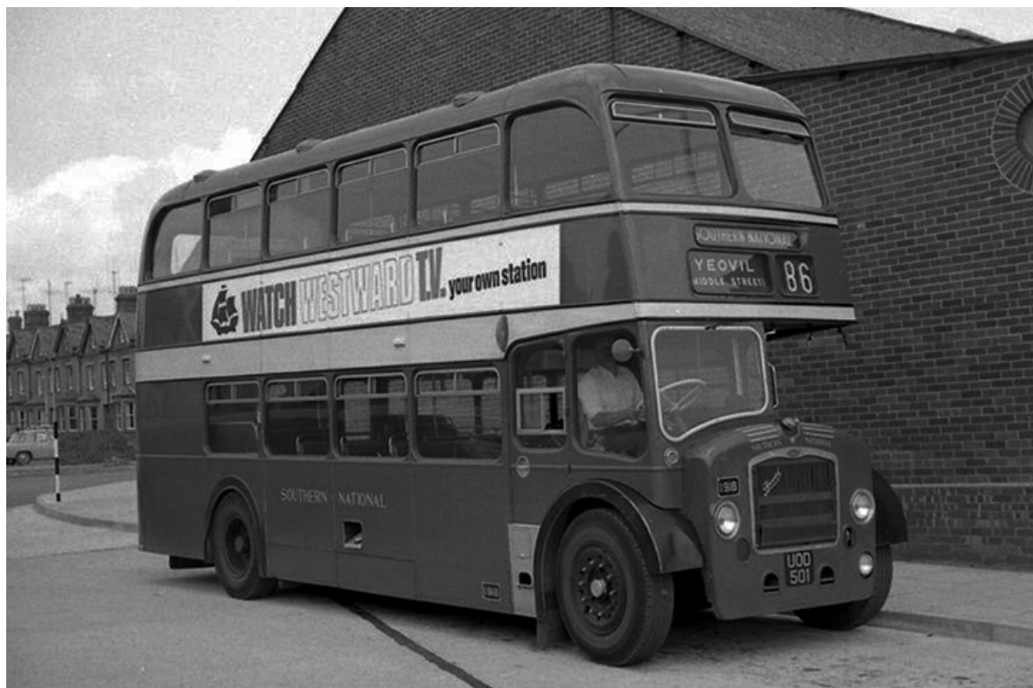
No. 1918 (UOD501) was a 1957 Bristol LD6B with ECW H33/27RD bodywork. (John Boylett courtesy John Kaye).
