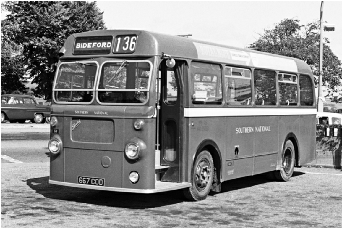
No. 611 (667COD) was a 1960 Bristol SUS4A with ECW B30F bodywork. In 1969 it passed to Western National with the rest of the Southern National fleet. (LTHL collection).
