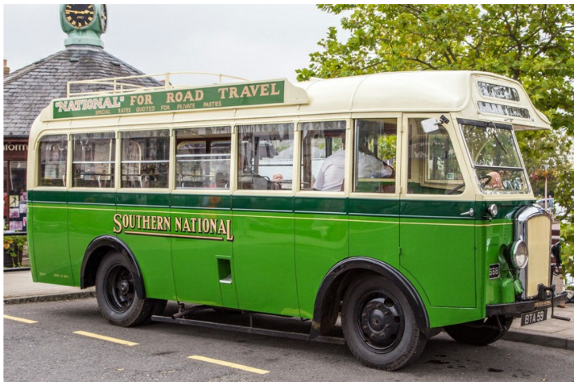
Dennis Mace No. 668 (BAT59), now in preservation, dates from 1934 and carries an Eastern Counties B26F body. (LTHL collection).
