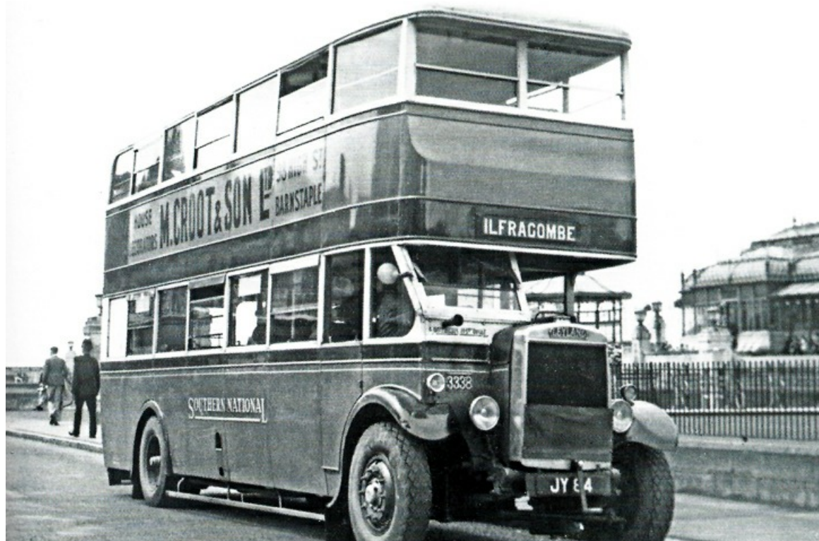
No. 3338 (JY84) was a 1932 Leyland TD2 with Strachans L27/28R bodywork which was later re-bodied by Beadle, continuing in service for a total of 23 years. (LTHL collection).
