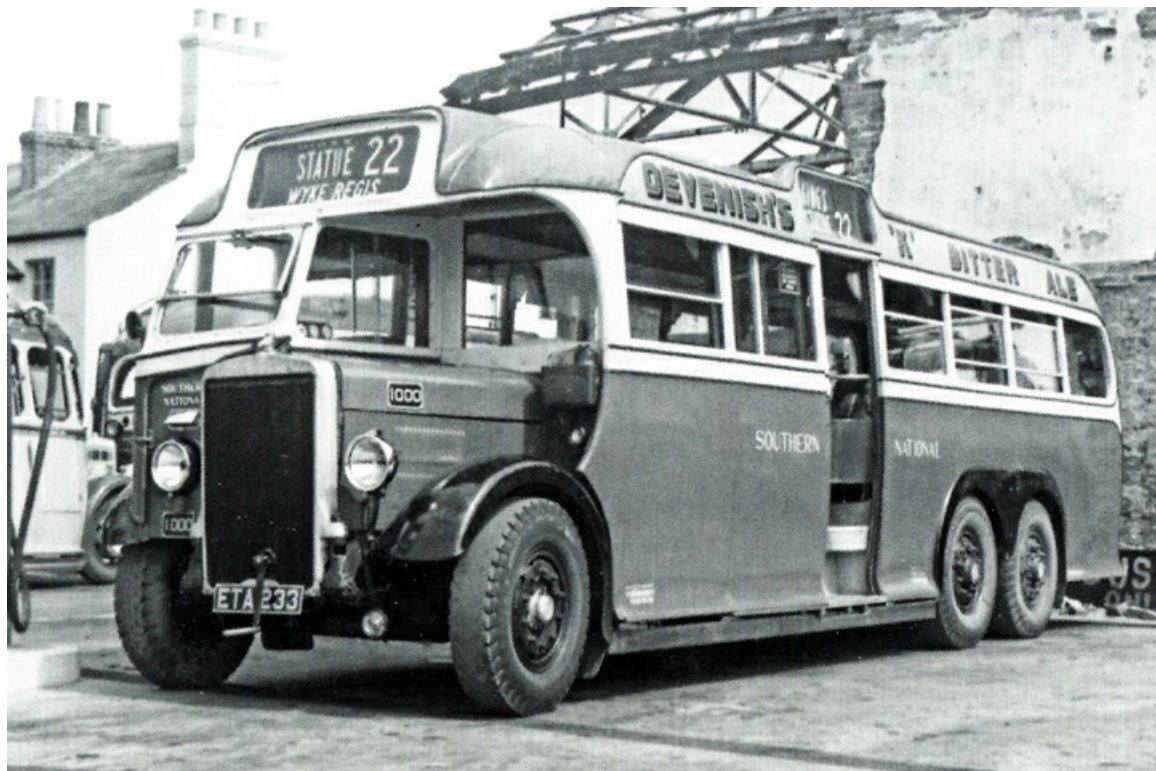
No. 1000 (ETA233) was one of 6 Leyland TS7D six-wheel chassis with Beadle 44-seat centre-entrance bodywork dating from 1937. All spent their working lives on the Weymouth-Portland services. (LTHL collection).
