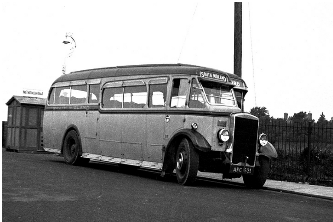
No. 33 (AFC531) was a Leyland TS6 with Harrington 32-seat coachwork dating from 1934. (Bus Archive).
