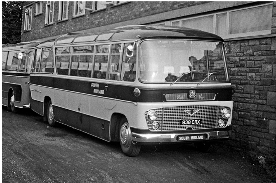
No. C408 (838CRX) was a Bedford SB13 with Duple 37-seat coachwork, one of three similar vehicles that joined the fleet in 1964. (Bus Archive).
