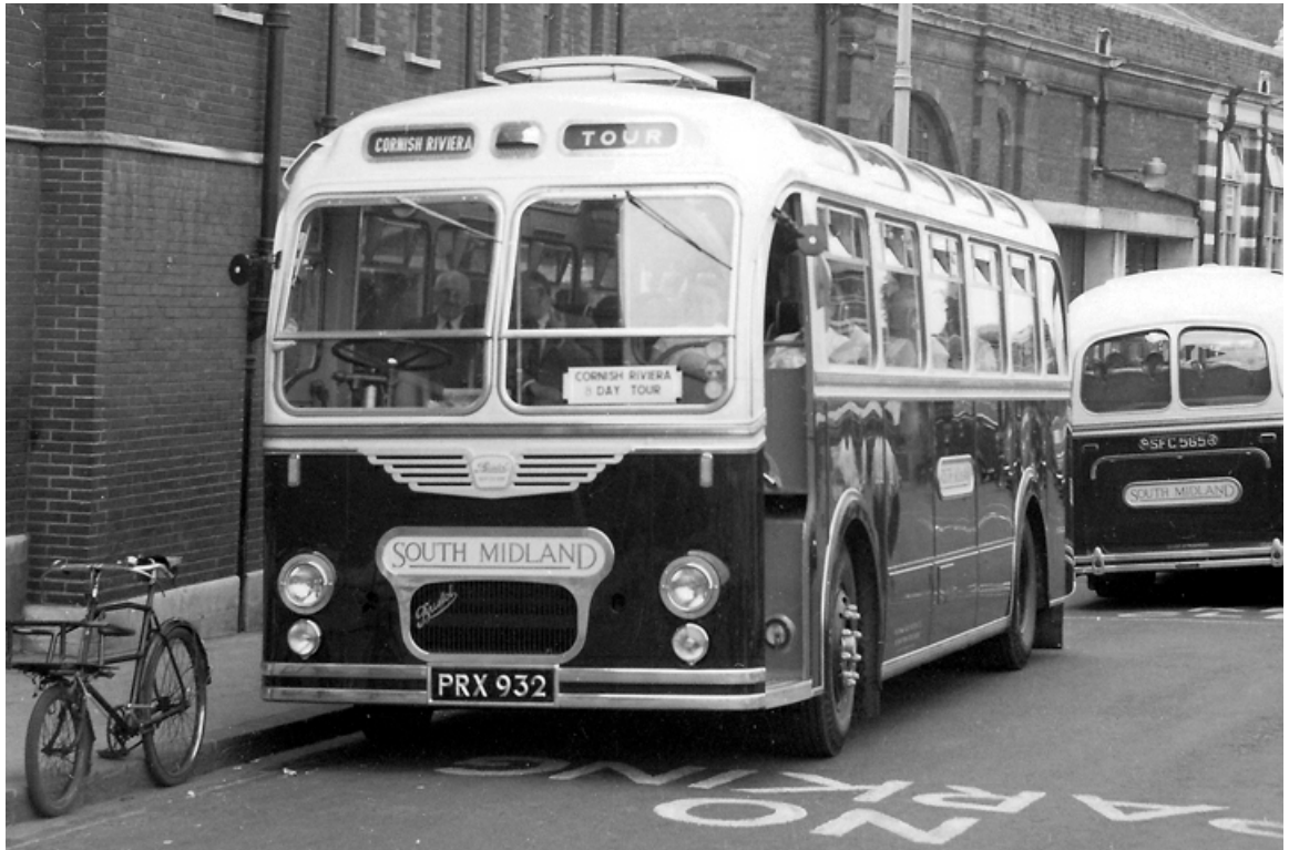
From 1954 vehicles had been numbered in the main Thames Valley fleet. No. 806 (PRX932) was a 1959 Bristol MW6G with ECW 34-seat coachwork, later re-seated to 38-seat. (Bus Archive).
