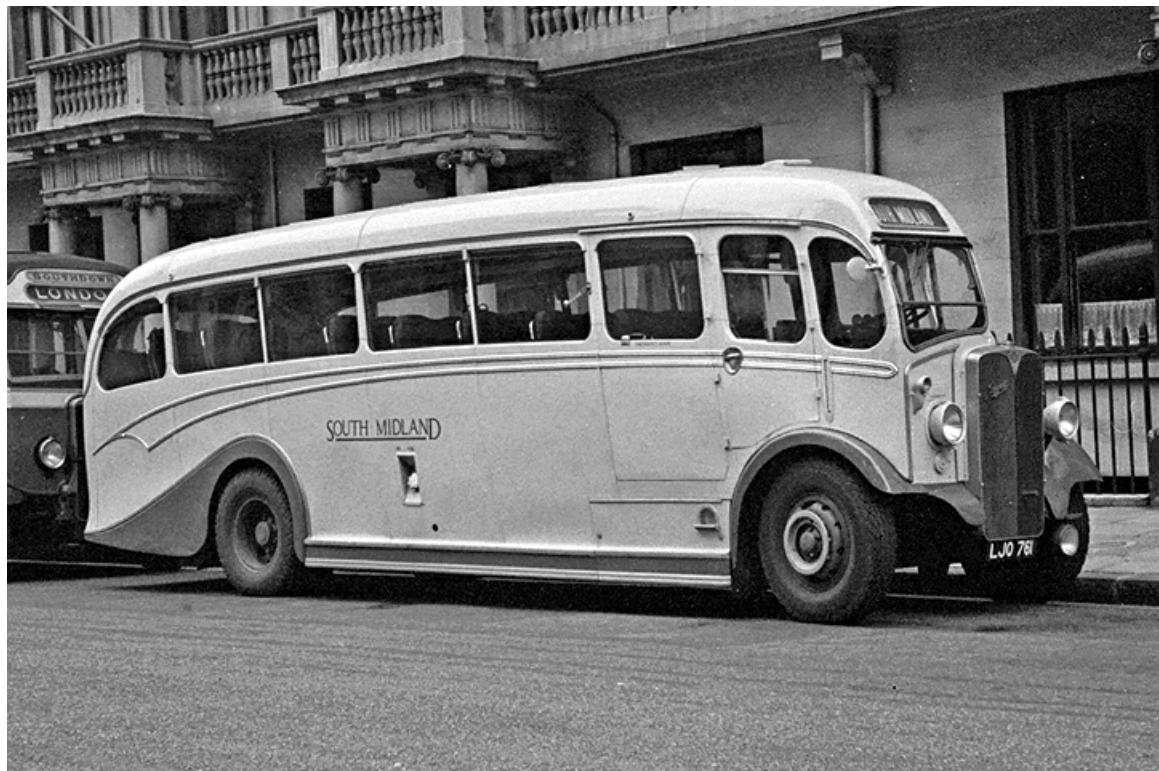
No. 48 (LJ0761) was a 1948 AEC Regal with Duple 33-seat coachwork. (Bus Archive).
