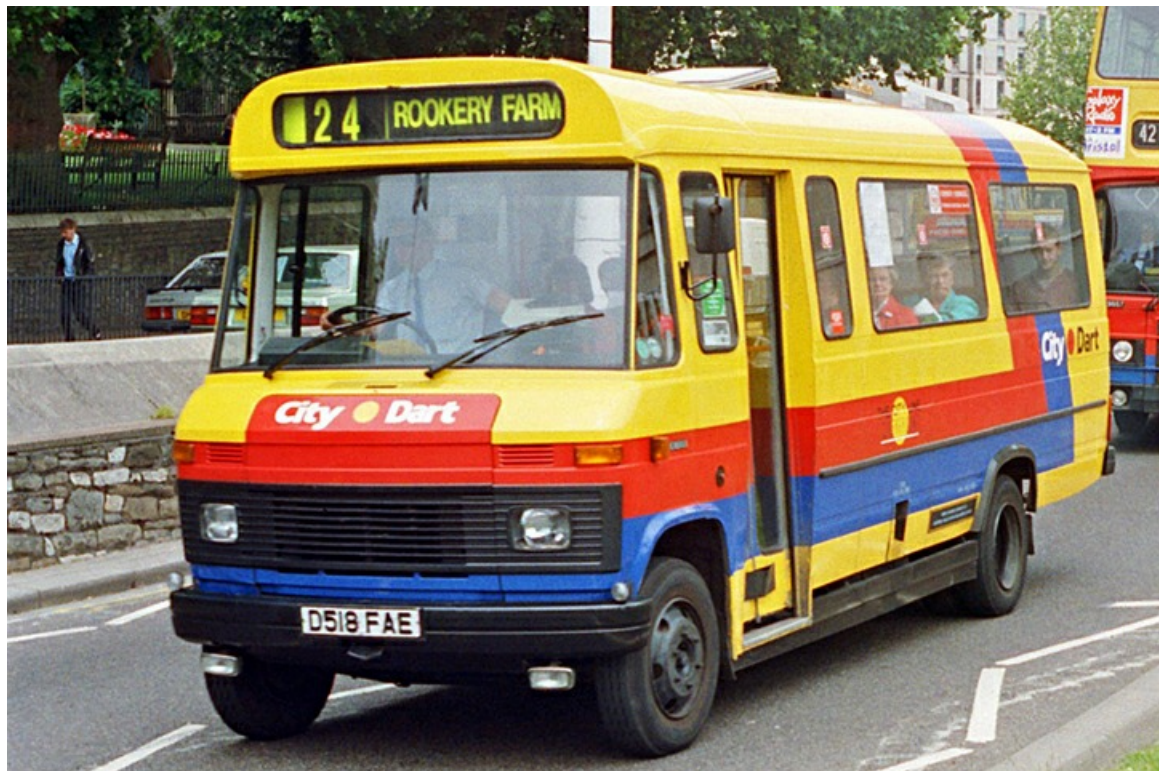
7518 (D518FAE), in City Dart livery was a 1986 Mercedes-Benz L608D with Dormobile B20F bodywork. (Kevin Smith).
