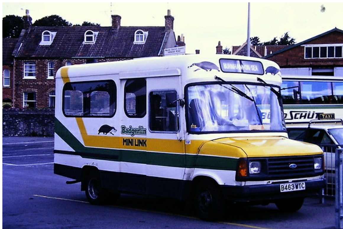
4463 (B463WTC) was a Ford Transit 190D with Carlyle B16F bodywork on Dormobile frames new in 1985. (Stephen Day).
