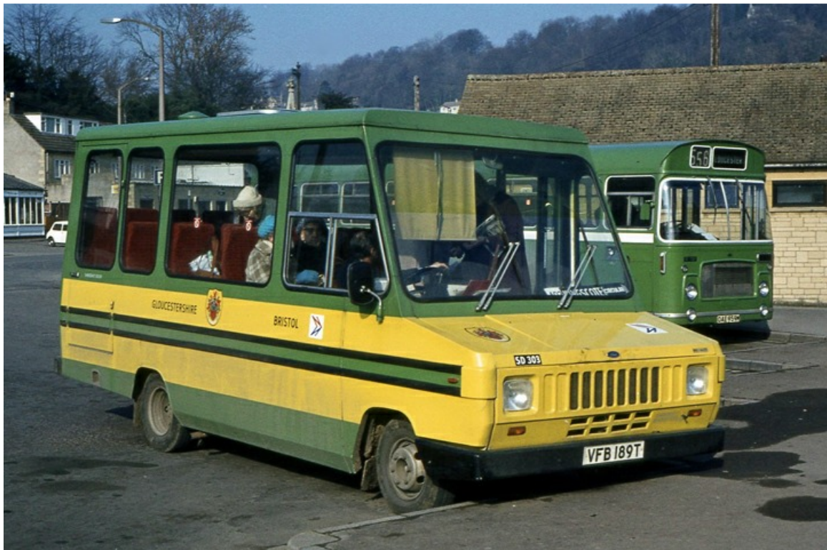
303 (VFB189T) was a 1979 Ford Transit with Reeve Burgess DP17F bodywork, owned by Gloucestershire County Council and operated by Bristol Omnibus Company on their behalf. (David Flett).
