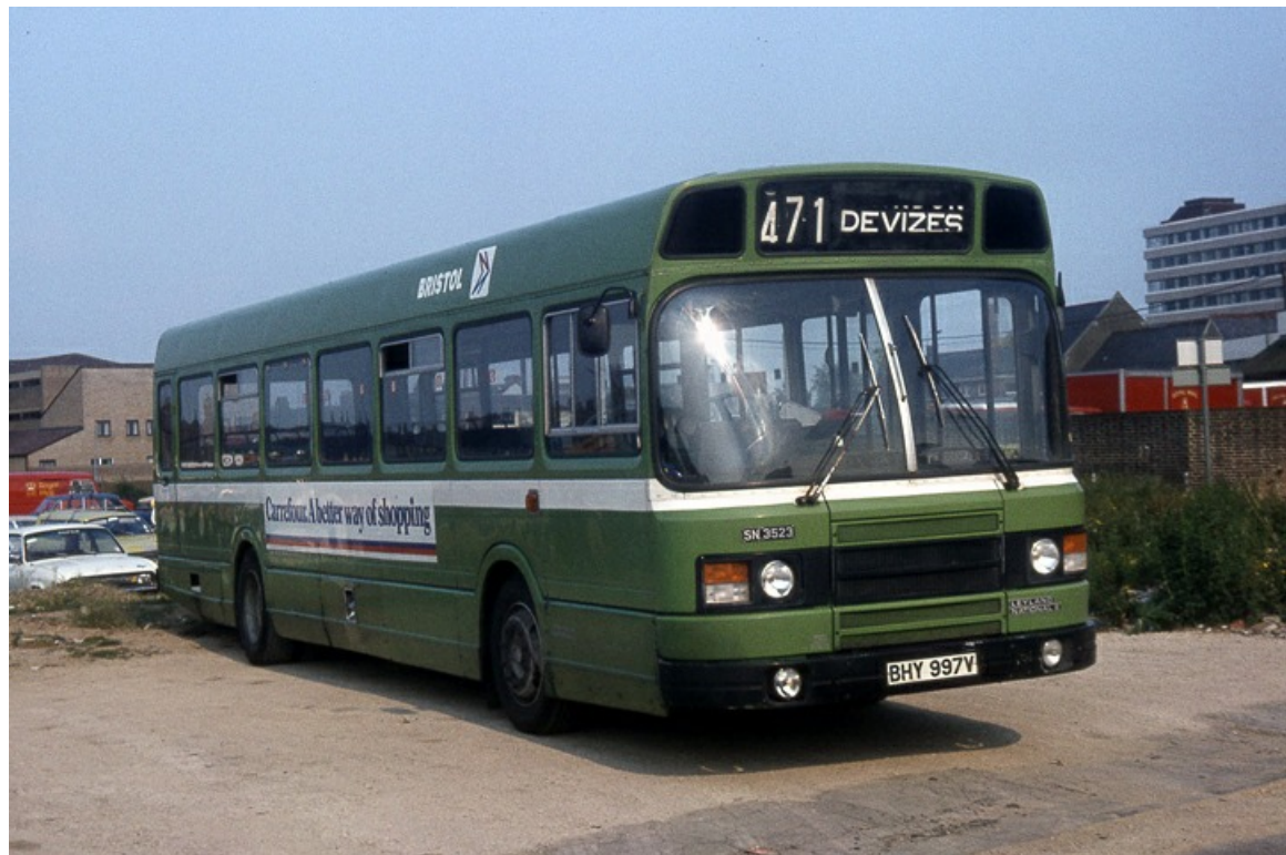
3523 (BHY997V) was a Leyland National 2 with B52F bodywork, dating from 1980. (John Law).
