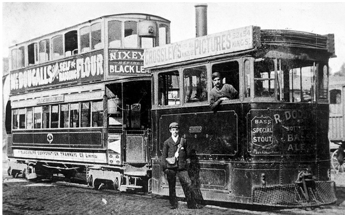
A Thomas Green steam tram loco of Blackburn Corporation Tramways Company, one of fourteen purchased in 1887. (LTHL collection).
