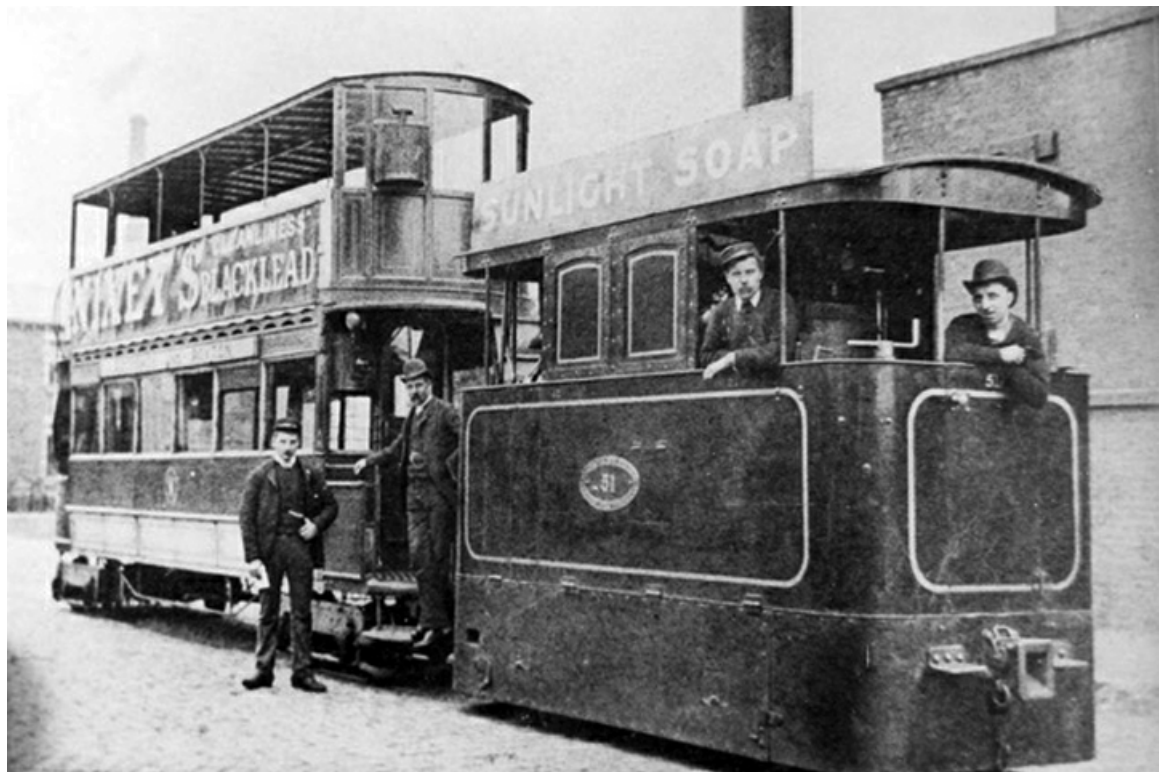
Black Hawthorn built steam tram loco No. 51 of the Manchester, Bury, Rochdale & Oldham Steam Tramways Company dating from 1884. (LTHL collection).
