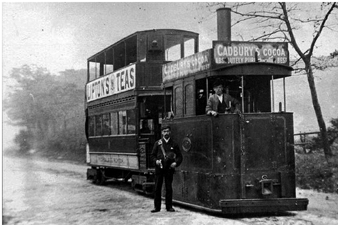
A Wilkinson steam locomotive and trailer, probably at the Summit in Heywood. One of several 3ft 6ins narrow gauge engines supplied to the Manchester, Bury, Rochdale and Oldham Steam Tramways Company. (Tramways & Light Railway Society).
