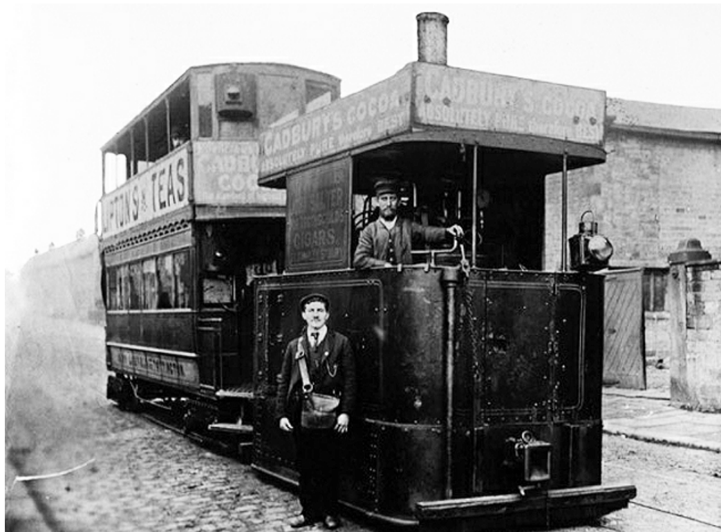
Beyer Peacock built this steam tram loco (No. 77) to the Wilkinson patent for the Manchester, Bury, Rochdale & Oldham Steam Tramways Company in 1886. (LTHL collection).
