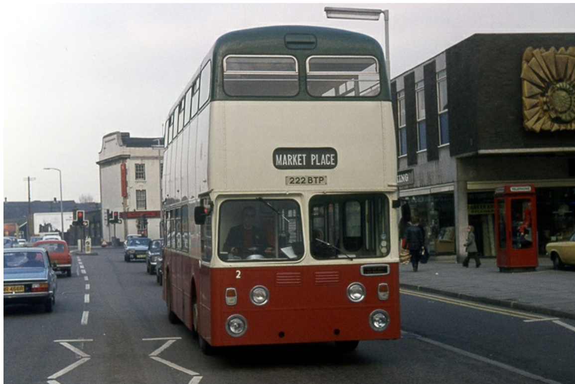
No. 2 (222BTP) was an ex-Portsmouth Corporation Leyland PDR1/1 with MCCW H43/33F bodywork new in 1963 and acquired in 1976. (John Law).
