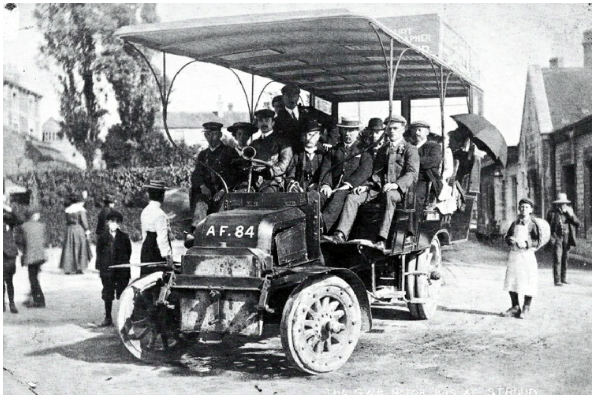
No. 15 (AF84) a 1904 Milnes-Daimler with covered charabanc body typical of those fitted by the GWR in summer, but see the following illustration for AF84 in another guise. (LTHL collection)
