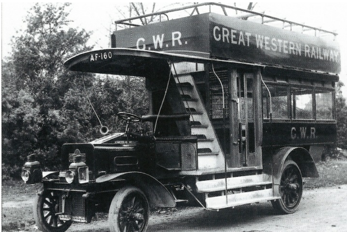
No. 79 (AF160) was fitted with an experimental front entrance body by Scammell & Nephew but was later replaced with a conventional 018/1600 body, after (apparently) female passengers complained that drivers could see their ankles as they climbed the stairs! (LTHL collection).
