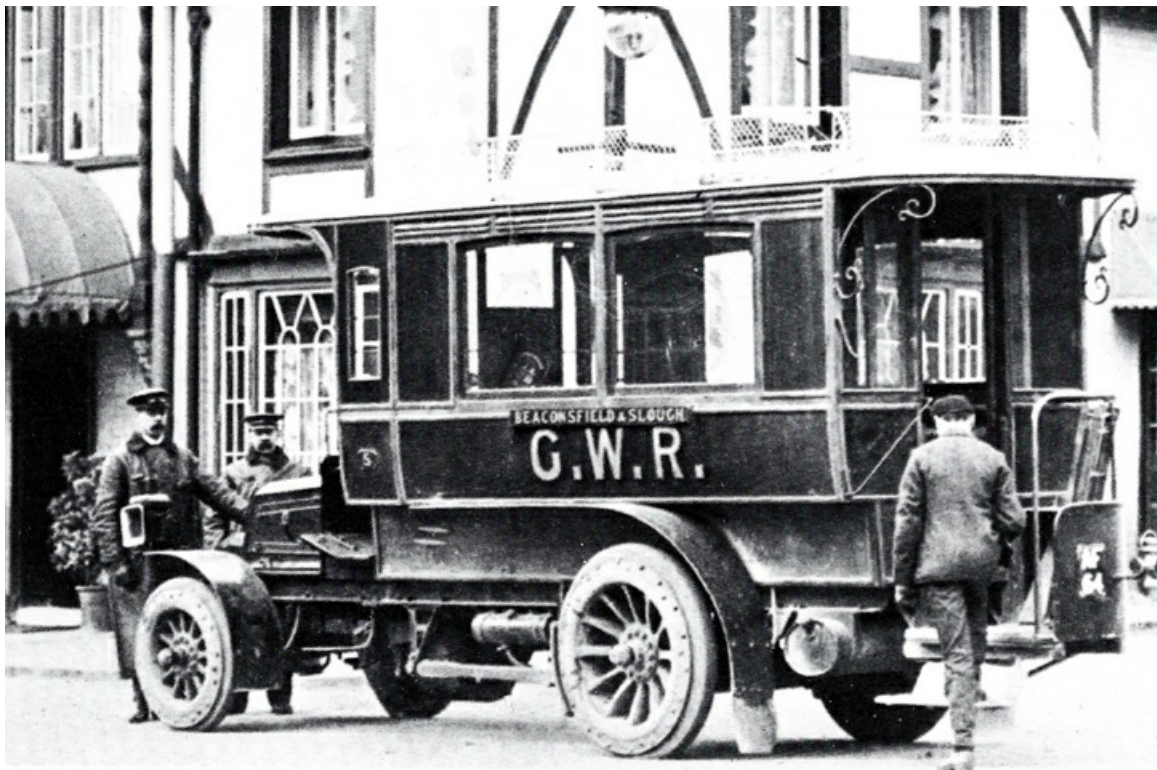
No. 5 (AF64) with enclosed single-deck body of varnished wood manufactured by the London firm of Thrupp & Maberley. It was later replaced by the small double-deck body shown on page 14. (LTHL collection).
