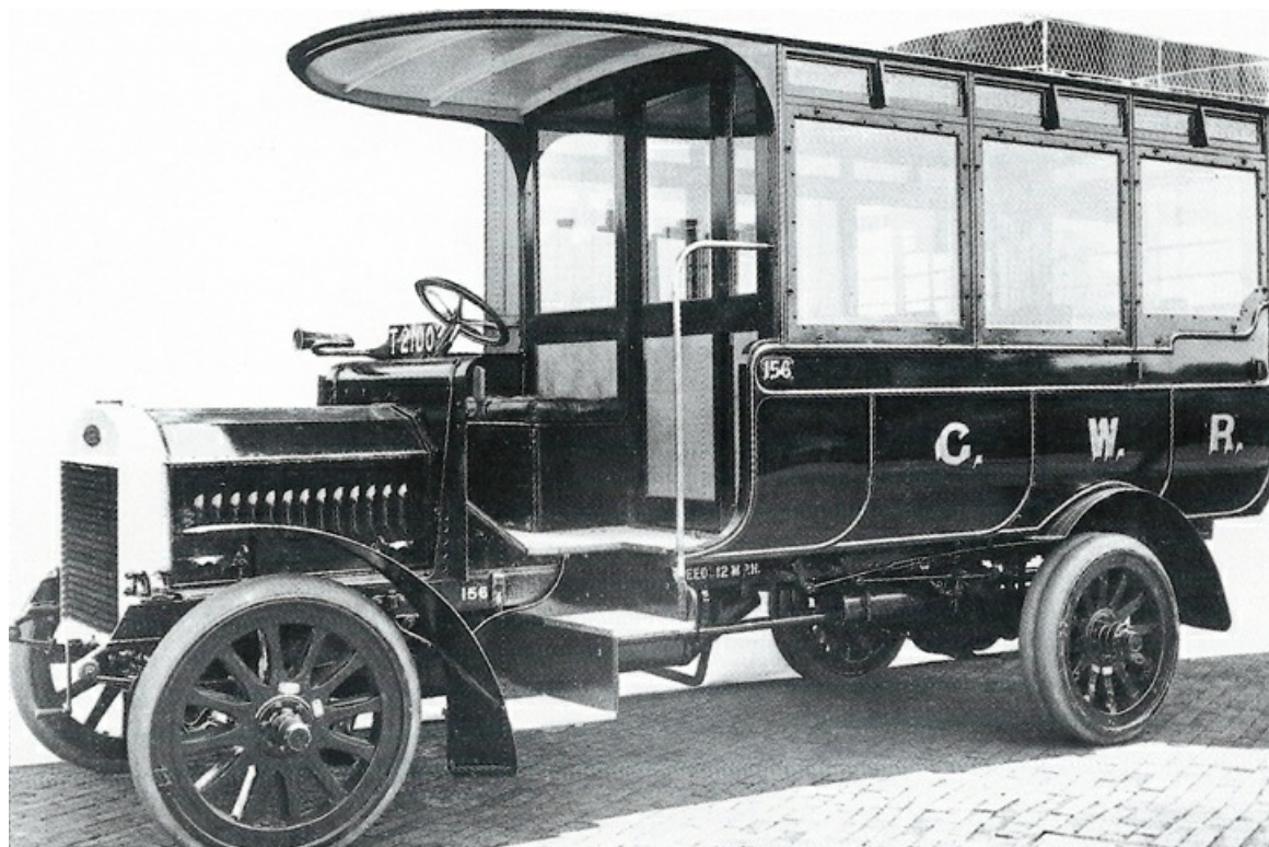
No. 156 (T2100) was a 1911 Dennis 20hp with 16-seat bodywork built at Swindon by the GWR themselves. (LTHL collection).
