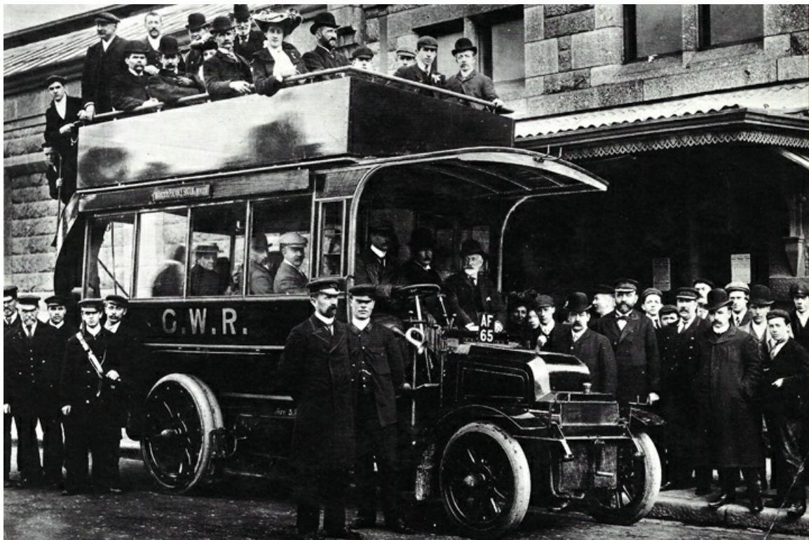
No. 6 (AF65) was the GWR's first double-deck and illustrates the standard double-deck 018/16RO body. The body was probably by Dodson who was the main subcontractor for Milnes-Daimler. (LTHL collection).
