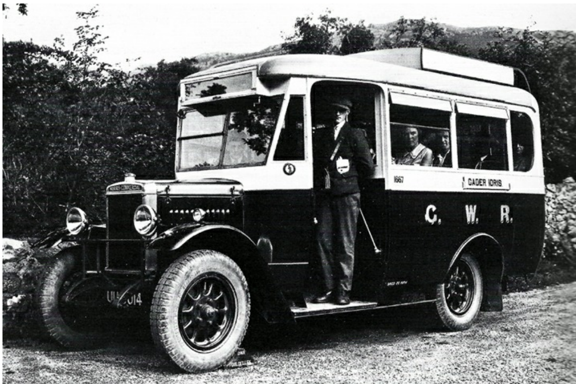
Numerically the last GWR bus purchased was No. 1667 (UU5014) a Morris R with Buckingham 14-seat bodywork. (LTHL collection).
