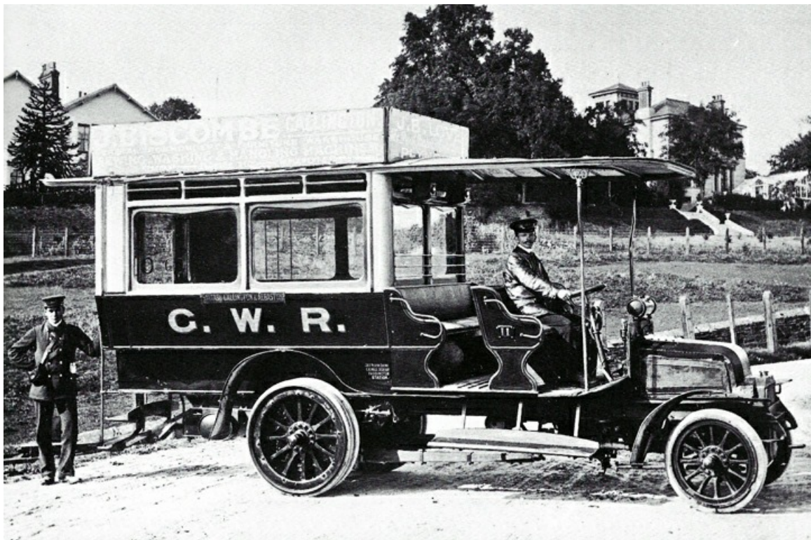
No. 11 (AF74) was a 1904 Milnes-Daimler with composite single-deck body. The enclosed non-smoking rear compartment seated 16 passengers on transverse seating with 6 more outside seats for smokers. (LTHL collection).
