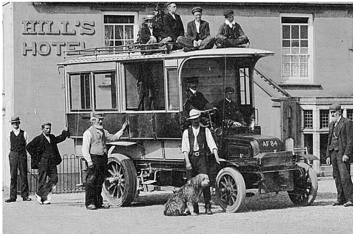
No. 15 (AF84) at Hill's Hotel, The Lizard c. 1910 with rear 10-seat saloon and luggage/mail compartment. Two more passengers could be seated next to the driver. (LTHL collection).
