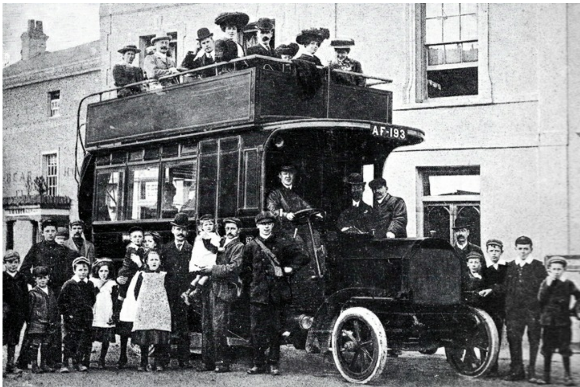
No. 67 (AF193) a 1906 Milnes-Daimler with standard double-deck body with mail compartment, reducing seating capacity to 018/12R0. (LTHL collection).
