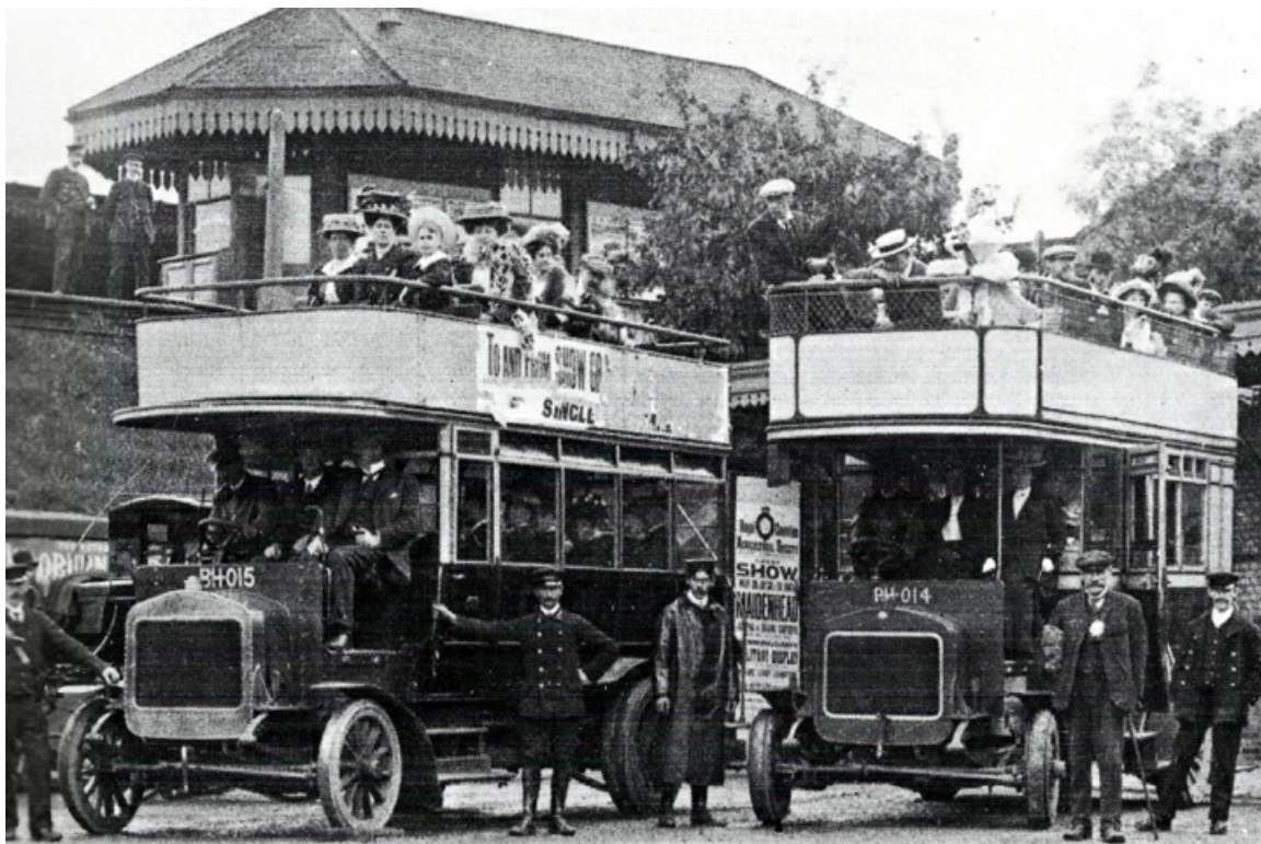
The two Wolseley buses of 1906 (Nos. 63 and 77) originally had bodies by Dodson which proved too heavy for the chassis and were removed and replaced by lighter bodies. This photograph shows the buses in original condition. (LTHL collection).
