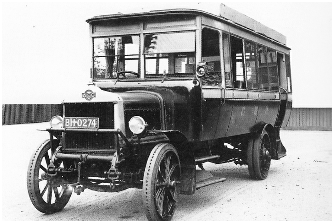
No. 232 (BH0274) with GWR-built B31R bodywork. It became a lorry in 1928. (LTHL collection).
