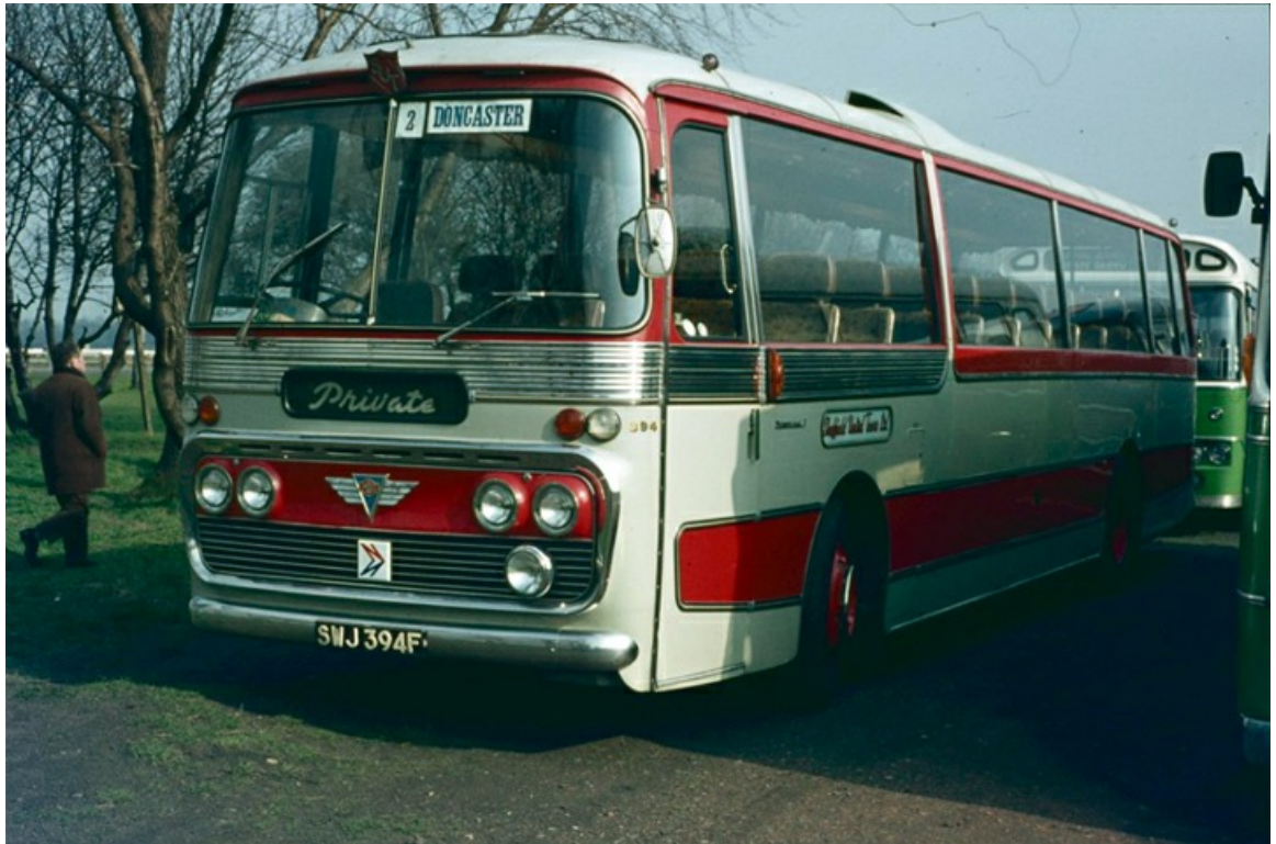
No. 394 (SWJ394F), now sporting its NBC logo, was a 1968 AEC Reliance with Plaxton 49-seat coachwork. (Richard Simons).
