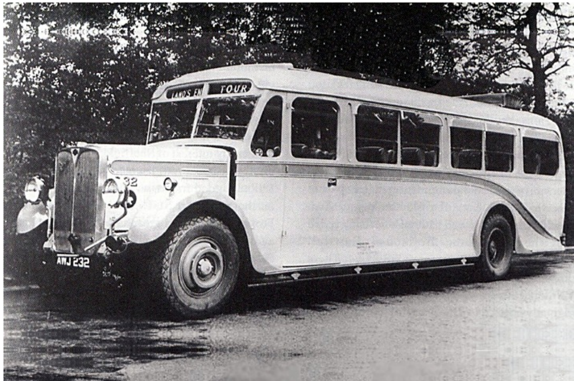
No. 32 (AWJ232) was one of the first new vehicles for Sheffield United Tours. It was a normal control AEC Ranger with local Cravens 26-seat coachwork. (LTHL collection).
