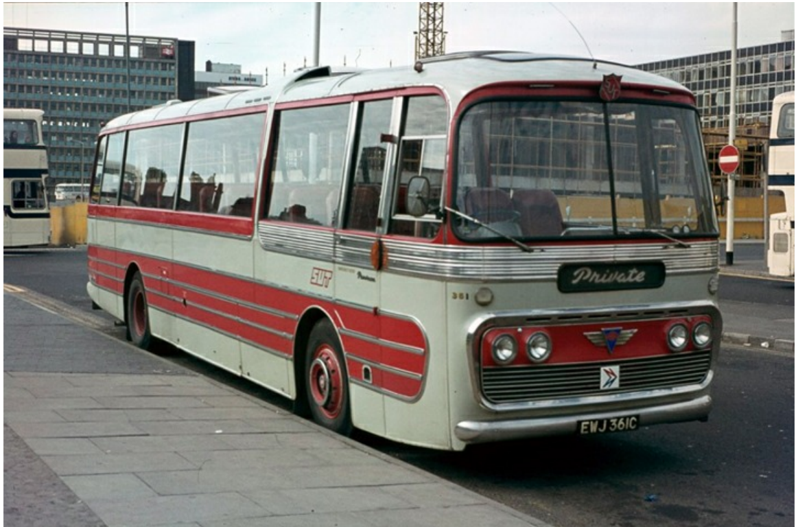
No. 361 (EWJ361C) was a 1965 AEC Reliance with Plaxton 45-seat coachwork. It passed to National Travel in 1974 with the rest of the fleet. (Richard Simons).
