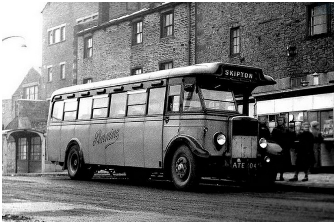
ATE804 was one of two ex-Lancashire United MCCW-bodied Leyland TS7's put into service in 1951. Both dated from 1936, whilst two others purchased at the same time served as donor vehicles to keep them running, which they did for another 5 years. (LTHL collection).
