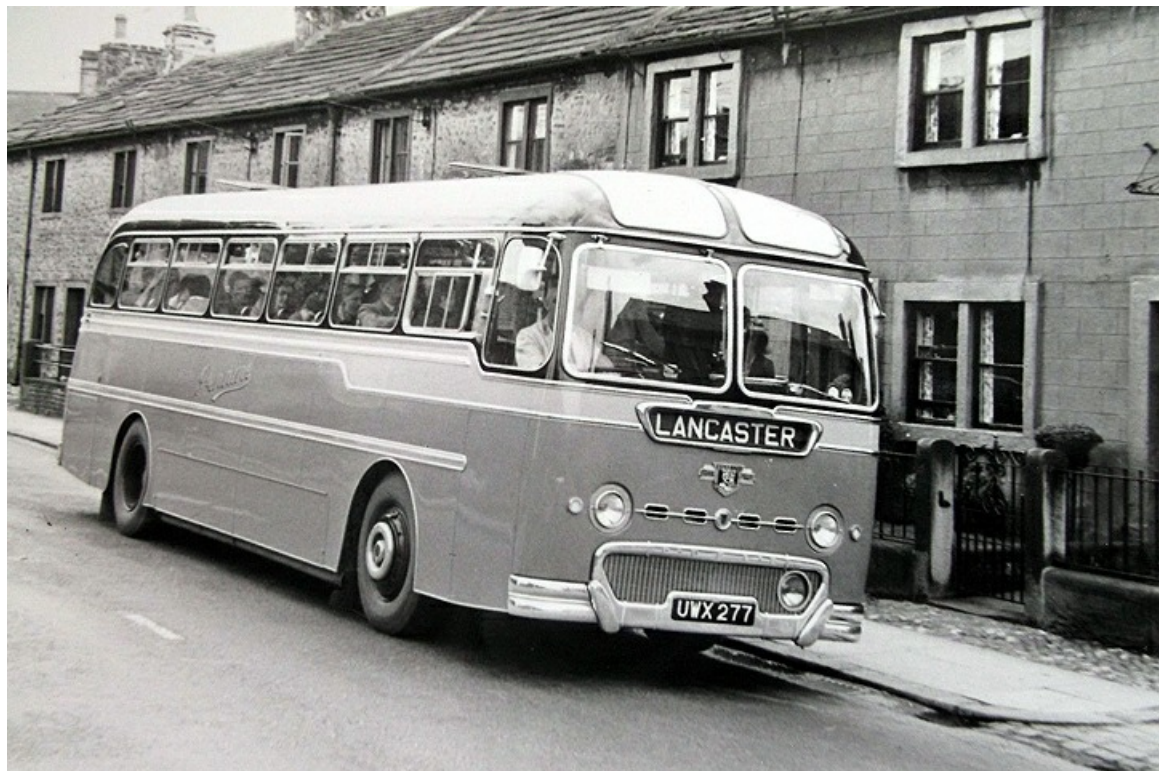
En route to Lancaster is UWX277 a 1958 Leyland PSUC1/2 'Tiger Cub' with Duple Midland dual-purpose 41-seat bodywork. (LTHL collection).
