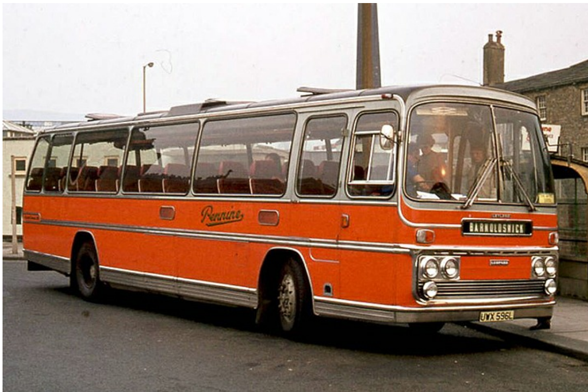
1973 Leyland PSU3B/4R 'Leopard' UWX596L with Plaxton 53-seat coachwork, seen in Skipton Bus Station in April 1974. (John Kaye).
