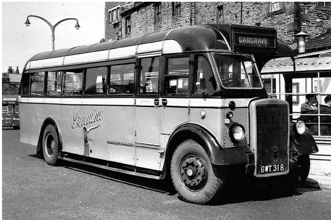
GWT318 was one of a pair of Leyland PS1 'Tigers' with Burlingham 35-seat bodywork purchased in 1947. (LTHL collection).
