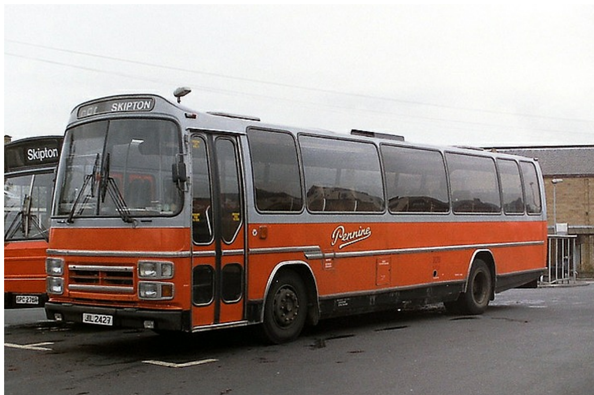
One of the last Leyland/Plaxton's to be acquired was JIL2427 (originally MAP347W then OUF50W) and was a 1981 PSU3F/4R 'Leopard' with Plaxton 48-seat coachwork that came via Southdown Motor Services. (Stephen Day).
