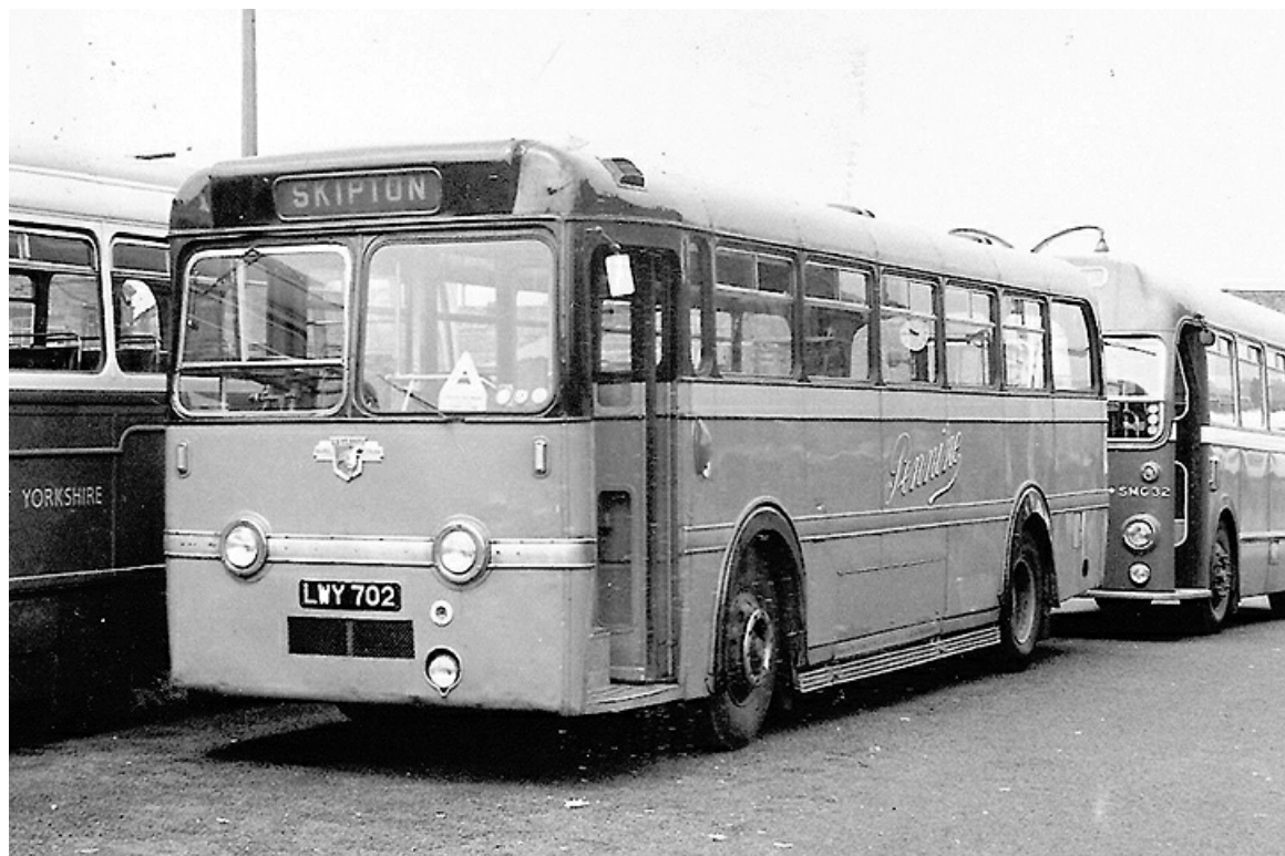
LWY702 was a 1953 Leyland PSU1/17 with Leyland 44-seat bodywork that gave 18 years of service before being withdrawn in 1971. (LTHL collection).
