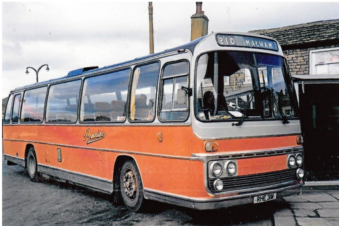
RHE31M was a second-hand purchase from Yorkshire Traction in 1986 and dated from 1974. It was a Leyland PSU3B/4R 'Leopard' with Plaxton 49-seat bodywork and gave another 4 years service before being withdrawn in 1990. (LTHL collection).
