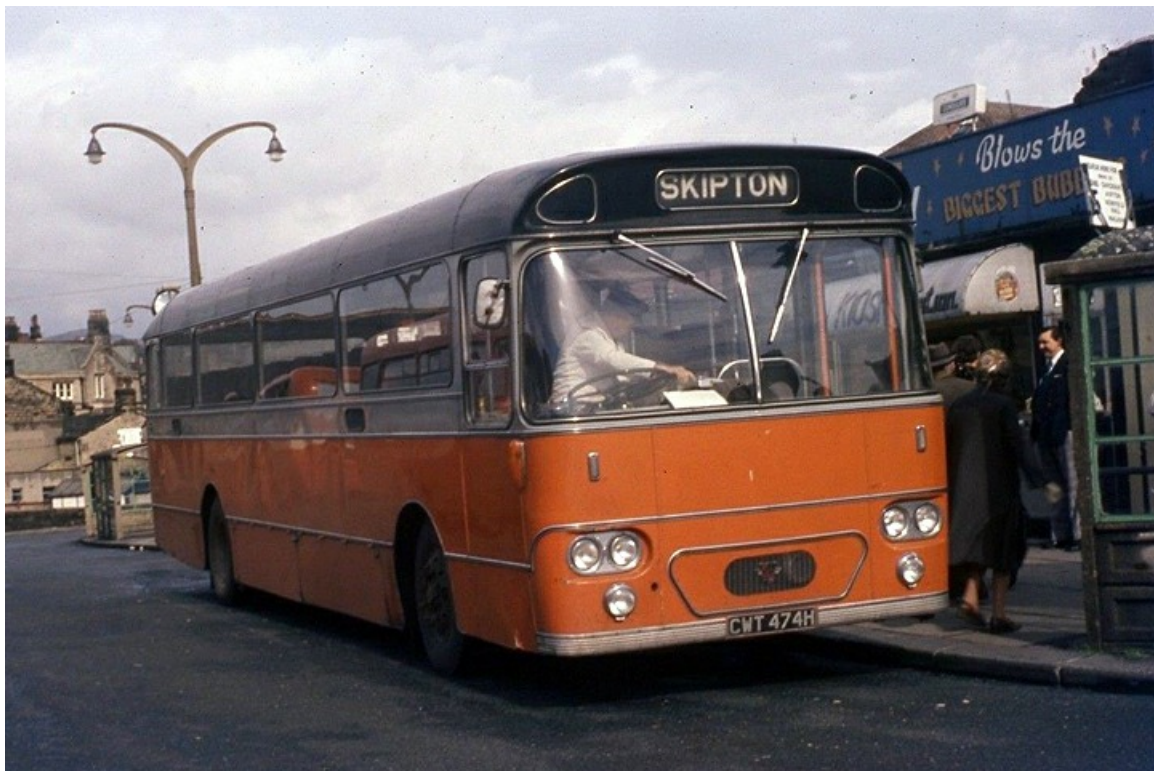
CMT474H was a 1970 Leyland PSU3A/4R 'Leopard' with 49-seat dual purpose bodywork by Willowbrook. (LTHL collection).
