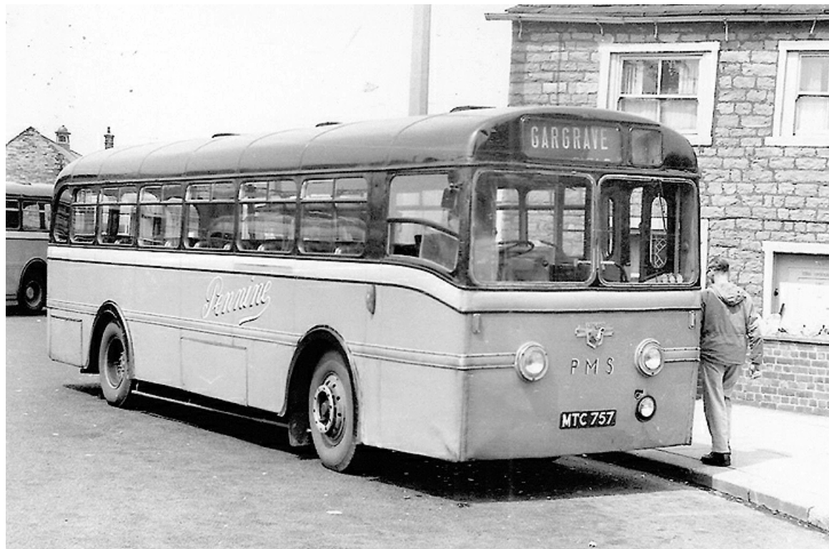
MTC757 was an ex-Leyland PSU1/13 demonstrator built in 1950 and acquired in 1951. It had a Brush B44F body and underfloor engine and marked the end of the half-cab era. (LTHL collection).
