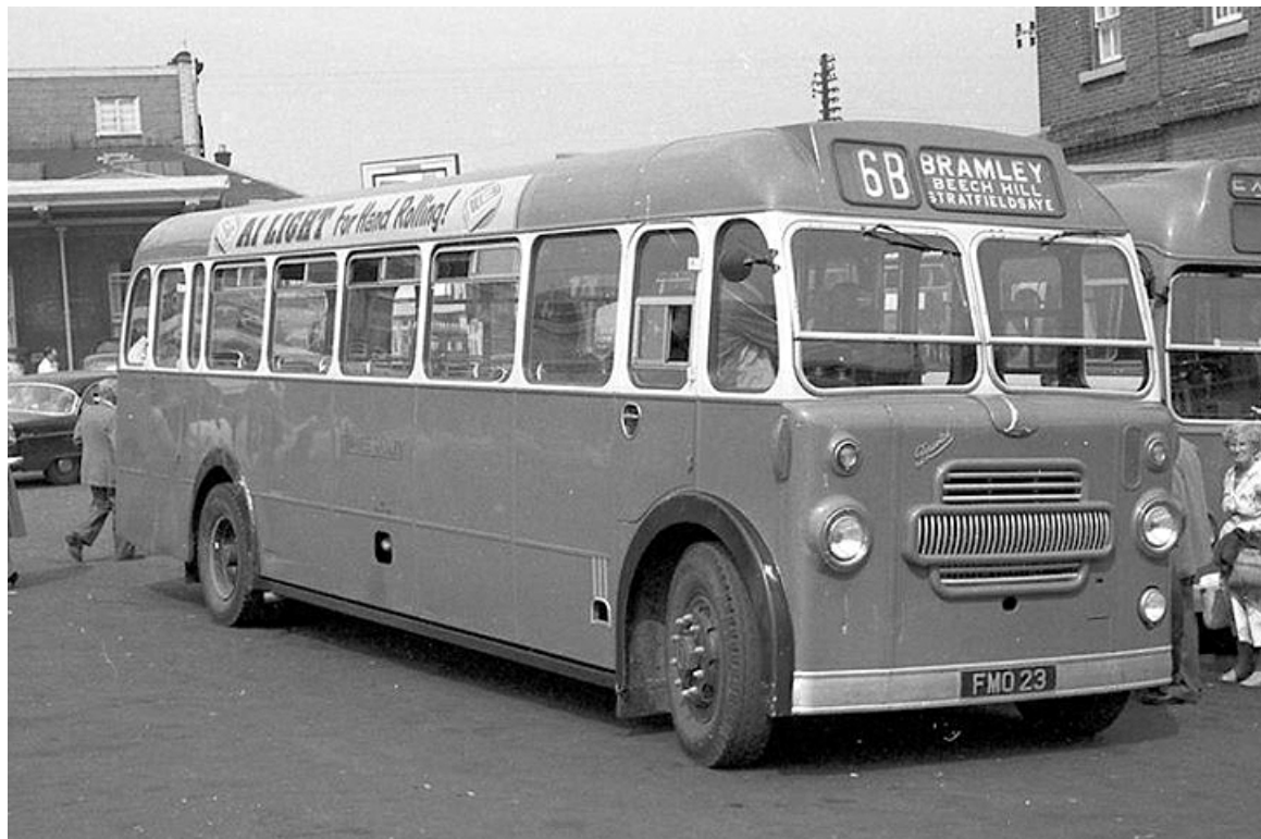
No. 819 (FM023) was a 1950 Bristol L6B. Originally No. 546, it carried a Windover 33-seat coach body, but was withdrawn in 1958, rebuilt to 30ft and re-bodied by ECW for one-man operation. (John Boylett courtesy John Kaye).
