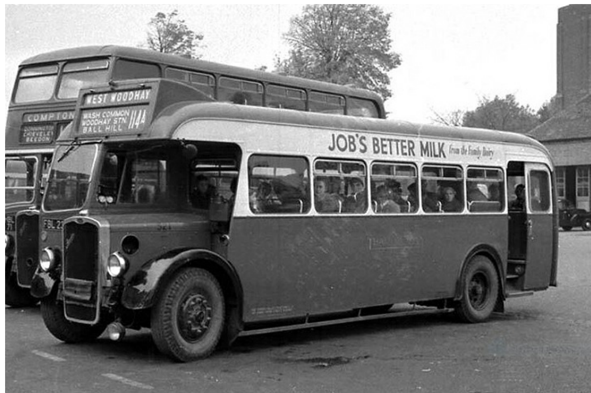
No. 521 (FBL23) was a 1949 Bristol L6B with ECW 35-seat bodywork. (John Boylett courtesy John Kaye).
