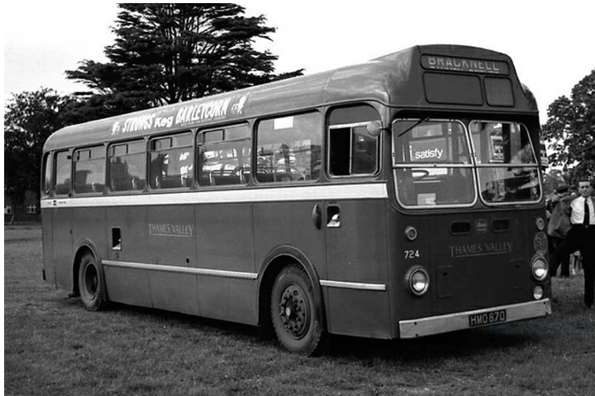
No. 724 (HM0870), one of just 3 Bristol LS6G's delivered in 1955. It had an ECW 45-seat bus body and is seen here at Ascot Racecourse in June 1965, by which time it had been re-seated to 41. (John Boylett courtesy John Kaye).
