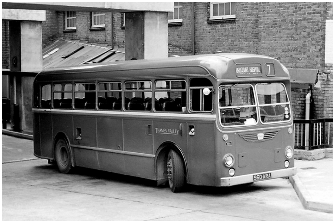
No. 155 (960ARA), a Bristol LS6G with ECW bodywork, dating from 1956 was acquired from Midland General in 1970. It was re-seated from B45F to B41F before entering service. (Eric Simpson)
