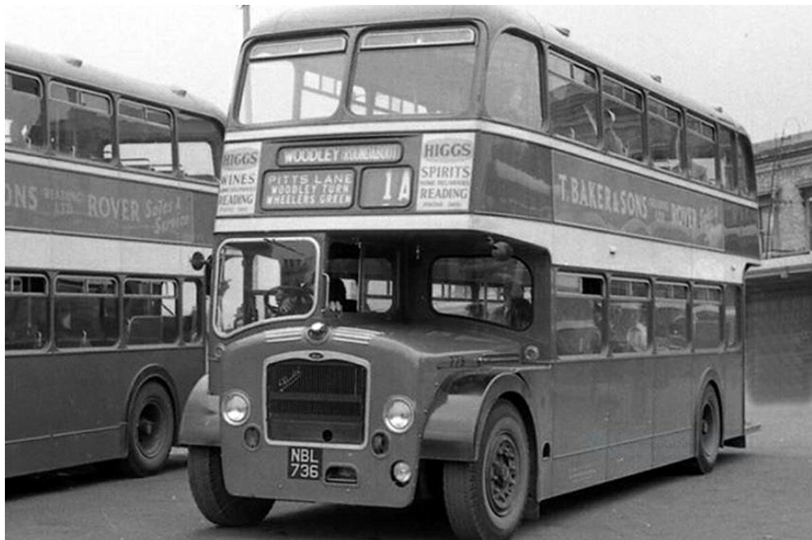
Seen at Reading Station in June 1958 is Bristol LD16G No. 779 (NBL736) sporting an ECW 70-seat body. It passed to Alder Valley in 1972 as their No. 548, by which time it had been fitted with platform doors. (John Boylett courtesy John Kaye).
