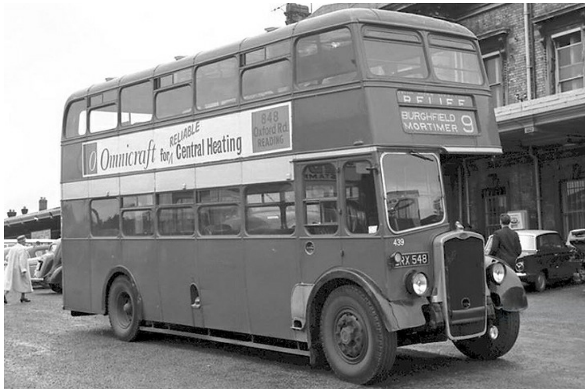
No. 439 (CRX438) was a 1946 Bristol K6A with ECW 55-seat lowbridge bodywork, seen here outside Reading Station in August 1963. (John Boylett courtesy John Kaye).
