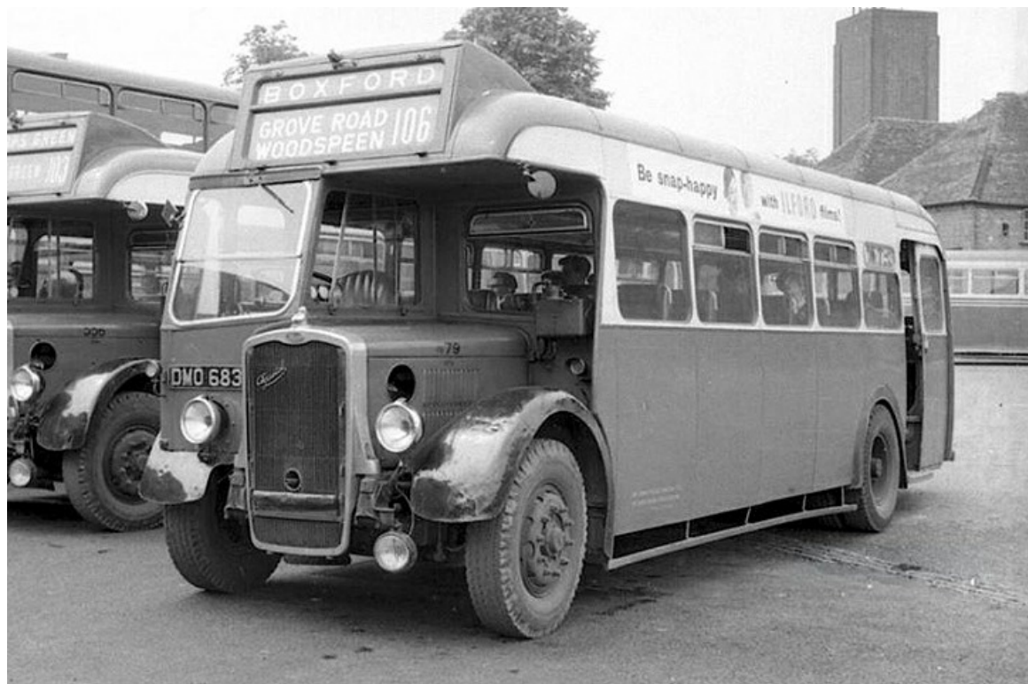
Seen at The Wharf, Newbury in June 1958 is No. 479 (DM0683), a 1948 Bristol L6A with ECW 31-seat dual-purpose bodywork. (John Boylett courtesy John Kaye).
