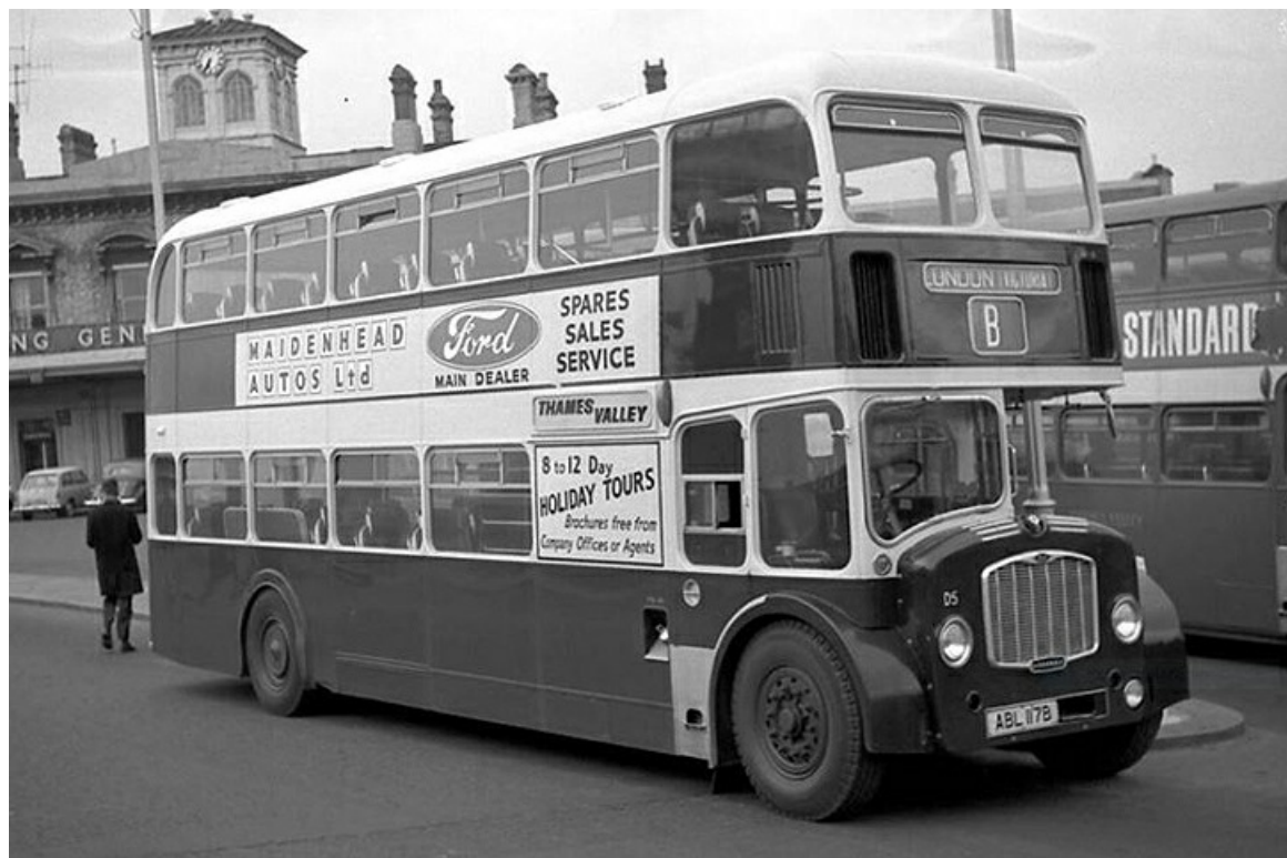
No. D5 (ABL117B), a 1964 Bristol FLE6B with ECW 65-seat double-deck coach body at Reading Station in March 1966. (John Boylett courtesy John Kaye).
