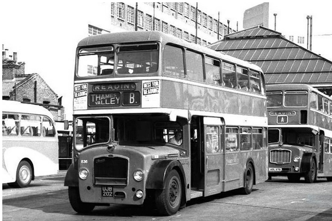
No. 837 (UJB202) was a 1960 Bristol FLE6G with ECW 65-seat double-deck coach body. It was downgraded to bus duties in 1971 and passed to Alder Valley in 1972 as their No. 603. (David Lang).
