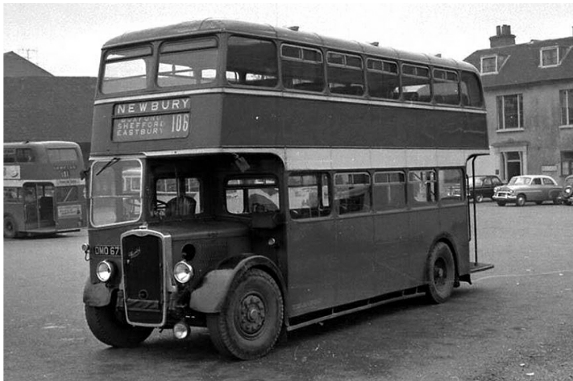
No. 467 (DMO671), at The Wharf in Newbury during October 1958, was a 1947 Bristol K6A with ECW 55-seat lowbridge bodywork. It was withdrawn in 1962. (John Boylett courtesy John Kaye).
