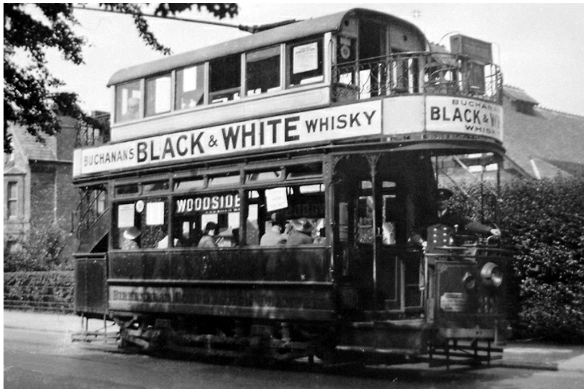
No. 32 was a 1901 Milnes-built double-deck car seating 55. Originally open-top it had been fitted with a short top-cover by the time of this photograph. (LTHL collection).
