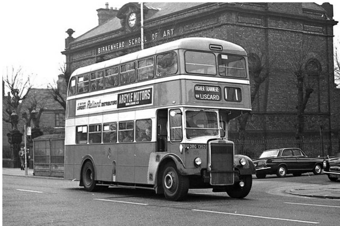
No. 135 (DBG135D) was a 1966 Leyland PD2/40 with Massey H36/30R bodywork. (Mike Beamish).
