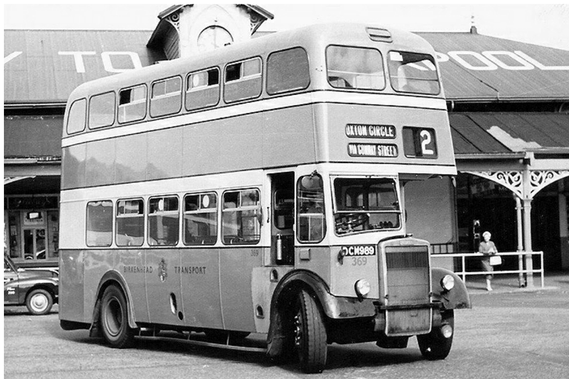
No. 369 (DCM989) was a 1955 Leyland PD2/12 'Titan' with Weymann H33/26R bodywork. (LTHL collection).
