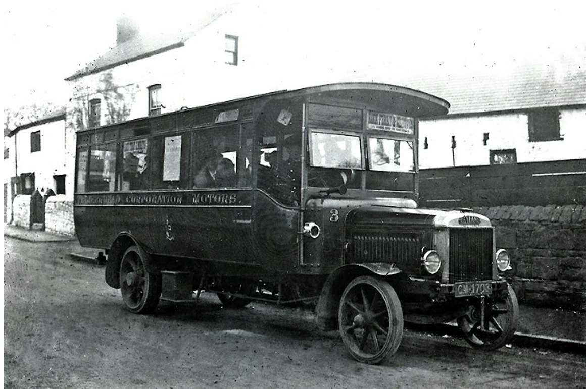
One of Birkenheads' first intake of buses included No. 3 (CM1703), a 1919 Leyland O with Leyland B32R bodywork. (Bus Archive).
