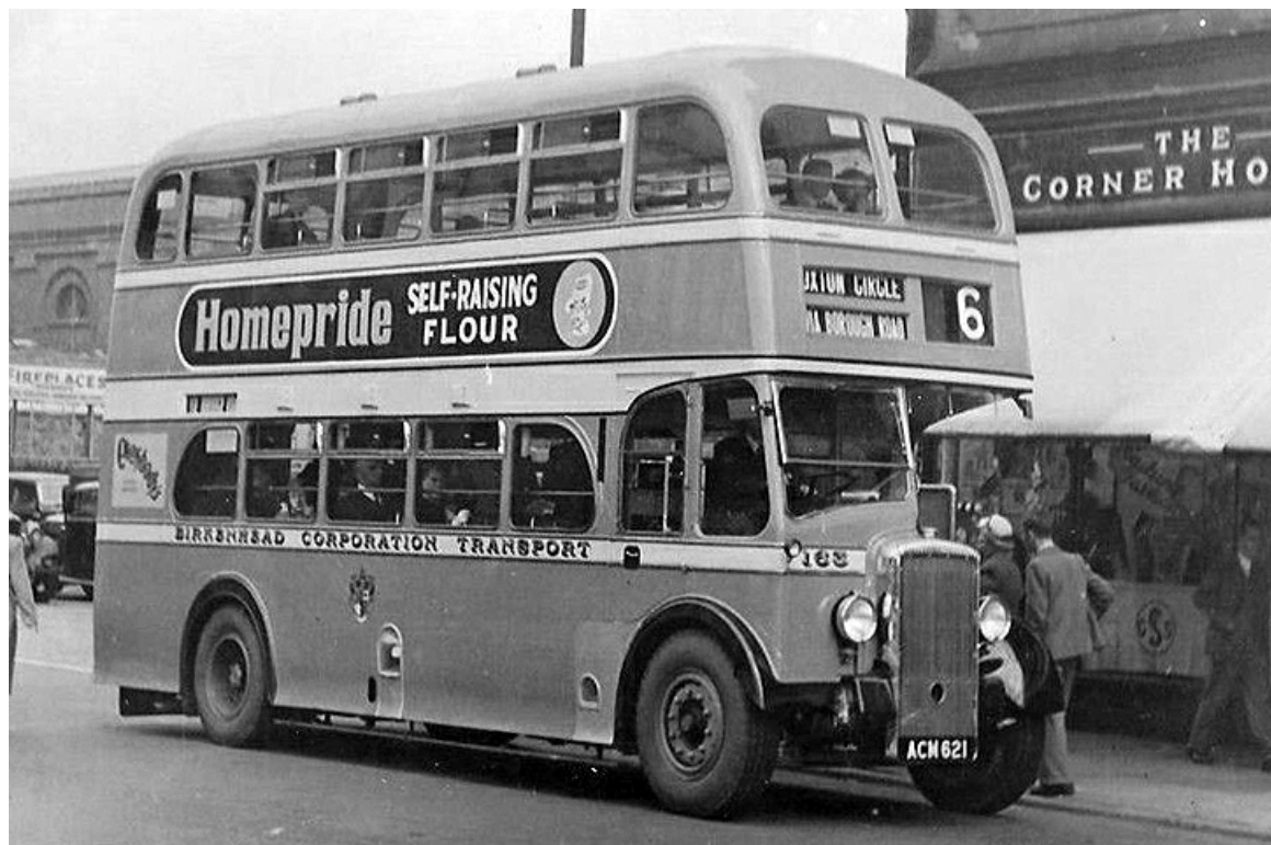
No. 163 (ACM621) was one of a batch of 15 Daimler CVG6 with Massey H30/26R bodies which entered service in 1949. (LTHL collection).
