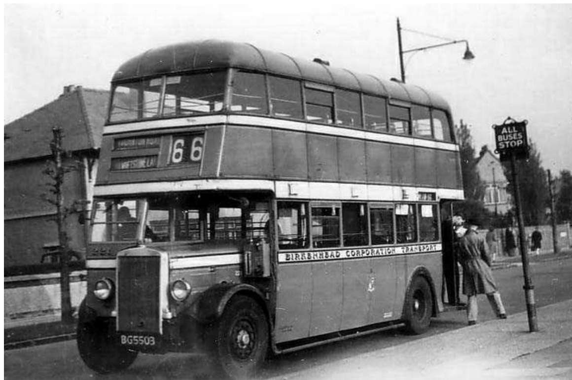
No. 221 (BG5503) was a 1937 Leyland TD5c with Massey H30/24R bodywork. (LTHL collection).
