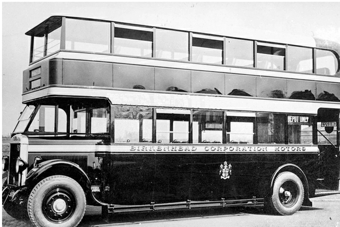
No. 96 (CM8723) was a 1929 Leyland TD1 with Leyland L24/24R bodywork. (LTHL collection).
