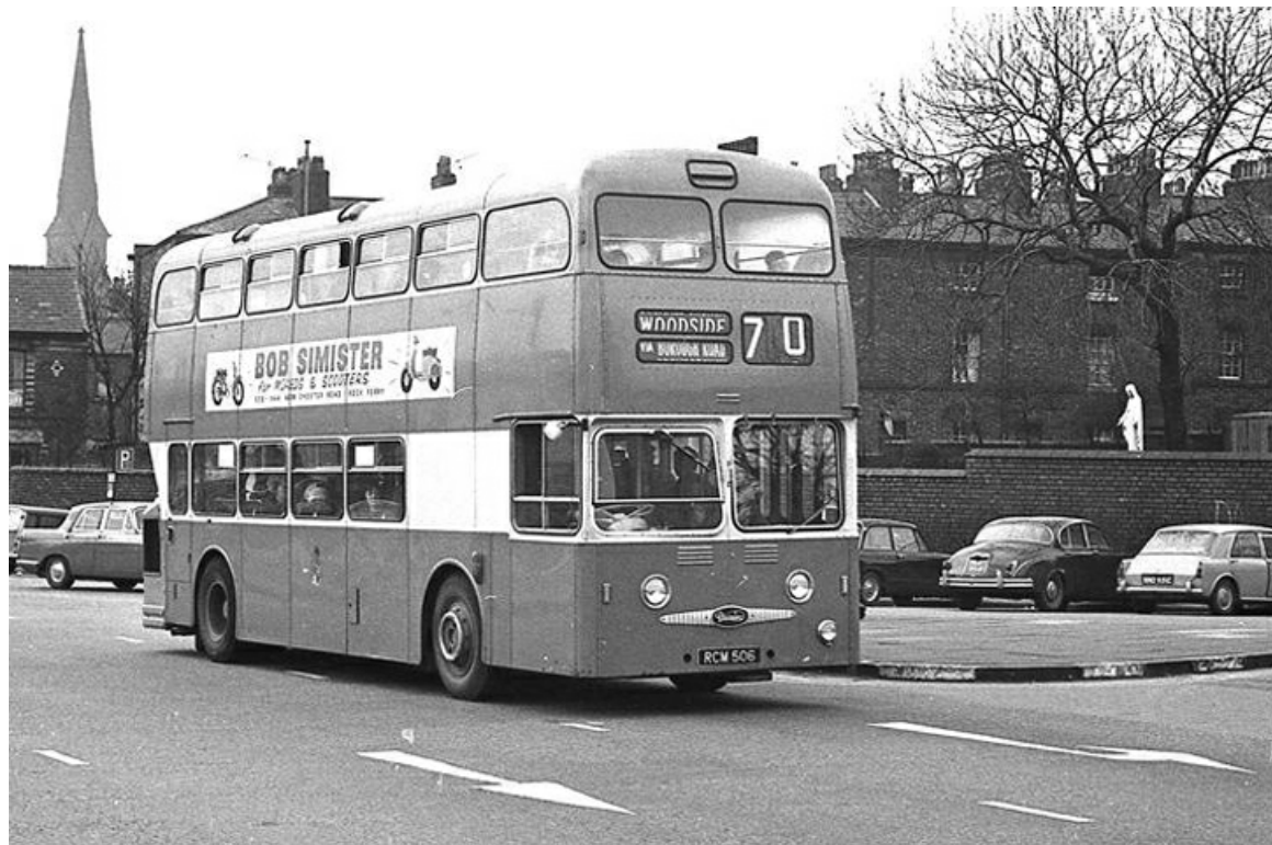
No. 106 (RCM506) was one of Birkenhead's first rear-engined vehicles. It was a 1964 Daimler CRG6LX with Weymann H44/33F bodywork. (Mike Beamish).
