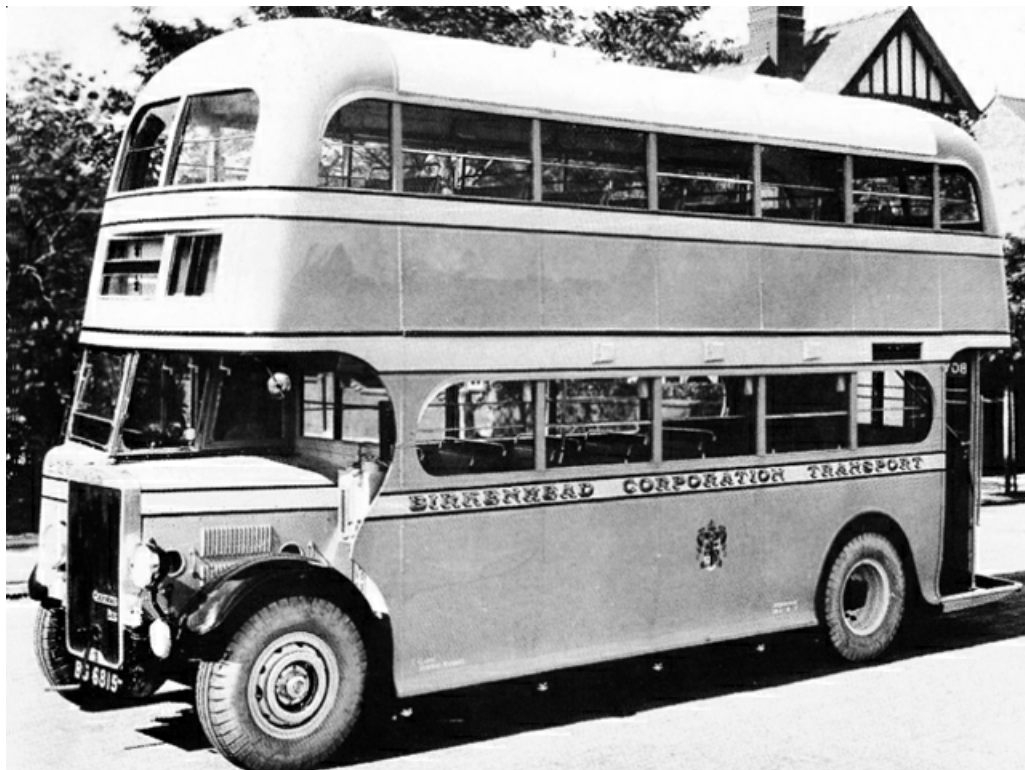
No. 273 (BG6815) was a 1938 Leyland TD5c with Northern Counties H28/26R bodywork. It was withdrawn in 1954 after 16 years service. (LTHL collection).
