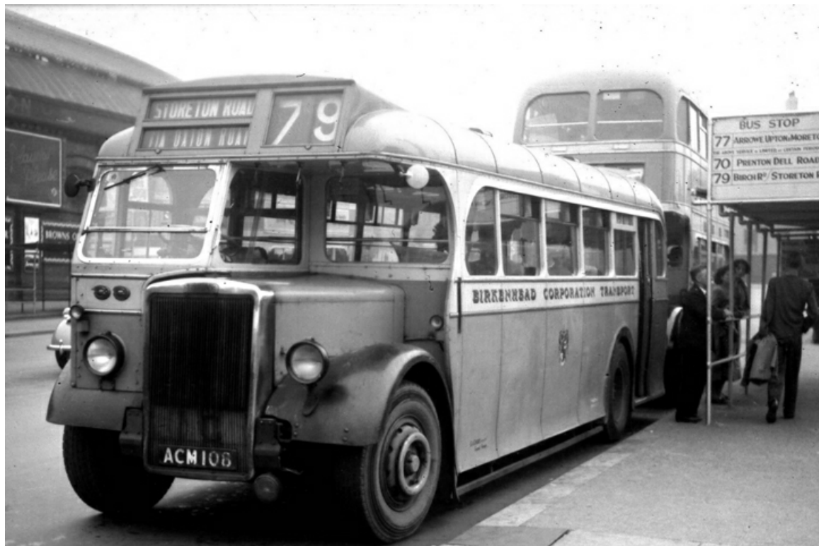
No. 99 (ACM108) was a 1948 Leyland PS1 'Tiger' with Massey 33-seat rear-entrance bodywork. (LTHL collection).
