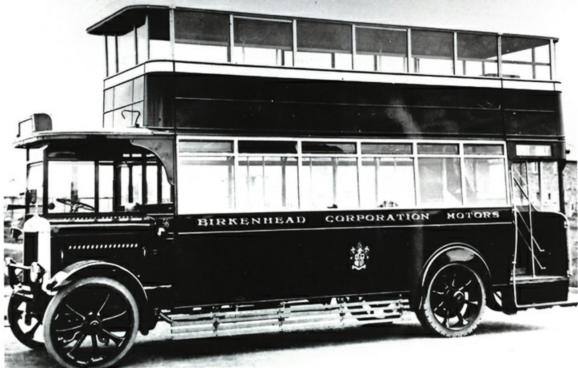
No. 56 (CM6612) was a Leyland PLSP1 with Leyland H28/27R bodywork dating from 1927. (Bus Archive).
