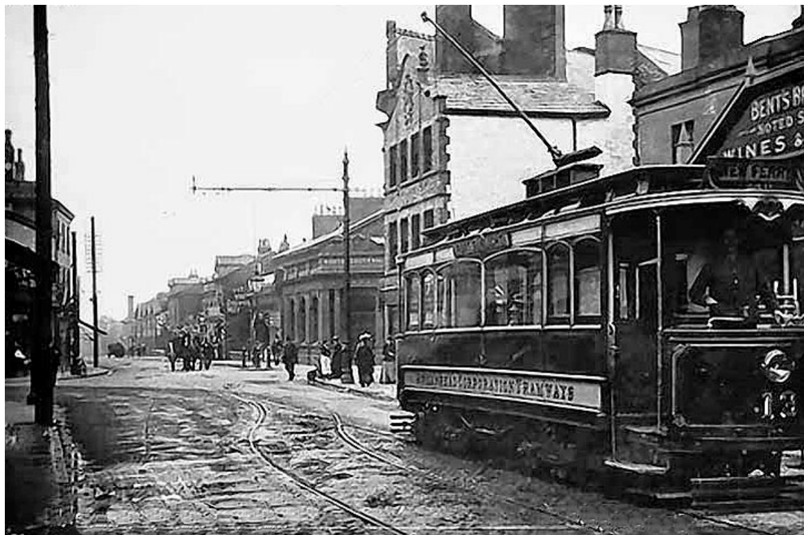
No. 13 was a 1901 Milnes built single-deck saloon seating 31. It was rebuilt as a low-height double-deck car in 1908. (LTHL collection).
