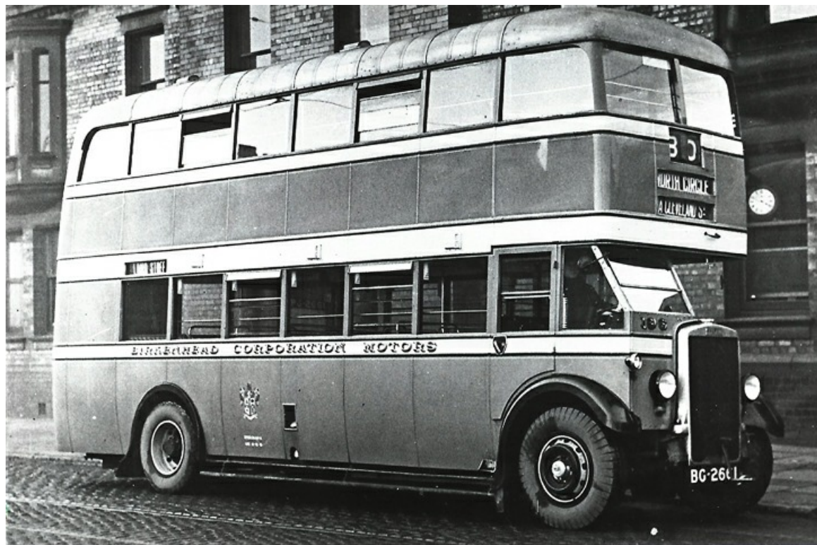
No. 196 (BG2661) was a 1934 Leyland TD3c with Massey H28/24R bodywork. (Bus Archive).
