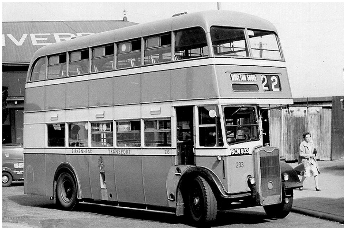
In 1952 Birkenhead returned to the Guy Arab chassis purchasing 15 with East Lincs H33/266 bodies. This is No. 233 (BCM933). (LTHL collection).
