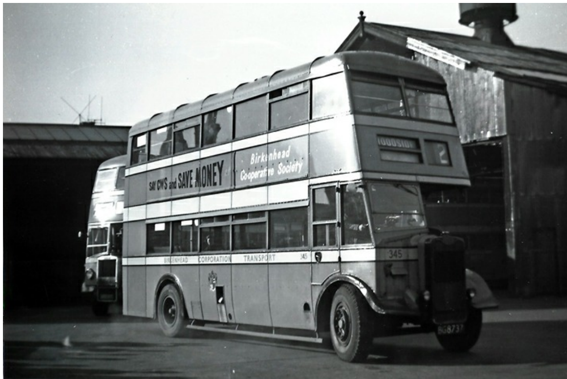
No. 345 (BG8737) was a 1946 Guy Arab II with Northern Counties H30/26R bodywork. (Bus Archive)
