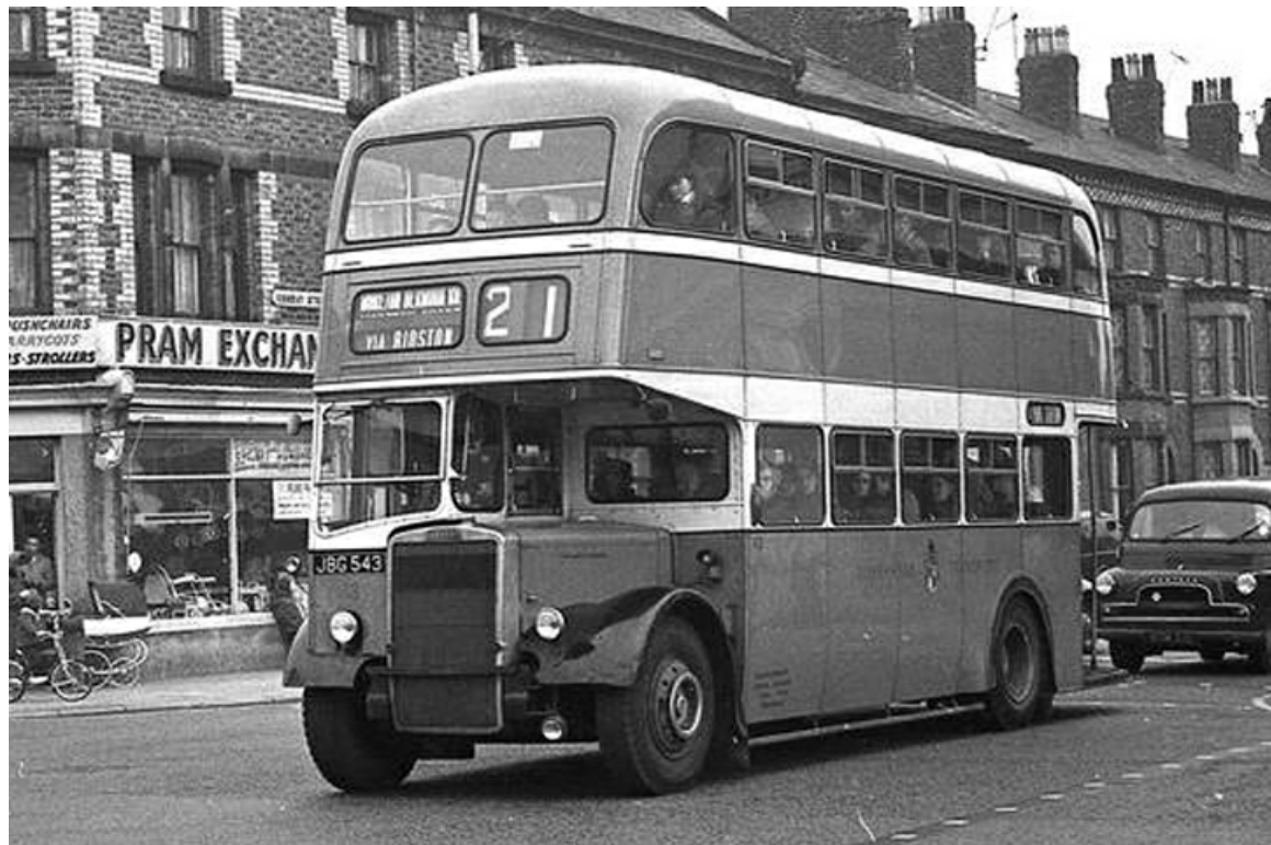
No. 43 (JBG543) was a 1960 Leyland PD2/40 with Massey H35/28R bodywork. (Mike Beamish).
