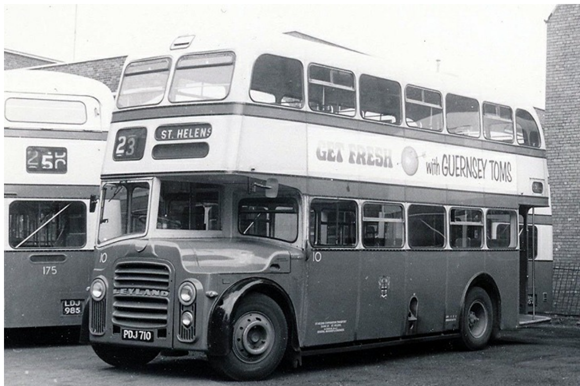
L10 (PDJ710) was a Leyland PD2A/30 with East Lancs 64-seat bodywork; new in 1961 it was withdrawn in 1973. (LTHL collection).
