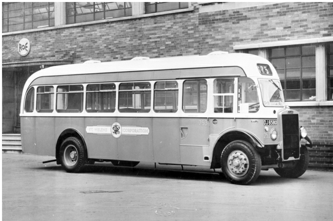
Seen outside the Roe works after receiving its new Roe B33D body in 1950 is No. 67 (DJ6580), a Leyland TS6c dating from 1935. (Bus Archive).
