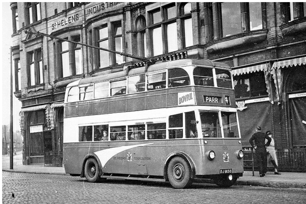
No. 155 (DJ8130) was a 1938 Ransomes D4 with Massey 50-seat lowbridge bodywork. (Bus Archive).
