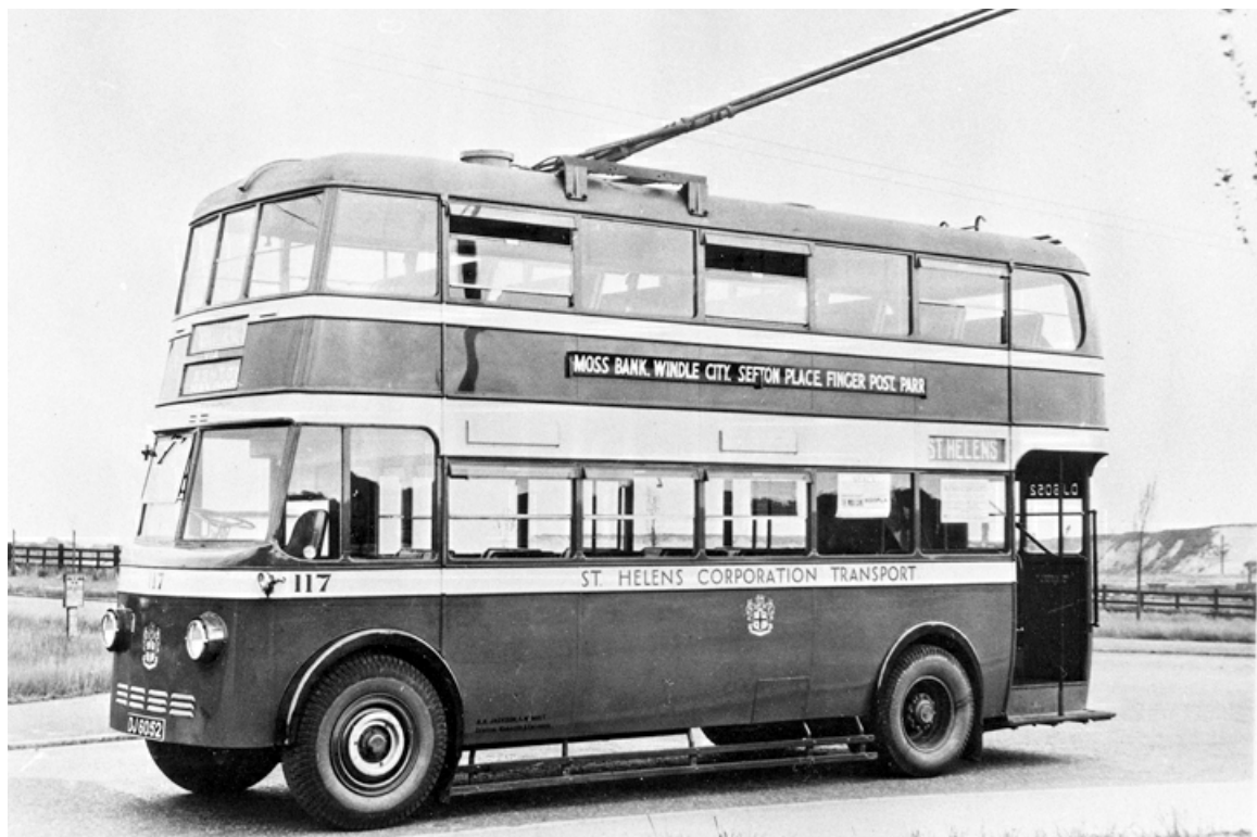
No. 117 (DJ6052) was a 1934 Ransomes D4 with Brush 50-seat bodywork. It was withdrawn in 1945. (Bus Archive).
