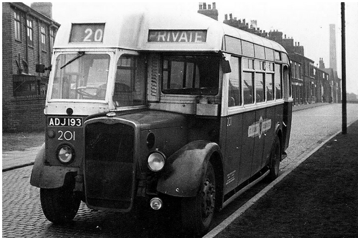
No. 201 (ADJ193) was a 1948 Bristol L6A with Roe 35-seat rear-entrance bodywork. (LTHL collection).
