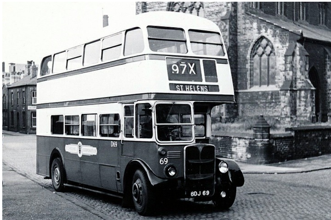
1950 AEC Regent III No. D69 (BDJ69) with London-style Park Royal 56-seat bodywork. (LTHL collection).
