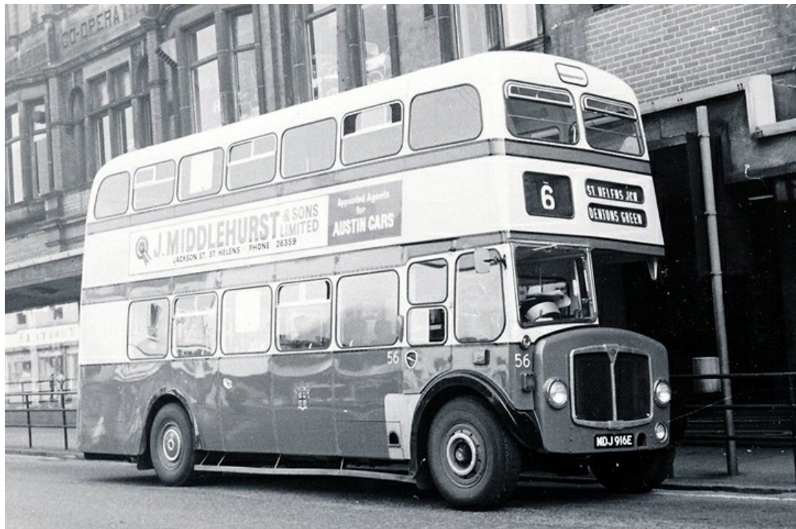
No. 56 (MDJ916E), a 1967 AEC Regent V with MCCW 65-seat bodywork. It passed to Merseyside PTE in 1974. (LTHL collection).
