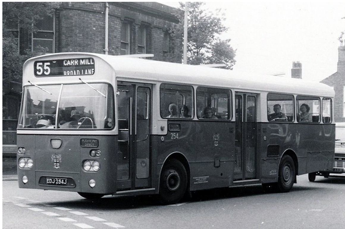
1971 AEC Swift No. 254 (EDJ254J) carried a Marshall 44-seat dual-door body. (LTHL collection).
