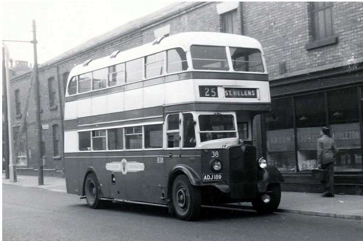
B38 (ADJ189) was a 1948 AEC Regent II with East Lancs 53-seat lowbridge bodywork. It was withdrawn in 1958. (LTHL collection).
