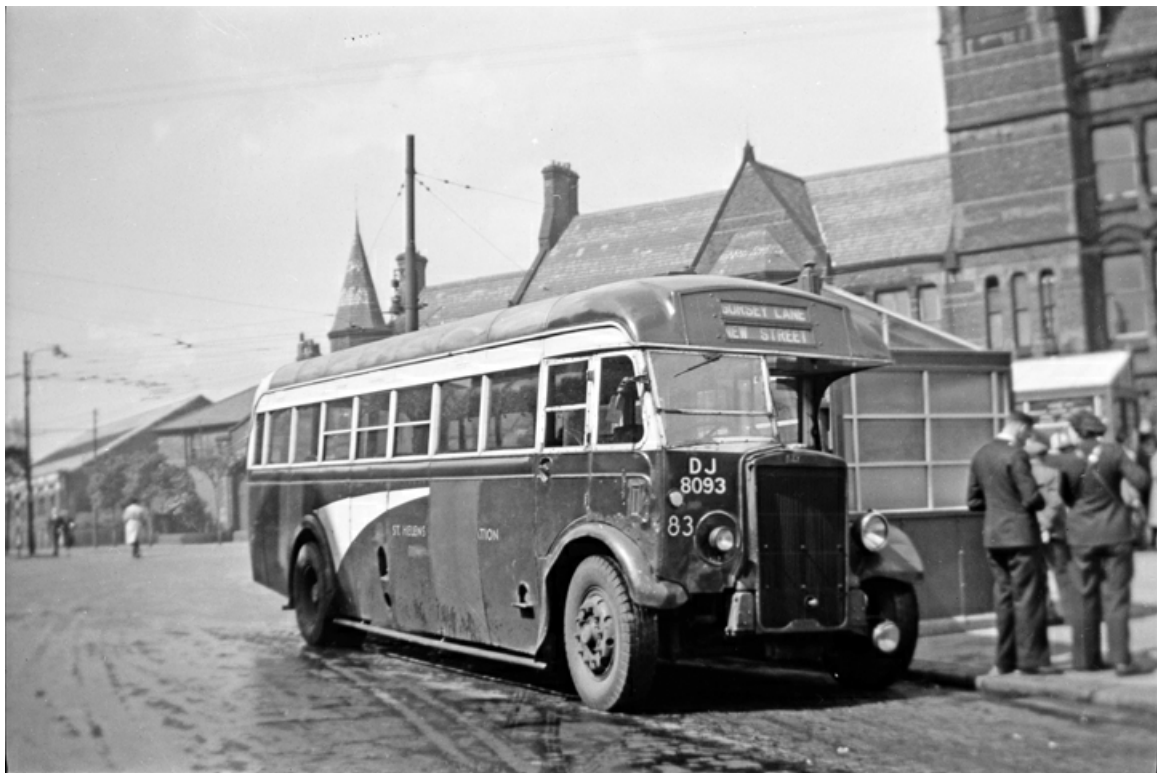
No. 83 (DJ8093) was a 1938 Leyland TS8c with Leyland B32F bodywork seen prior to 1948 when it was re-numbered 249. (Bus Archive)
