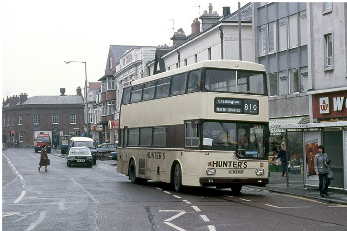
No. 64 (OTN446R) was a 1977 Scania BR111DH with MCW 76-seat bodywork, one of three acquired for service from Tyne & Wear PTE in 1986. (John Law).
