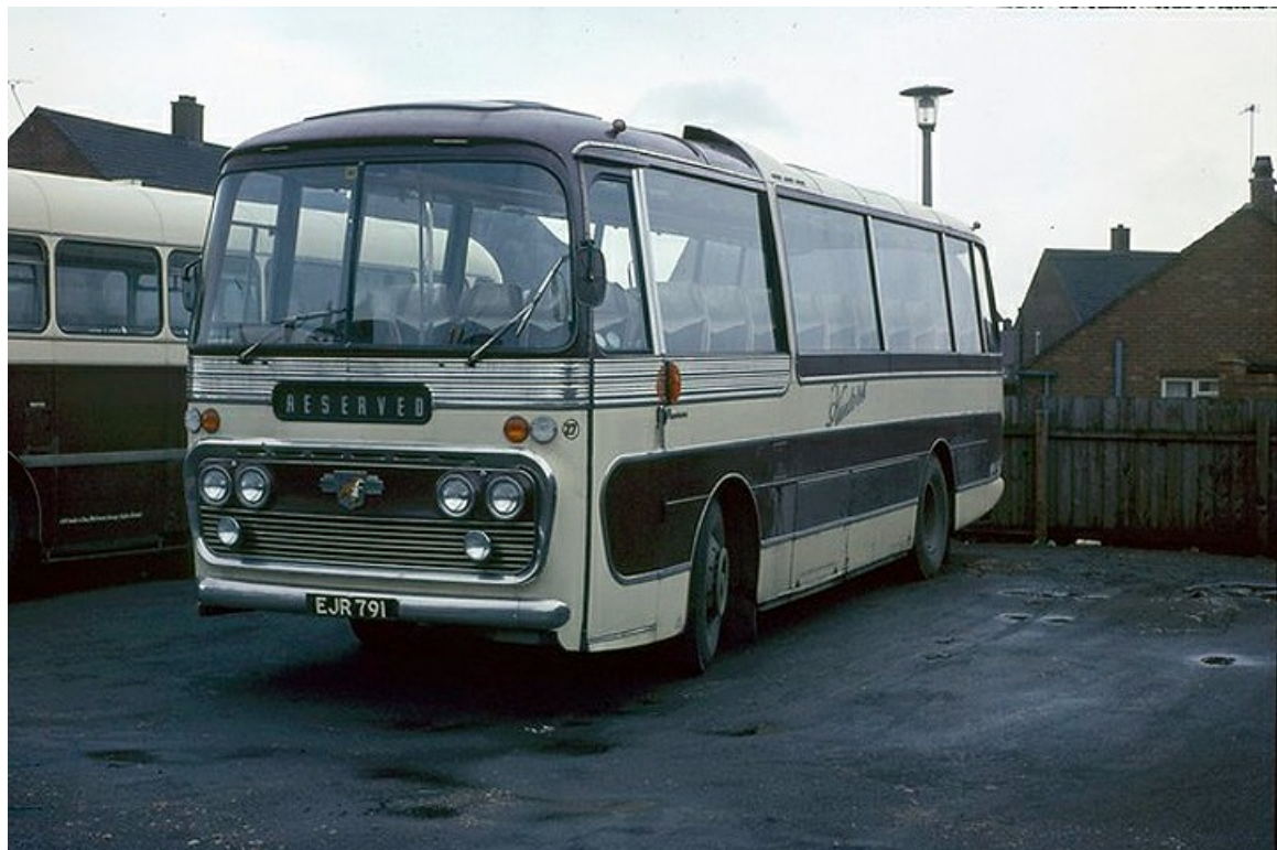
No. 27 was a 1952 Leyland PSU1/15, originally with Burlingham 41-seat centre-entrance bodywork, but seen here after being re-bodied by Plaxton with this 43-seat coach body. (Richard Simons).
