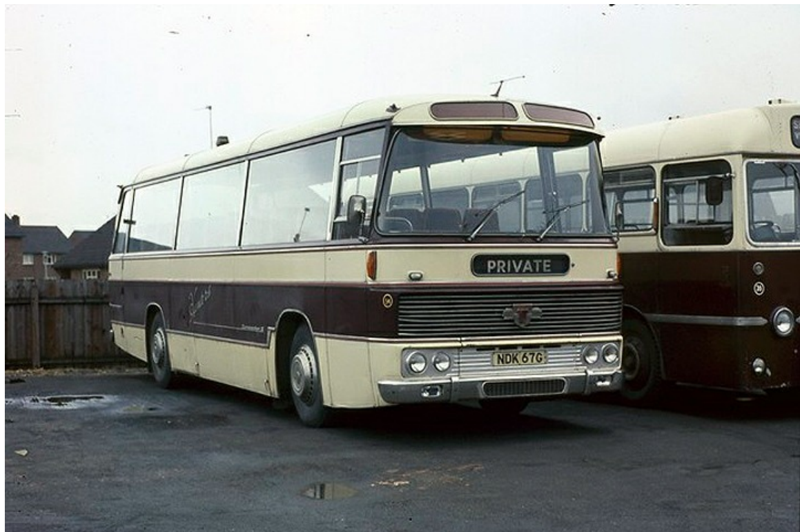
No. 34 (NDK67G) was a second-hand purchase from Pickup of Norden in 1975 and was a 1969 Leyland PSU4/3R with Duple Northern 45-seat coachwork. (Richard Simons).
