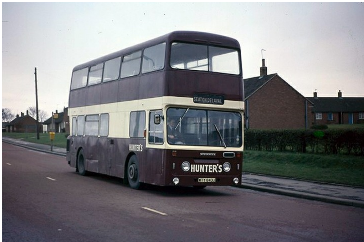
No. 30 (WTY843J) was Hunter's third double-decker, a 1971 Leyland PDR1A/1R 'Atlantean' with Roe 72-seat dual door bodywork. (Richard Simons).
