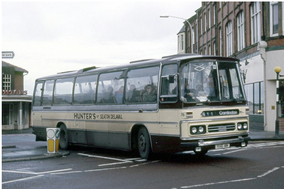
Ex-Burnley & Pendle Duple-bodied 1974 Leyland PSU3E/4R 'Leopard' No. 76 (YHG4N) heads towards Cramlington on the extended stage service. (John Law).
