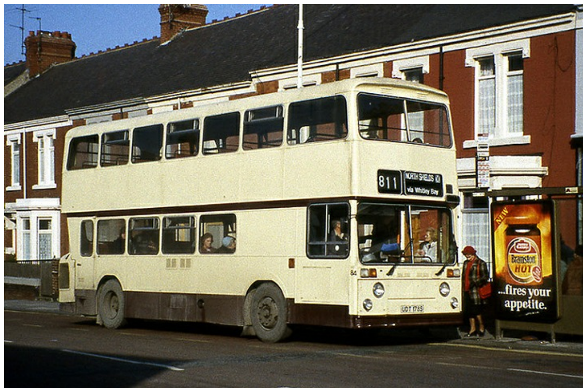
No. 84 (UDT178S), a 1978 Leyland AN68/1R 'Atlantean' with East Lancs dual door 74-seat bodywork. (John Law).
