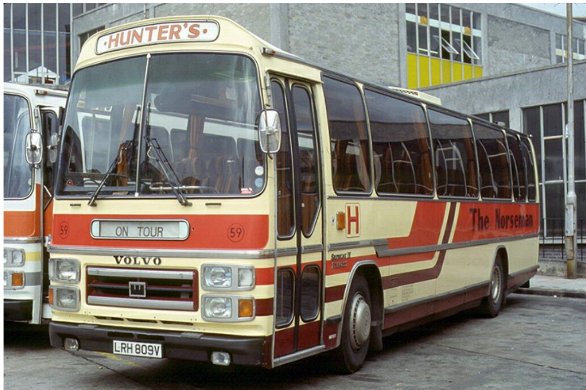
No. 59 (LRH809V) was a 1980 Volvo B58-56 with Plaxton 53-seat coachwork that had been new to Holt, Newport. (Cliff Essex).
