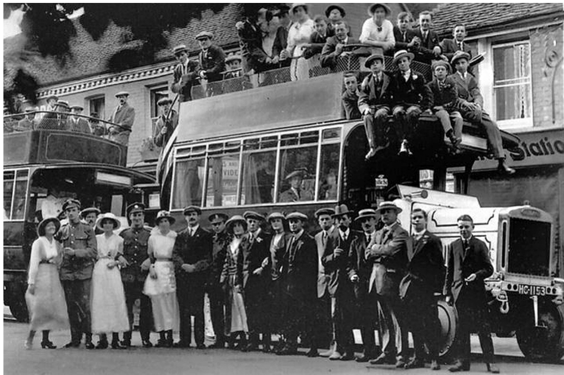
HC1153 was a Leyland War Subsidy chassis that received the Leyland 38-seat body from the former No. 33 (HC589 - see previous page) in 1916. It was later rebuilt to single-deck by Eastbourne in 1927-28. (LTHL collection).
