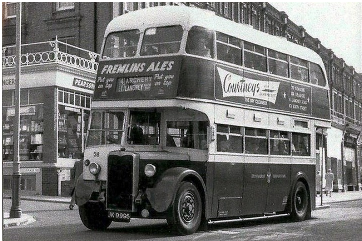
In 1949 Eastbourne purchased nine Crossley DD42/5's with East Lancs 50-seat bodywork. This is No. 38 (JK9995). (LTHL collection).
