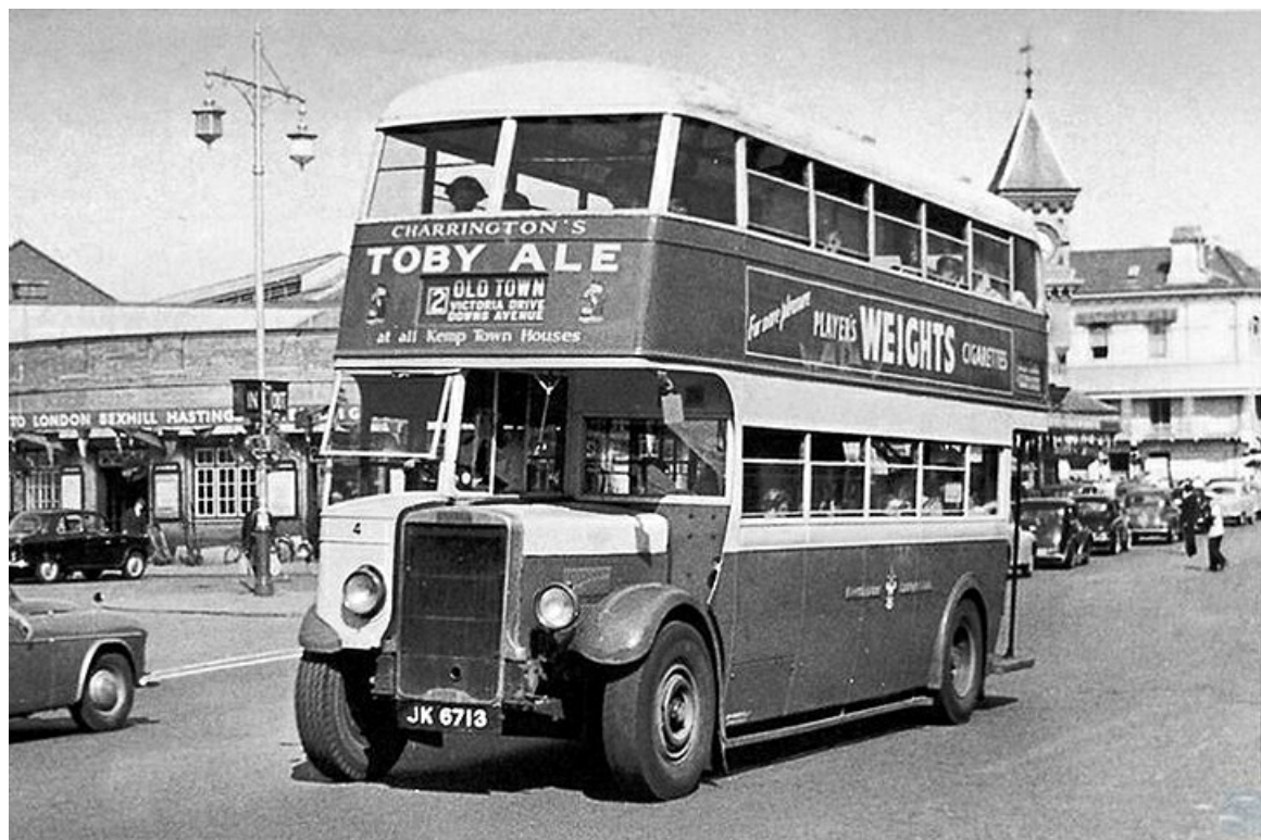
No. 4 (JK6713) was a 1937 Leyland TD5c with Leyland 48-seat bodywork that survived in the fleet until 1957. (LTHL collection).
