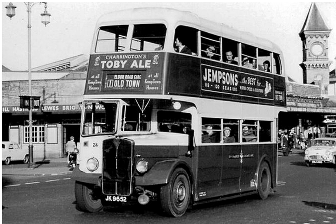
No. 24 (JK9652) was a 1947 Weymann 50-seat bodied AEC Regent III on the Old Town route. (LTHL collection).
