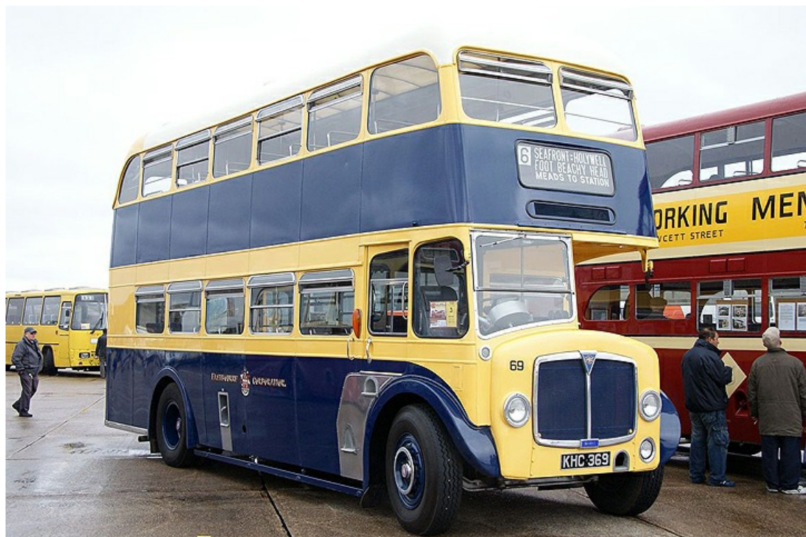
Another preserved vehicle is No. 69 (KHC369) a 1963 AEC Regent V with East Lancs 60-seat bodywork, representative of the vehicles purchased in the early 60's. (LTHL collection).
