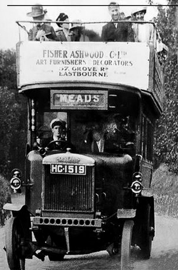
No. 48 (HC1519) was a 1919 War Subsidy Leyland lorry chassis fitted with an open-top 32-seat body by an unknown maker. It was later fitted with a Brush 45-seat body and was not withdrawn until 1936. (LTHL collection).
