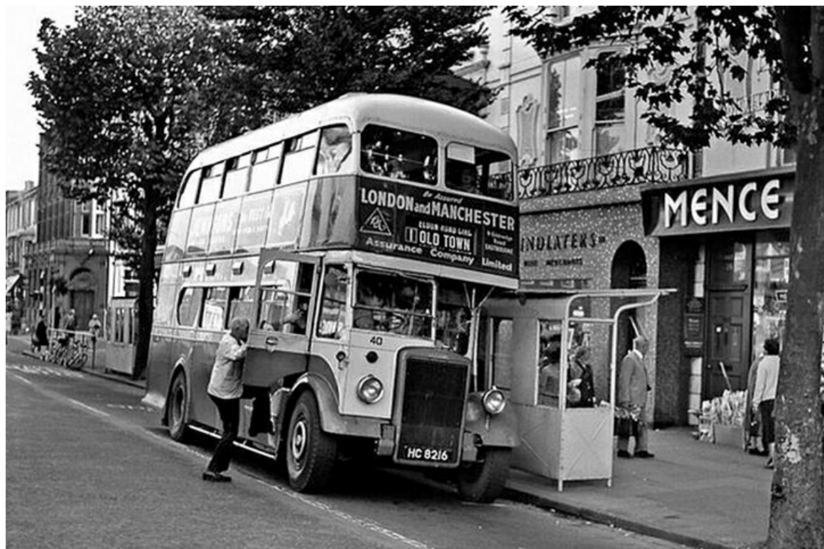
No. 40 (HC8216) was a 1948 Leyland PD2/1 with Air Dispatch (the forerunner of Bruce Coachworks) 52-seat bodywork on East Lancs frames. (LTHL collection).
