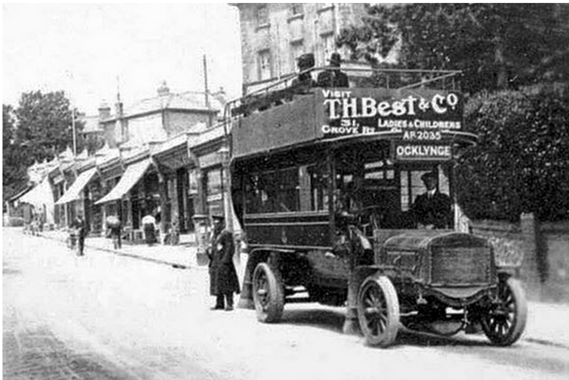
No. 26 (AP2035), a 1905/06 De Dion with 32-seat bodywork by an unknown builder that came second-hand from the Associated Omnibus Company of London, makes its way along a car-free street to Ocklynge. (LTHL collection).
