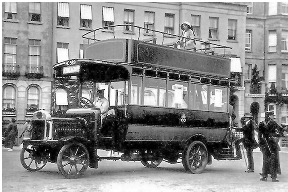
HC589 was a 1914 Leyland B (No. 33) that spent just 4 months with Eastbourne Corporation before its chassis was impressed by the War Department - its Leyland 38-seat open-top body was transferred to a later vehicle. (LTHL collection).
