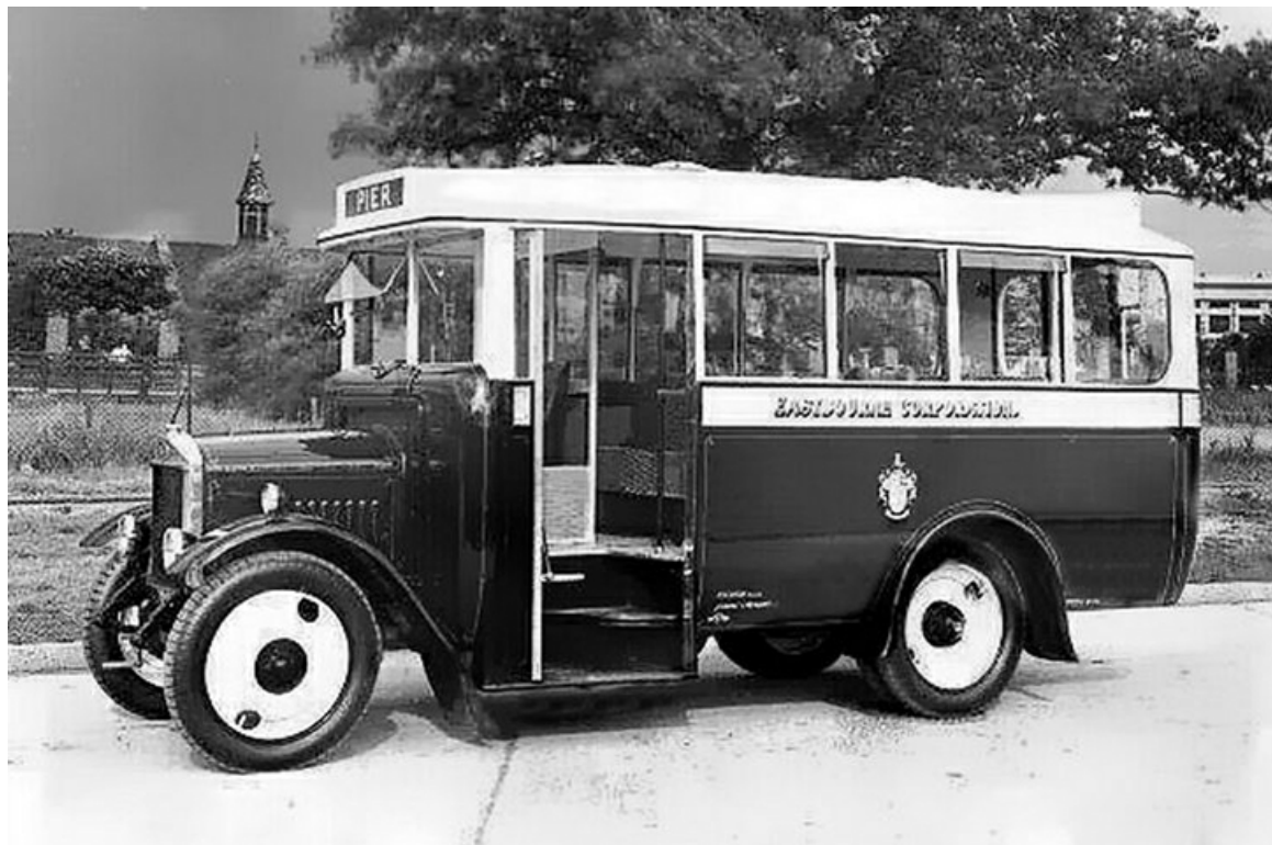
One of three Dennis 30cwt buses purchased for use on the sea front service in winter. They had Hall Lewis 14-seat bodywork. (LTHL collection).
