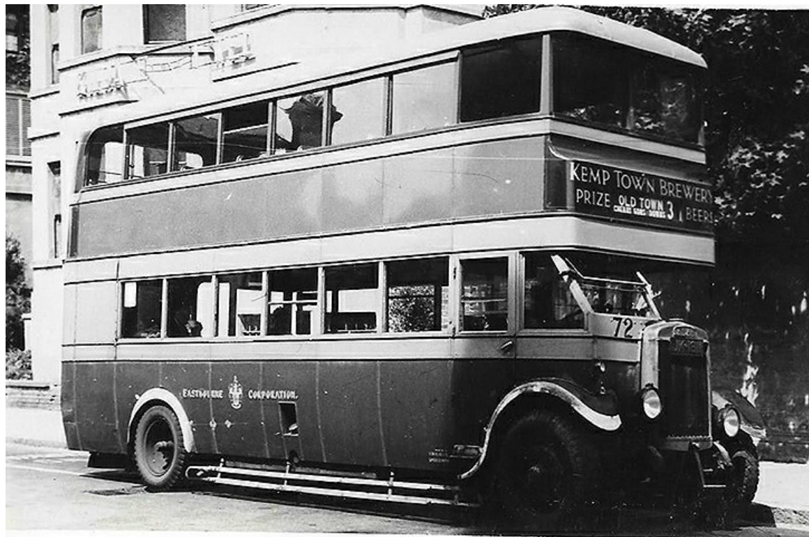
1931 Leyland TD1 No. 72 (JK1811) with Leyland 48-seat bodywork on the Old Town route. It was withdrawn in 1948. (W. J. Haynes).
