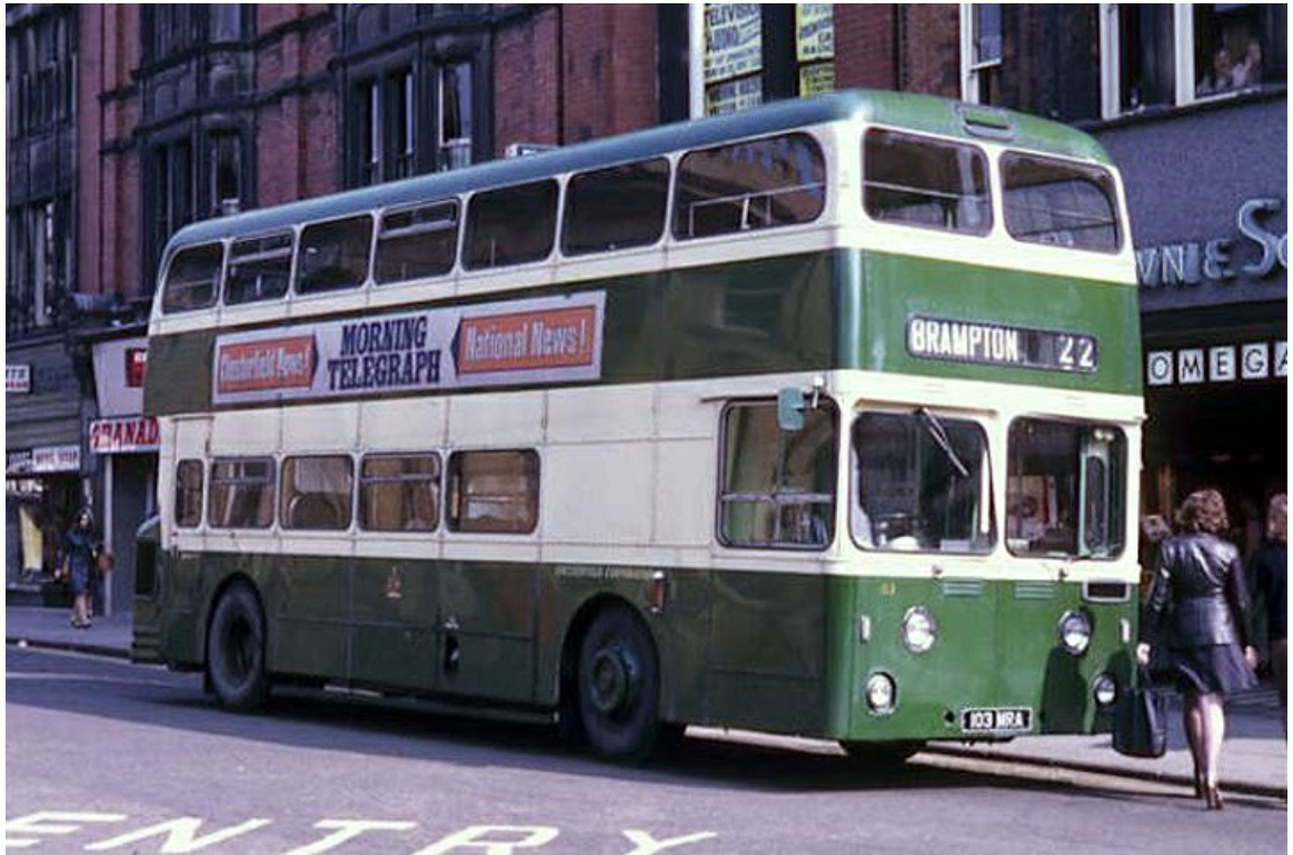
Chesterfield's first rear-engined vehicles arrived in 1960. They were Leyland PDR1/1's with Weymann 73-seat lowbridge bodywork. No. 103 (103MRA) is seen in Stephenson Place in 1974. (George Cropper courtesy Donald Hudson).
