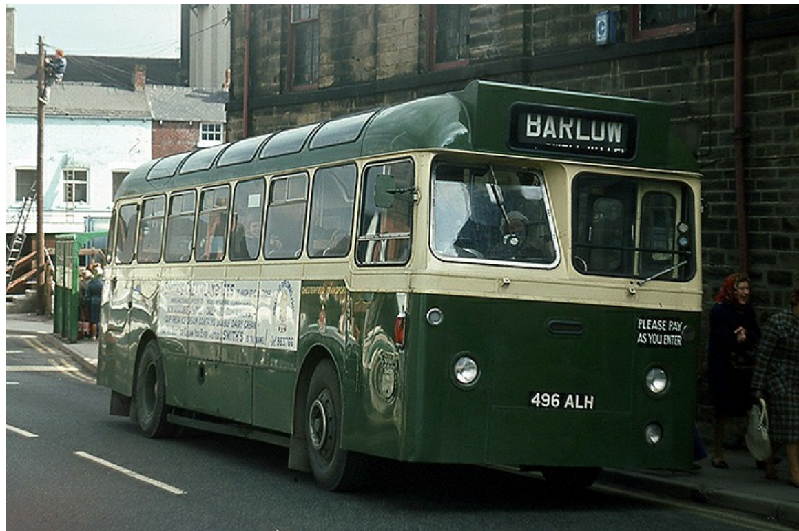
No. 19 (496ALH) was a 1960 AEC Reliance with Willowbrook dual door bodywork, one of three acquired from London Transport in 1963. (LTHL collection).
