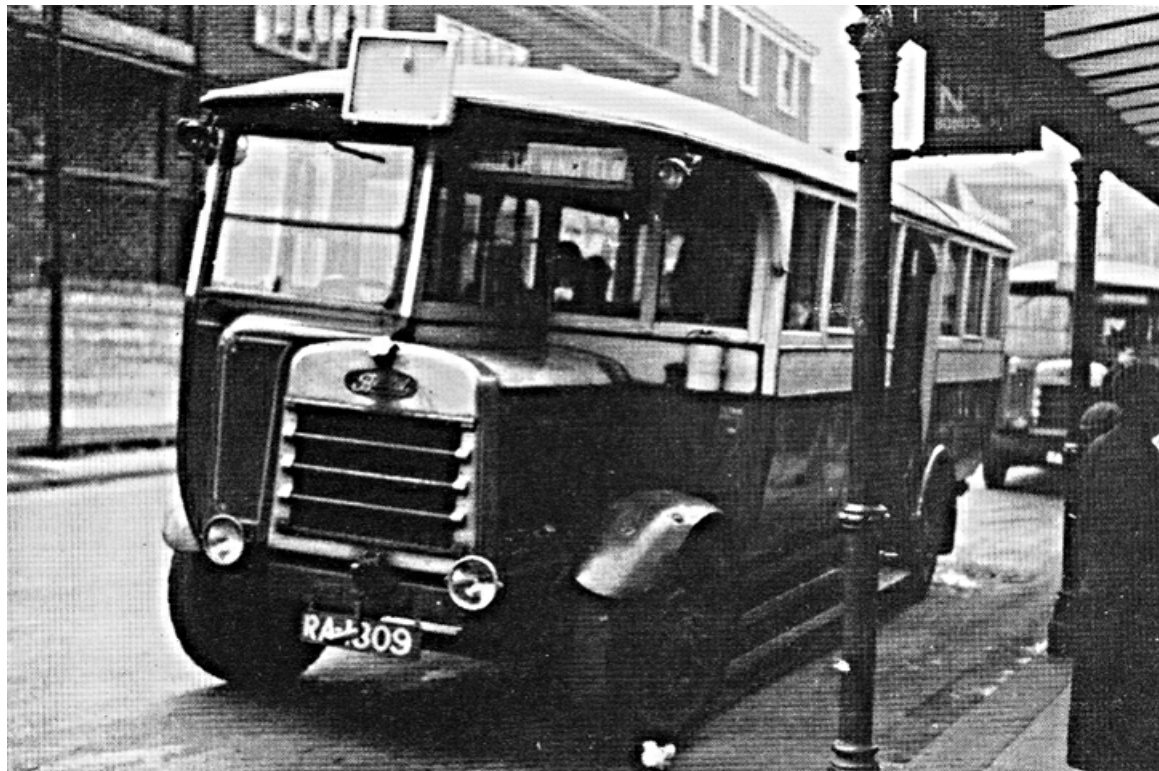
No. 40 (RA1809) a 1927 Bristol B with Reeve & Kenning 30-seat centre-entrance bodywork. (LTHL collection).
