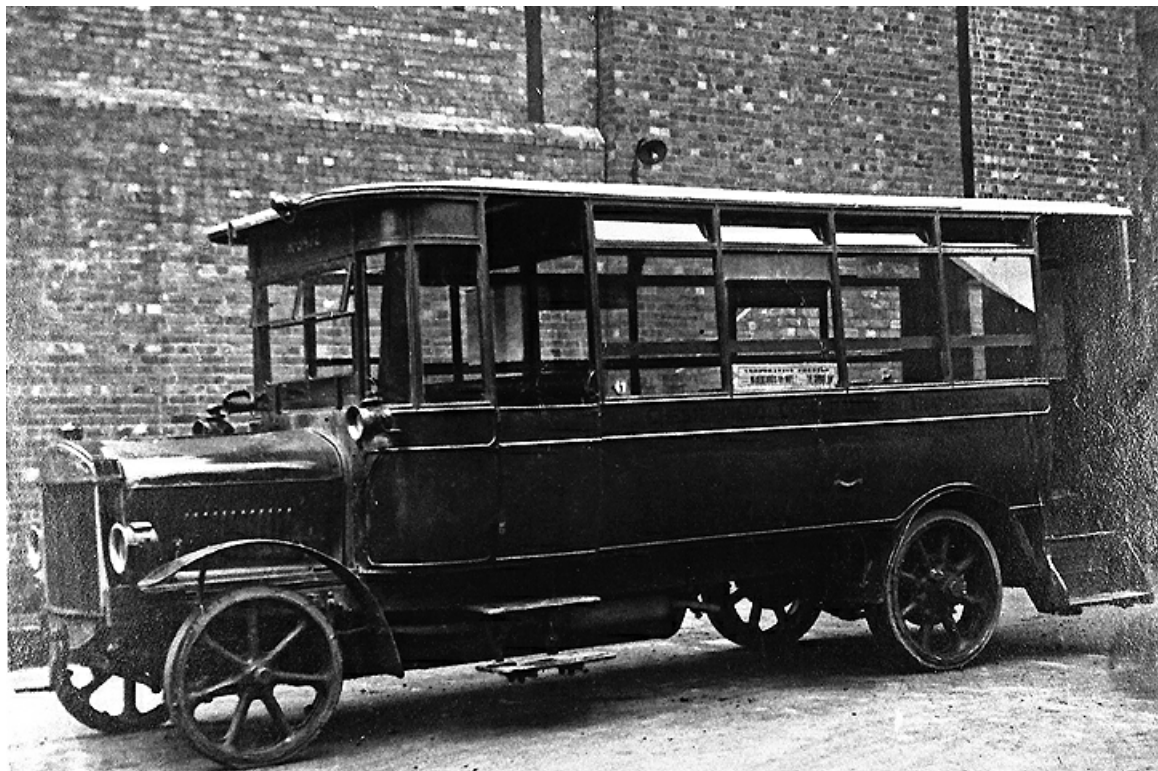
No. 37 (R3472) was a 1919 Tilling-Stevens with Bartle B28R bodywork and was withdrawn in 1927. (Bus Archive).
