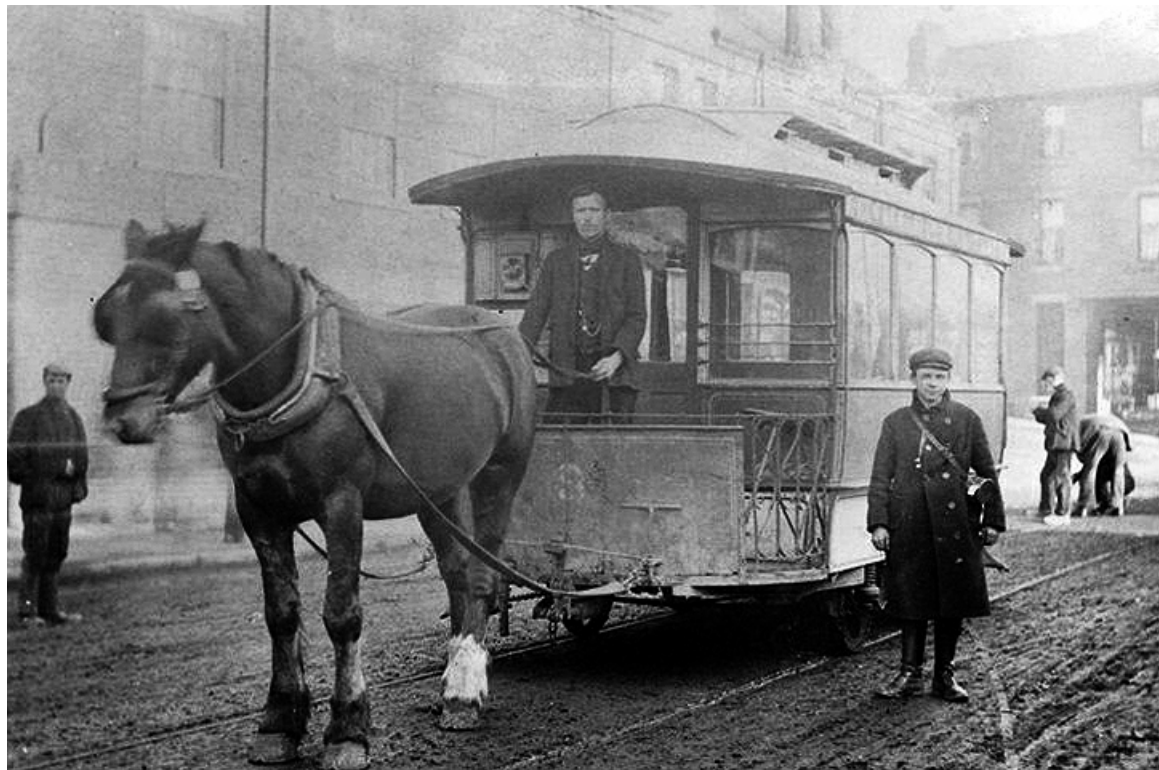
No. 8 was purchased in 1899 and was a one-horse single-deck saloon seating 16 built by George Milnes of Birkenhead. (Tramway & Light Railway Society).
