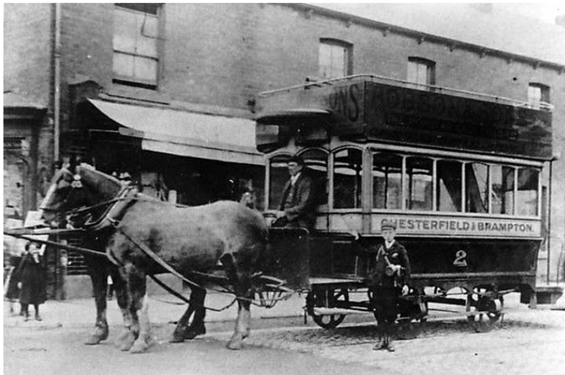
No. 2 was an 1882 Ashbury Railway & Carriage Company built two horse double-deck seating 32. (National Tramway Museum).
