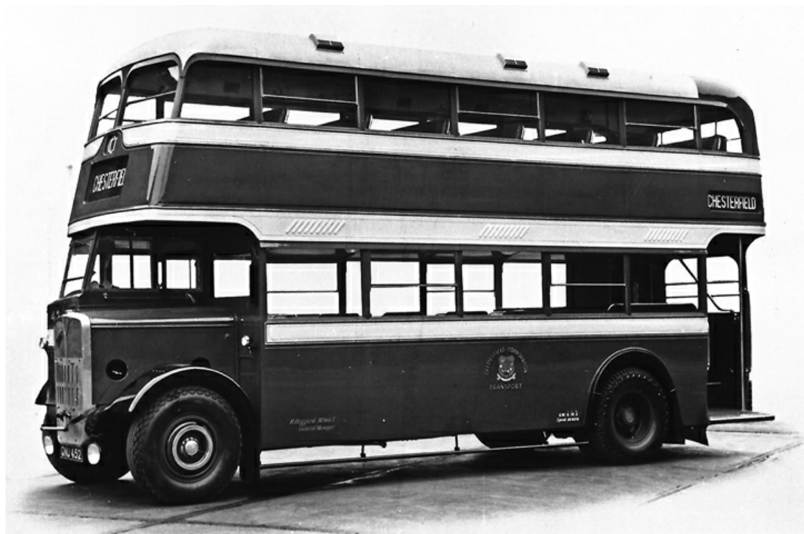
AEC chassis were not common in the Chesterfield fleet. No. 43 (GNU452) was an AEC Regent dating from 1939 and carried a Metro-Cammell L26/26R body. (Bus Archive).
