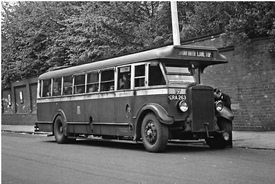
Leyland TS7c No. 37 (CRA263) carried a Metro-Cammell B32R body and dated from 1936. (Bus Archive).
