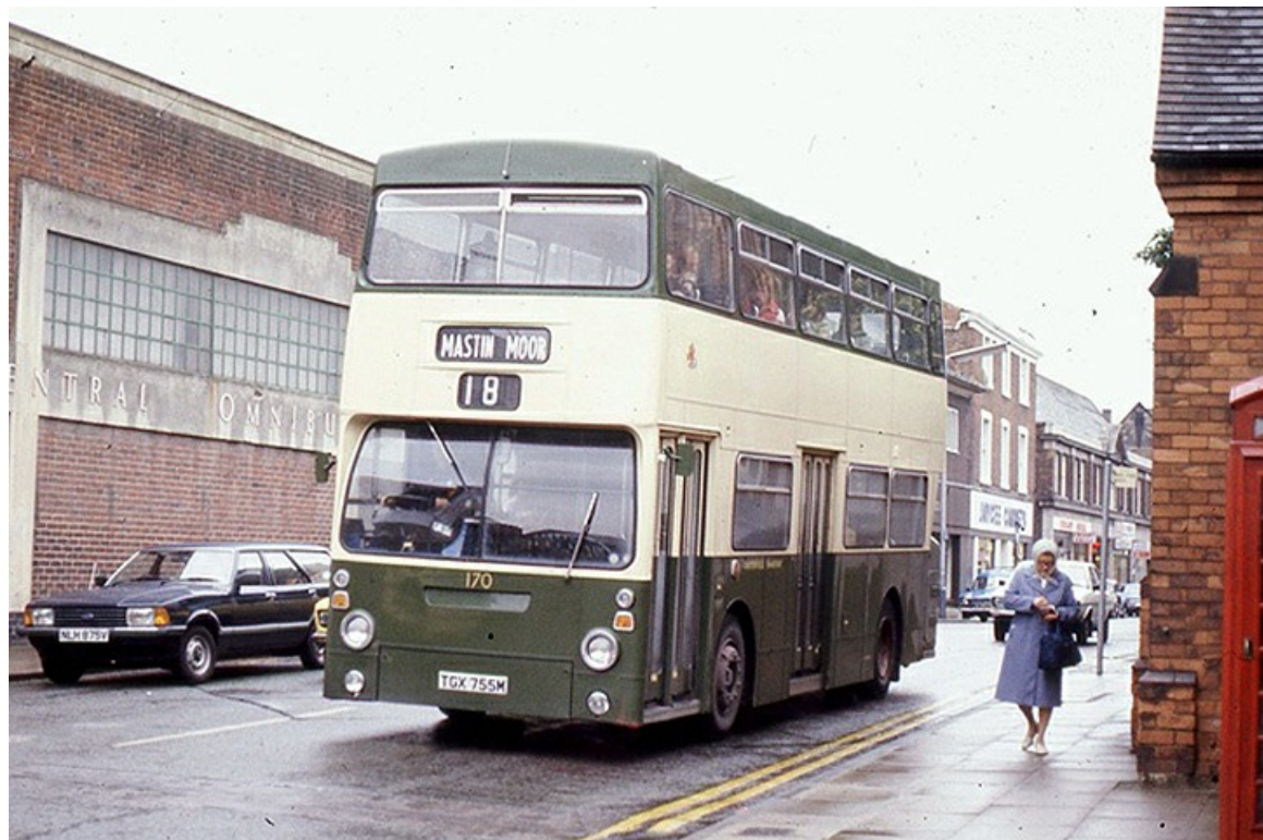
No. 170 (TGX755M) was another ex-London Transport Daimler CRL6 with Park Royal bodywork, dating from 1973 and acquired in 1981. (Mike Beamish).
