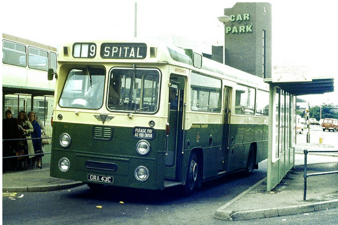
On route 9 to Spital is Neepsend 42-seat dual-door bodied 1965 AEC Reliance No. 43 (GRA43C). (Steve Guess).
