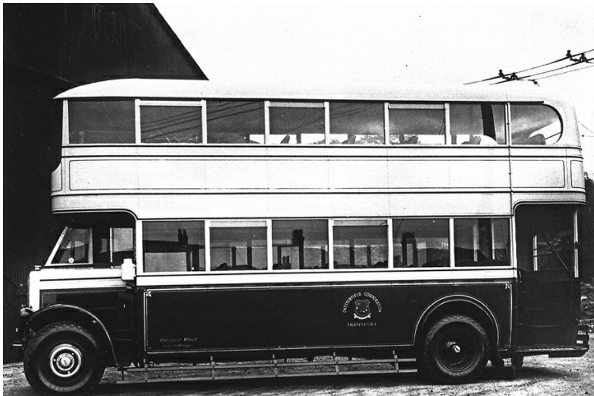
No. 41 (RB4884) was the first numerically of six Leyland TD1's with Leyland L24/24R bodywork delivered in 1931. (Bus Archive).
