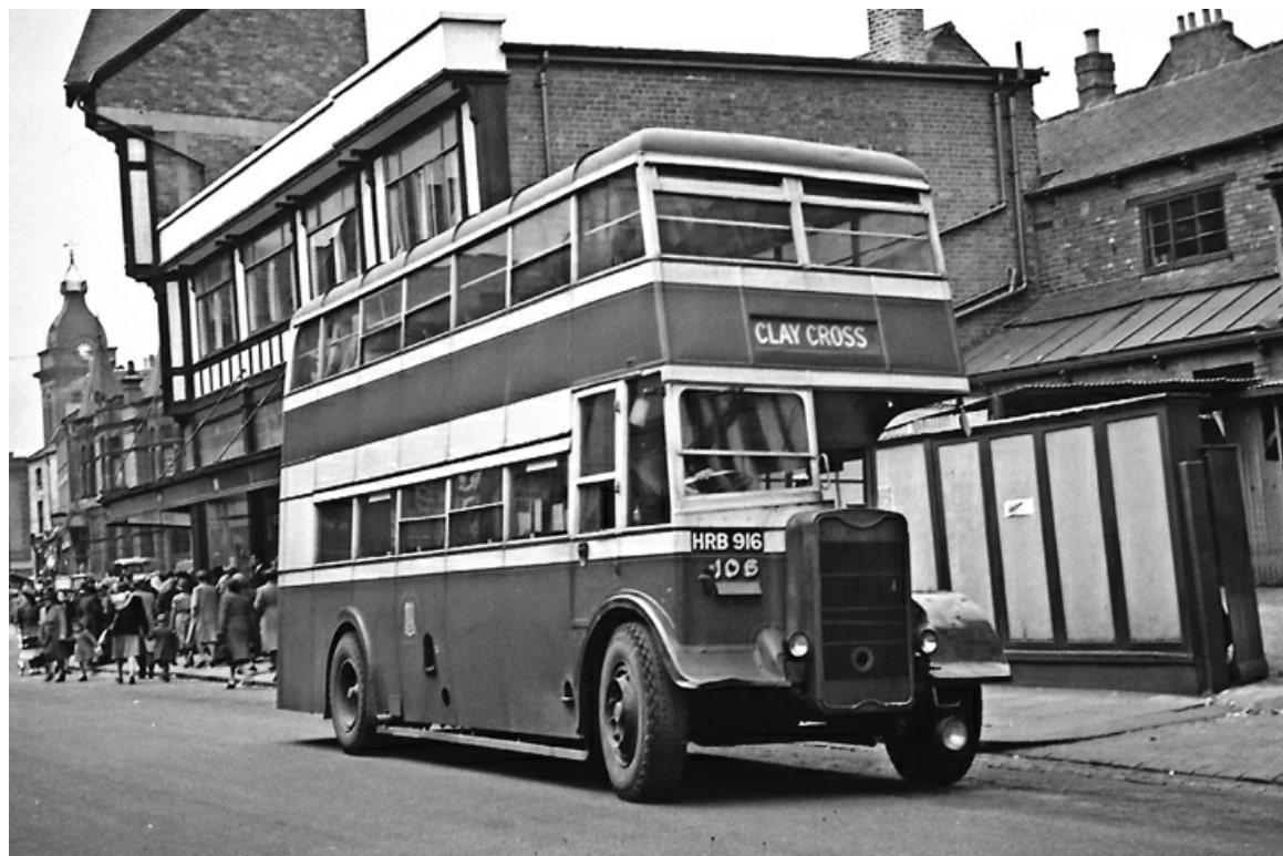
Guy Arabs made their almost obligatory appearance in the Chesterfield fleet during the War. This is No. 106 (HRB916) a 1945 Guy Arab II with Weymann L27/28R bodywork. (Bus Archive).
