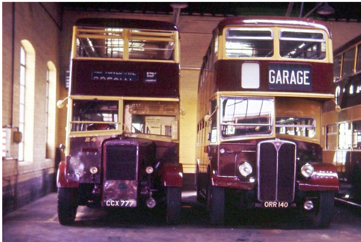
Side by side in the depot are No. 24 (CCX777) an ex-Huddersfield Daimler CWA6 with Duple L27/28R bodywork dating from 1945 and No. 21 (ORR140) a 1954 AEC Regent III with Willowbrook L27/28R bodywork. (John Huddleston).
