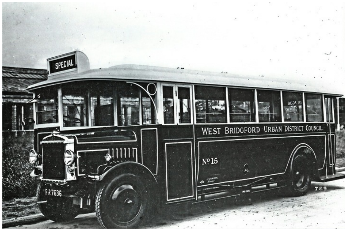
No. 15 (RR7636) was an ADC 416A with Hall Lewis B32D bodywork dating from 1927. (Bus Archive).
