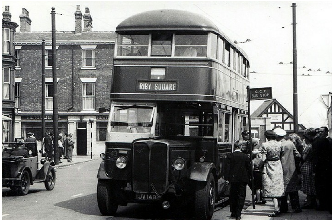
No. 43 (JV1482), a 1932 AEC Regent with Roe 48-seat centre-entrance bodywork. It was rebuilt by Grimsby in 1948 and withdrawn in 1950. (LTHL collection).
