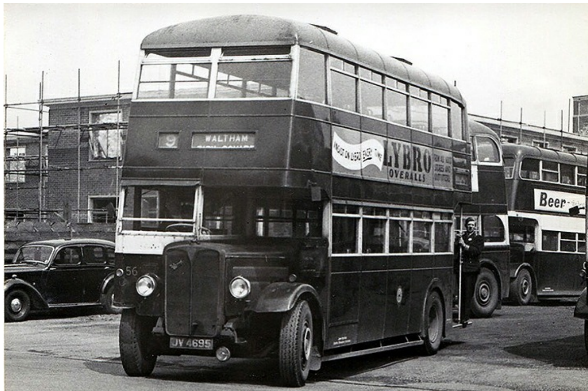
No. 56 (JV4695) a 1936 AEC Regent with Northern Coachbuilders 56-seat bodywork, which had replaced its original centre-entrance body in 1945 after it had been destroyed by enemy action. (LTHL collection).
