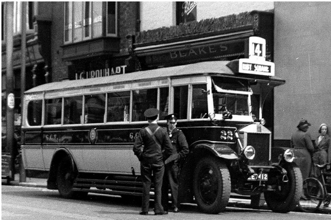
No. 22 (EE7412), the second of the 1927 Albion PM28's showing the later modification of route and number indicators above the driver's cab. (LTHL collection).
