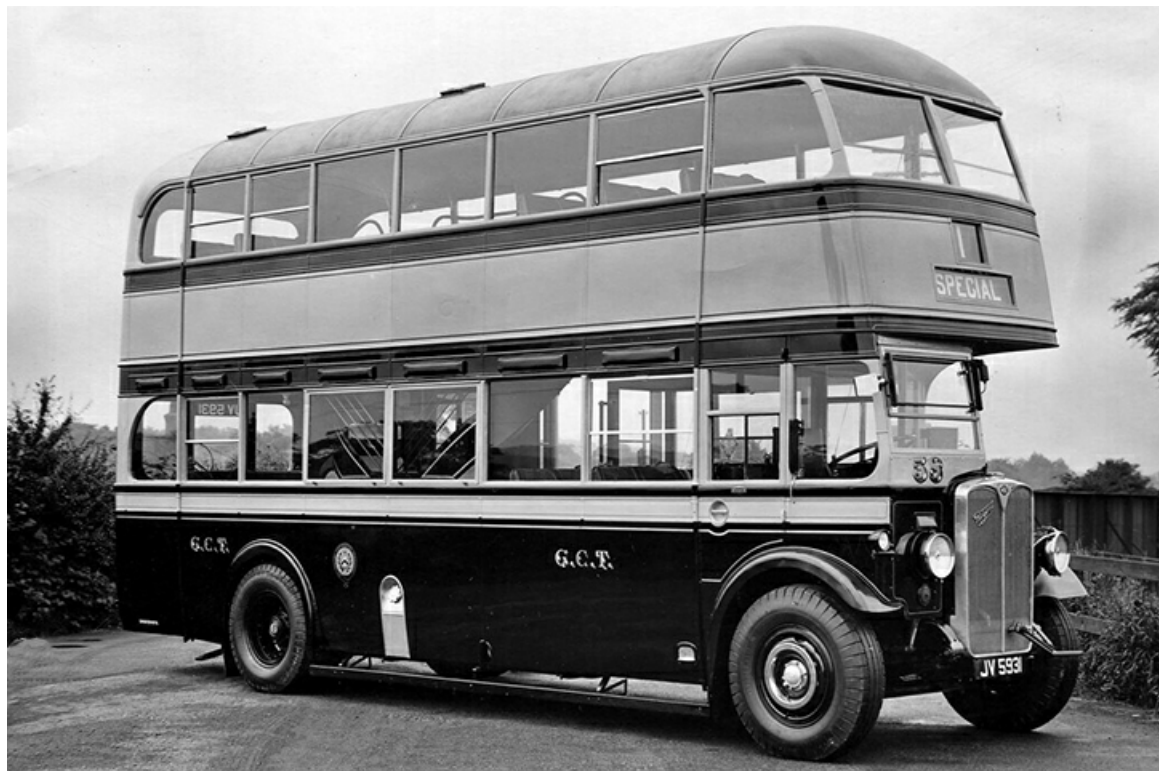
No. 58 (JV5931), seen here when new, was a 1937 AEC Regent with Roe 48-seat centre-entrance bodywork. (LTHL collection).
