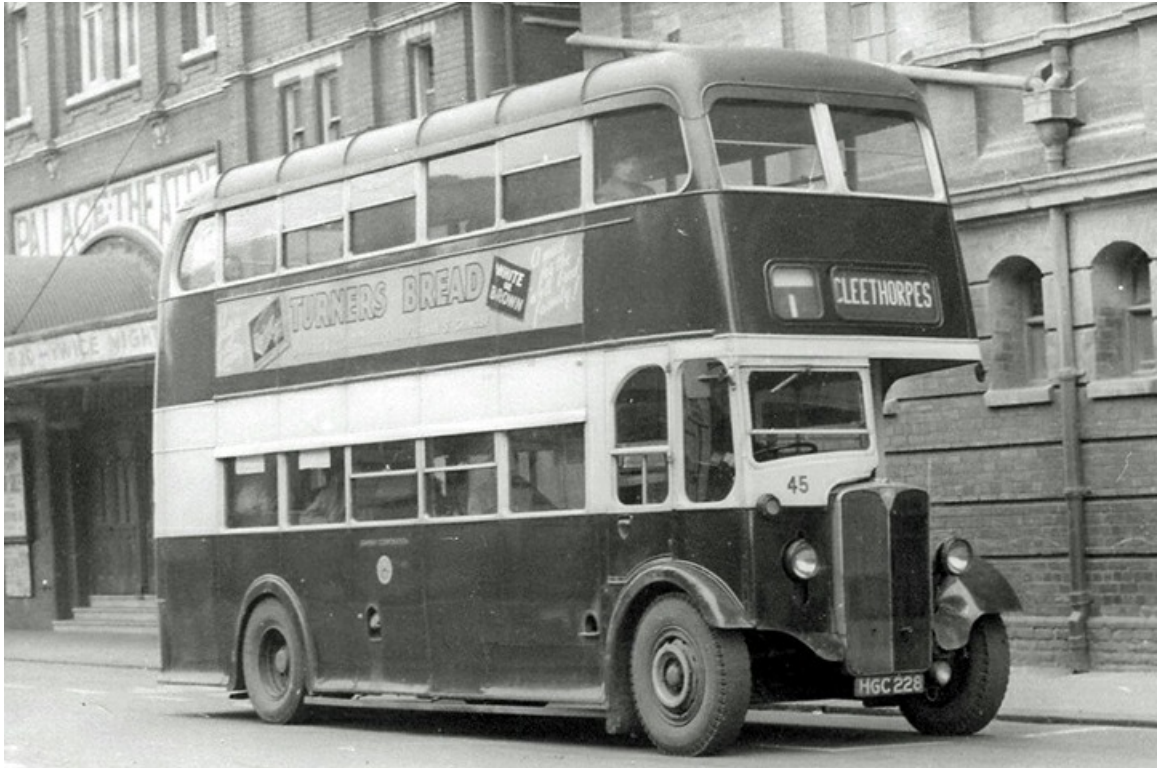
No. 45 (HGC228) was one of six AEC Regent's, new in 1946, purchased from London Transport in 1955. It had a Weymann 56-seat body. (LTHL collection).
