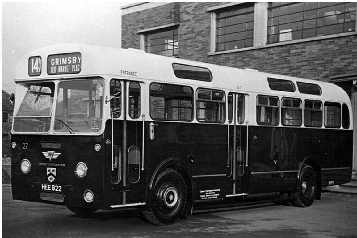
Grimsbys's last purchases before the merger with Cleethorpes were 6 AEC Reliance MU3RV chassis. This is No. 27 (HEE822) with Roe 41-seat dual entrance/exit bodywork, seen here at the Roe works before delivery. (LTHL collection).
