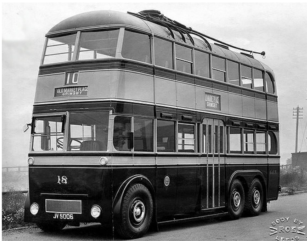
An official photograph of No. 18 (JV5006), a 1936 AEC 663T with Roe 58-seat centre-entrance bodywork. (LTHL collection).
