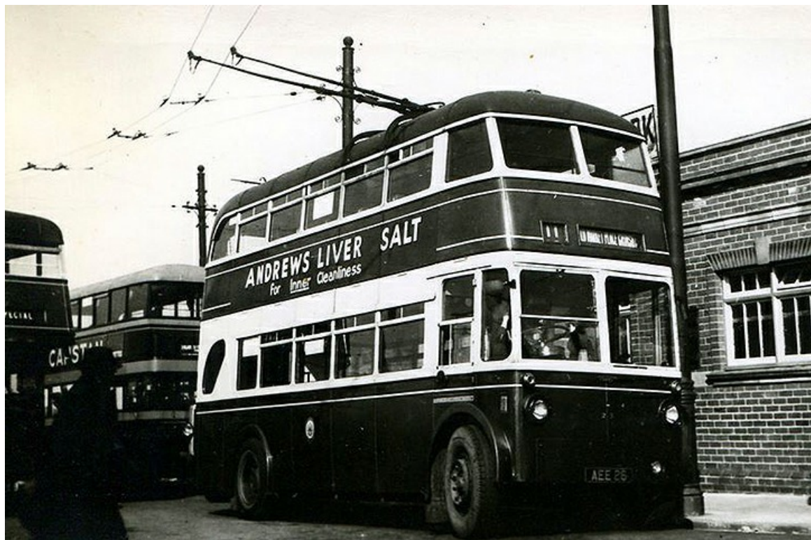
Grimsby's final trolleybuses were purchased in 1947 and No. 23 (AEE26) is one of them. It was a Karrier W with Roe 56-seat bodywork. (LTHL collection).
