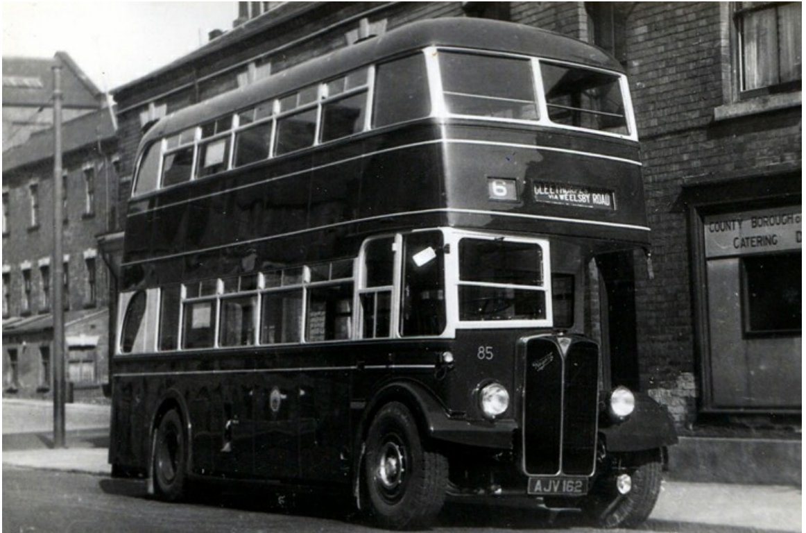
No. 85 (AJV162) a 1948 AEC Regent III with Roe 56-seat bodywork seen here on the through route to Cleethorpes via Weelsby Road. (LTHL collection).
