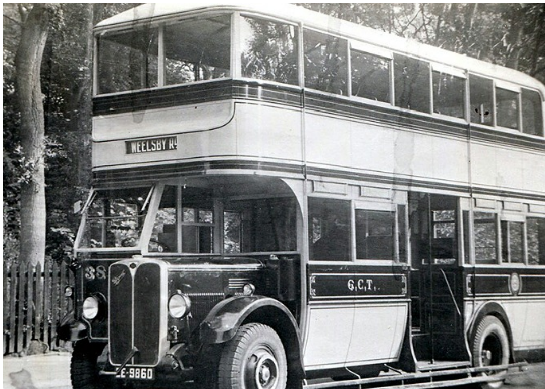
Grimsby's first double-deck bus was No. 38 (EE9860), a 1930 AEC Regent with Roe 48-seat centre-entrance bodywork. It had the distinction of being the first centre-entrance double-decker in Great Britain. (LTHL collection).
