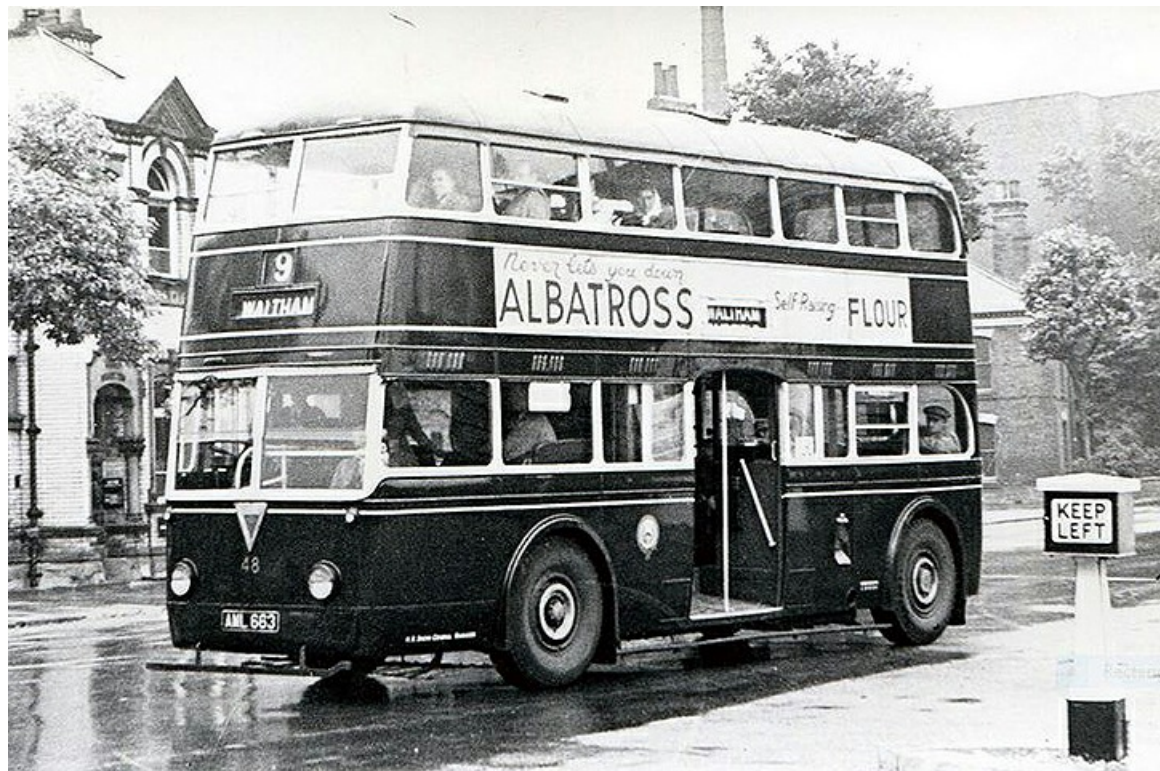
No. 48 (AML663), a 1933 AEC Q was built to Grimsby's specifications with centre-entrance. It survived long enough to pass to Grimsby-Cleethorpes JTC in 1/1/57 albeit as a withdrawn vehicle. (LTHL collection).
